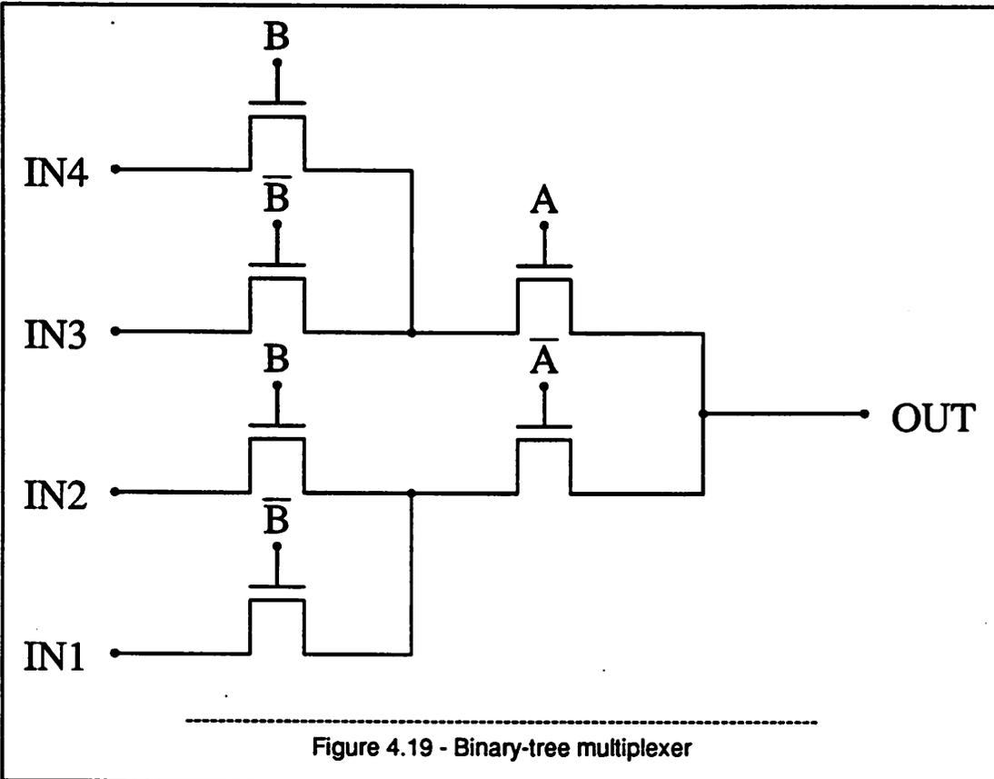
$$R_{on} = \frac{1}{k' \frac{W}{L} (V_{gs} - V_t)} \quad (4.28)$$
