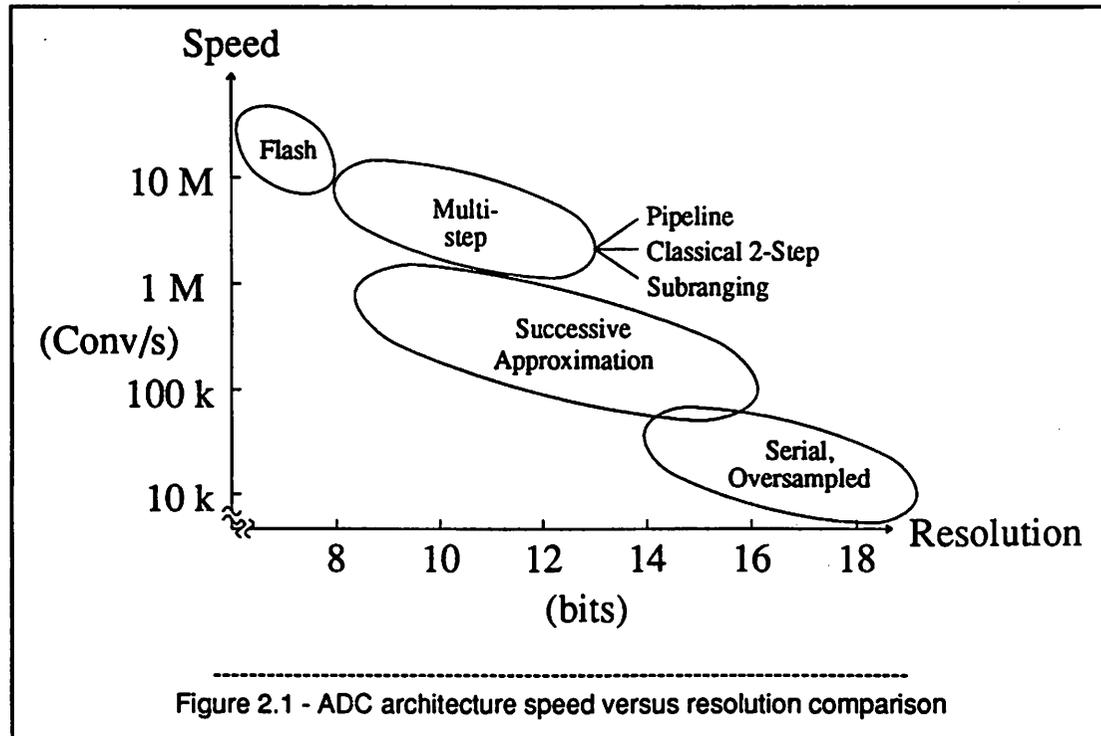
Video ADCs fall into the 8 to 10-bit resolution and 10 to 20 Msample/s conversion range. Although 8-bit resolution is acceptable for video at the consumer level, 10-bit resolution and its increased dynamic range is desired so that digital signal processing can be applied at the studio level and for HDTV.
