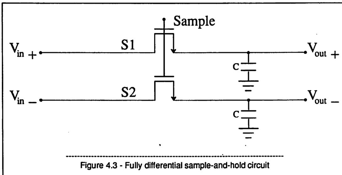
This method is quite effective. One main limitation is that of how well the technology can match the two switches. In an actual design it is expected that 80-90% of the charge injection error will be eliminated.
