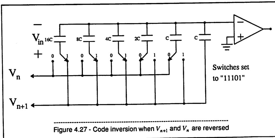
Thus for "odd" inputs to the multiplexer  $V_{n+1}$  and  $V_n$  are reversed and the preset code of each sub-ADC is complemented and 1 is added. Thus the sub-ADCs are now preset as shown in Figure 4.28.
