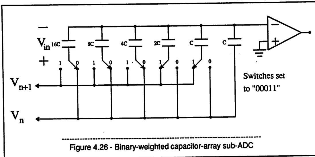
The key point is that it is preset for a code, say 00011. That means capacitors 16C, 8C, 4C and one of the units, C, are connected to  $V_n$  and capacitors 2C and C are connected to  $V_{n+1}$ . If the roles of  $V_{n+1}$  and  $V_n$  are reversed as shown in Figure 4.27 then 16C, 8C, 4C and 1 unit C are connected to  $V_{n+1}$  and capacitors 2C and C are connected to  $V_n$ . This configuration is preset to code 11101.
