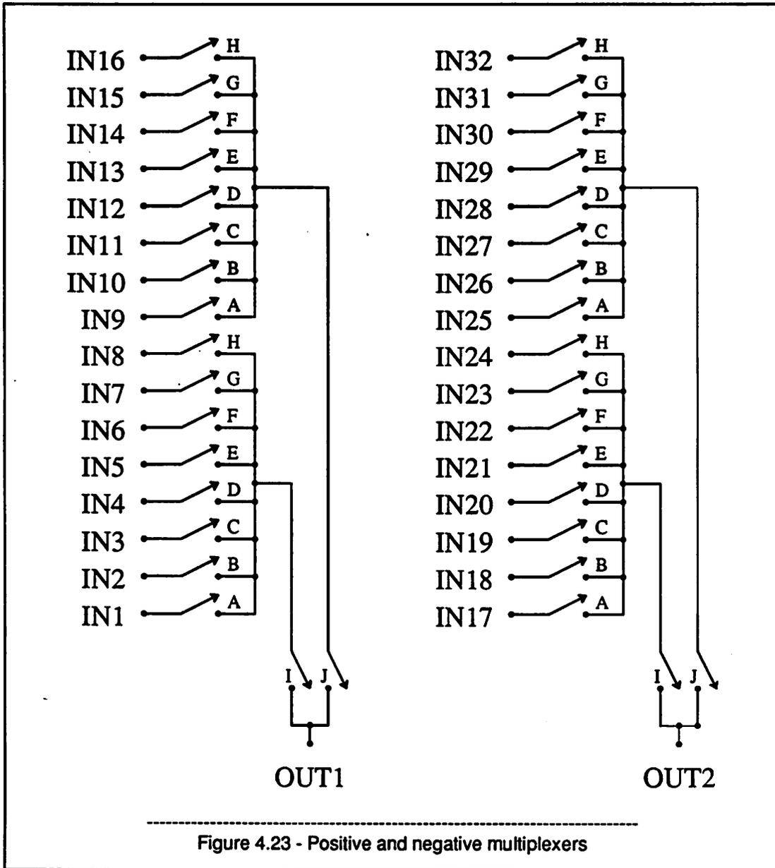
The next improvement is to notice that the multiplexer that selects the inputs for  $V_{n+1}$  selects taps that are always one tap away from the multiplexer that selects the  $V_n$  taps. Thus each multiplexer can again have half of the inputs (half of the parasitic loading capacitance) and select alternate taps as shown in Figure 4.24. (Note: 2 multiplexers are in Figure 4.24. 4 are needed.)
