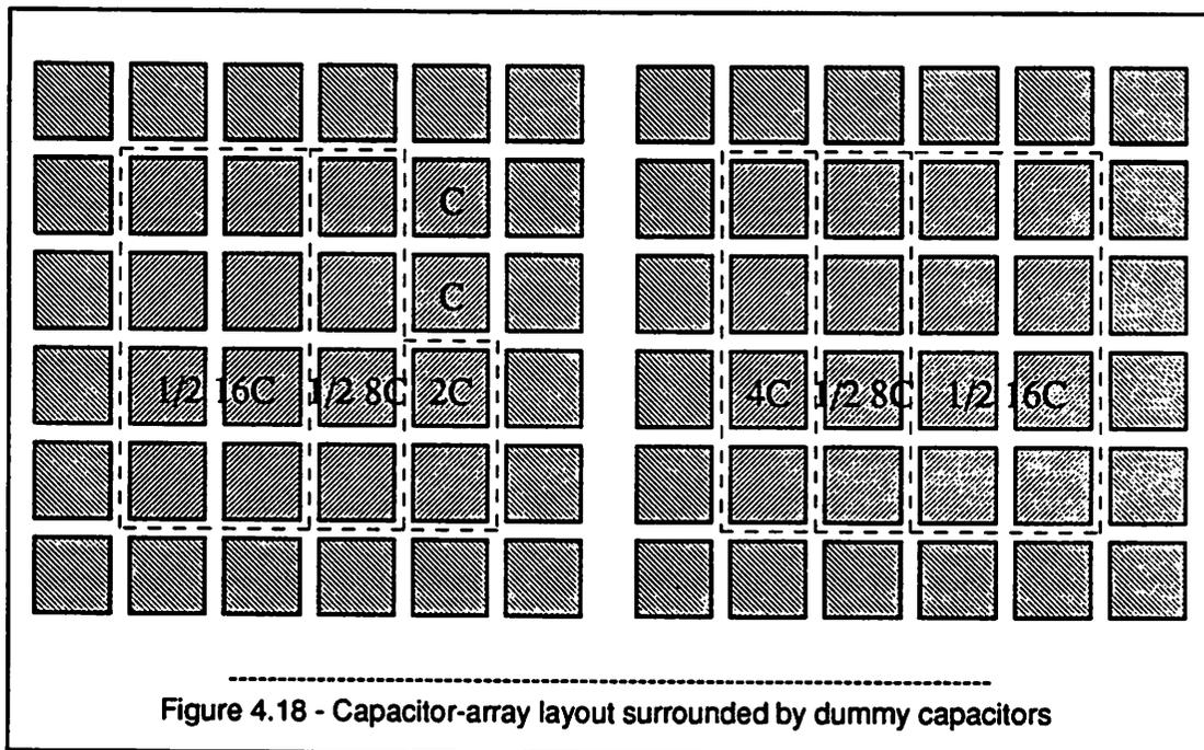
The capacitor construction is a bottom plate of metal1, a combination oxide and nitride dielectric and a metal2 top plate. The contact to the top plate is made with a via from metal2. Since only 8-bit accuracy is needed problems with nitride in the dielectric such as dielectric relaxation or residual polarization should not be significant.
