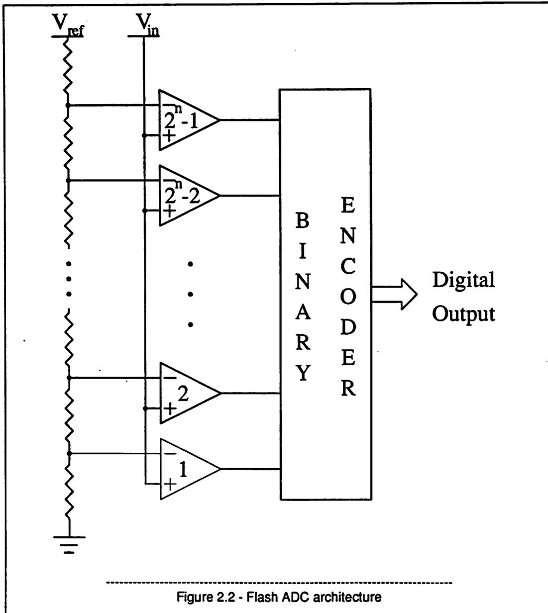
tors and encoding. (The comparators are usually the speed-limiting component.)
