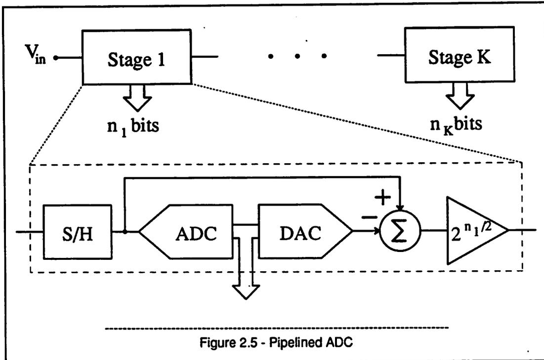
The pipelined ADC is actually an improved subranging ADC. While its operation is to subrange, the use of multiple stages operating concurrently leads to higher speed operation. One conversion is done each clock period. This however is not as fast as the flash converter since the flash converter offset cancels and makes one comparison per period the pipeline must do a sample and hold, a comparison, D/A conversion, subtraction and amplification each period.
