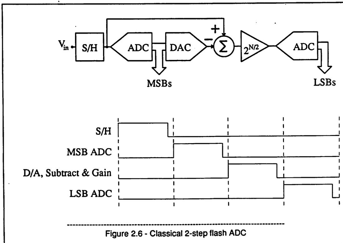
from the held input and the result is amplified. The fourth phase is the second step where the LSBs are converted. If there was a S/H after the gain stage this would be a 2-stage pipeline.
