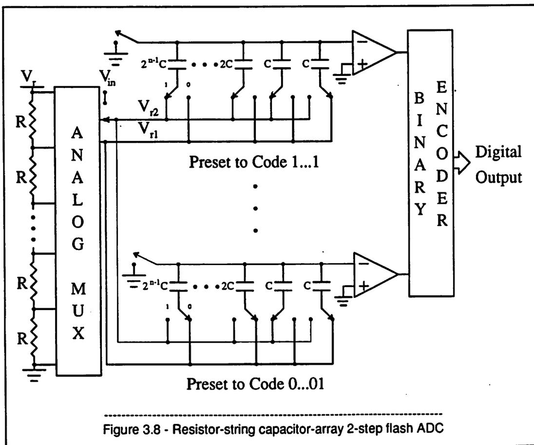
The operation proceeds in two steps. In the first step the input is sampled and a flash MSB decision is made using the resistor string. Then the LSBs are obtained by subdividing the voltages at the two resistor-string taps adjacent to the unknown input voltage with the capacitor arrays in a second-step flash decision.
