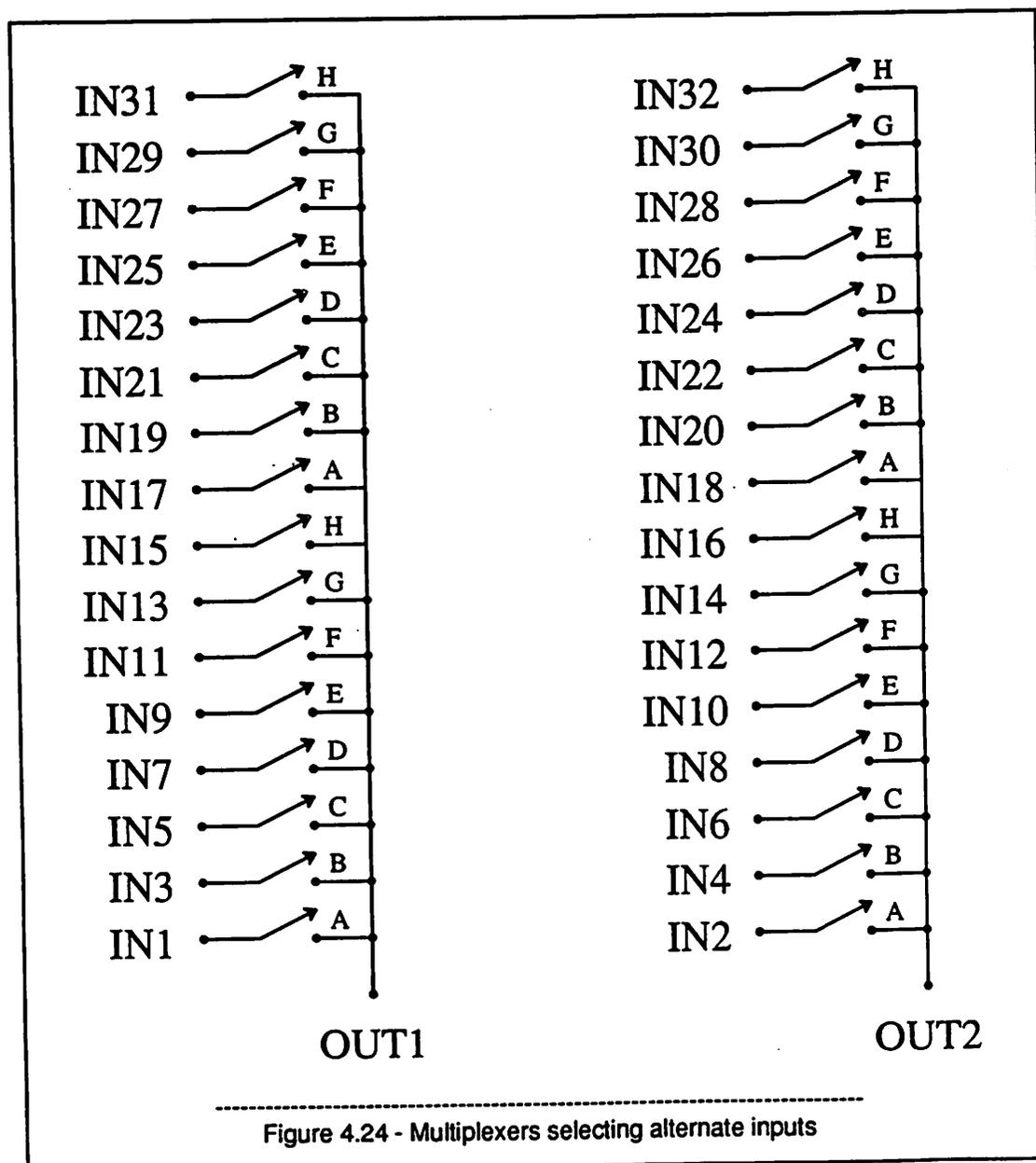
The problem is that multiplexer 1 selects  $V_{n+1}$  and multiplexer 2 selects  $V_n$ . This is fine for even inputs,  $|V_{n+1}| > |V_n|$ . But for odd inputs  $|V_{n+1}| < |V_n|$ . They could be switched with the switches shown in Figure 4.25 but this adds more series resistance.
