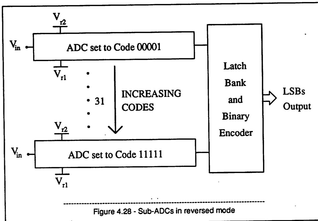
Now the thermometer code starts at the top and goes down. To decode this a second thermometer to 1-of-n decoder that decodes from top to bottom is added and its outputs are selected when needed.
