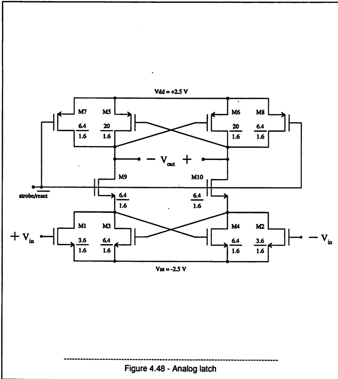
disconnecting the input from the load. M7 and M8 pull the outputs high while any input voltage pulls the drains of M3 and M4 low. When the strobe goes high the two halves are connected and the positive feedback latching occurs. In a conventional latch the time constant is  $C/g_m$ , but in this case there are 2 latching elements so the time constant decreases to  $\frac{C}{g_{mN}+g_{mP}}$ . The simulated results are in
