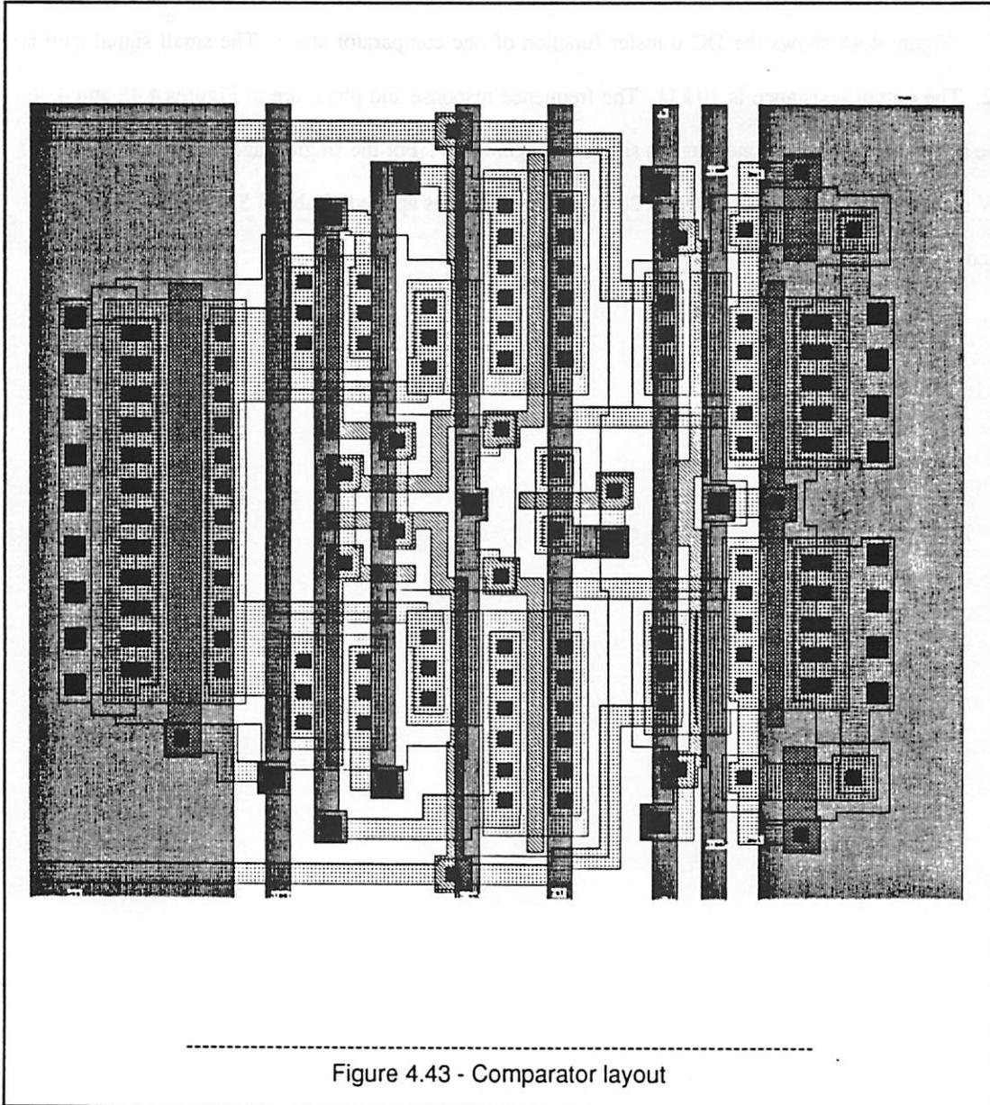
the reset switch gate, are perpendicular to the axis of symmetry so that a shift in the polysilicon or diffusion masks could not cause a mismatch in the two halves. 20  $\mu\text{m}$  wide metal lines were used for Vdd and Vss to minimize their voltage drop.
