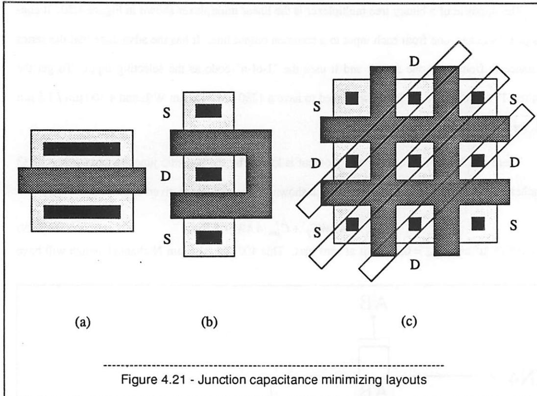
1.5 pF of parasitic junction capacitance and all 33 of them will have 50 pF. This is clearly much too large a load and it is over 3 times worse for the P-channel switches.
