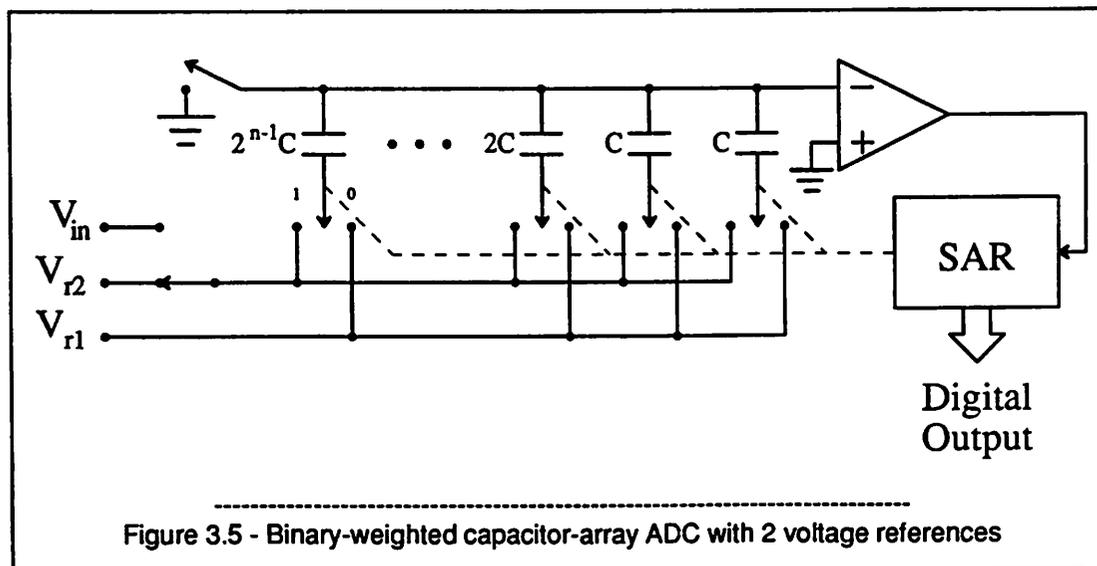
and  $V_{r2}$  as shown in Figure 3.5. The operation is the same. The charge redistribution goes as follows:
