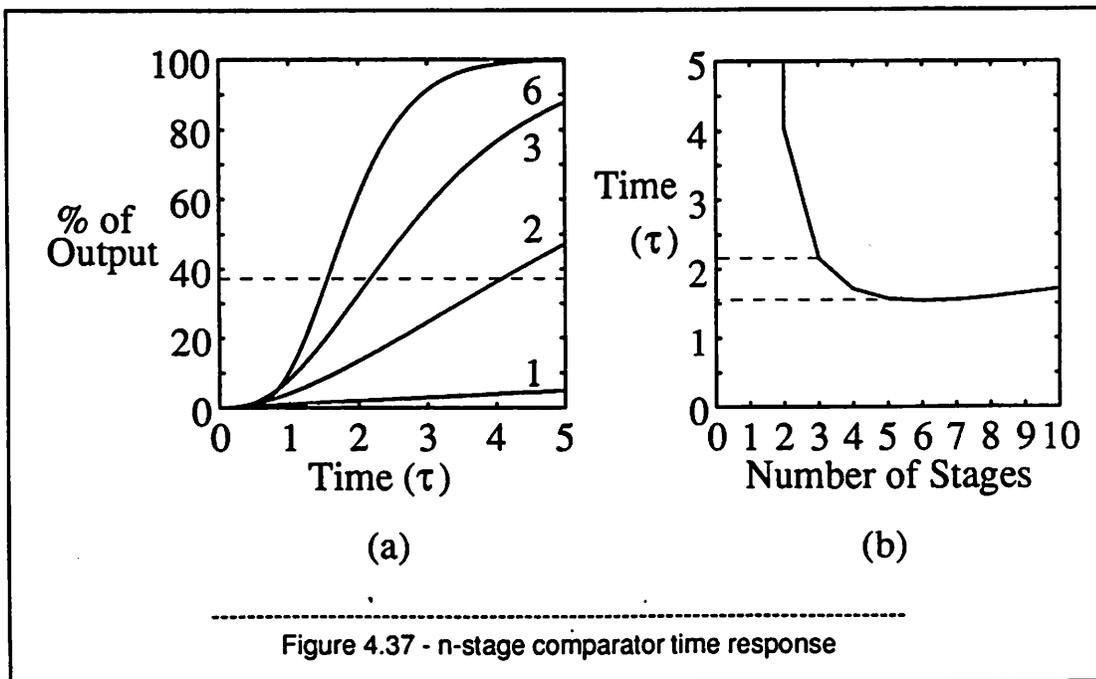
gain. If one time constant is allotted to the latch it will have a gain of  $e$ . Thus consider the comparator amplification complete when it gets to  $\frac{1}{e}$  of its final value as shown by the dotted line in the graph. The time to reach the dotted line versus the number of stages is plotted in Figure 4.37b. The fastest response is for 6 stages. This is almost the same as the result of Section 5.3.1 and Section 5.3.2 evaluated here:
