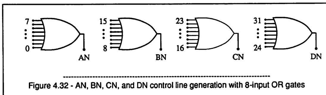
8-input OR gates are just a brute-force solution and impractical to implement. A better way is to check the thermometer code and see what quarter of the resistor string the input voltage lies in. For example, line AN is active for codes less than or equal to 7. Line BN is active for codes less than or equal to 15 and greater than or equal to 8, etc. Figure 4.33 shows the simple logic needed to do this.
