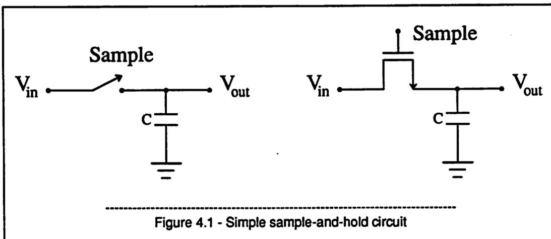
From Equation 4.1 it is seen that the errors are technology dependent from the terms  $C_{ol}$ ,  $C'_{ox}$  and  $V_t$  and they have components based upon the design parameters  $W$ ,  $L$ ,  $C$ ,  $V_H$  and  $V_L$ . Even when the design attempts to minimize the charge-injection error often it is too large to tolerate. The two most common circuit solutions to combat it are dummy switches and differential circuitry.
