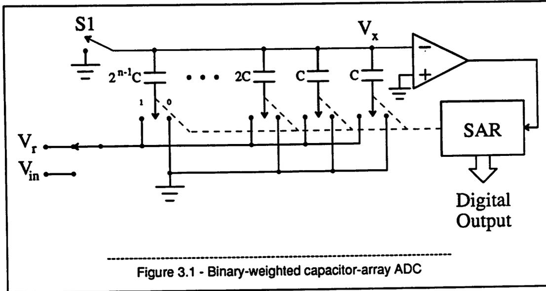
The voltage at the top plate and comparator input is  $V_x$ .
