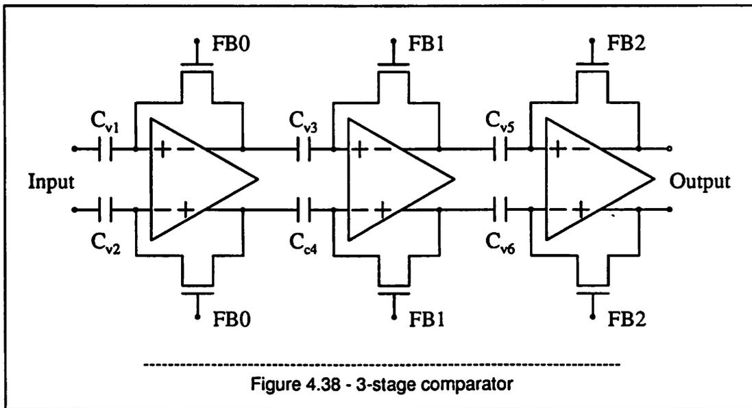
timing developed by Allstot<sup>19</sup> the charge-injection error from the first stage can be canceled if the ADC has an external S/H. When FBO opens its charge-injection error is a voltage on capacitors  $C_{v1}$  and  $C_{v2}$  that is amplified by the first stage and stored on capacitors  $C_{v3}$  and  $C_{v4}$  before the other feedback switches are opened. The experimental results of canceling the charge injection error are in Chapter 8, Section 2.1.1.1.
