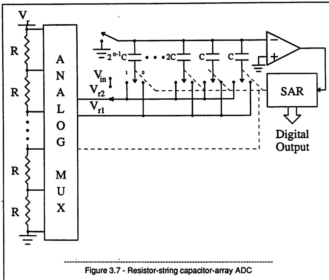
capacitor array, used as one capacitor, and do a successive-approximation search on the resistor string for the MSBs. Once they are found the resistor whose tap voltages encompass the unknown input is selected and the voltages at its endpoints are selected by the multiplexer and used as the two reference voltages for the capacitor array ADC. The capacitor array ADC then does a second successive-approximation search for the LSBs.
