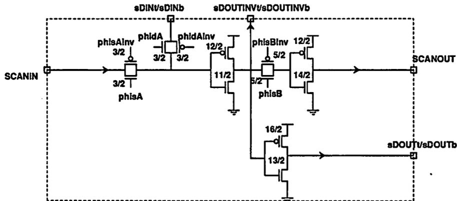
Figure 6.3: Circuit diagram of scan latch. The latch operates on only one phase during normal operation.
