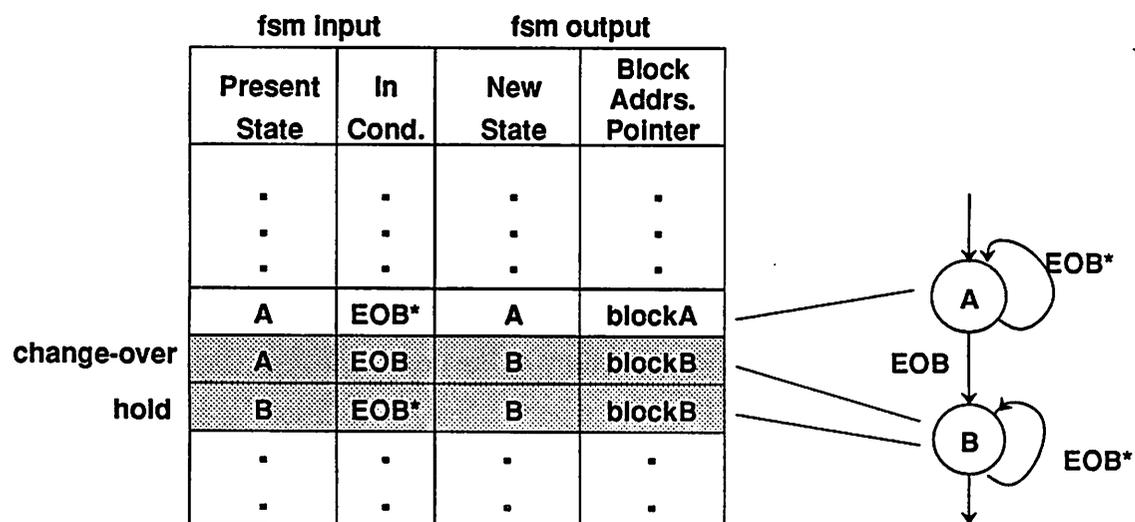
Figure 3.7: Fsm state transitions and state-table. Each transition requires two entries in the table: change-over and hold. In the change-over state, which lasts for only one cycle following EOB, the first instruction of blockB is executed. The remaining instructions of blockB are executed during hold state of B.
