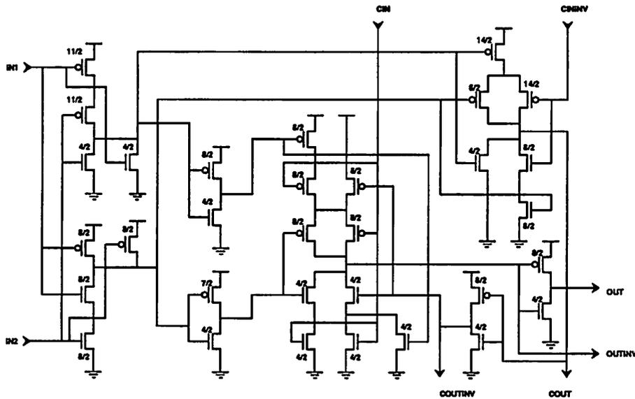
Figure 5.32: Circuit diagram of the even slice of the adder. For the MSB slice, CININV is also brought out as COUTN-1INV.
