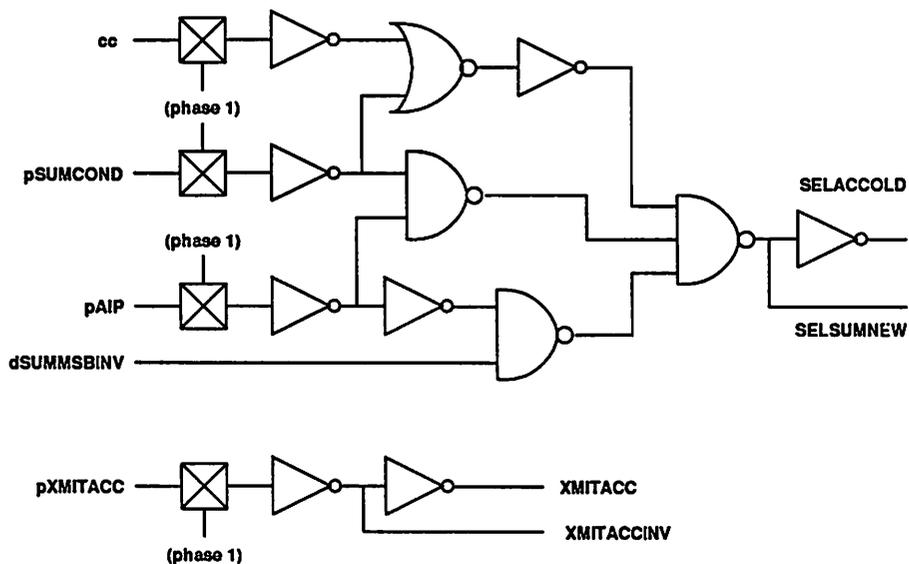
Figure 5.38: Control circuits for accumulator.
