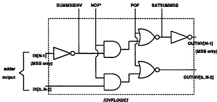
Figure 5.35: The adder outputs are saturated to either positive maximum or negative maximum on overflow.
