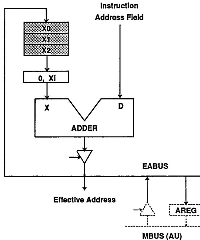
Figure 3.27: Address processing unit block diagram.
