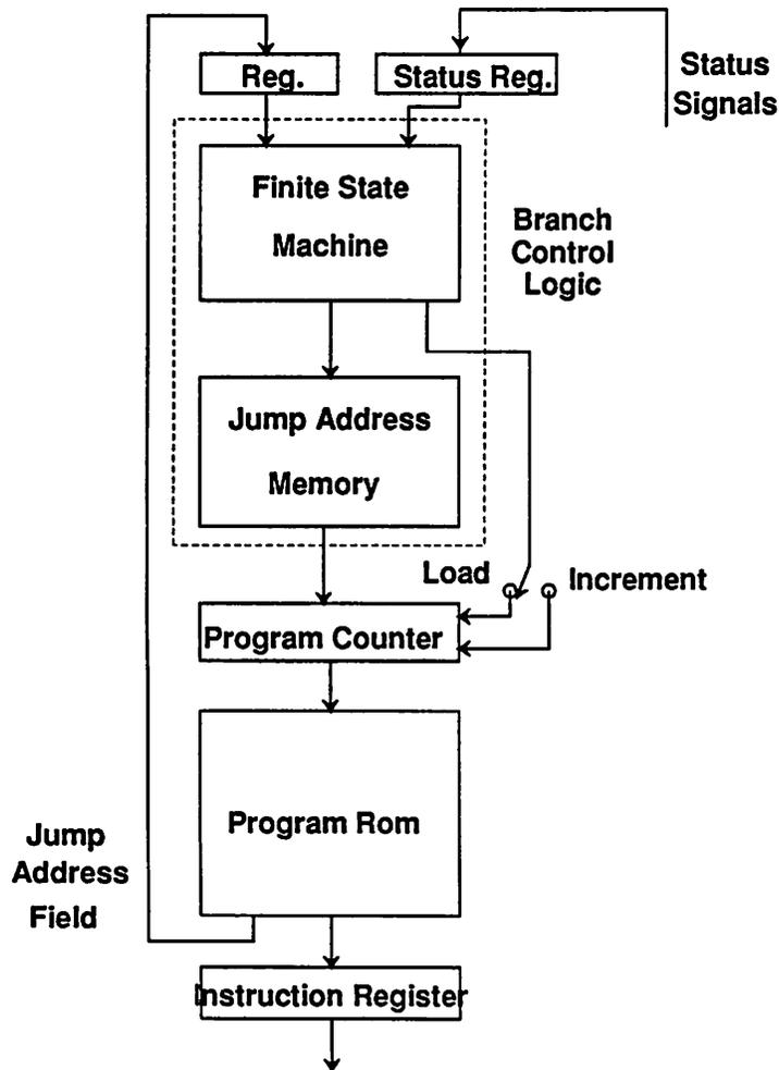
Figure 3.16: Control unit used in the Cathedral design system for DSP circuits.
