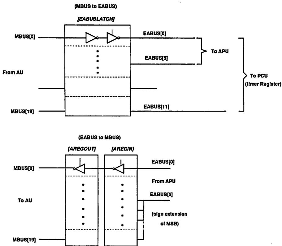
Figure 5.44: Interconnection network between EABUS and MBUS.
