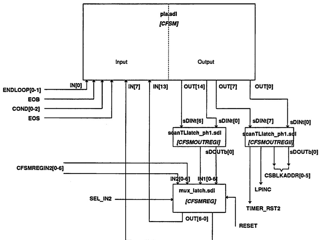
Figure 5.10: Block diagram of the PCU's finite state machine.
