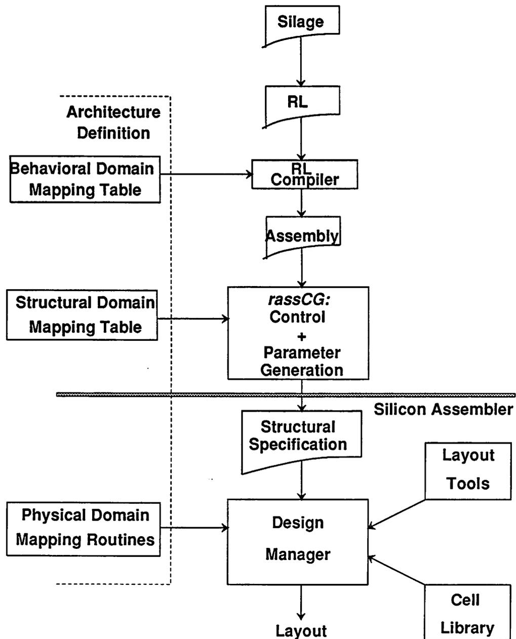
Figure 4.1: Lager-III silicon compiler system.
