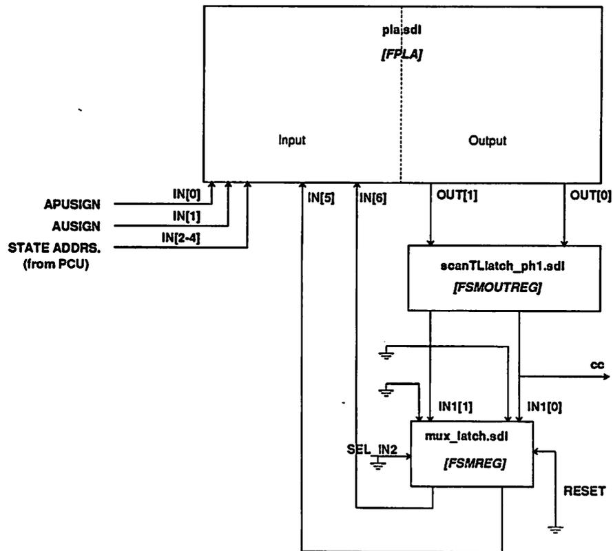
Figure 5.52: The logical unit is essentially a finite state machine.
