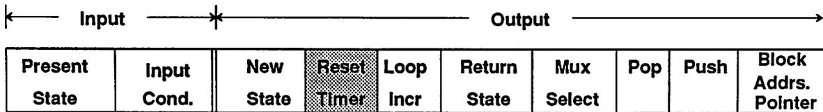
Figure 3.14: Fsm input and output fields. Timer reset control bit is high lighted.
