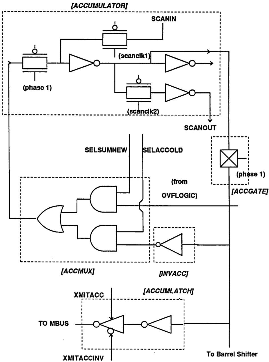
Figure 5.37: Accumulator circuits.
