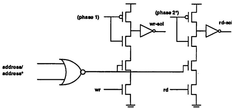
Figure 5.50: The address decoding circuits.
