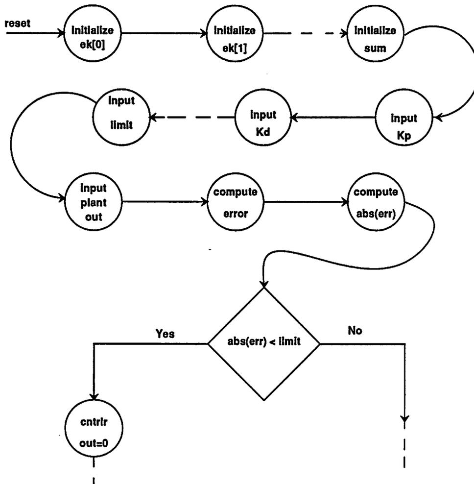
Figure 3.2: A partial state transition diagram for a PID control algorithm
