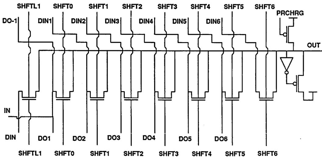
Figure 5.41: The barrel shifter is based on dynamic CMOS circuit design technique with a PMOS pull-up.
