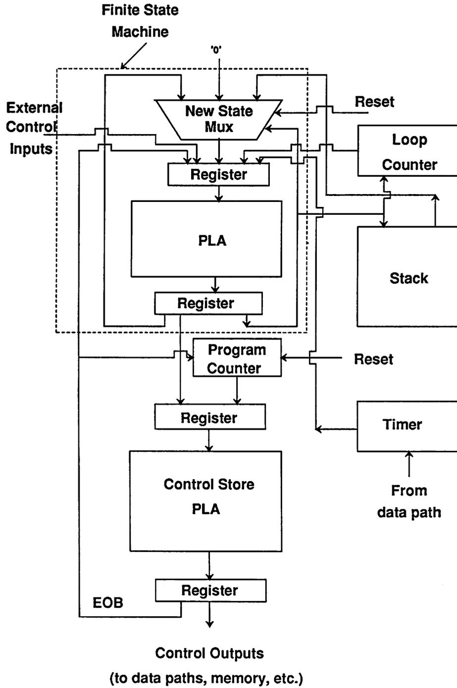
Figure 3.15: Block diagram of the complete PCU.
