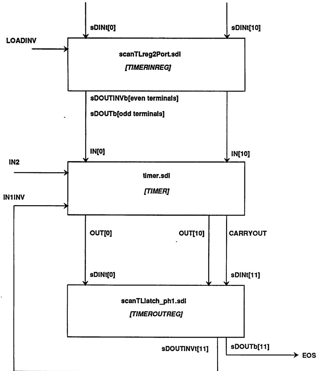
Figure 5.19: Block diagram of the timer-Macro.
