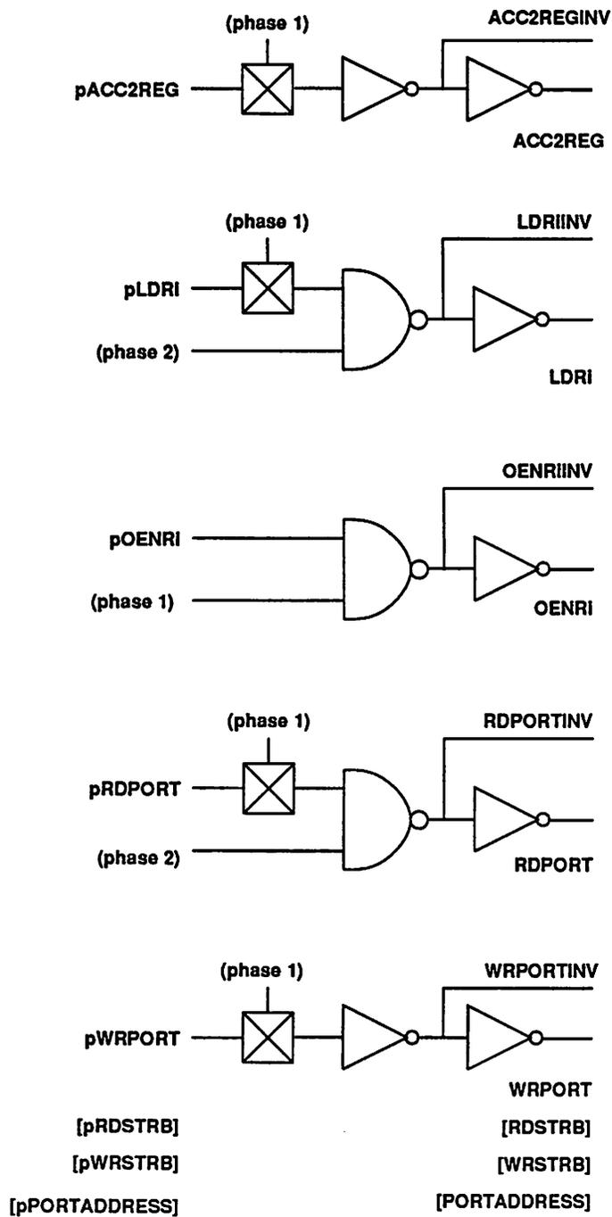
Figure 5.40: Control circuits for registers and I/O port.  $WRPORT$ ,  $RDSTRB$ ,  $WRSTRB$ ,  $PORTADDRESS$ , and their complement signals are all generated using the same type of circuits.  $i$  in  $OENR_i$  and  $LDR_i$  refers to the register number ( $i = 1$  or  $2$ ).
