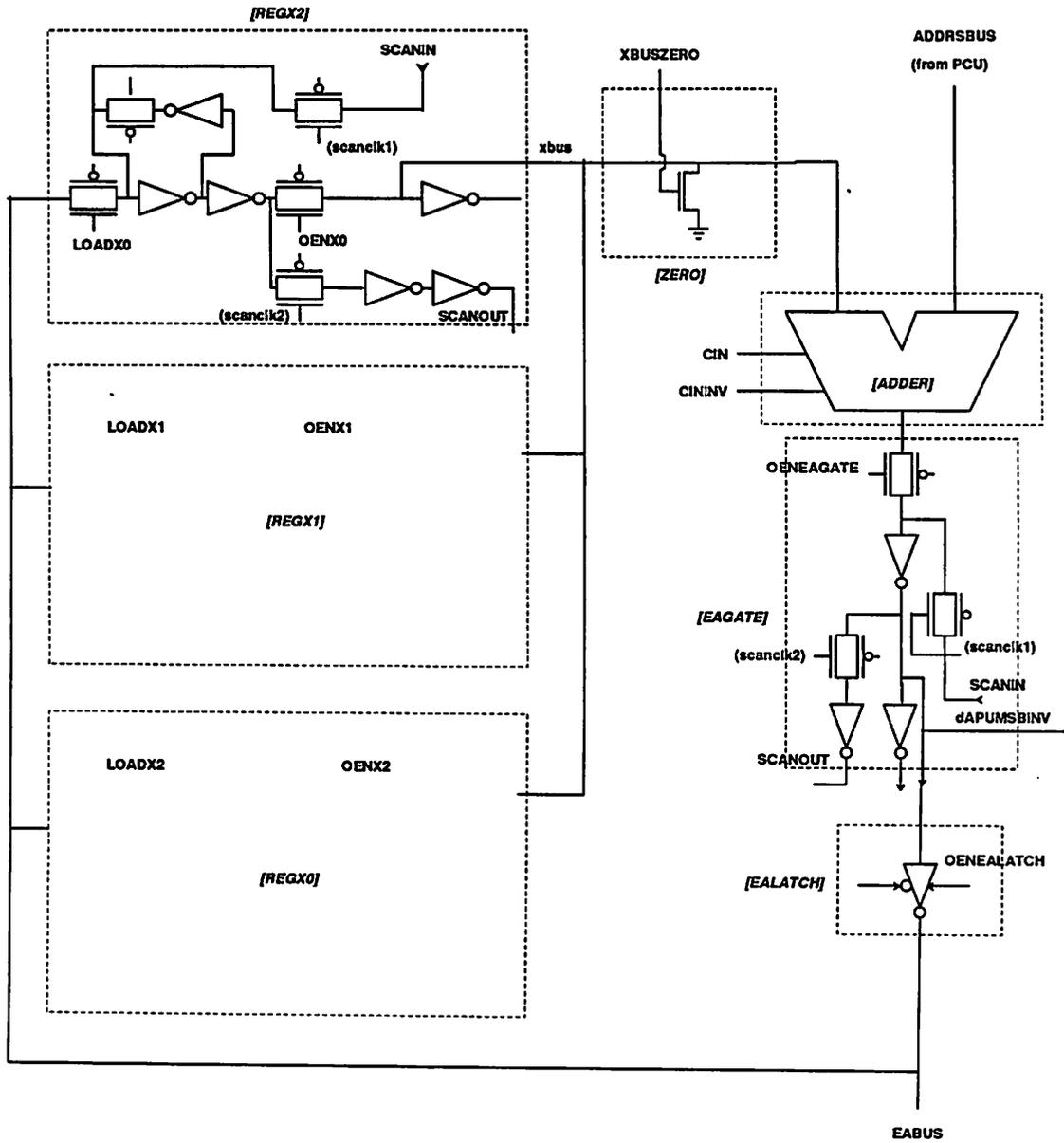
Figure 5.45: Circuit diagram of APU.
