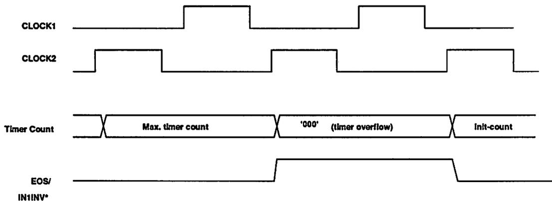
Figure 5.21: Timing diagram for the timer.
