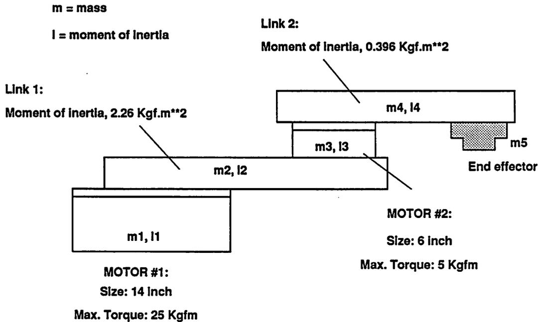
Figure 2.3: A two-axis, direct-drive robot arm from NSK/Motornetics Corp., Santa Rosa, California
