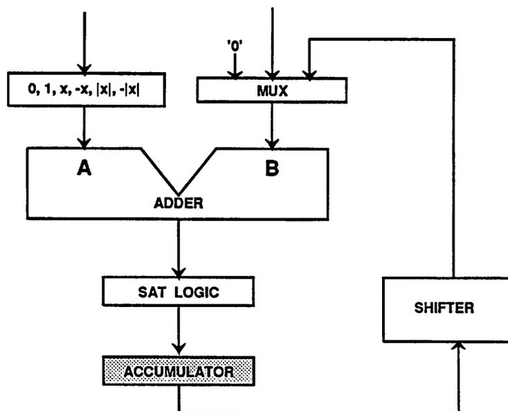
Figure 3.23: Section of the AU data path which performs add, shift and other arithmetic operations. The coefficient register used in shift/accum. multiplication is not shown here.
