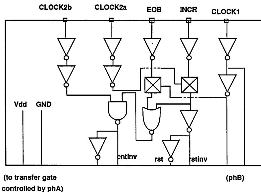
Figure 5.16: Control circuits for the loop counter.
