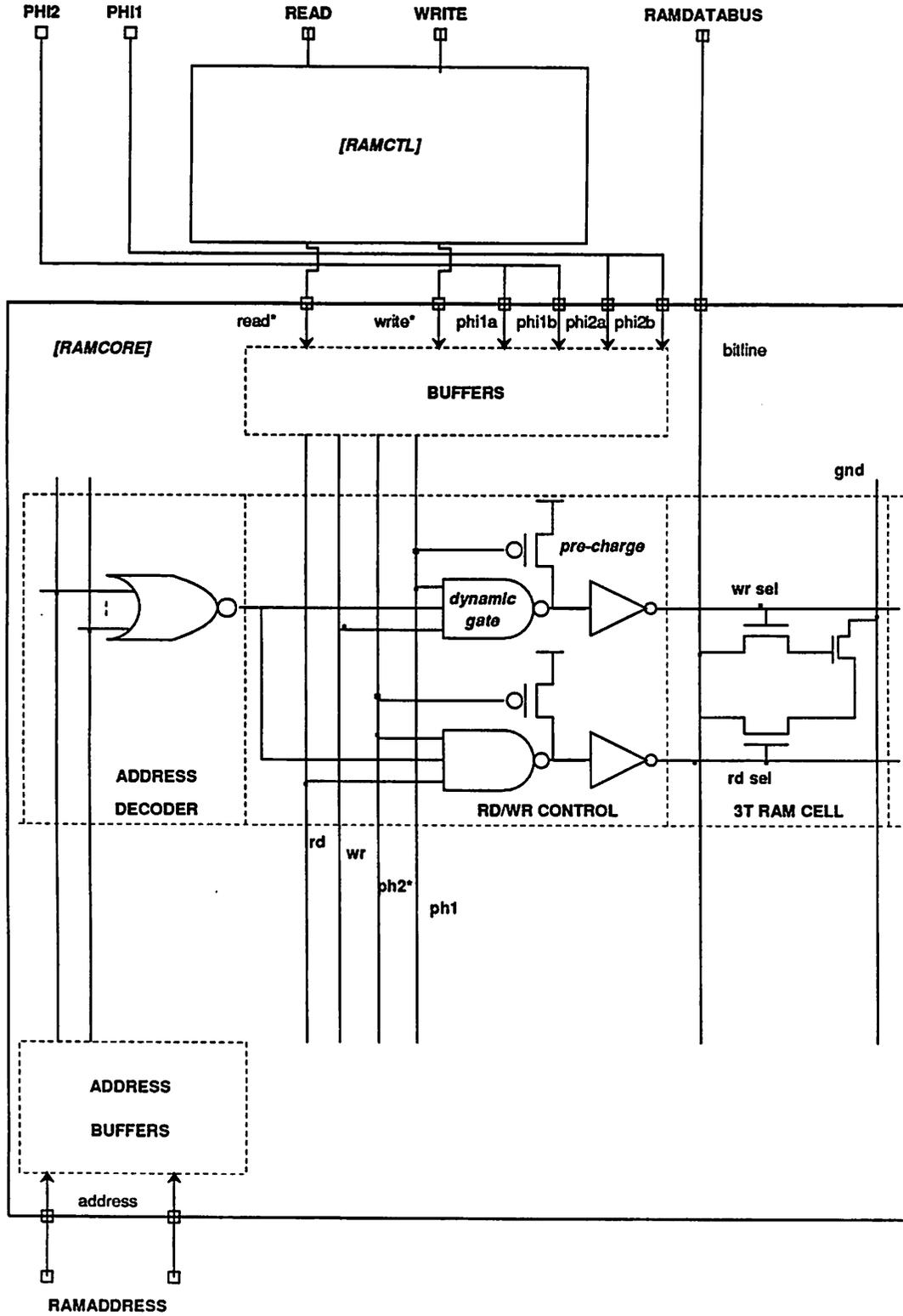
Figure 5.47: The ram macrocell is composed of two child macrocells: RAMCORE and RAMCTL.
