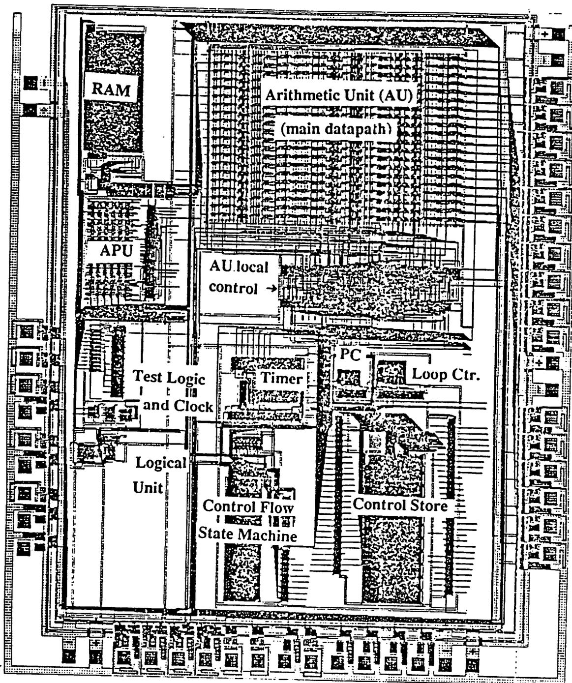
Figure 7.5: A cifplot of the robot controller chip showing the major macrocells.
