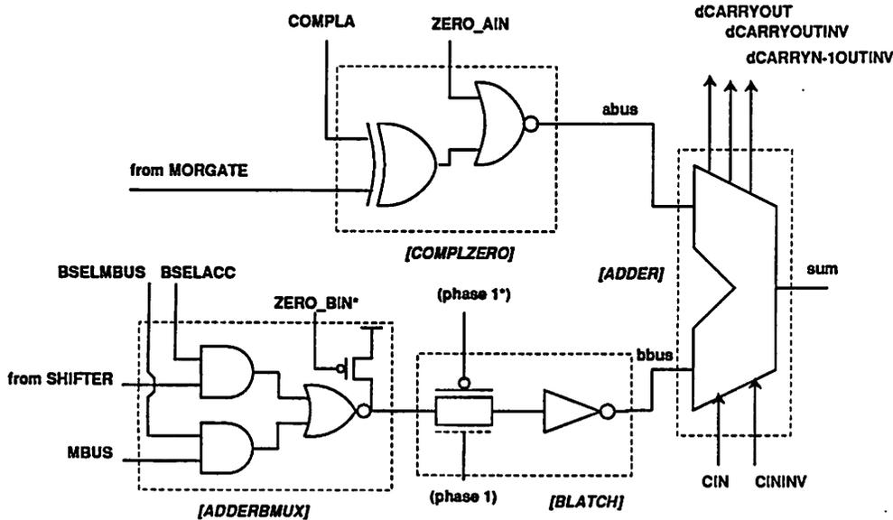
Figure 5.30: Arithmetic section of the data path.
