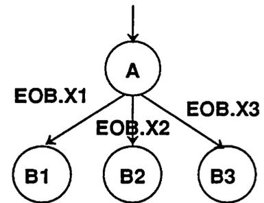
Figure 3.8: Change-over states and the corresponding state table entries for a multi-way branch. Entries for the hold states are not shown.
