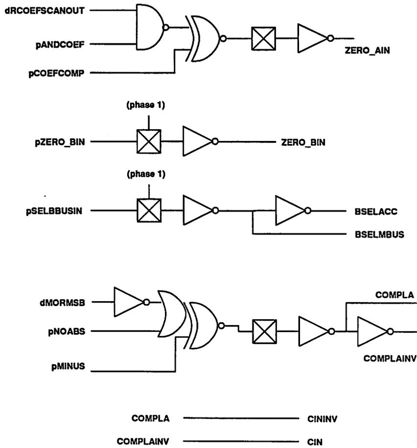
Figure 5.31: Control circuits for the arithmetic section.
