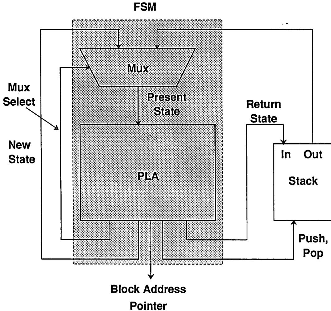
Figure 3.10: Figure showing the addition of a mux and a stack to the PCU for supporting subroutine. The control store and program counter are not shown.
