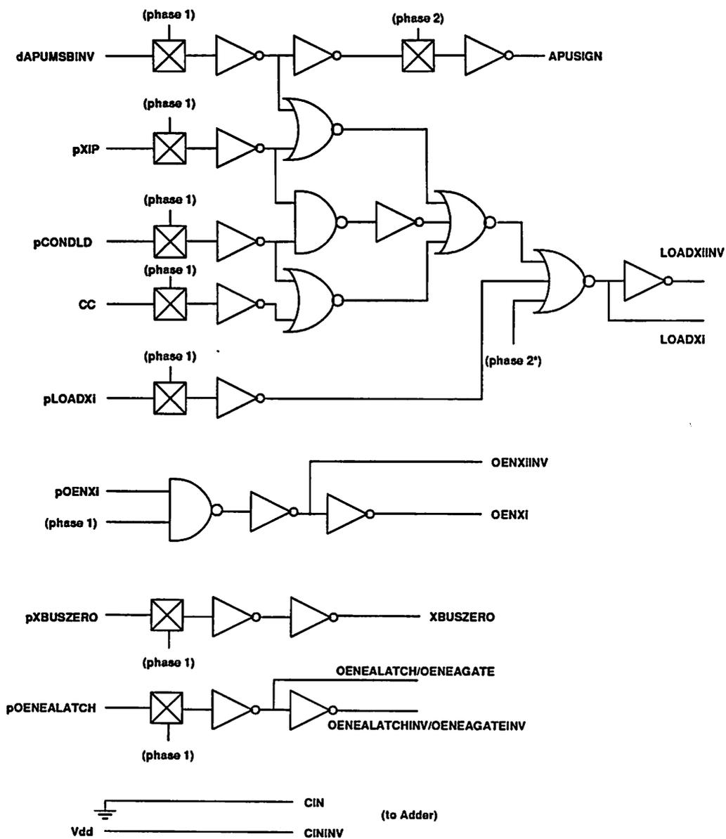
Figure 5.46: Control circuits for the APU. The control circuits for loading and enabling the registers are identical for all the three registers. *i* indicates register number (as in `LOADXi`).
