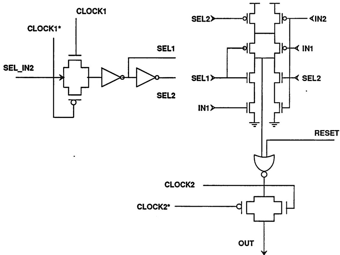
Figure 5.11: Mux\_latch circuit is used to latch either the state output from the FSM or the return state from the stack. Mux\_latch also provides means for forcing the FSM into zero state for reset purposes.
