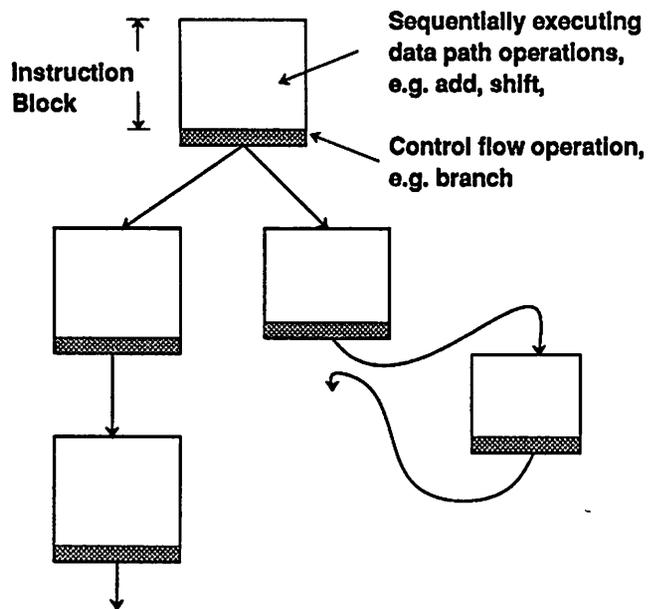
Figure 3.3: Program model showing data path operations and control flow operations.
