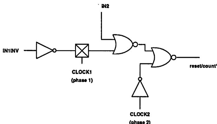
Figure 5.20: Control circuit for resetting the timer.
