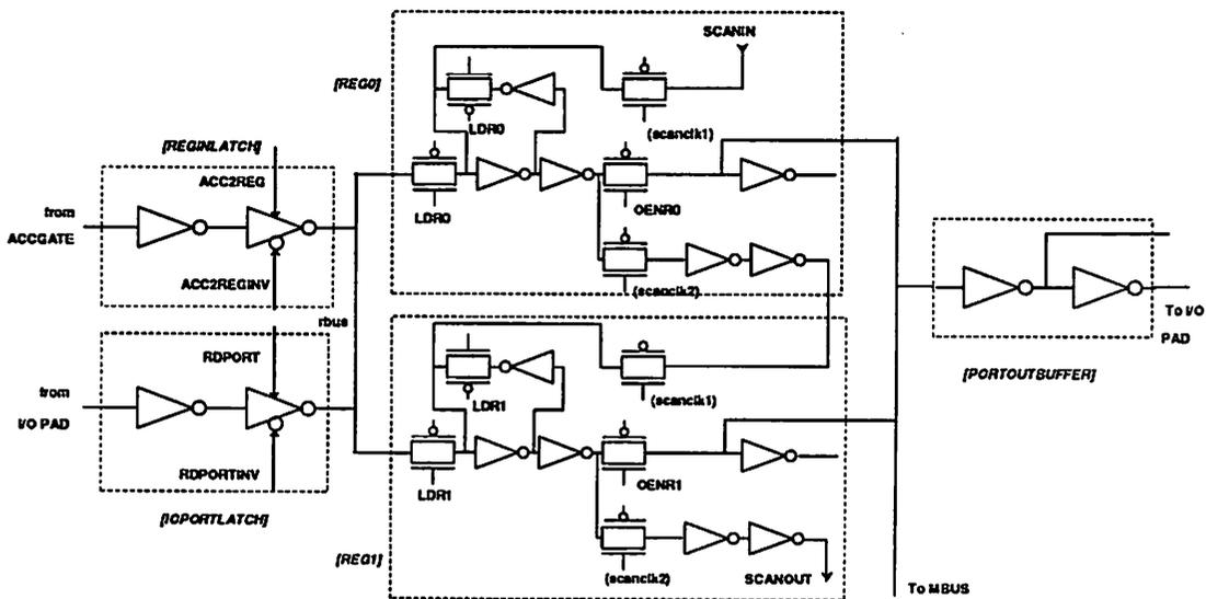
Figure 5.39: Register circuits for the AU data path.
