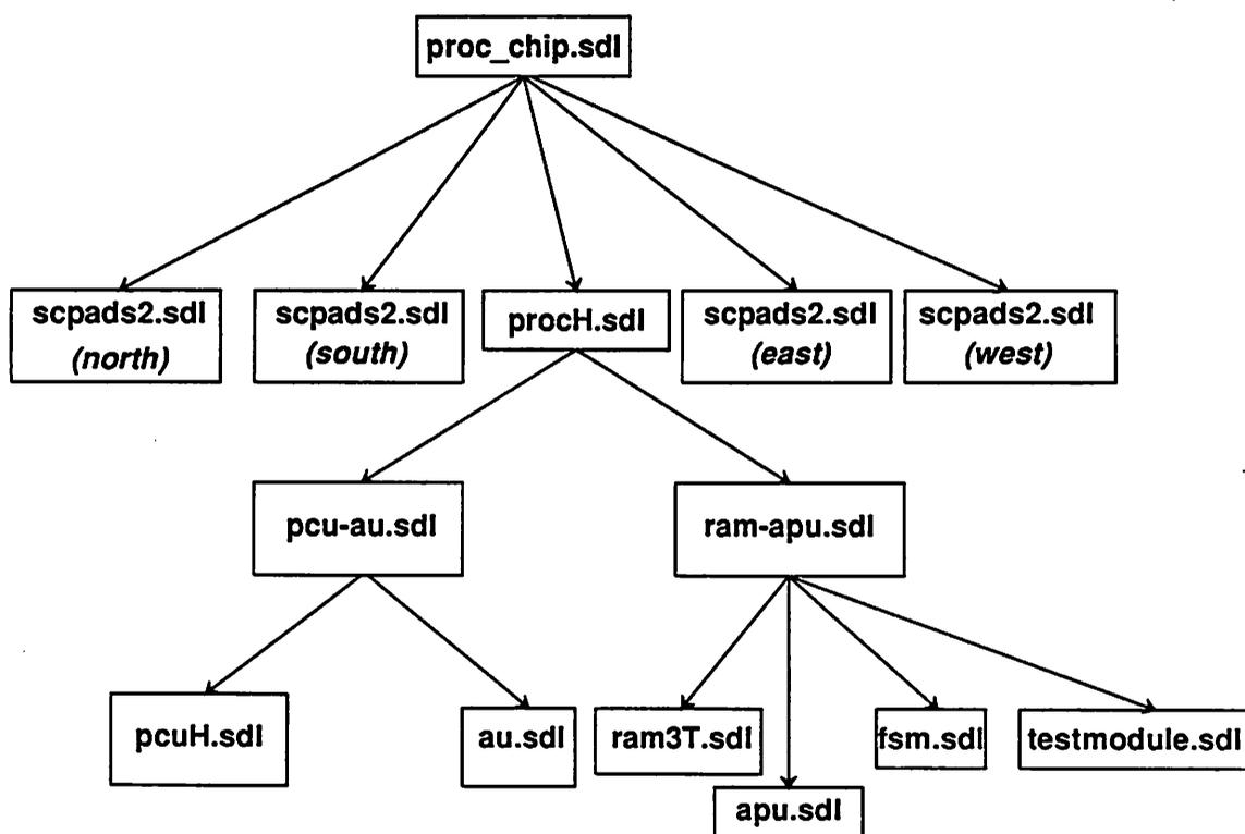
Figure 5.1: The structural hierarchy of the robot control processor. In this figure, the five cells at the bottom are the five major macrocells in the processor.
