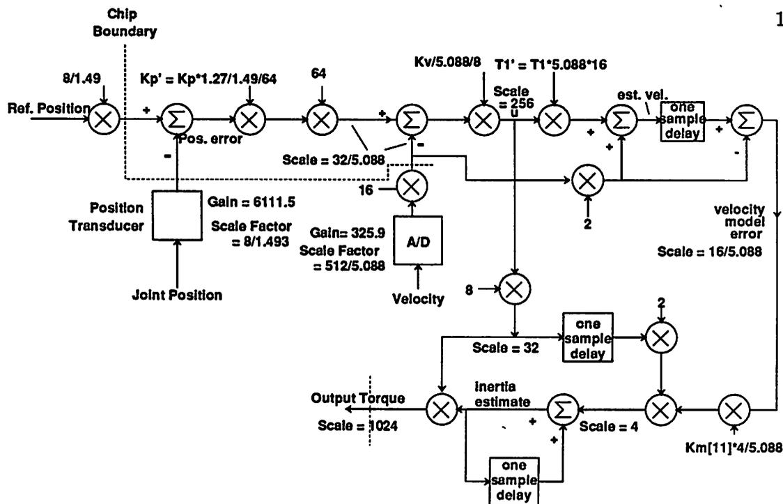
Figure 7.1: Partial flow-diagram showing scale factors at various nodes. Multiplication with constants are done through shifting. All the coefficients are first read from an external source. These coefficients are pre-scaled with the appropriate factors as shown. Position and velocity measurements are also pre-scaled before being read into the chip.
