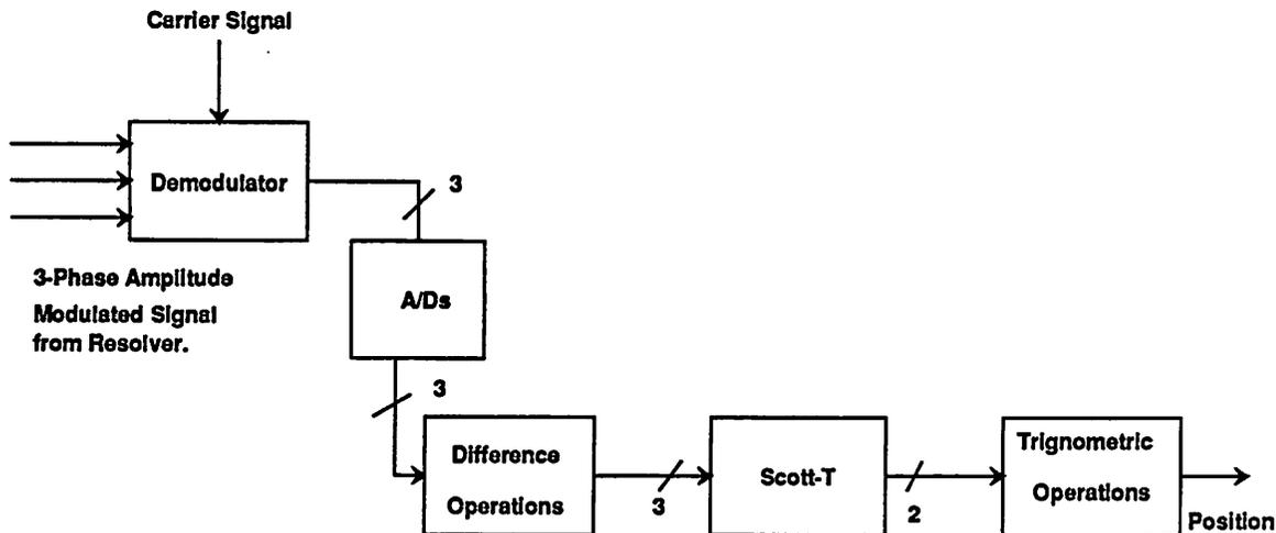
Figure 2.8: Block diagram showing the operations required to obtain the position information from the resolver output.
