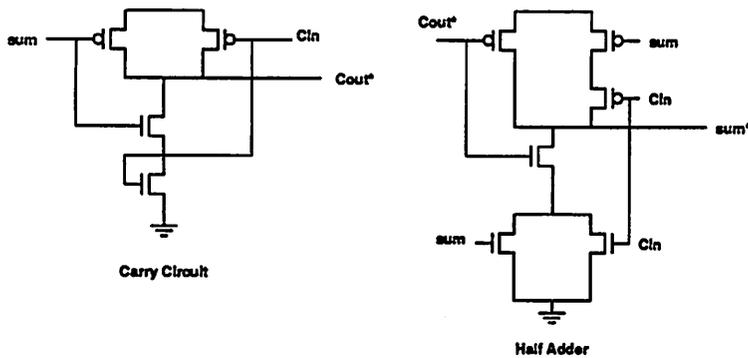
Figure 5.14: Half-adder and carry circuits for the even-slice of the counter. The sum input is the previous sum whereas sum\* is the complement of the new sum. The odd-slice circuits are just the complement of the even-slice.
