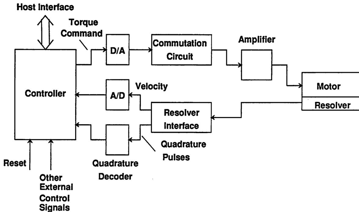
Figure 2.6: Robot controller with external signals and I/O circuits for one joint
