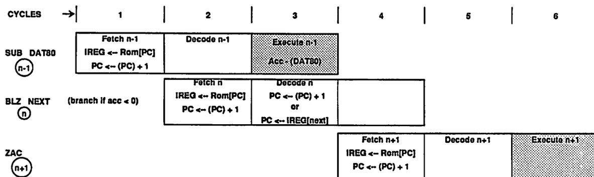
Figure 3.20: Execution of branch instruction in TMS32020. During cycle 3, based on evaluation of the branch conditions, PC either gets the address of the next sequential rom instruction or the address of the branch target. Note that between the execution of the (n-1)th instruction and the (n+1)th instruction, the branch operation takes up two cycles. (The actual increment in the PC during fetch cycle may be more than one, depending on the number of words required by the current instruction.)
