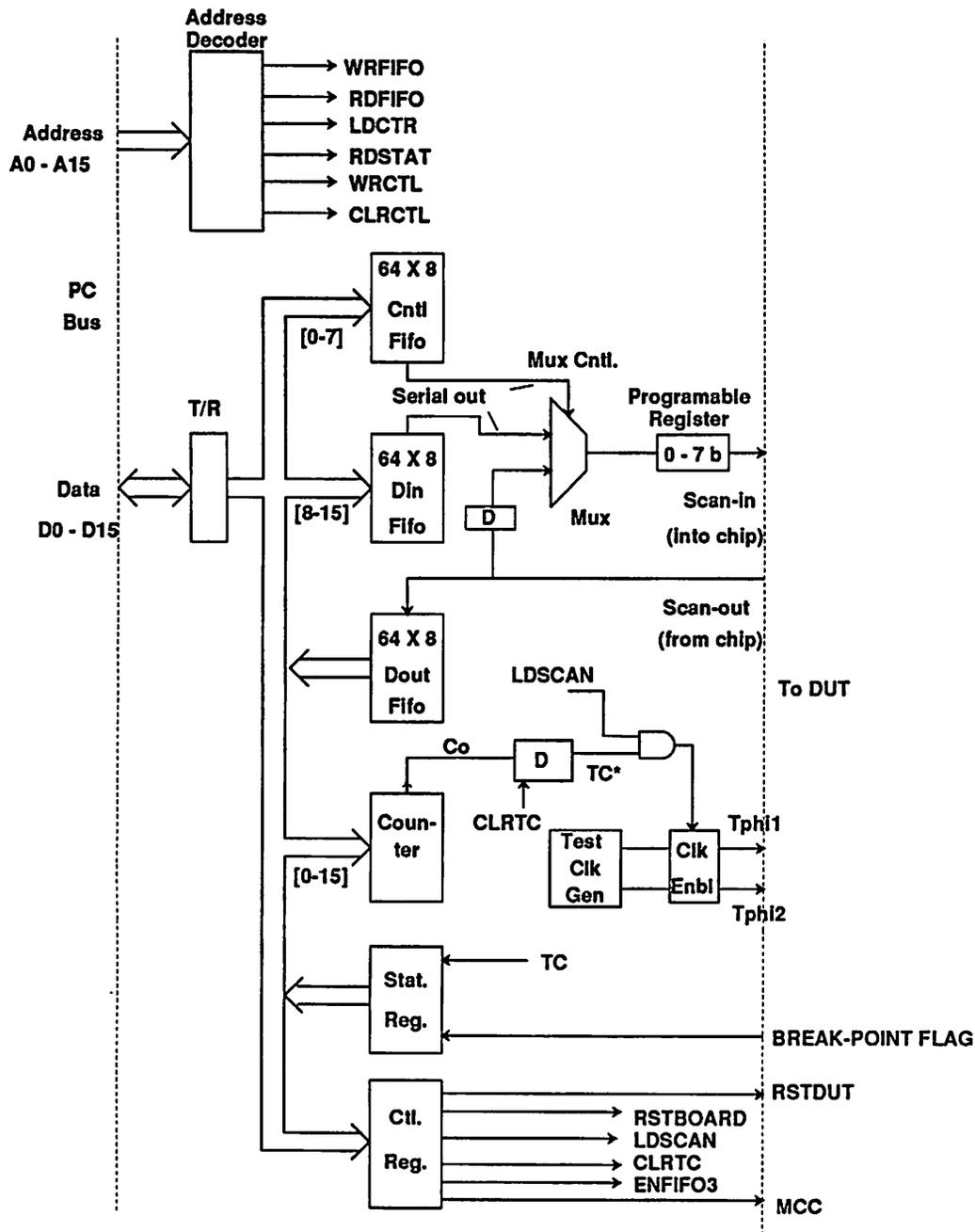
Figure 6.7: Schematic of the test-board. Only the essential components and signals are shown here.
