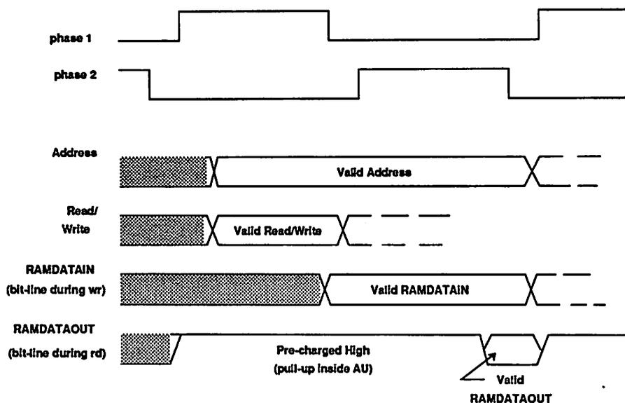
Figure 5.51: Timing diagram for the ram.
