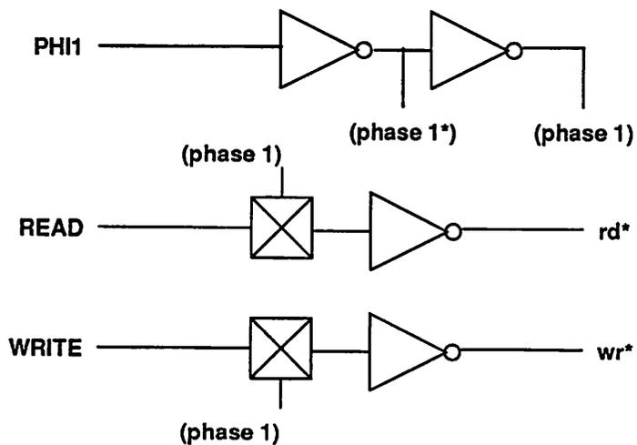
Figure 5.49: Control circuits for the ram.
