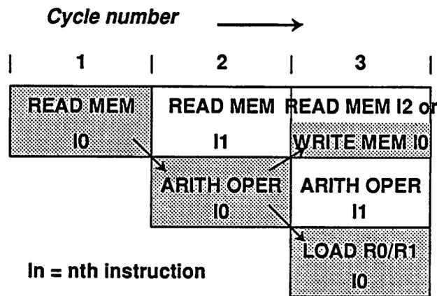
Figure 3.26: The three pipeline stages of the data path.
