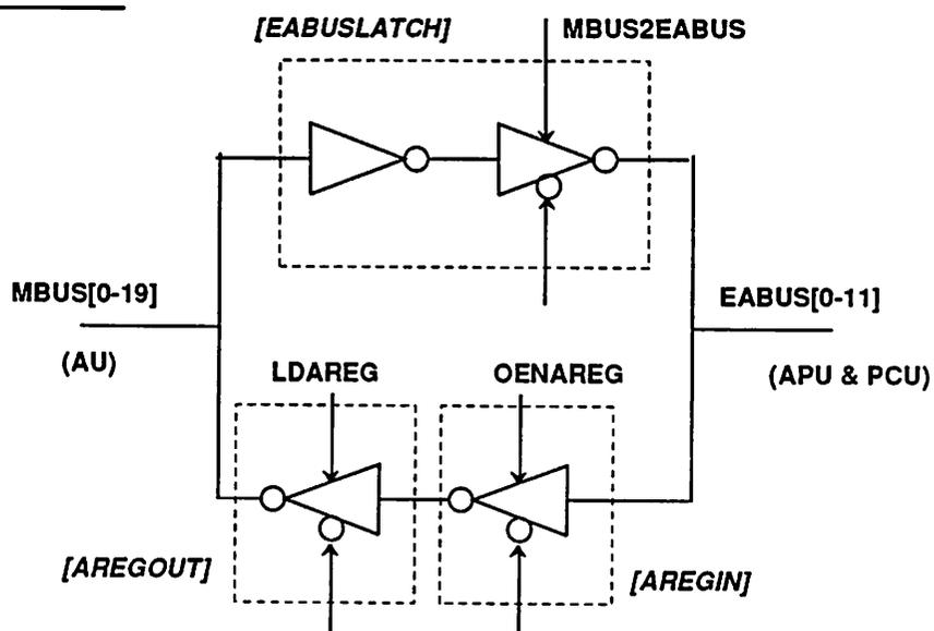
Figure 5.43: MBUS-EABUS interface circuits and their control circuits.
