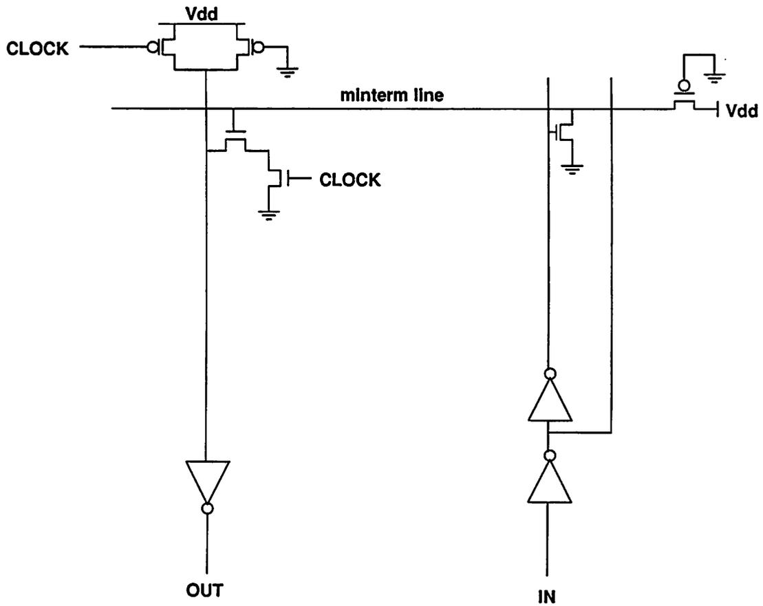
Figure 5.8: PLA circuit showing one input line, one minterm line and one output line. The active high outputs become valid when CLOCK, which may be connected to phase 1 or phase 2, goes high.
