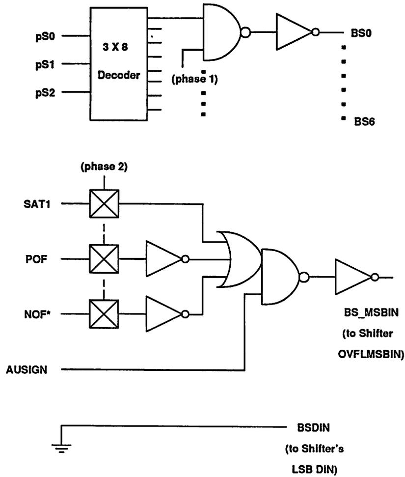
Figure 5.42: Control circuits for the barrel shifter.
