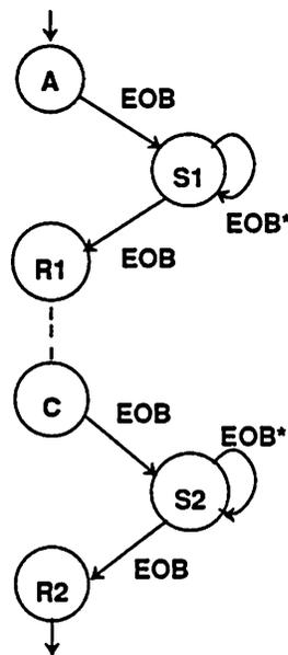
Figure 3.9: Implementation of limited subroutine capability without using stacks. Figure showing both subroutine states S1 and S2 pointing to the same instruction block, blockS. Because they return to different states R1 and R2 respectively, the two states cannot be merged.
