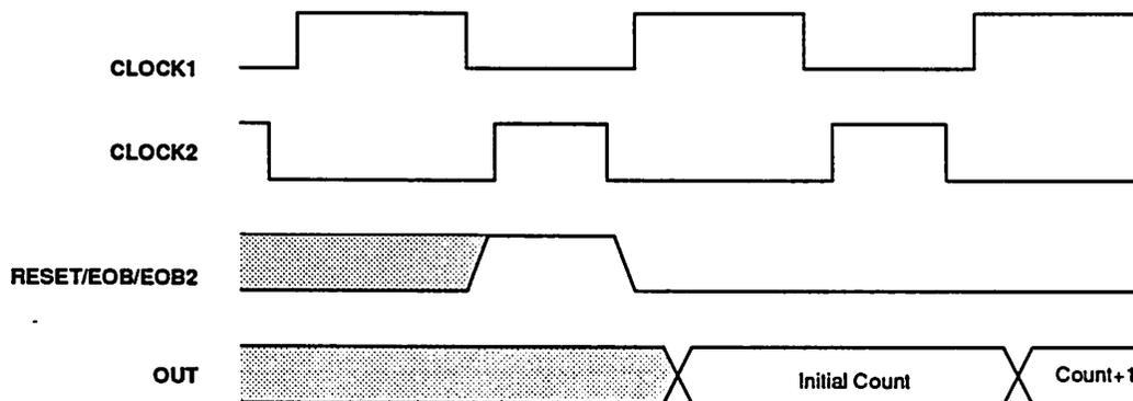
Figure 5.15: Timing diagram for the program counter.
