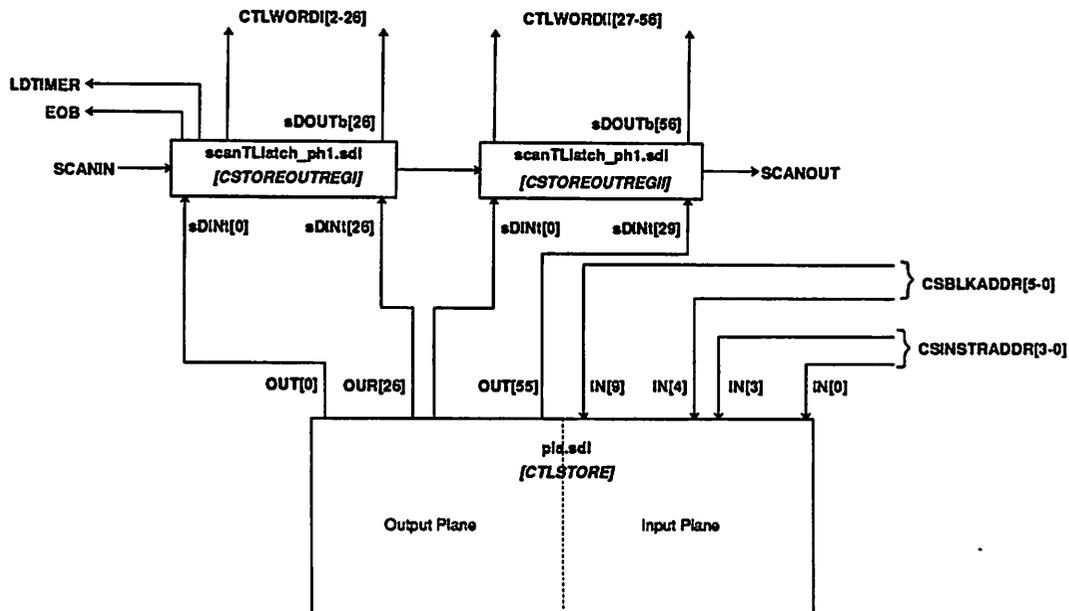
Figure 5.7: The cstore-Macro consists of a pla and two scan-type latches.
