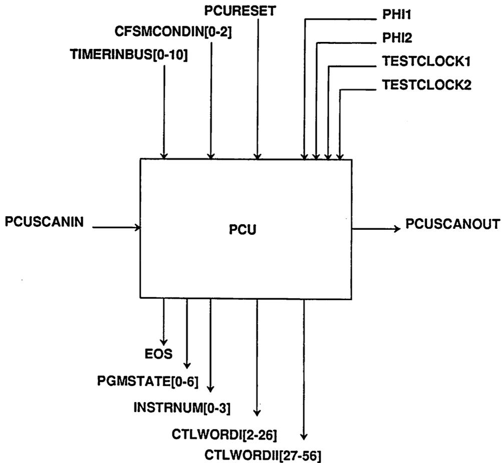
Figure 5.6: Boundary terminals of the PCU. The number inside [] give the actual bus widths for the robot controller design.
