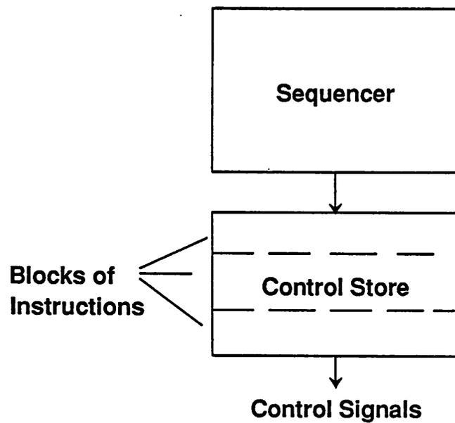
Figure 3.4: Hardware model for the control unit.
