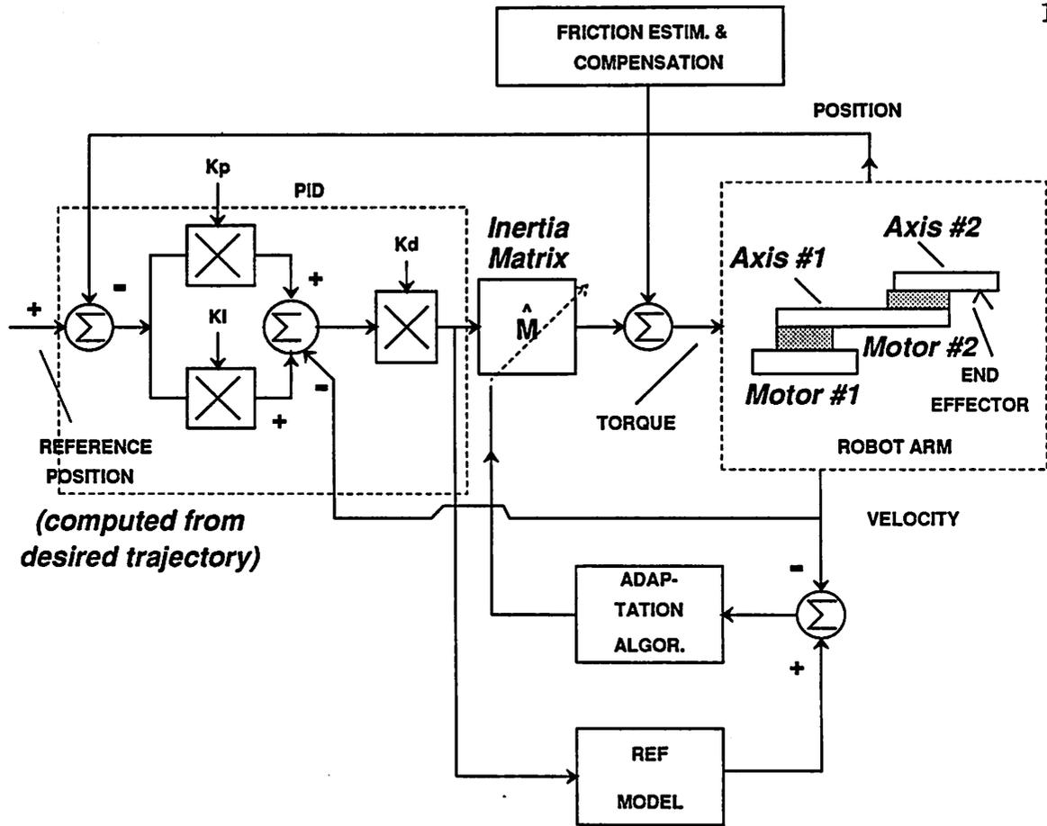
Figure 2.4: Block diagram of the control algorithm showing PID section, adaptive section, and friction compensation
