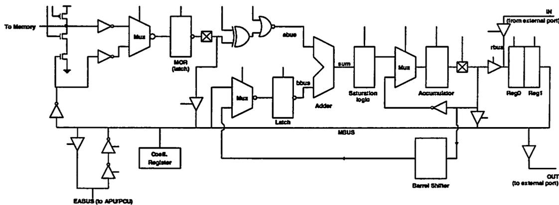
Figure 5.26: Schematic of the arithmetic unit data path.
