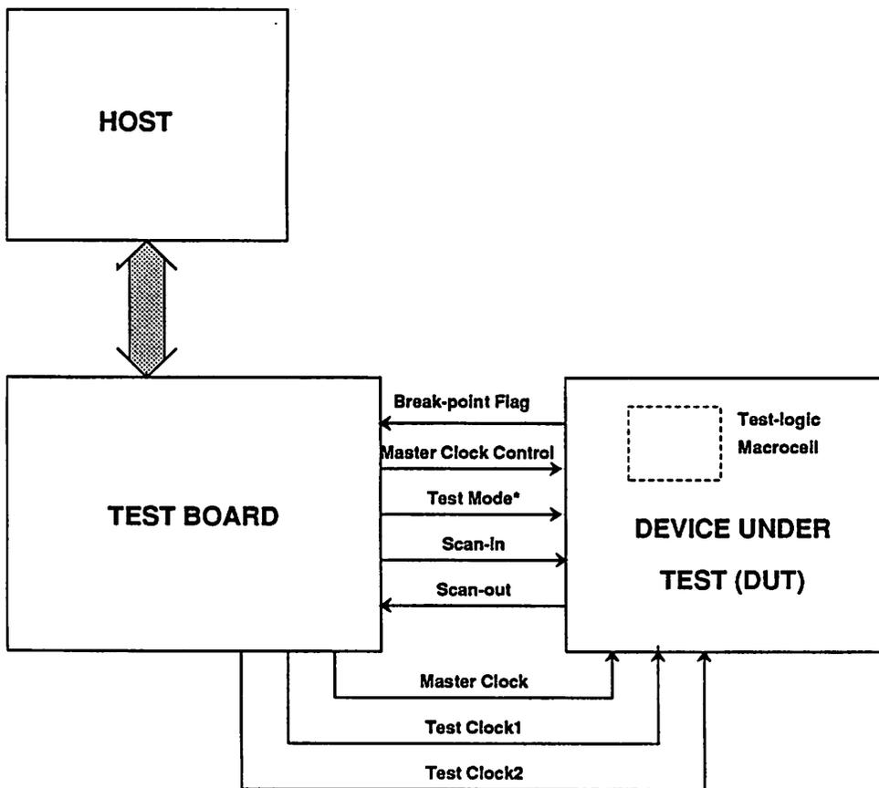
Figure 6.1: Block diagram of the test setup.
