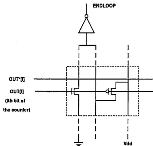
Figure 5.18: Count-detect circuits for the loop counter.
