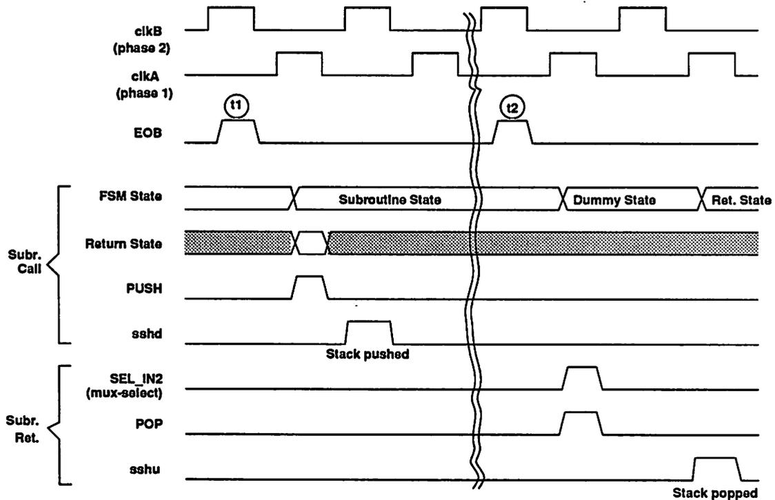
Figure 5.24: Timing diagram showing stack operations for subroutine call and return. EOB signal and FSM state transitions are also shown.
