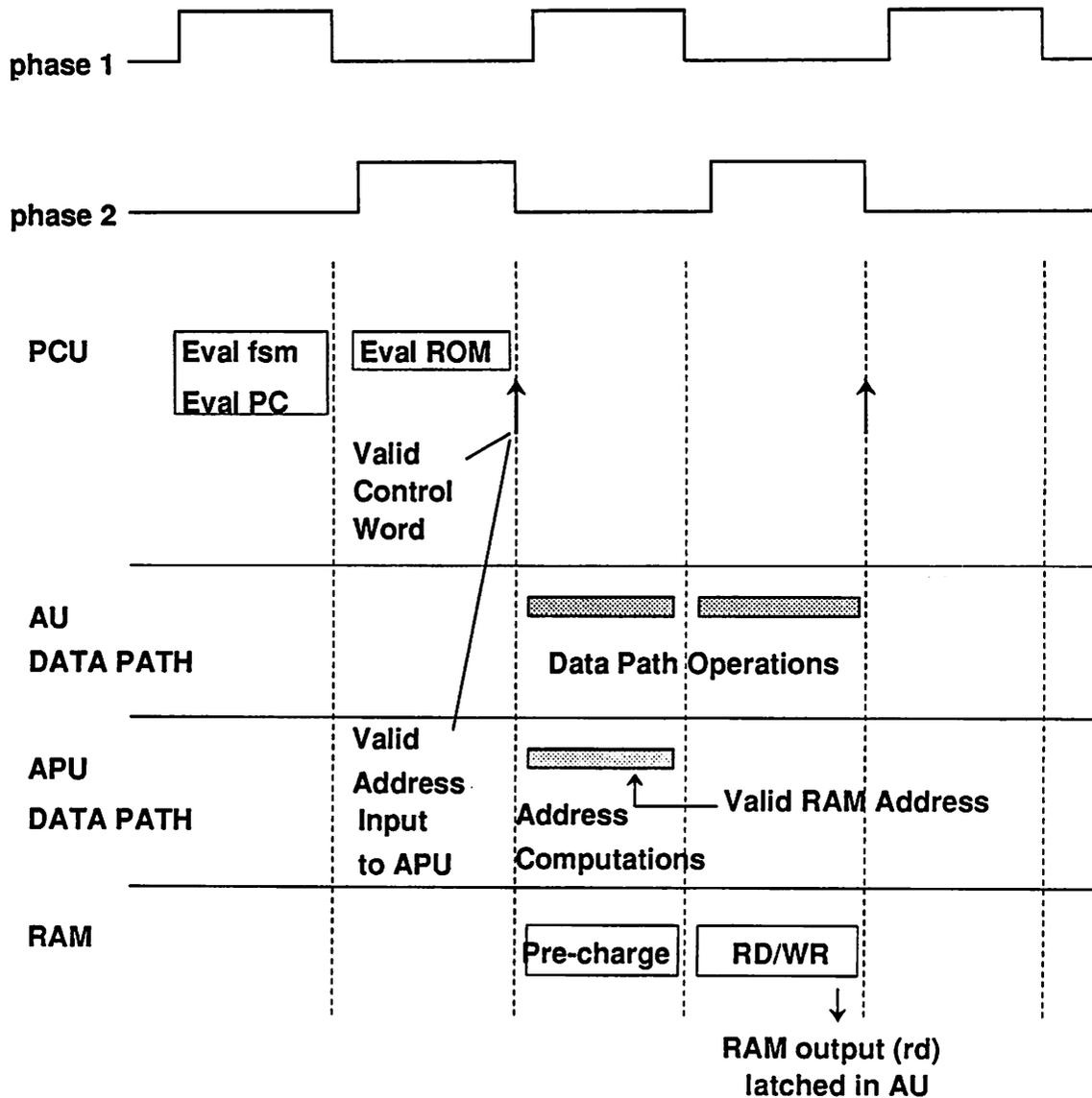
Figure 5.3: The global timing scheme of the processor is based on a two phase non-overlapping clock. On each cycle a new control-word is generated which determines the data path and ram operations in the following cycle.
