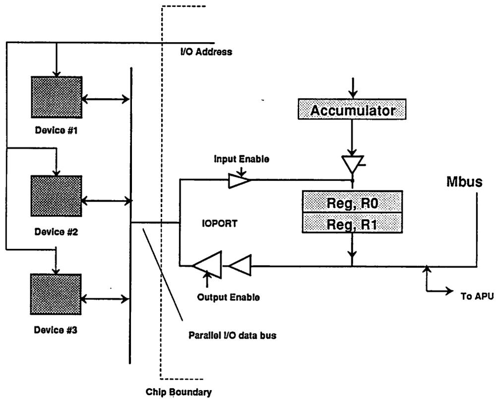
Figure 3.24: Section of data path showing I/O bus and registers. All data transfers to and from the data path are done through parallel lines.
