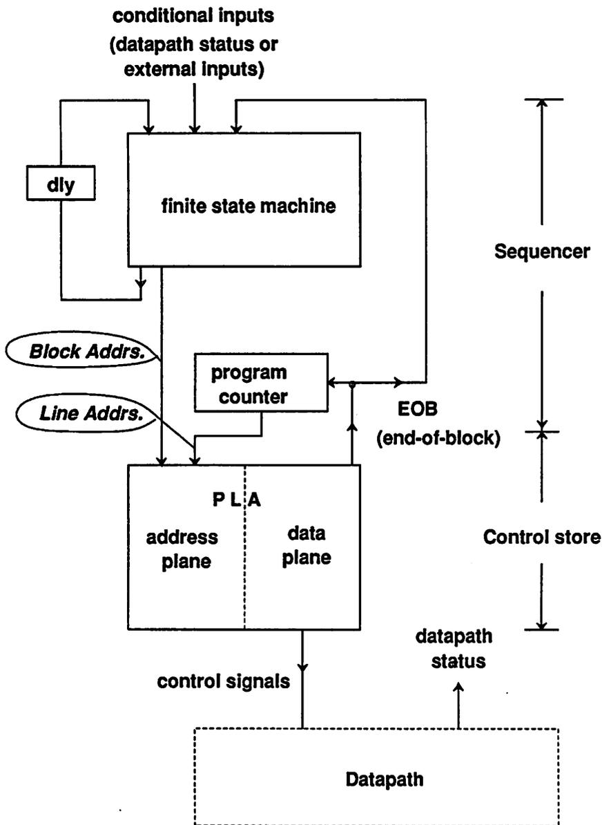
Figure 3.5: Block diagram of the basic control unit. The higher order bits (block address) of the control store address are provided by the fsm and the lower order bits (instruction line address) are provided by the program counter.
