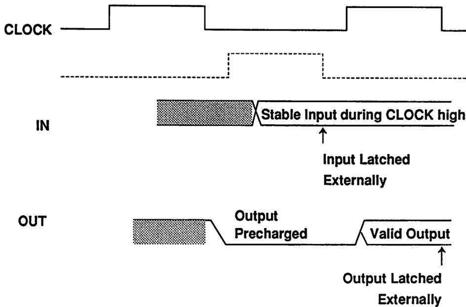
Figure 5.9: Timing diagram showing the operation of the control-store.
