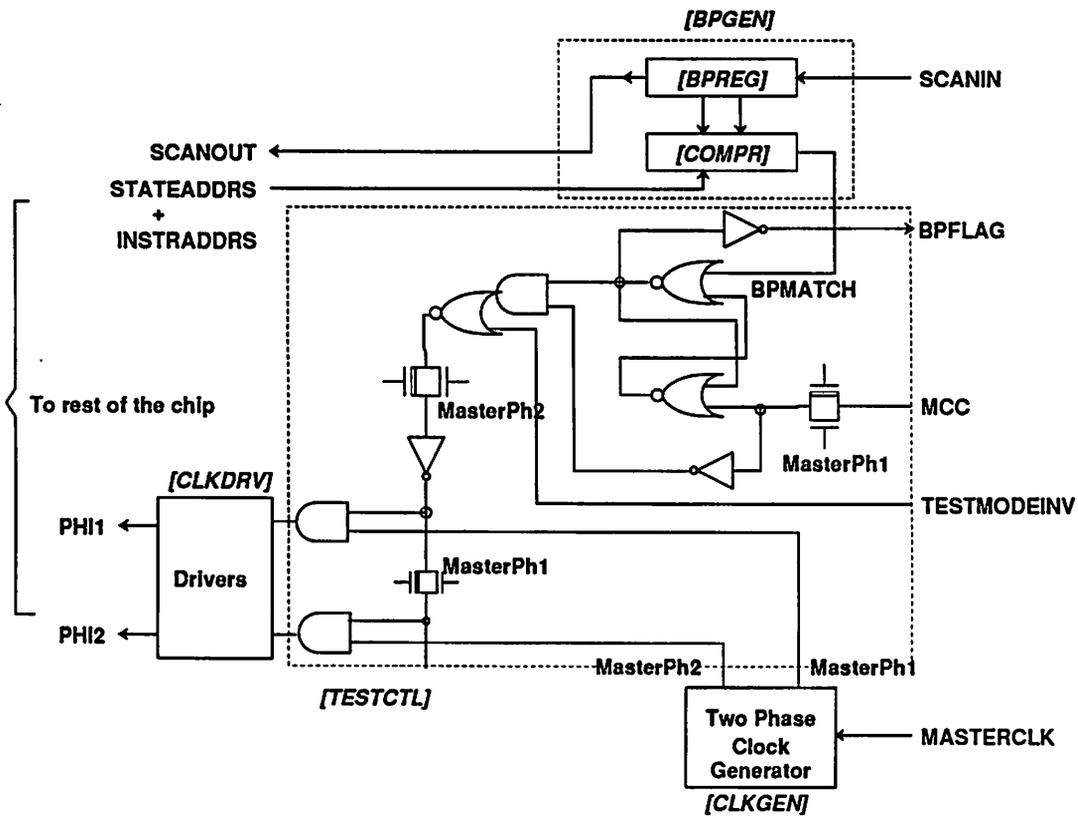
Figure 6.6: Schematic of the Test-logic macrocell.
