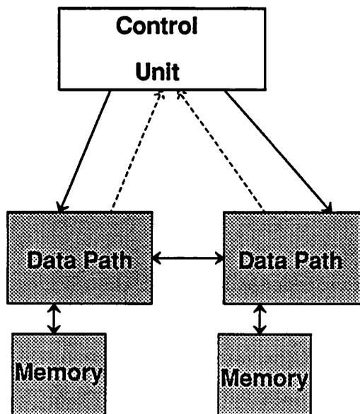
Figure 4.2: Architecture model consisting of a central control unit, application specific data paths, and memory.
