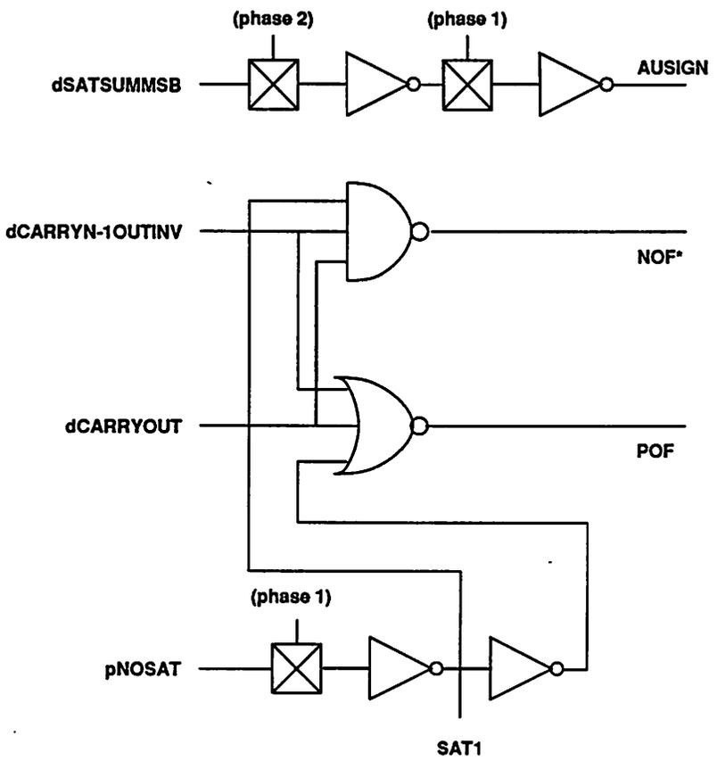
Figure 5.36: Control circuits for the saturation logic.
