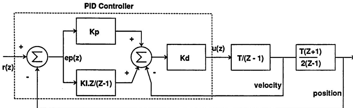
Figure 2.5: PID controller for a robot joint modelled as a double integrator.  $T$  is the sample period.
