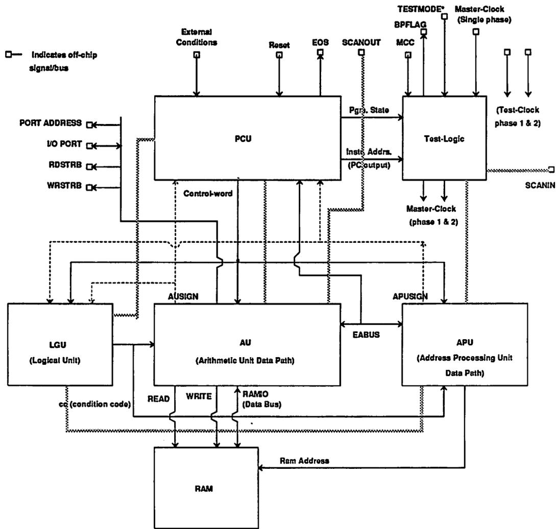
Figure 5.4: Top-level interconnection network of the processor. Dotted lines indicate data path status signals. Scan path connections are shown as cross-hatched lines.
