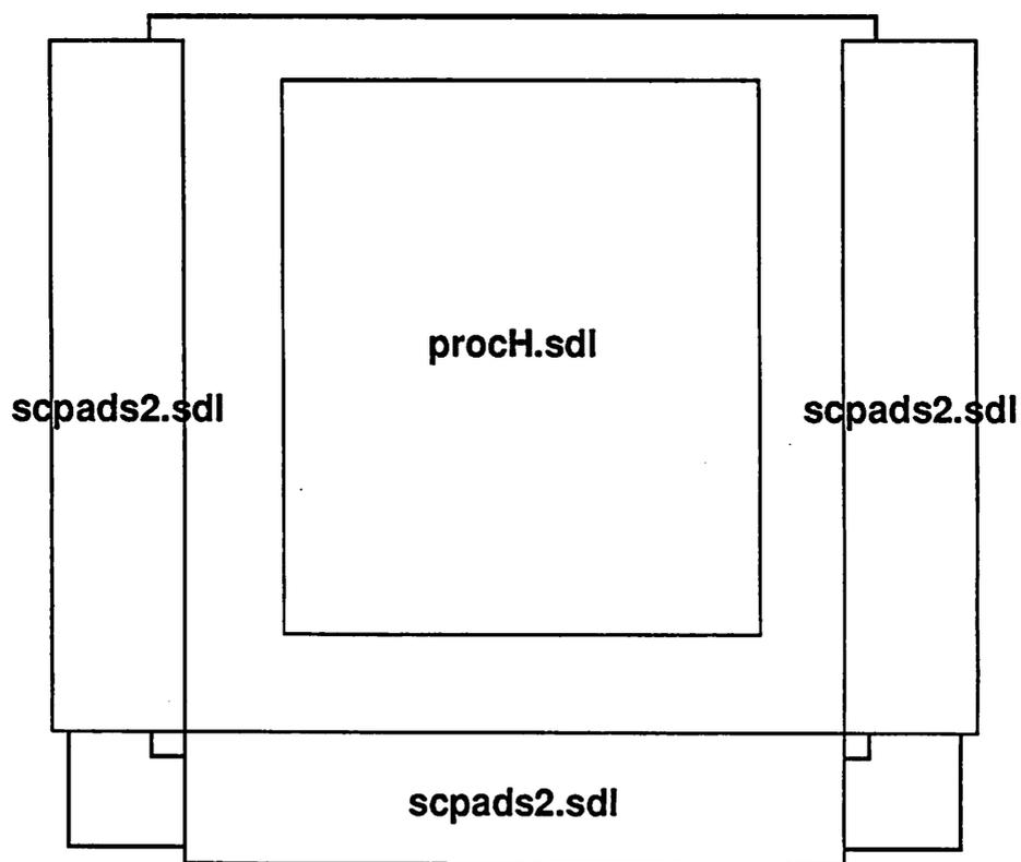
Figure 5.2: Top-level view of the robot controller chip layout showing three pad groups surrounding the core processor cell. The North pad group is deleted since it does not have any actual pads in this example.
