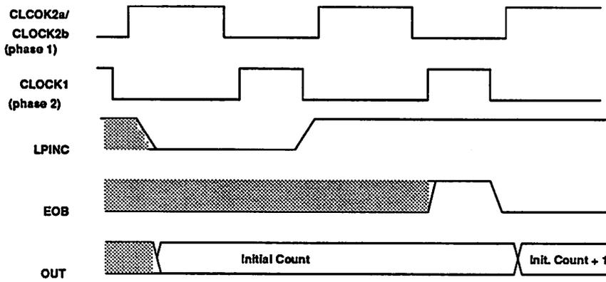
Figure 5.17: Timing diagram for loop counter.
