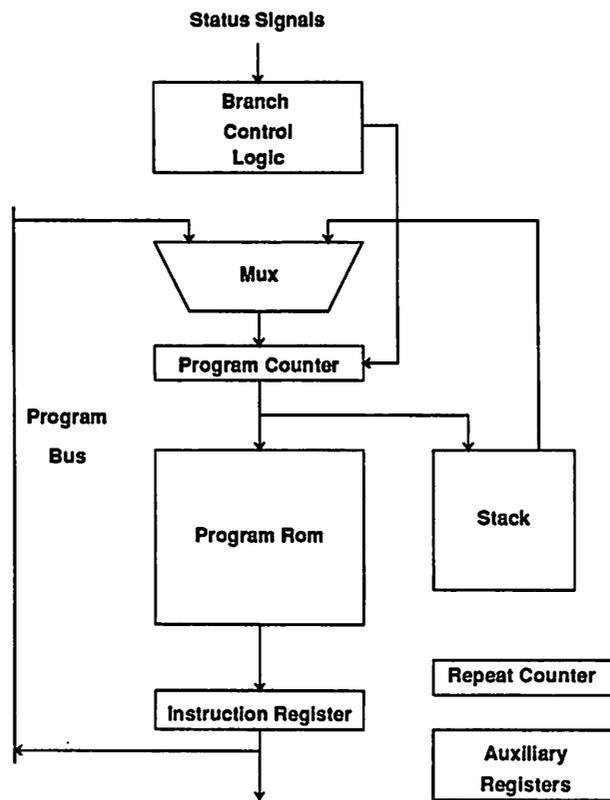
Figure 3.19: Block diagram of the TMS32020 control section.
