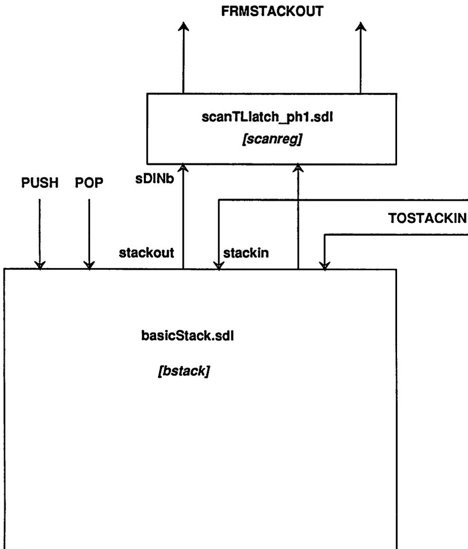
Figure 5.22: Stack-Macro consists of a basic stack and a scan-type latch.
