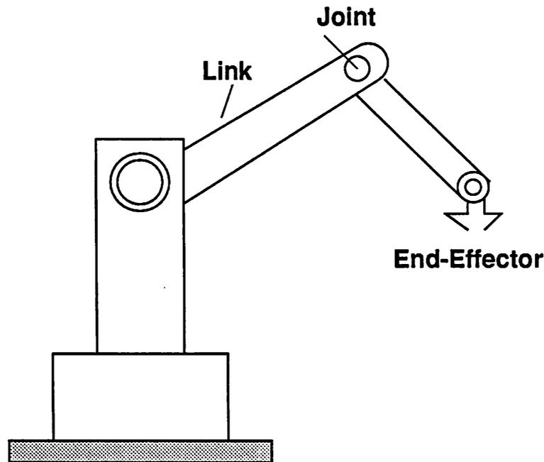
Figure 2.1: A robot arm consists of links and joints
