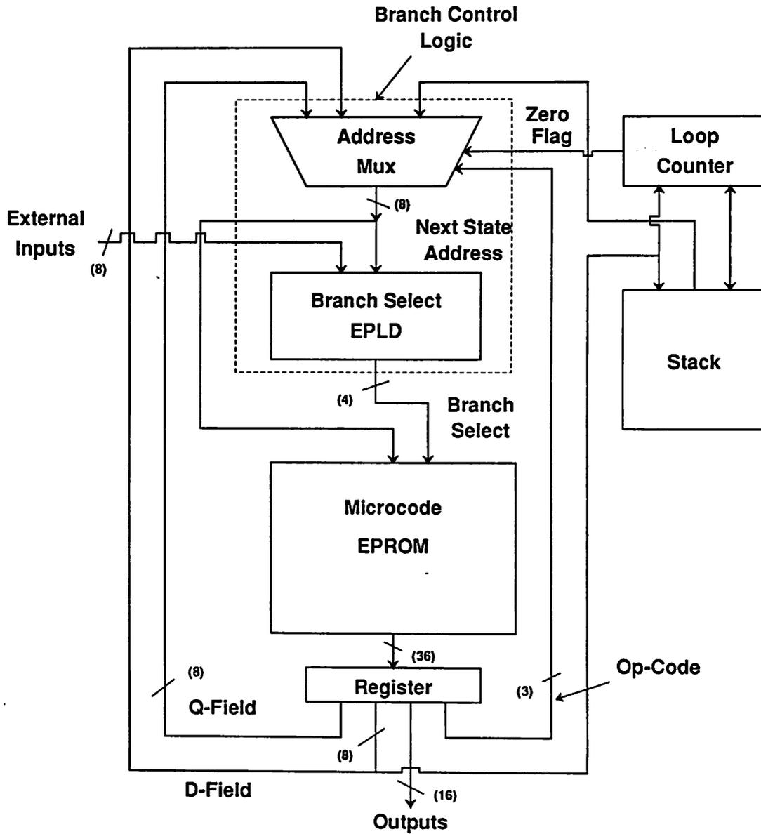
Figure 3.17: Block diagram of the recently introduced Altera EPS448 stand alone microsequencer (SAM). The operation of the SAM has many similarities with the PCU's operation
