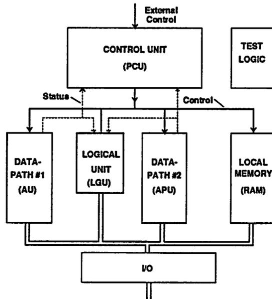
Figure 3.1: Processor architecture for the robot controller
