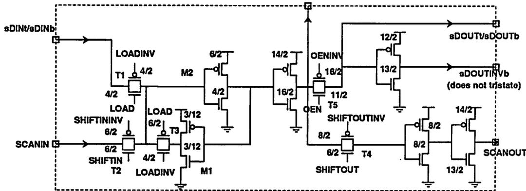
Figure 6.4: A two phase scan register.
