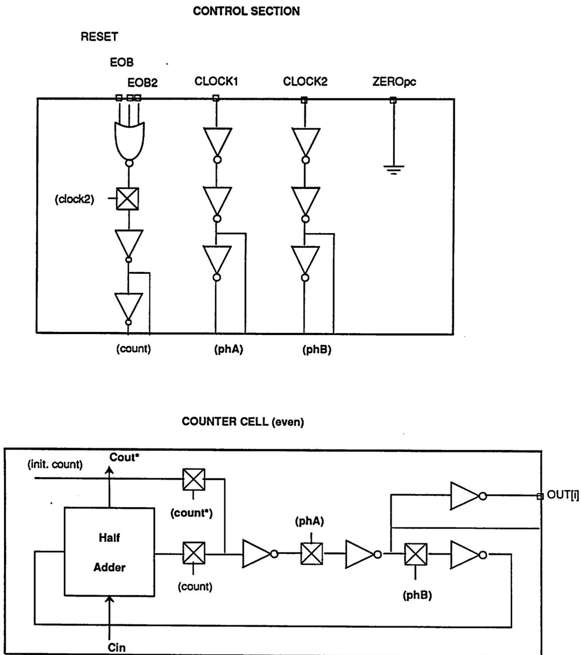
Figure 5.13: Control and counter circuit for the program counter.
