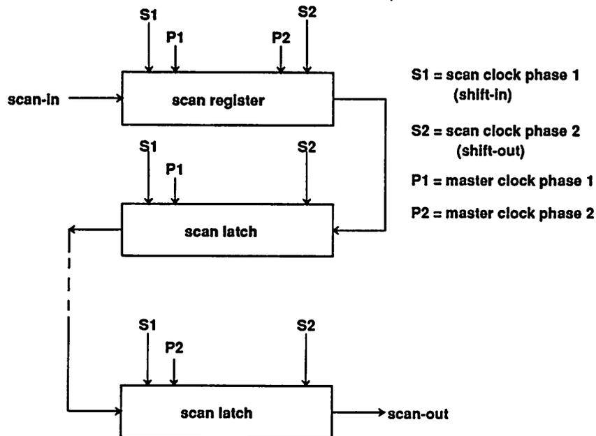
Figure 6.2: Hooking scan registers and latches into a serial scan path. Note the two scan latches in the figure operate on different clock phases during normal operation. By keeping the scan clock independent of the master clock, any timing conflicts that may arise due to serial connection of latches operating in different phases are avoided.
