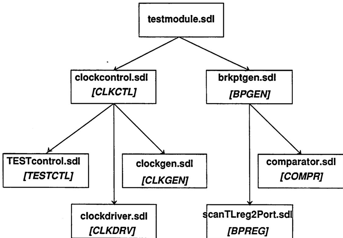
Figure 6.5: Cell hierarchy of the Test-logic macrocell.
