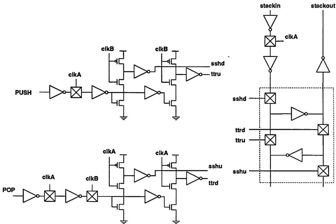
Figure 5.23: Circuit diagram of a stack cell and stack control circuits. The circuit within the dotted box contains the basic stack register cell. This cell is replicated horizontally for forming the stack word and vertically for increasing the stack depth.
