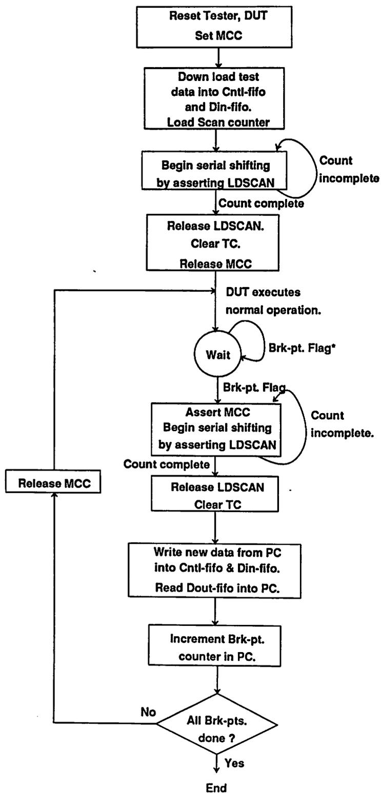
Figure 6.8: Flow chart for the testing procedure.
