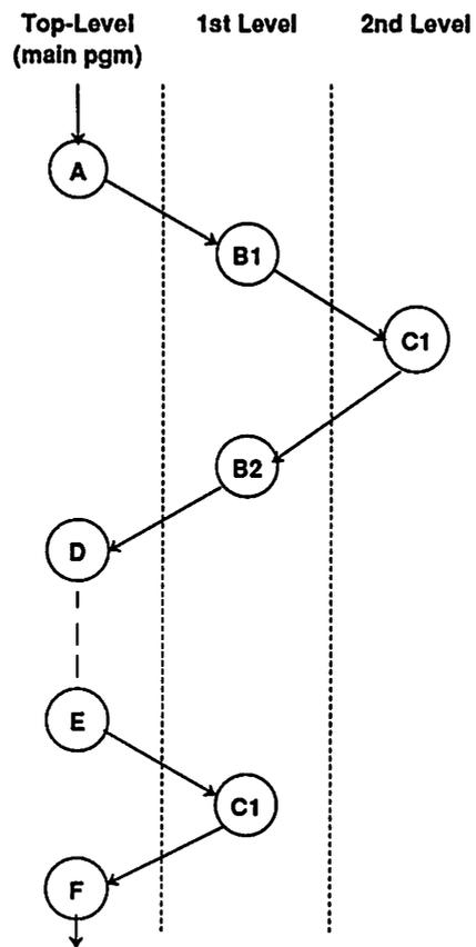
Figure 3.12: State diagram showing two levels of subroutine nesting. Total number of state entries is  $4 \times 2$  (for top-level states)  $+ 2 \times 2$  (for subroutine group B1-B2)  $+ 1 \times 2$  (for subroutine C1) = 14. A flattened state diagram would require  $8 \times 2 = 16$  state entries.
