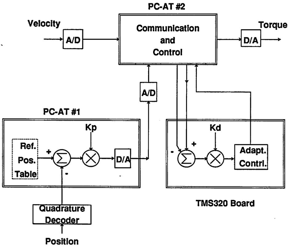
Figure 2.7: A TMS32010 based system implementing the adaptive control algorithm.
