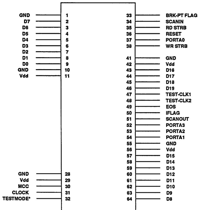
Figure 7.6: Pin out of the robot controller chip.
