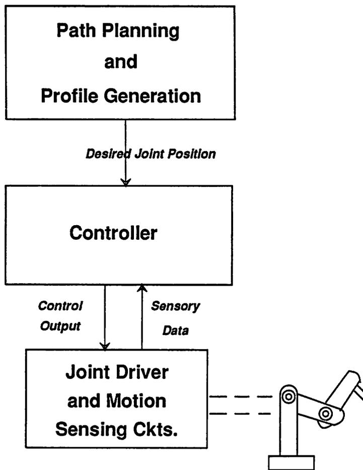
Figure 2.2: Robot control systems are hierarchically organized
