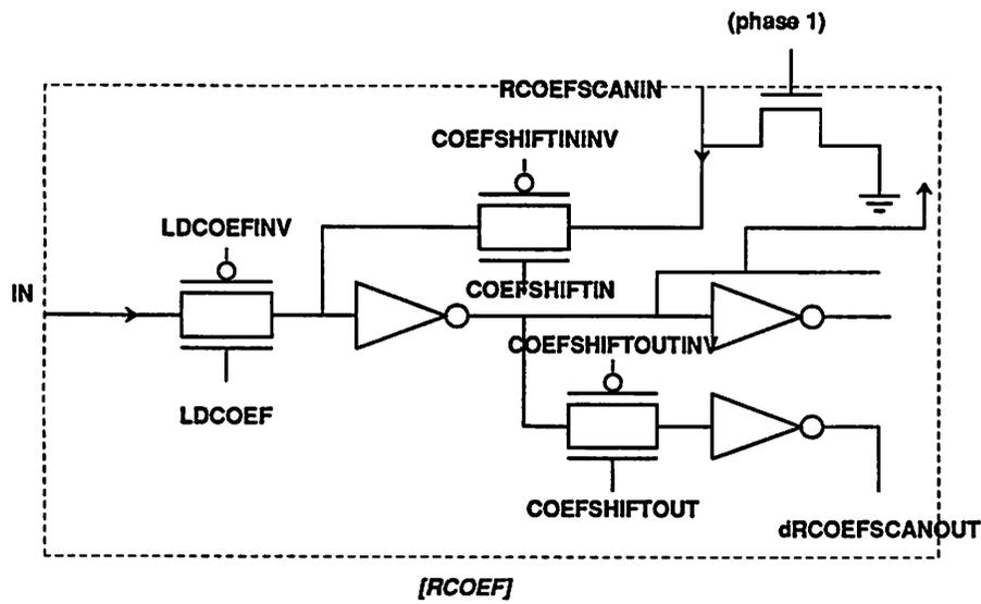
Figure 5.33: A scan-type latch is used as the coefficient register for multiplication.
