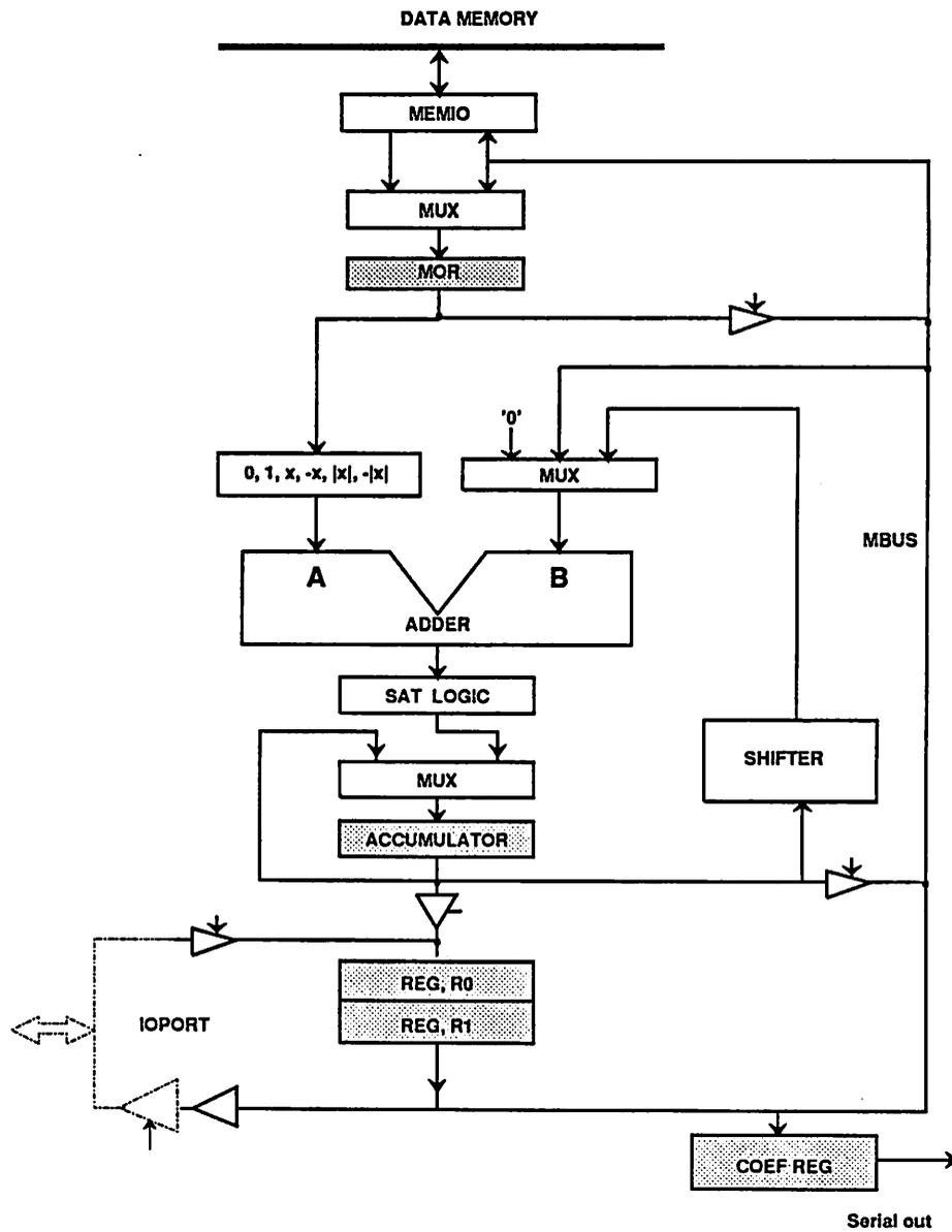
Figure 3.25: Block diagram of the data path.
