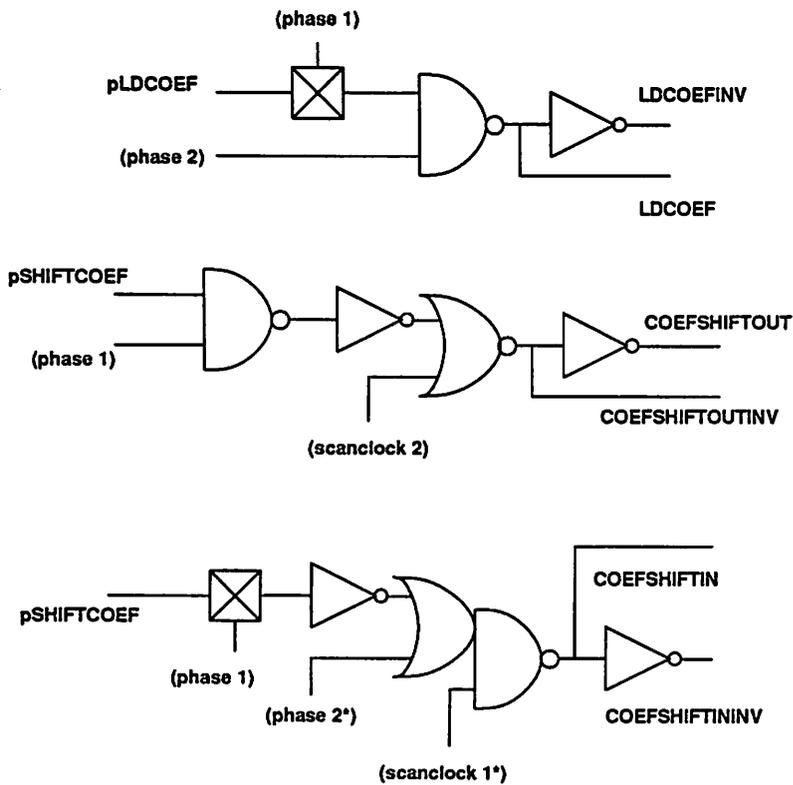
Figure 5.34: Control circuits for the coefficient register.
