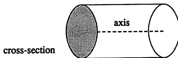
Figure 2.8: Sweeping rule: keep the cross-section constant and orthogonal to the axis.
