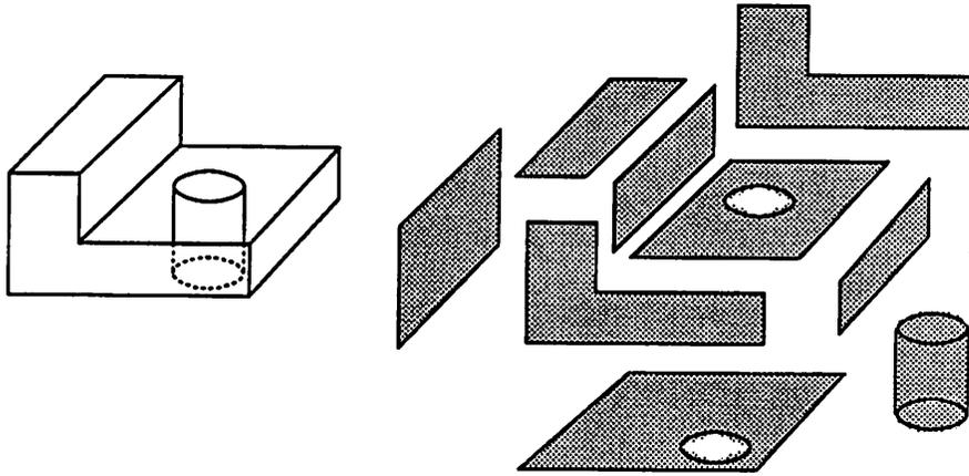
Figure 2.6: Surface boundary representation of a solid object (from [Requ83]).
