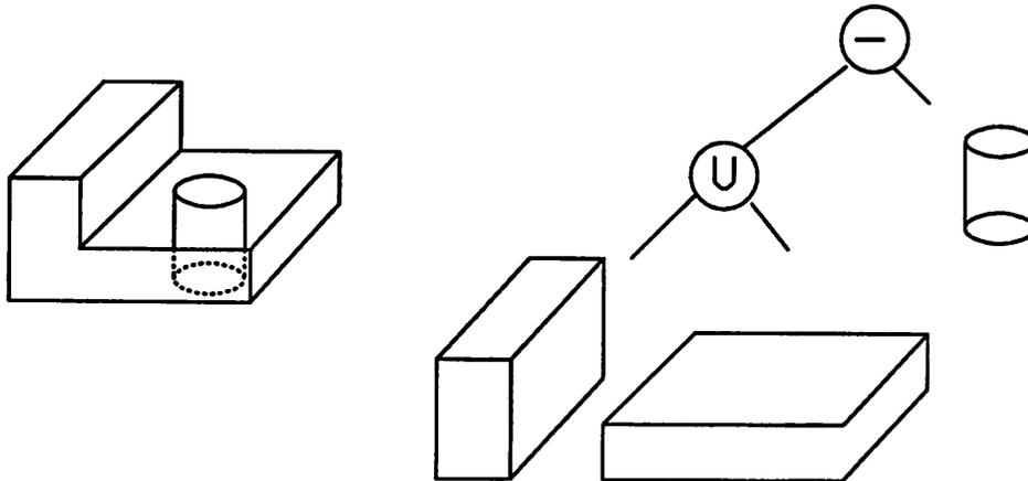
Figure 2.12: CSG representation of a solid object (from [Requ83]).
