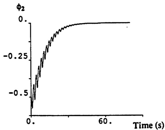
(b) Parameter Error  $\phi_2$
