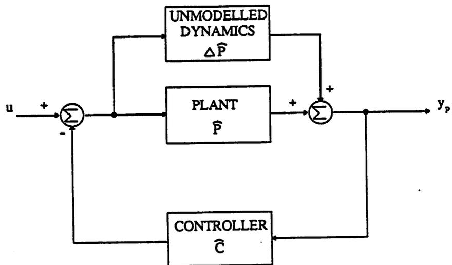
Figure 5.5.1  $^1$  S(P,C) Loop
