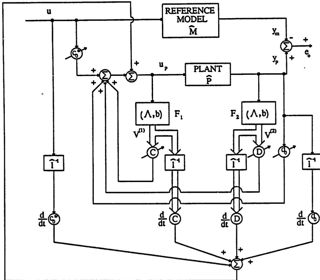
Figure 4.2.2 Modified Model Reference Adaptive Controller
