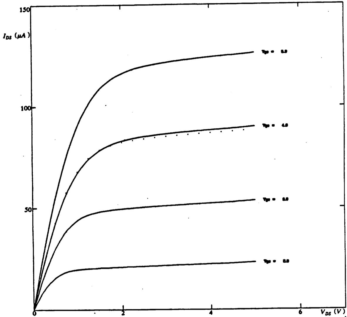
Example 3: Linear Interpolation -  $I_{DS}$  vs.  $V_{DS}$
