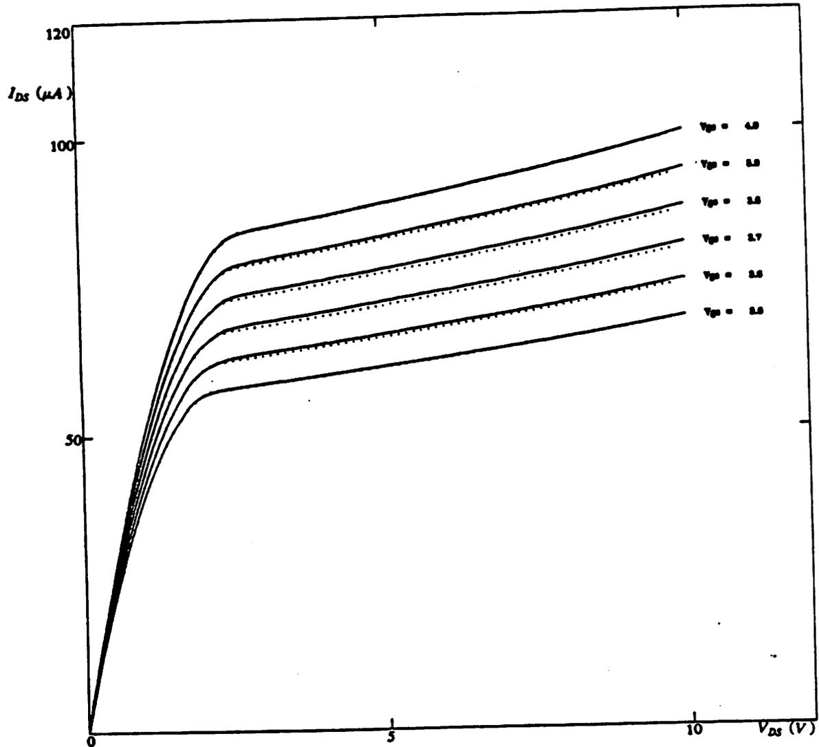
Example 2: Linear Interpolation -  $I_{ds}$  vs.  $V_{ds}$
