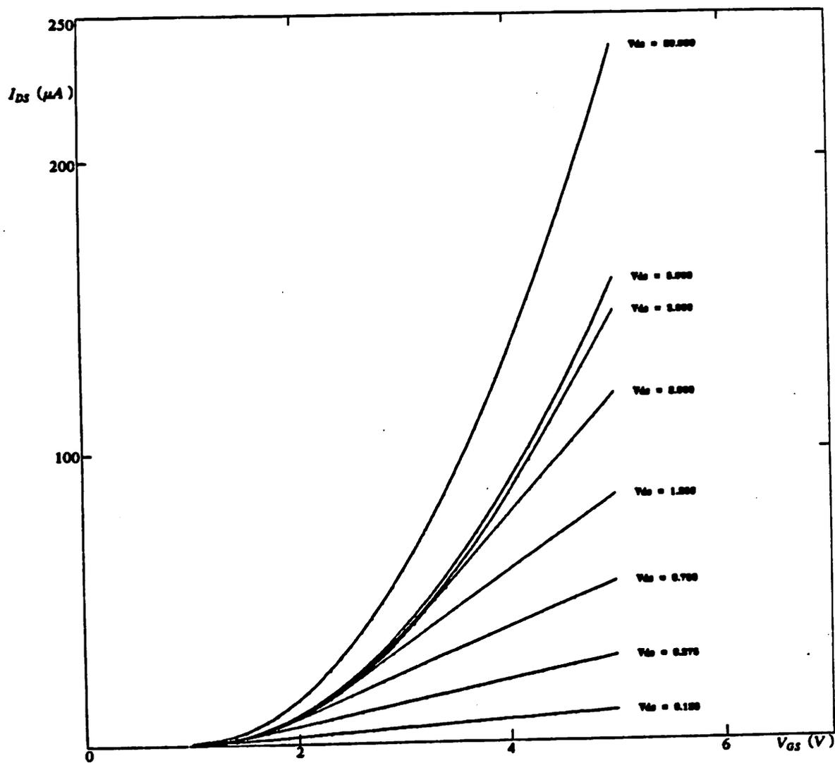
Example 2: Family of  $I_{ds}$  vs.  $V_{gs}$  Curves
