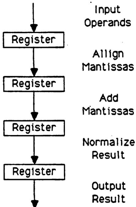
Pipelined Floating-Point Addition
