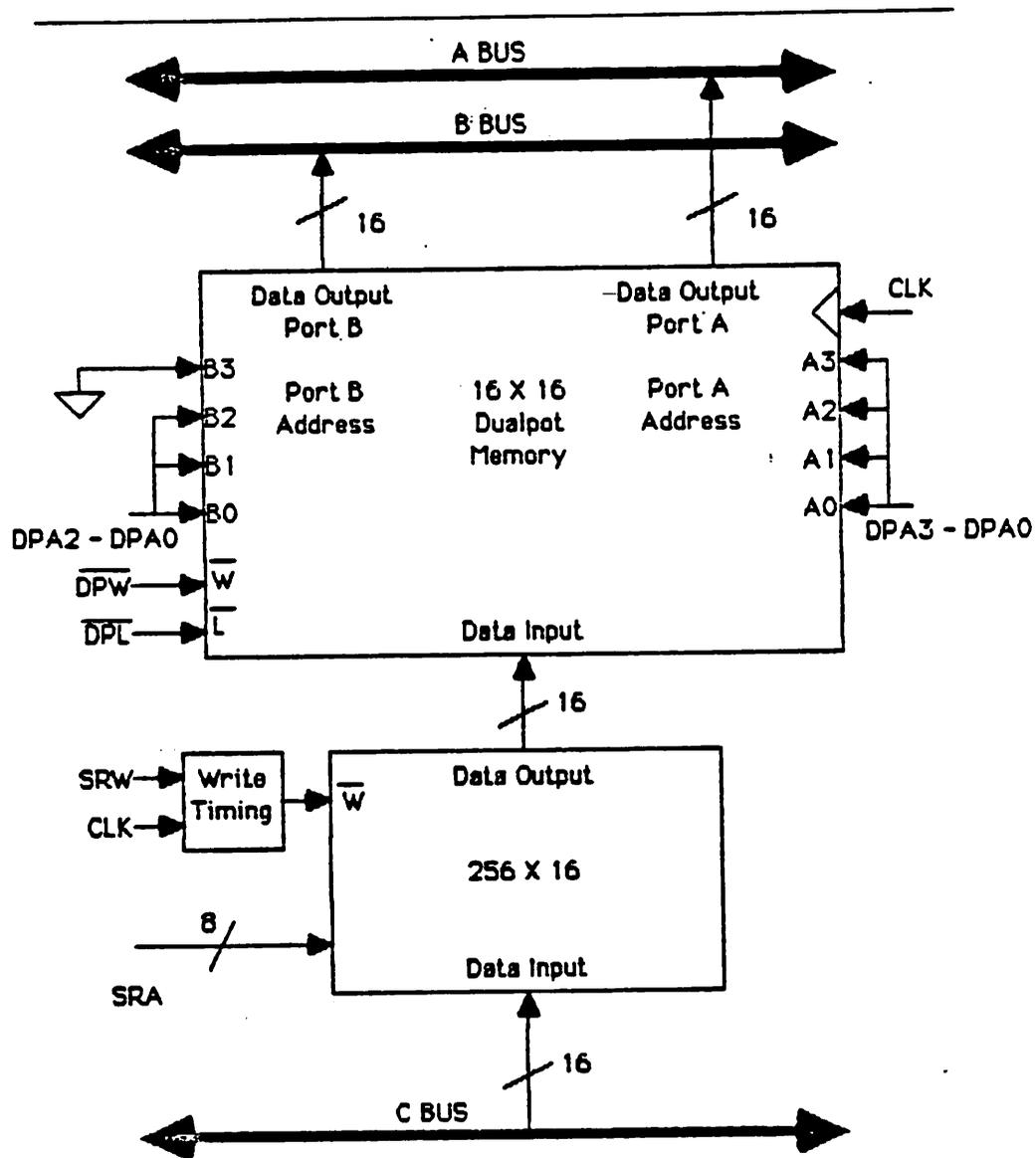
Block Diagram of the Coefficient Cache
