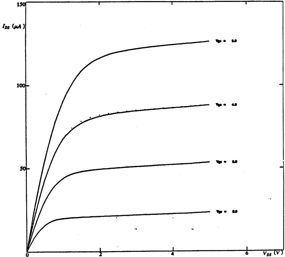
Example 3: Cubic Interpolation -  $I_{ds}$  vs.  $V_{ds}$
