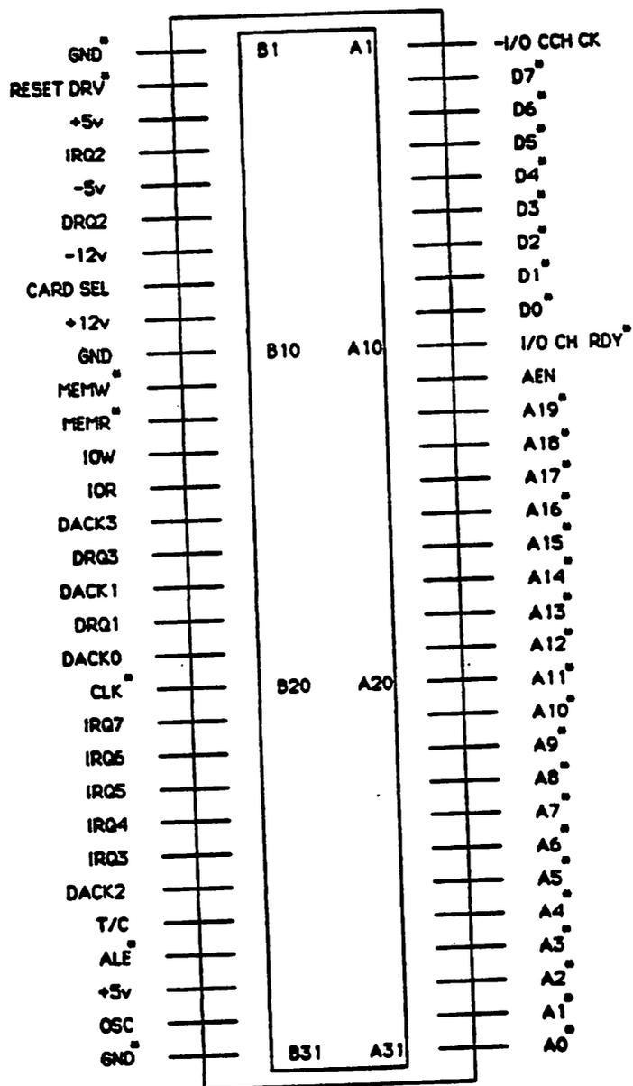
Diagram of the IBM PC Bus [IBM84]
