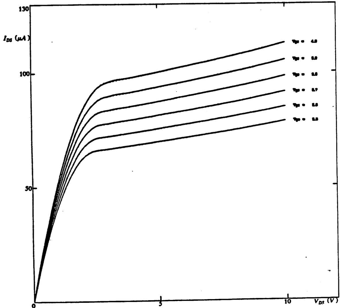
Example 1: Cubic Interpolation -  $I_{ds}$  vs.  $V_{ds}$
