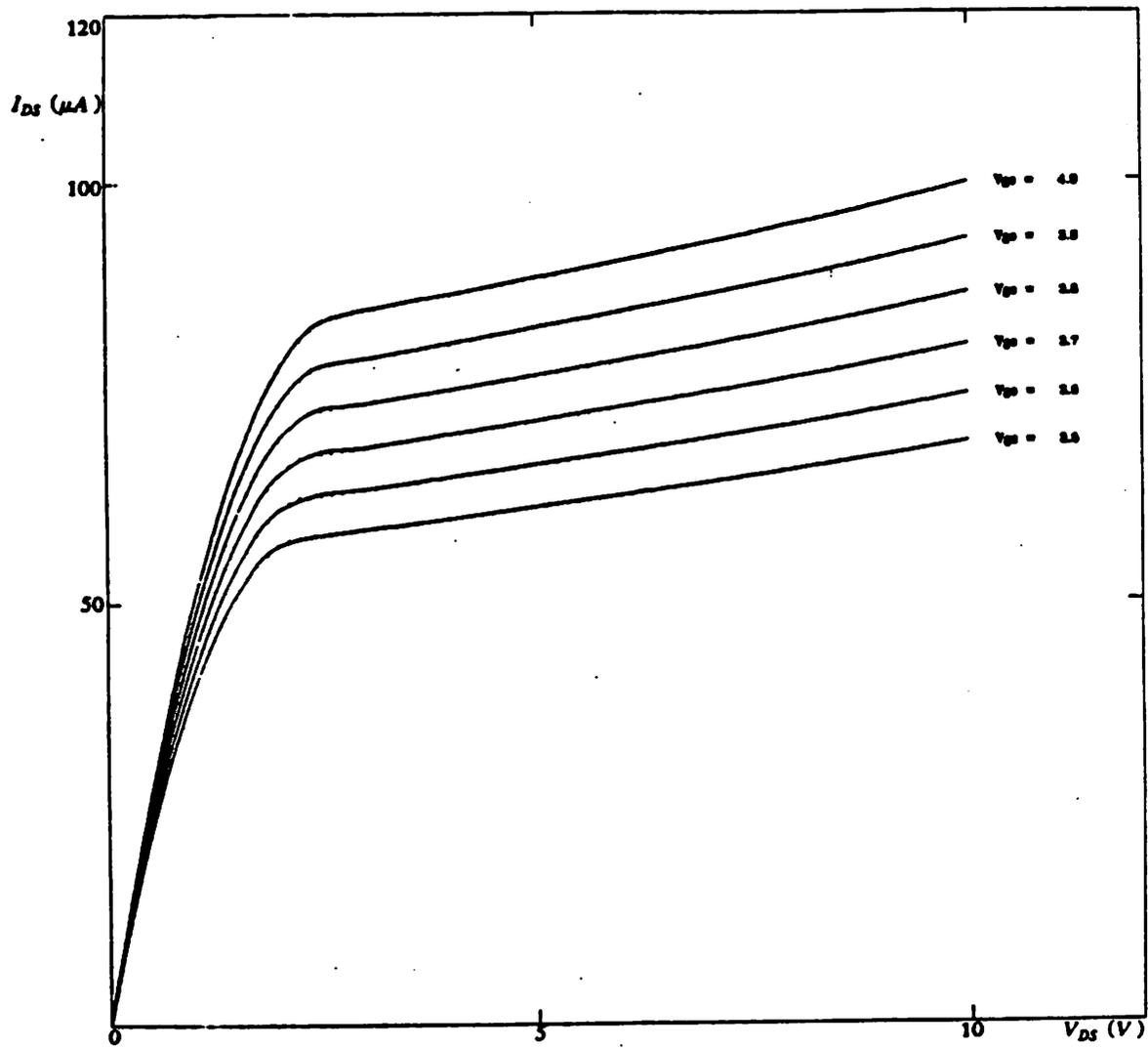
Example 2: Cubic Interpolation -  $I_{ds}$  vs.  $V_{ds}$
