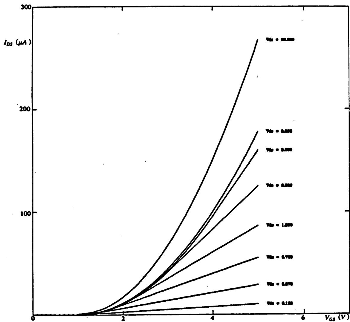
Example 1: Family of  $I_{ds}$  vs.  $V_{gs}$  Curves
