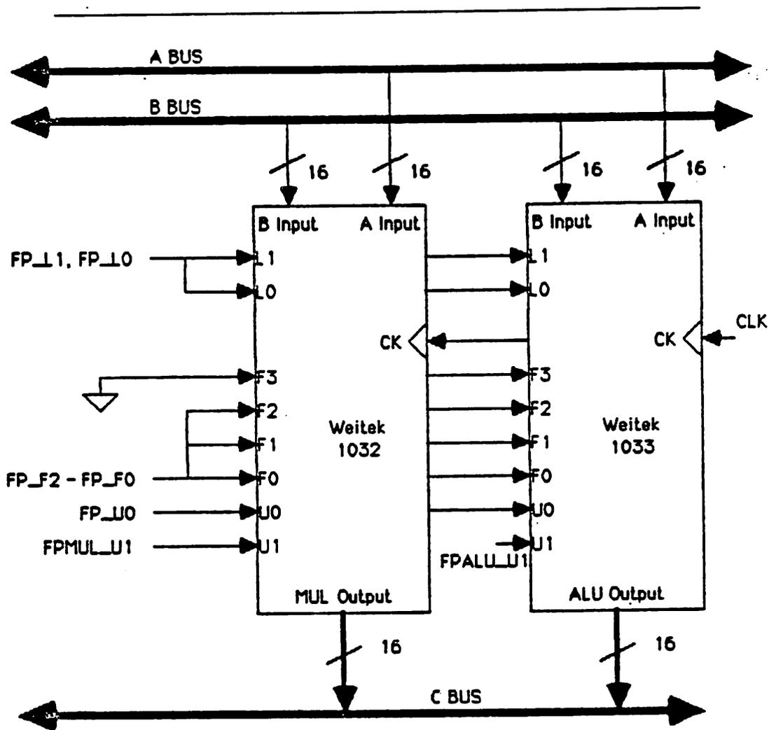
Block Diagram of the Floating-Point Unit
