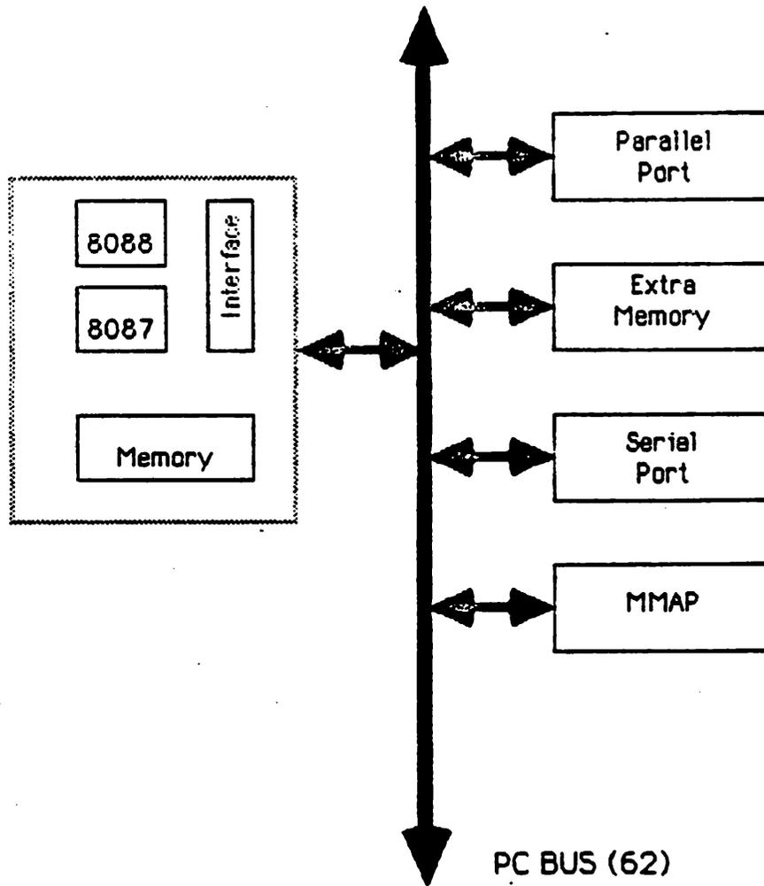
IBM PC-XT With Prototype MMAP
