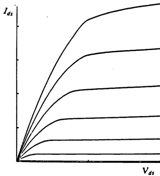
$I_{ds}$  vs.  $V_{ds}$
