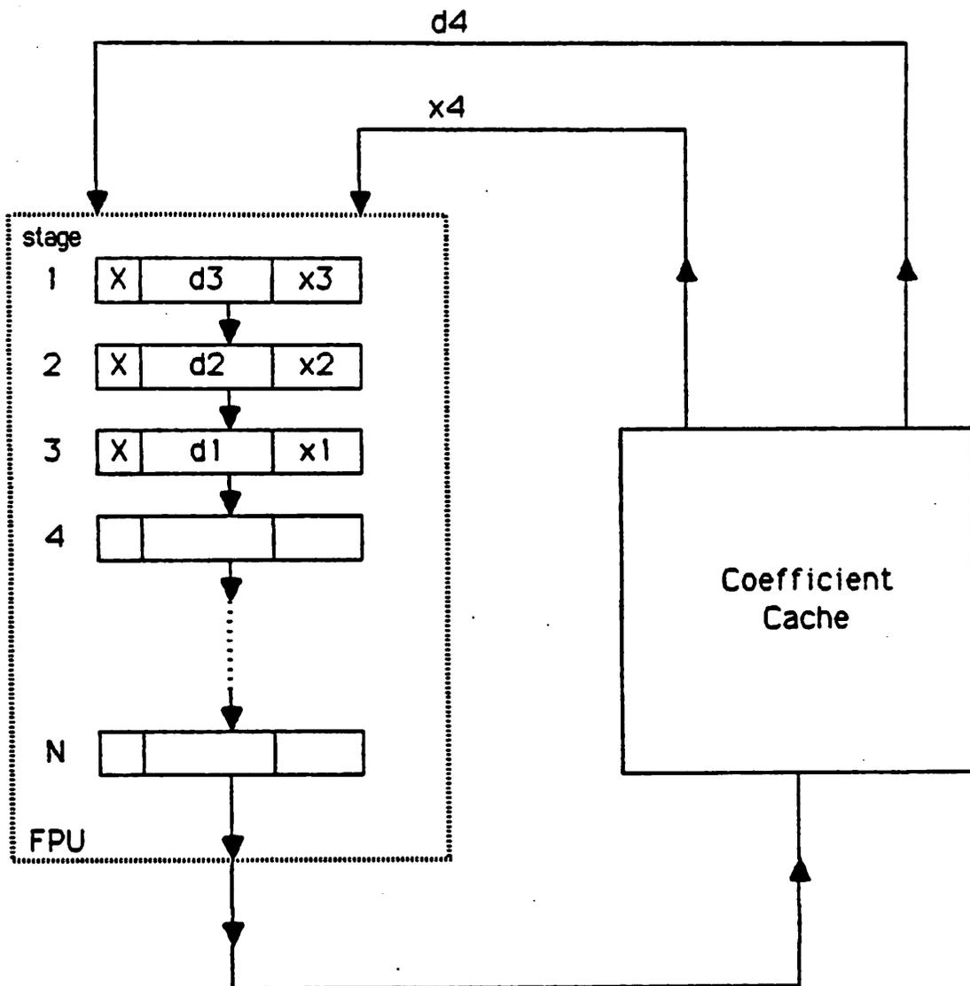
Loading the FPU's Pipeline
