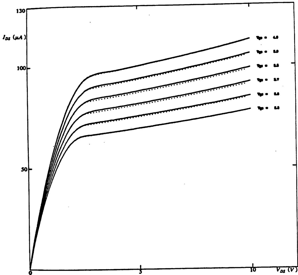
Example 1: Linear Interpolation -  $I_{ds}$  vs.  $V_{ds}$
