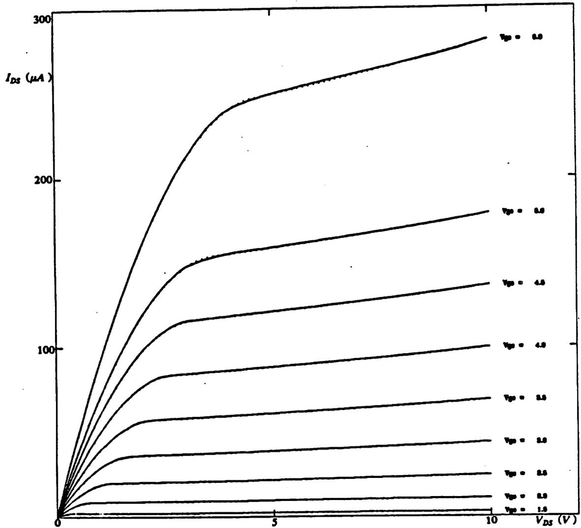
Example 2: Family of  $I_{ds}$  vs.  $V_{ds}$  Curves
