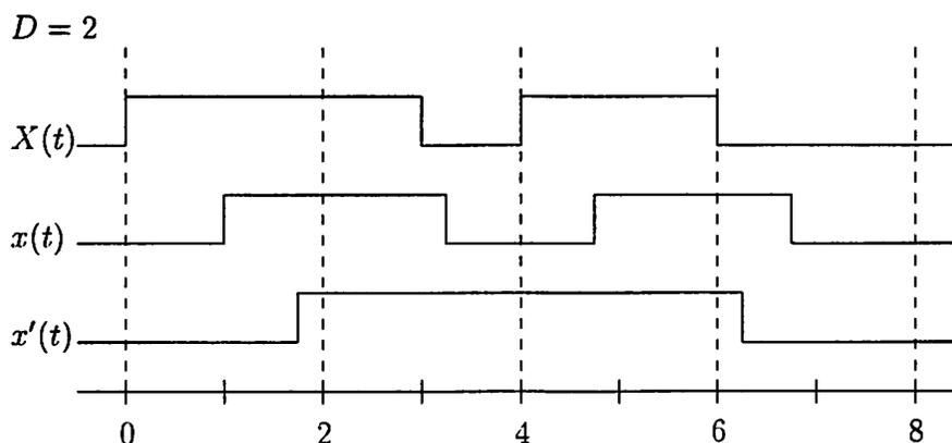
Figure 8: Up-bounded inertial delay waveforms.
