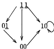
Figure 13: Possible state sequences over  $qz$ , for the RS-latch with input  $rs = 01$ .
