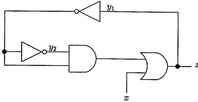
Figure 10: Different placement of delay elements affects output value.
