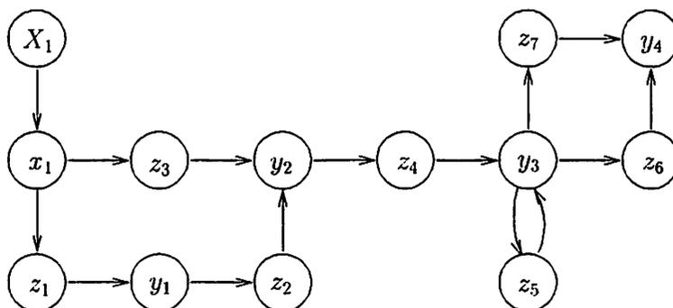
Figure 5: Circuit graph corresponding to the gate circuit in Figure 4 (Figure 4.6 from [4].)
