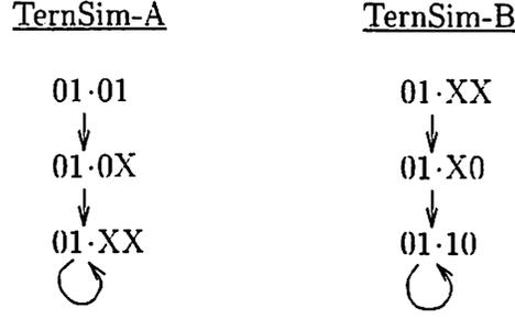
Figure 17: TernSim-A and TernSim-B in operation on the RS-latch, over states  $rs \cdot qz$ .
