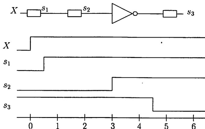
Figure 9: A UIN-history( $N, D, 1$ );  $D_1 = 1$ ,  $D_2 = 3$  and  $D_3 = 2$ . Delay elements are associated with the state vertices  $s_1, s_2$  and  $s_3$ .
