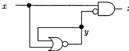
Figure 1: Well-behaved, even though  $y$  oscillates when  $x = 0$  (Figure 4b from Malik [13]).
