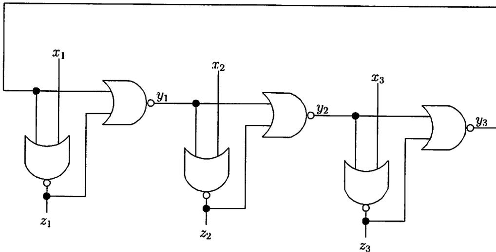
Figure 19: Kautz's circuit with a combinational cycle.
