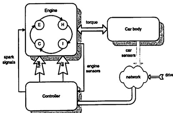
Figure 1.1: An engine control system
