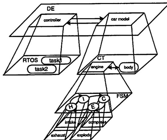
Figure 1.2: A hierarchical model for the engine control system
