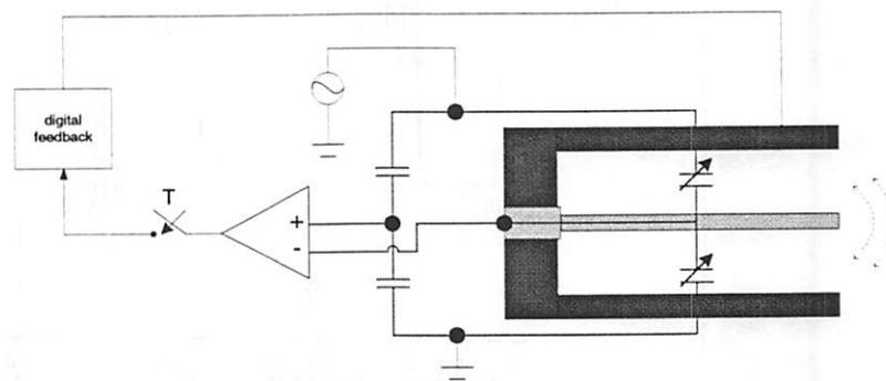
Figure 4.11: A physical structure illustrating a micro-accelerometer.
