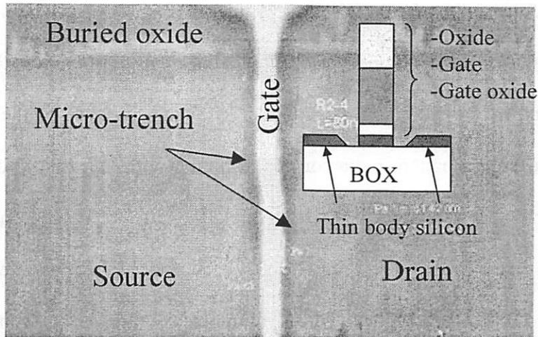
Figure 4.10 Top view of SEM photograph showing the gate and thin body silicon profile after the gate plasma etch with  $\text{CF}_4$  causing micro-trench. Inset is the cross-sectional diagram of the SEM photograph.
