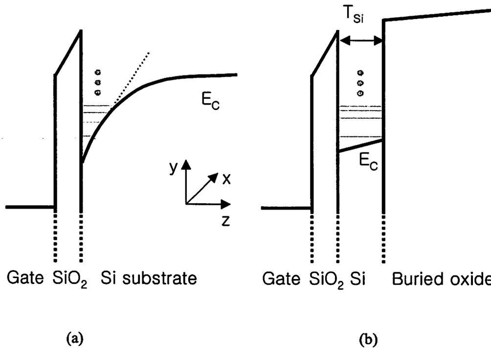
Figure 5.2 Energy band diagrams and eigen-energy states in (a) bulk MOSFET with heavily doped body and (b) ultra-thin body (UTB) MOSFET with lightly doped body.
