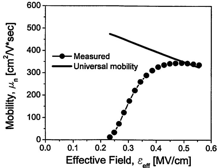
Figure 4.28 Electron mobility versus effective electric field.
