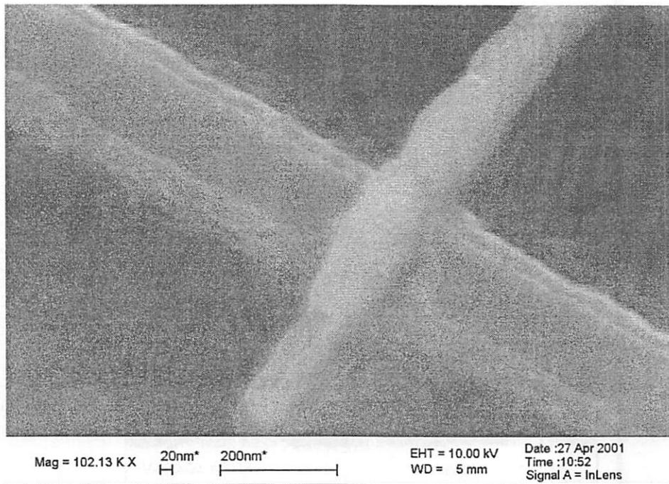
Figure 6.14 Bi-layer spacer profile after nitride plasma and HF wet etch.
