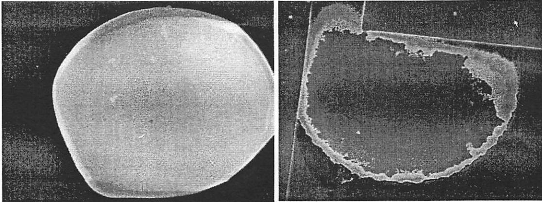
(a) SEM picture of bubble after RTA at 900°C for 1min
