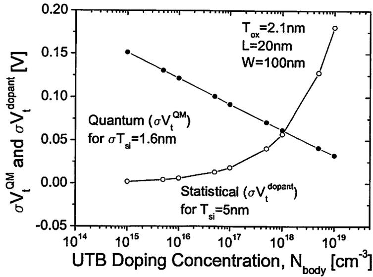
Figure 5.8 Standard deviation of threshold voltage induced by fluctuations in body thickness (solid circle) and body dopant concentration (open circle).
