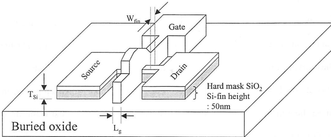
Figure 6.12 FinFET structure using e-beam lithography
