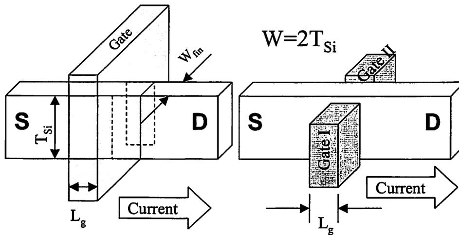
Figure 6.4 3-dimensional view of the FinFET structure.
