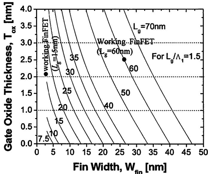
Figure 6.16 Contour plot of gate length versus a gate oxide thickness and silicon body thickness ( $W_{fin}$  in FinFET) for double gate MOSFETs (Adapted from [6.38]).
