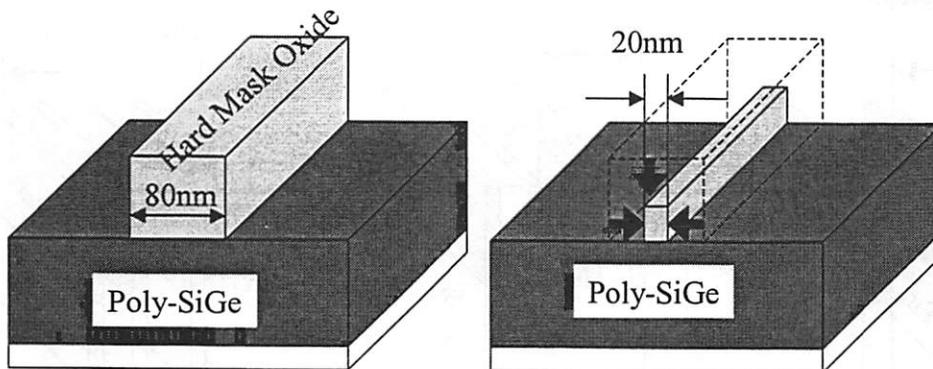
(c) After oxide hard mask etching (d) After hard mask oxide trimming with HF
