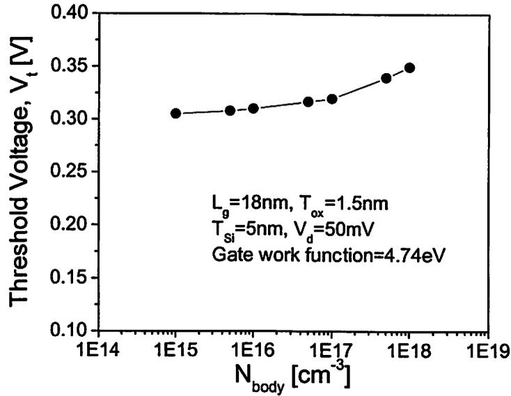
Figure 4.5 Threshold voltage behavior of NMOS relying on a body doping concentration.
