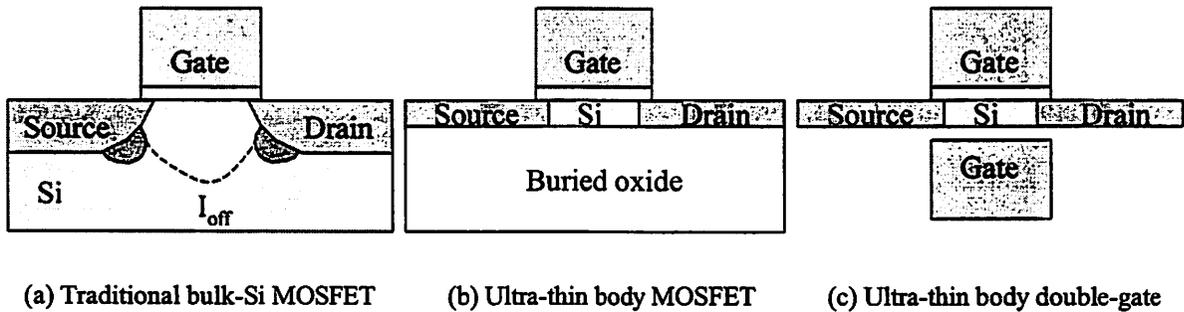
Figure 1.3 Cross-sectional schematic diagrams showing several novel device structures.
