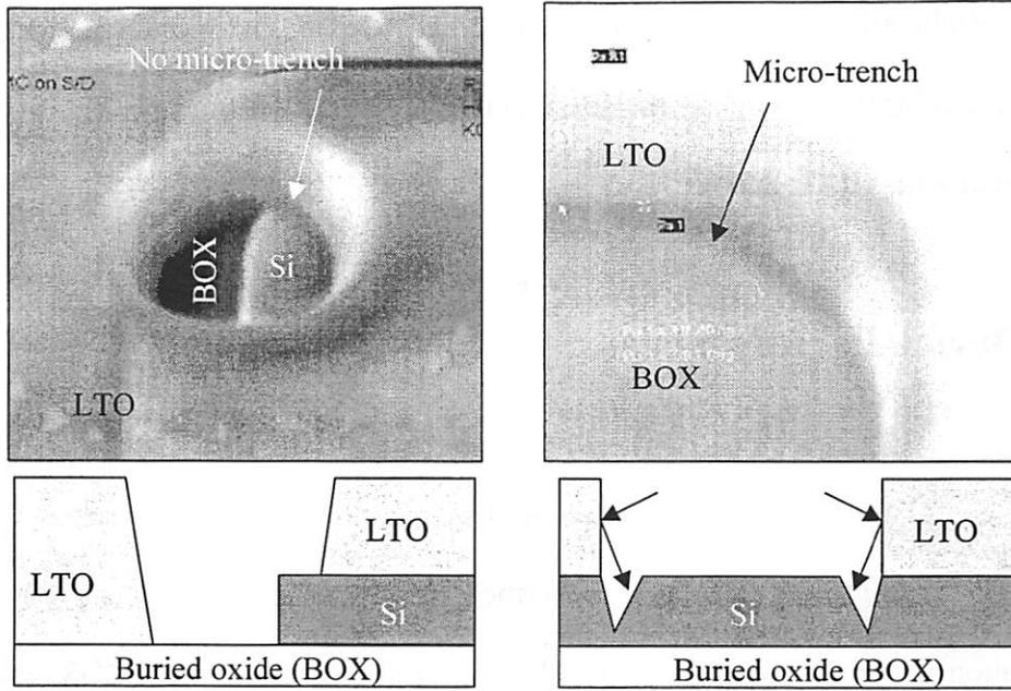
(a) Tilted SEM view of metal contact hole without micro-trench
