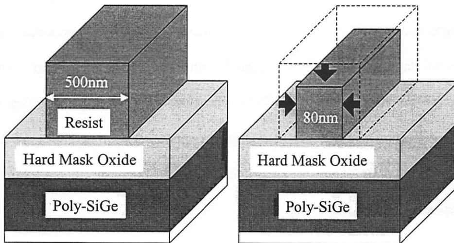
(a) After mask with i-line lithography (b) After resist ashing with O<sub>2</sub> plasma
