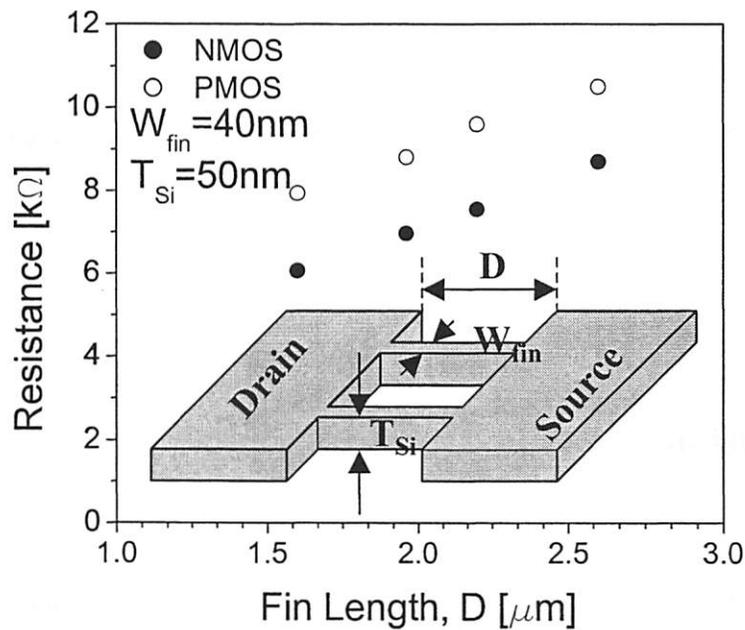
Figure 6.41 The total resistance of the fin is proportional to the fin length, D.
