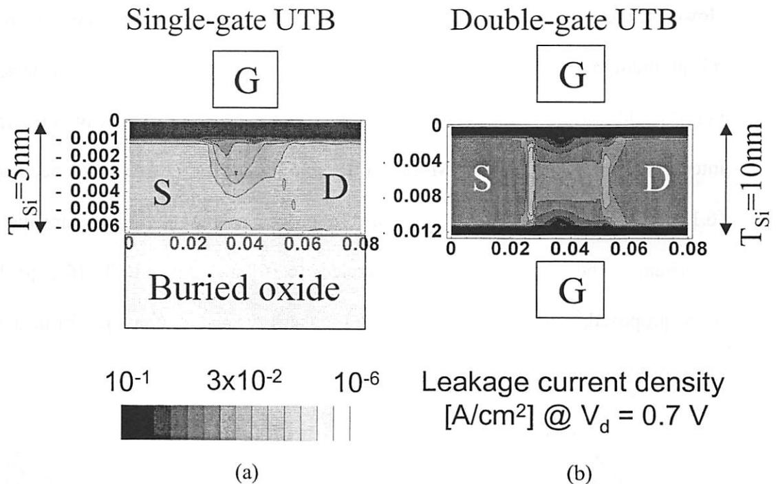
Fig. 6.2 Comparison of leakage current density for (a) single-gate MOSFETs with 5nm UTB and (b) double-gate MOSFETs with 10nm UTB ( $V_g=0V$ ,  $L_g=25nm$ ,  $T_{ox}=1.5nm$ ,  $N_{body}=1.0 \times 10^{15} cm^{-3}$ ).
