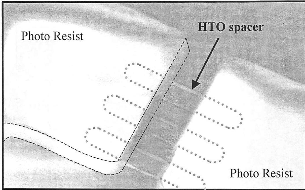
Figure 2.15 Tilted SEM photographs of HTO spacers for narrow fins and resists for S/D contact pads.
