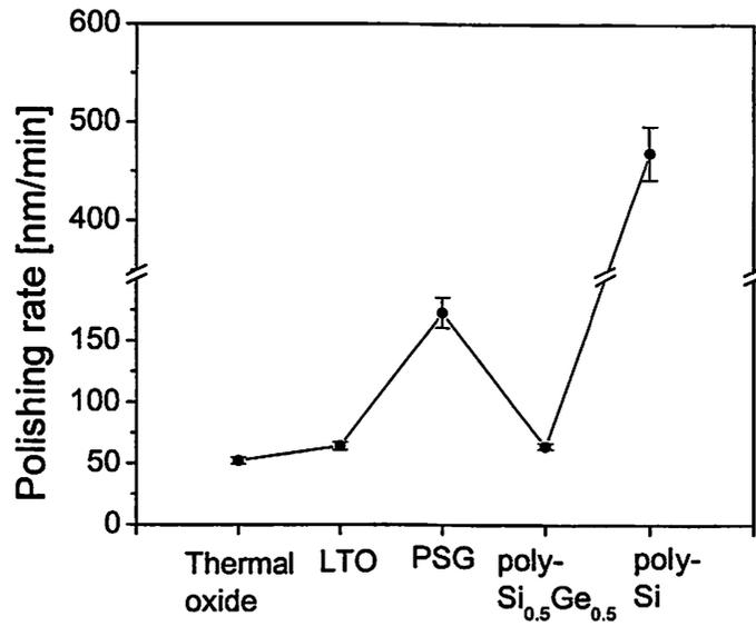
Figure 3.20 Polishing rates of thermal oxide, LTO, PSG, poly-Si<sub>0.5</sub>Ge<sub>0.5</sub>, and poly-Si.
