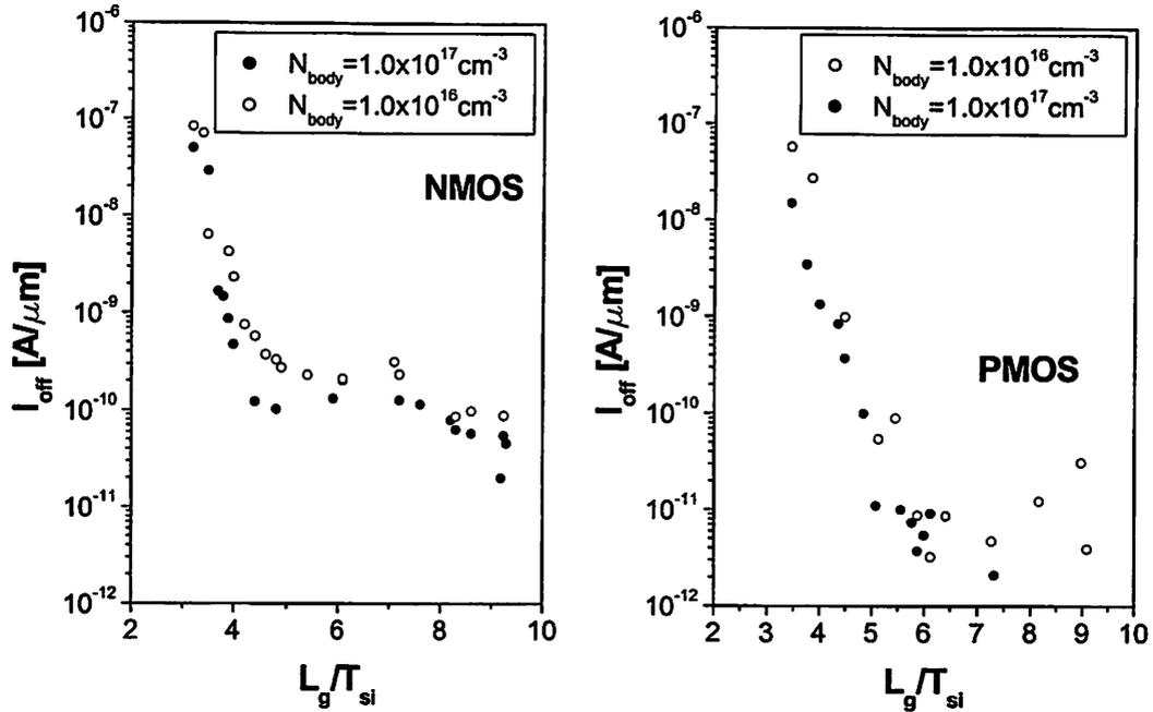
Figure 4.25 Off-state leakage current versus  $L_g/T_{Si}$ .
