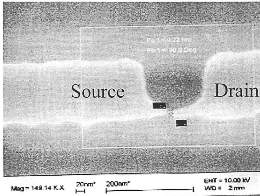
Figure 6.11 SEM top view of a sub-10nm width silicon fin.
