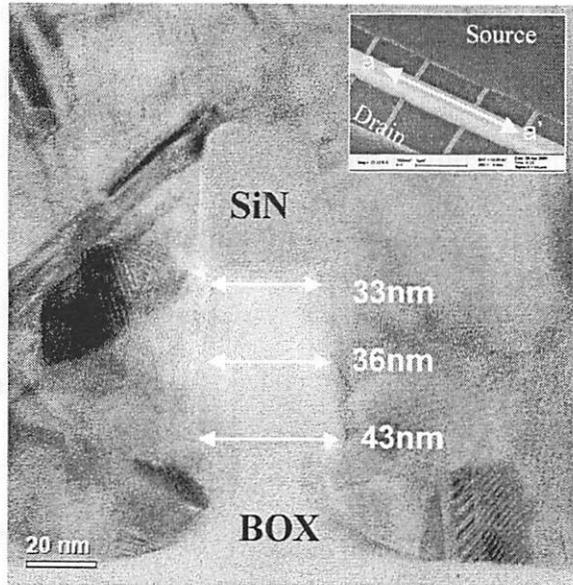
Figure 6.30 Cross-sectional TEM photograph of the silicon fin with a nitride hard mask along the a-a' direction in the inset.
