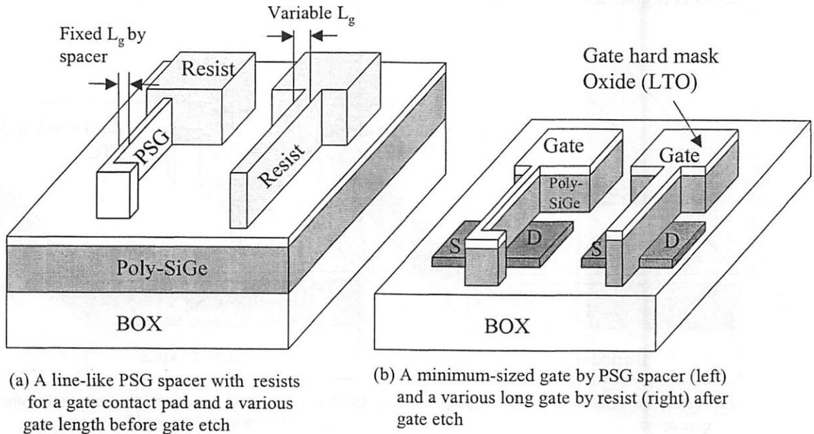
Figure 2.20 Schematic diagrams of (a) a line-like PSG spacer with a resist for gate contact pad (left), and a resist for a various and longer gate length (right) and (b) a minimum sized gate by PSG spacer (left), and a various and longer gate by resist (right).
