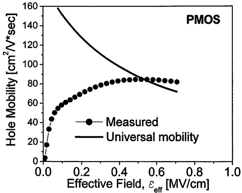
Figure 6.24 Measured hole mobility versus universal mobility (number of fins=150,  $W_{fin}=26\text{nm}$ ,  $T_{Si}=50\text{nm}$ ,  $L_g=14\mu\text{m}$ ,  $T_{ox}=2.1\text{nm}$ , and  $N_{body}=2.0 \times 10^{18} \text{cm}^{-3}$ ).  $\eta=1/4$  is used for holes.
