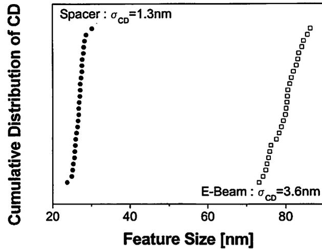
Figure 2.10 Measured CD uniformity of Si fin after Si fin etch and gate resist after e-beam lithography across a 4 inch wafer. CD uniformity by the spacer lithography is better than that by the e-beam lithography.
