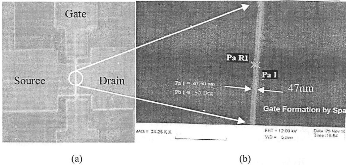
Figure 2.21 Optical microscope photograph (left) and SEM photograph (right). 47nm gate length was defined by a line-like PSG spacer.
