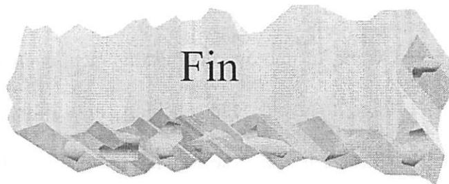
Figure 6.9 The silicon fin surface is rough due to lithography and plasma etch. The uneven profile along the fin is caused by a line edge roughness of the resist in lithography while further roughness is caused by etch damage.
