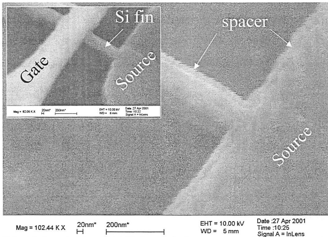
Figure 6.35 Tilted SEM photograph of spacer profile.
