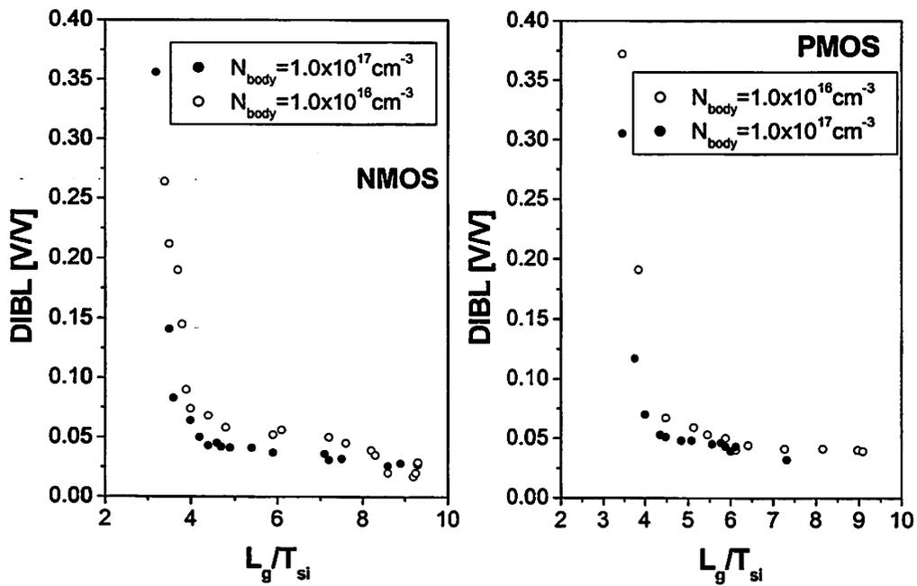
Figure 4.24 Drain induced barrier lowering (DIBL) versus  $L_g/T_{Si}$ .
