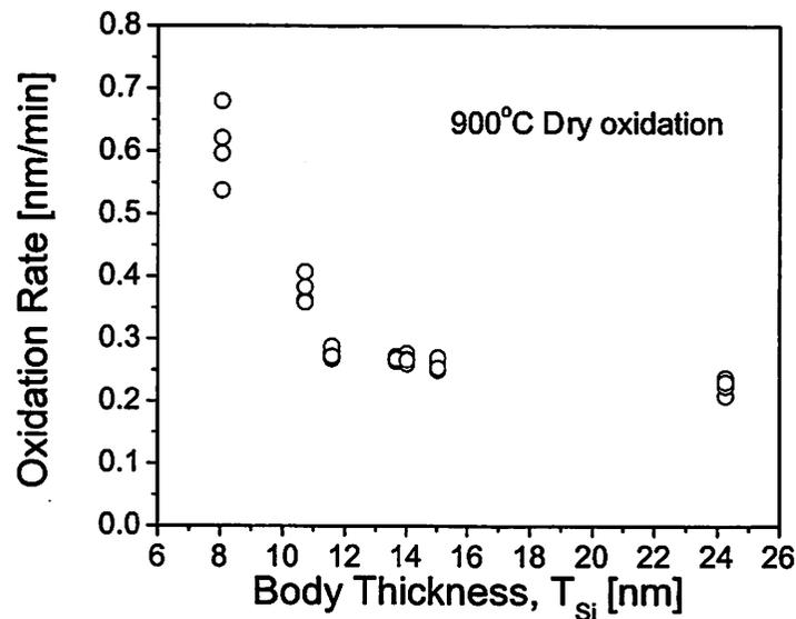
Figure 4.9 Oxidation rate vs. the thin thickness. One circle is the 5 die average value in a 4-inch wafer.
