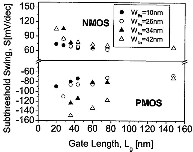
Figure 6. 19 Subthreshold swing versus gate length. A narrower fin width shows lower subthreshold swing.
