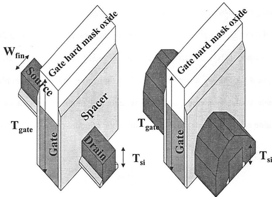
Figure 6.15 Schematic structures after spacer formation and selective Ge deposition.
