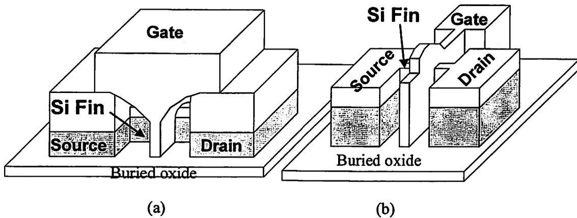
Figure 6.5 3-dimensional view of (a) original FinFET device [6.17][6.18] and (b) new FinFET device [6.23].
