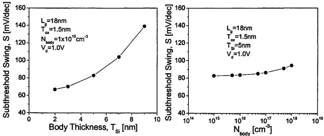
Figure 4.4 Subthreshold swing dependence on body thickness and body doping concentration.
