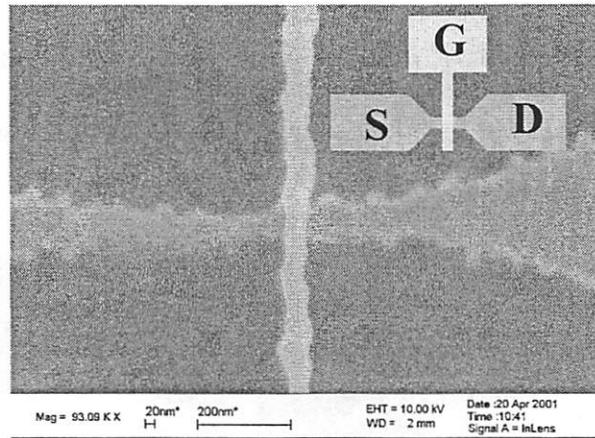
Figure 6.32 SEM top view of the gate ( $L_g=20nm$ ) and a single-fin ( $W_{fin}=40nm$ ).
