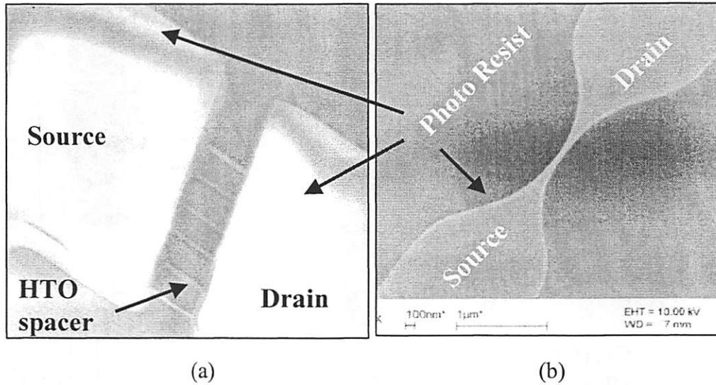
Figure 6.28 Tilted SEM photographs of multi-fins and single fins. (a) The narrowest multi-fins are defined by HTO spacers while S/D pads are defined by resist and (b) wide and variable single-fins can be defined by the same resist in (a).
