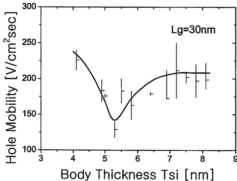
Figure 5. 10 Hole mobility is enhanced when the body thickness is thinner than 5nm.
