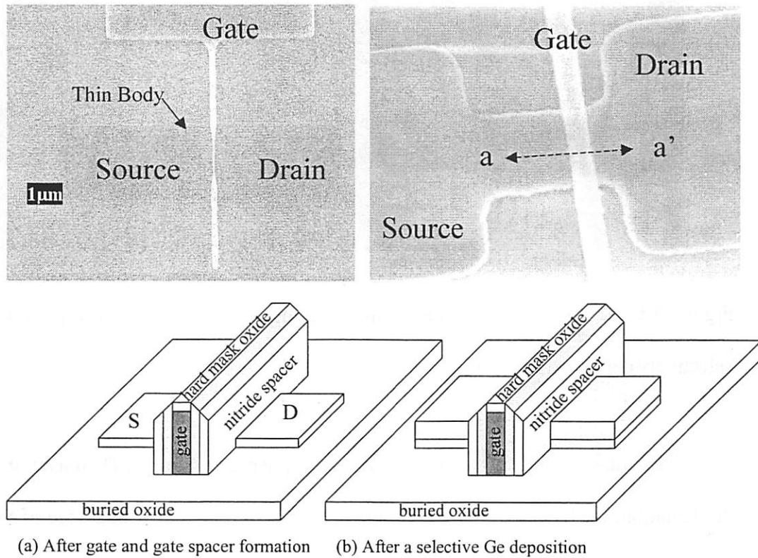
Figure 3.4 SEM photographs and schematic diagrams for raised S/D profile before and after Ge deposition. SEM pictures are taken at the different transistors between before Ge deposition and after Ge deposition.
