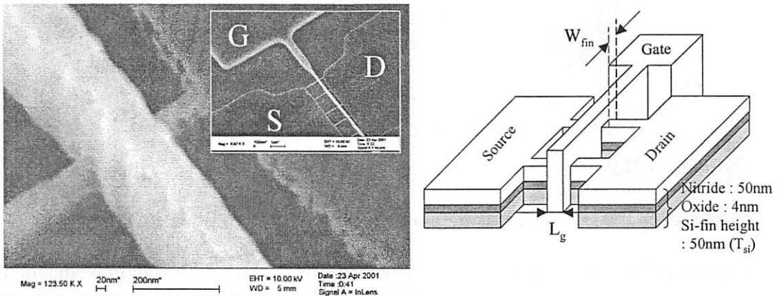
Figure 6.33 SEM tilted view of the gate ( $L_g=60nm$ ) in a multi-fin ( $W_{fin}=40nm$ ) structure. The gate is completely planarized by CMP.
