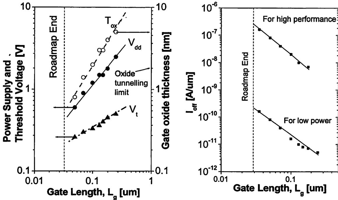
Figure 1.1 Scaling trends of power supply voltage, threshold voltage, and gate oxide thickness versus CMOS gate length [1.5].
