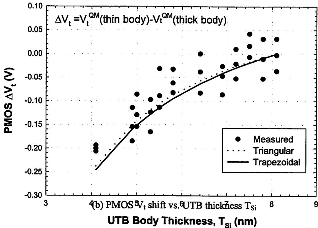
Figures 5.6 The threshold voltage shift ( $\Delta V_t$ ) for (a) NMOS and (b) PMOS as a function of body thickness ( $T_{Si}$ ) for measured data (solid circle), the analytical model based on a trapezoidal potential well (solid line), and the model based on triangular potential approximation (dashed line), respectively.
