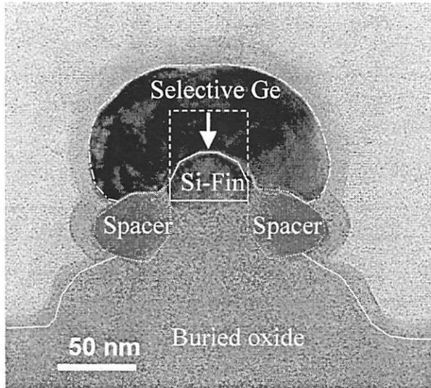
(a) TEM photograph of selectively deposited raised Ge on a fin (a-a' direction in Fig. 3.7)
