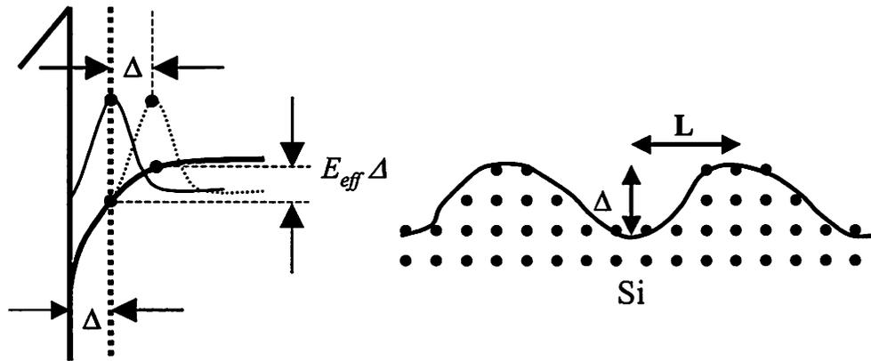
(a) Energy band diagram at rough Si-SiO<sub>2</sub> interface (b) Cross-section of rough surface
