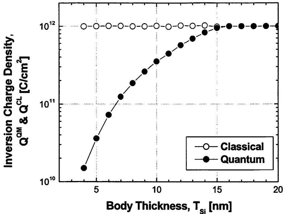
Figure 5.5 Inversion charge density for NMOSFET as a function of body thickness ( $T_{Si}$ ) with and without considering quantum confinement. For  $T_{Si} < 15$  nm, additional band bending is required for a UTB MOSFET to obtain the same amount of inversion charge density as in a bulk MOSFET.
