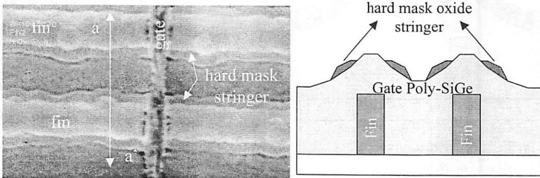
(a) SEM of photograph of stringers of gate hard mask oxide
