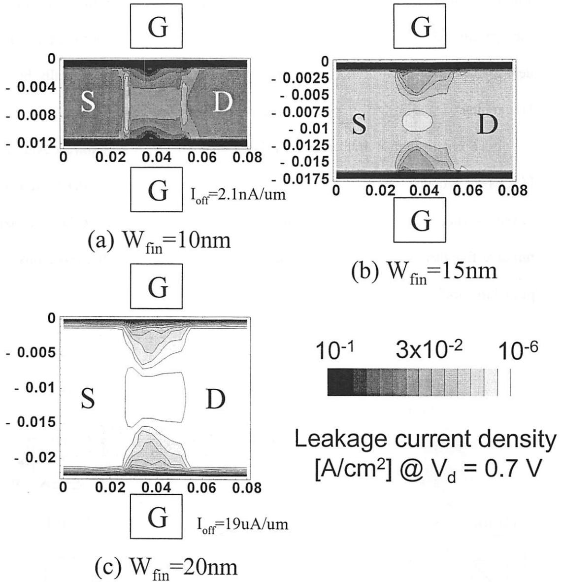
Figure 6.6 Narrowing the fin width eliminates paths far from the gate, thus improving short-channel effects and allowing for reduced gate lengths. ( $V_g=0\text{V}$ ,  $L_g=25\text{nm}$ ,  $T_{\text{ox}}=1.5\text{nm}$ ,  $N_{\text{body}}=1.0 \times 10^{15}\text{cm}^{-3}$ ) [2].
