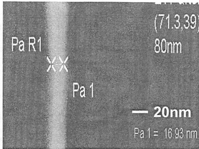
Figure 2.6 Tilted SEM photograph of 17nm SNR-2000 e-beam resist after ashing. Its initial line width is 80nm.
