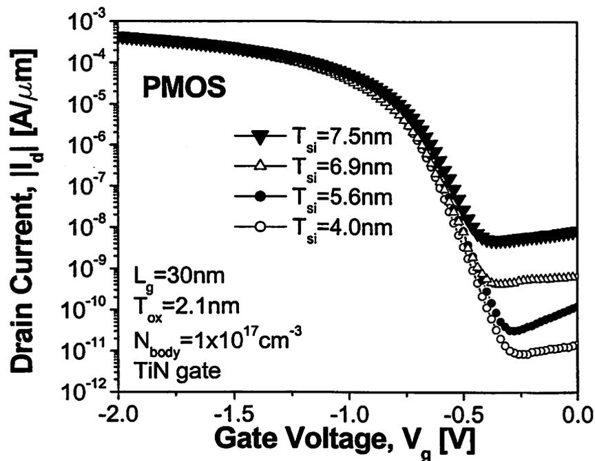
Figure 4.16 Measured off-state leakage current decreased as the body thickness reduced in UTBFETs. Threshold voltage shift is also found [4.54].
