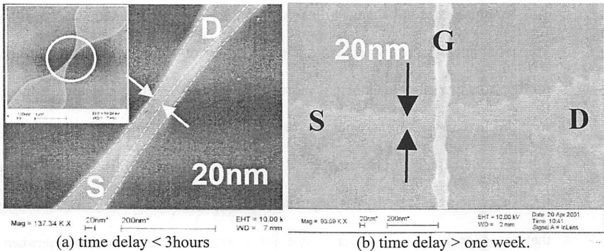
Figure 2.5 Tilted SEM photographs showing 20nm width resist after ashing (a) and 20nm width gate and Si fin profile after gate etch (b). A long time delay between resist development and ashing produces large line-edge roughness.
