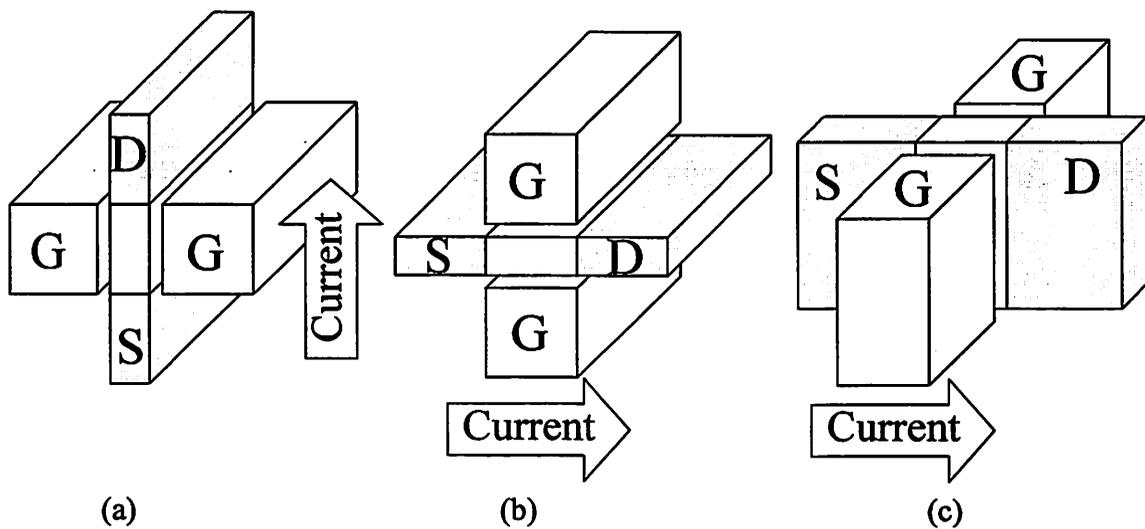
Figure 6.3 Three different double-gate structures. (a) vertical double-gate (b) horizontal double-gate (c) lateral double-gate.
