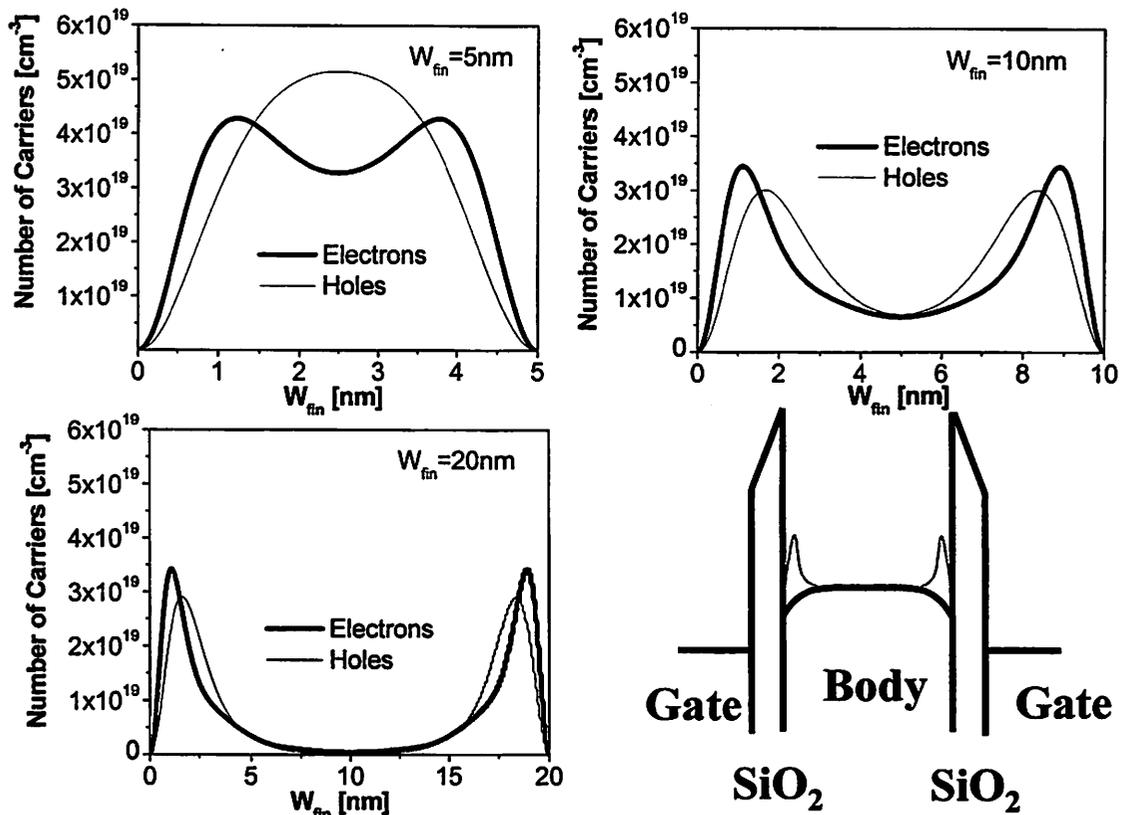
Figure 6.25. Inversion charge centroid versus fin width and energy band diagram of double-gate FinFETs. Data is obtained using Schred [6.49] ( $T_{ox}=1nm$ ,  $N_{body}=2.0 \times 10^{18} cm^{-3}$ , and  $V_g=0.8V$ ).
