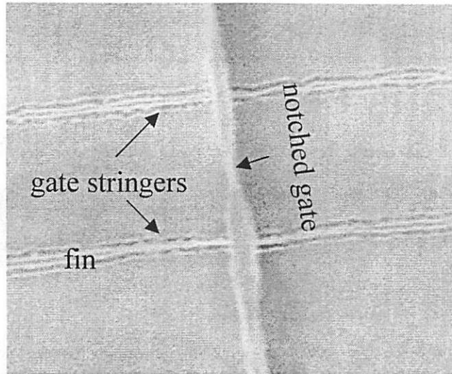
Figure 3.16 SEM photograph of a notched gate and gate hard mask oxide stringers.
