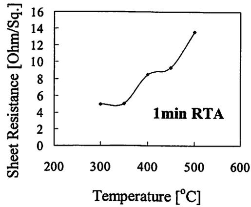
Figure 3.12 The sheet resistance of nickel-germanide increases as RTA temperature increases.
