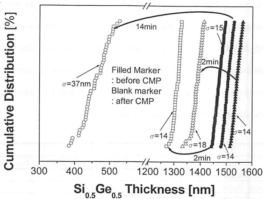
Figure 3.17 Poly-Si<sub>0.5</sub>Ge<sub>0.5</sub> thicknesses before and after CMP. The standard deviation of film uniformity increases as polishing time increases.
