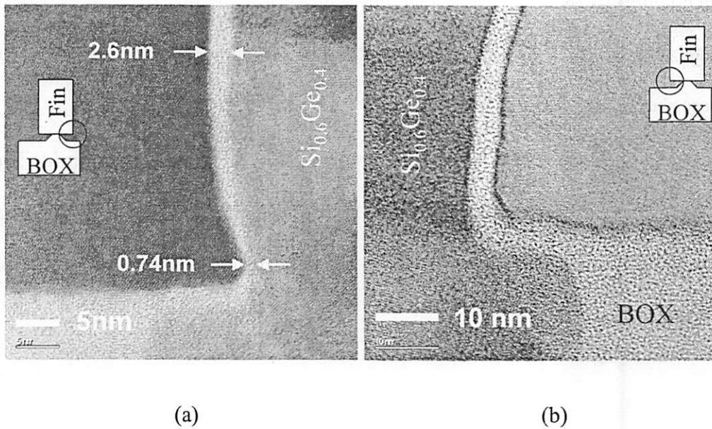
Figure 6.31 Cross-sectional TEM photographs of the gate oxide. At the sharp corner in (a), the gate oxide thickness is thinner because the growth rate is decreased by high stress.
