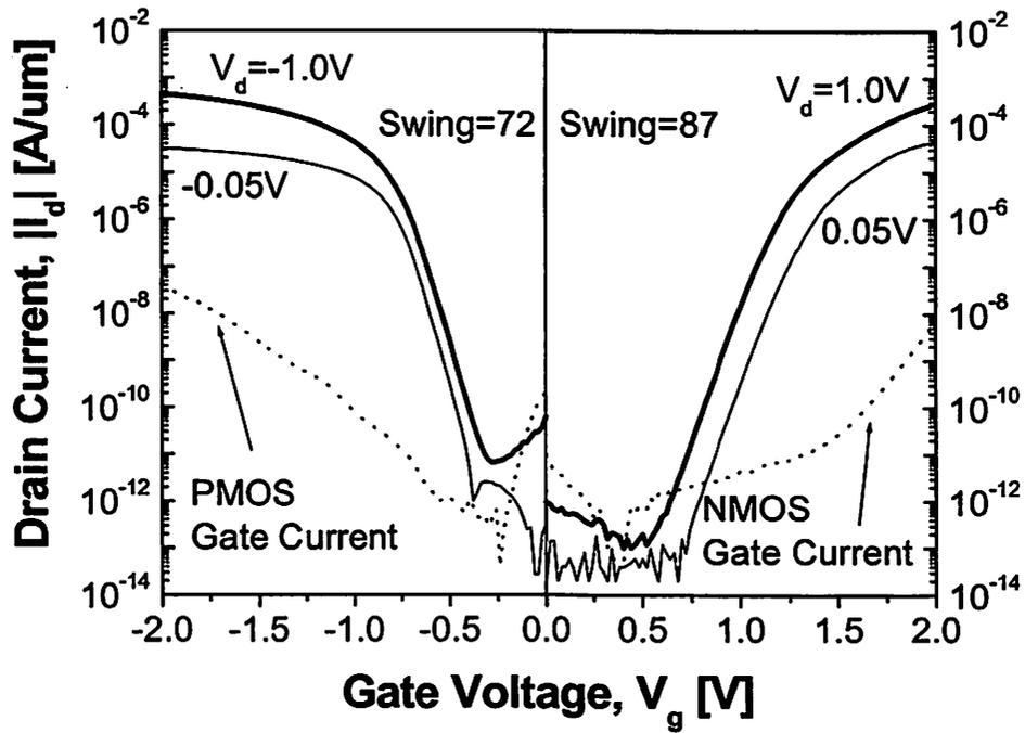
Figure 4.18 Measured  $I_d$ - $V_g$  characteristics for a separate NMOS and PMOS.
