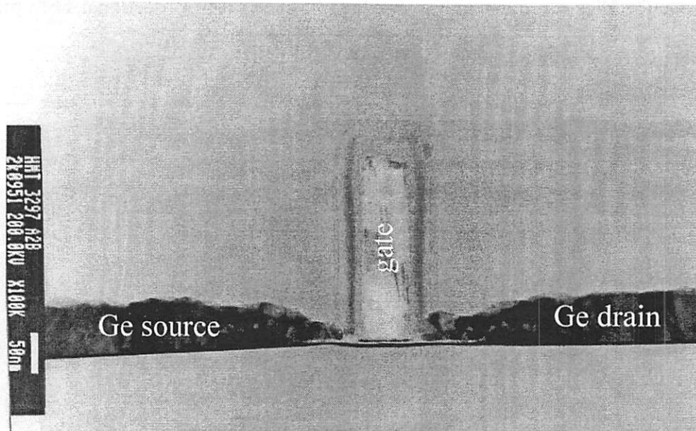
Figure 3.5 A cross-sectional TEM image along a-a' direction in Fig. 3.4 shows a selectively deposited raised Ge S/D.
