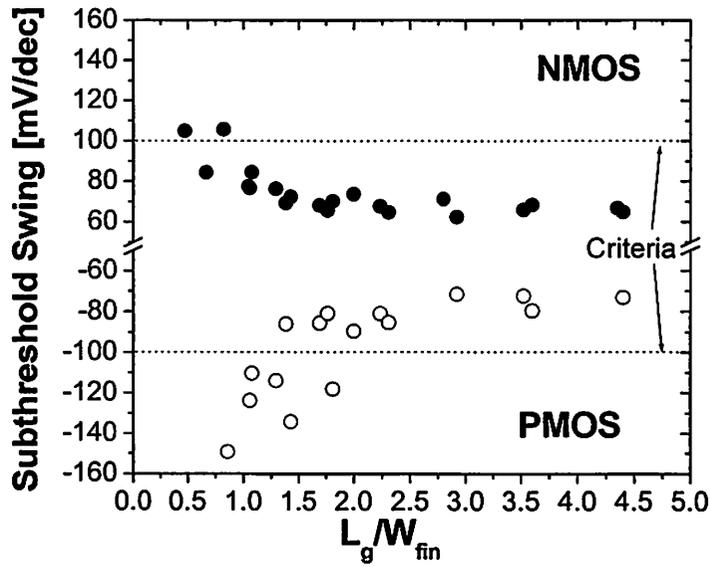
Figure 6. 21 Subthreshold swing versus  $L_g/W_{fin}$  for  $T_{ox}=2.1nm$ . When  $L_g/W_{fin}$  is larger than 1.5, both the NMOS and PMOS satisfy the criteria of subthreshold swing  $\leq \pm 100mV/dec$ .
