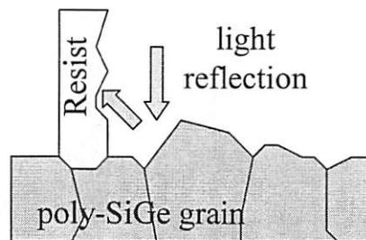
(b) Schematic of a resist notched by a rough grain structure of poly-SiGe
