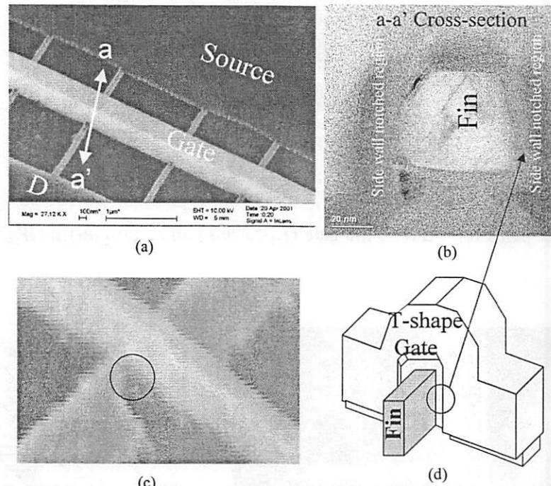
Figure 6.34 Notched gate profile at the vertical sidewall fin. (a) Tilted SEM image, (b) cross-sectional TEM image along a-a' direction in (a), (c) tilted SEM image of notched region (circle), and (d) drawing of the notched gate (circle). The light gray area in (b) is a notched region at the vertical sidewall.
