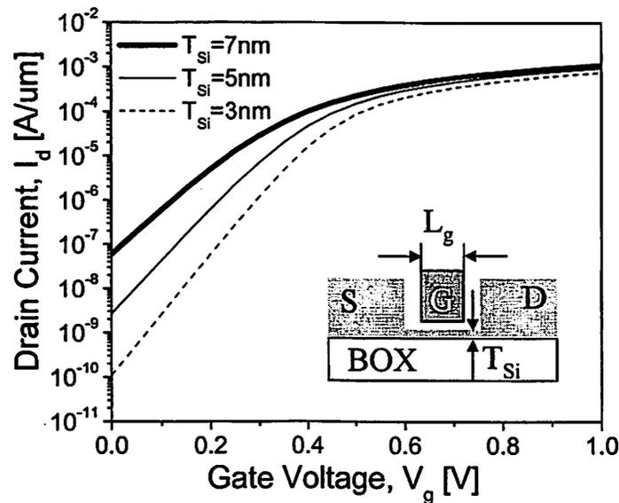
Figure 4.3 Impact of body thickness on the  $I_d$ - $V_g$  characteristics of UTB device. ( $T_{\text{ox}}=1.5 \text{nm}$ ,  $N_{\text{body}}=1 \times 10^{15} \text{cm}^{-3}$ ,  $V_d=1 \text{V}$ ).
