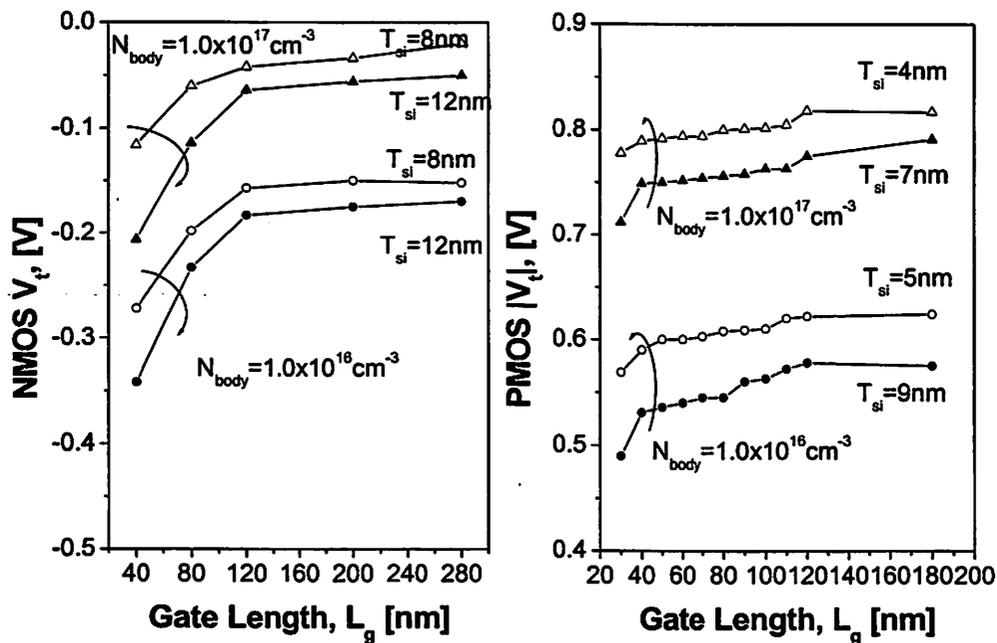
Figure 4.22 Threshold voltage roll-off characteristics of NMOS with N+ Si gate and PMOS with TiN gate.
