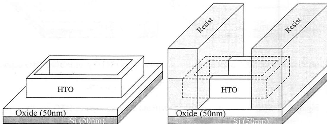
(a) A spacer HTO after removal of SiGe (b) A spacer HTO for Si fin and resists for S/D pads after S/D pad mask
