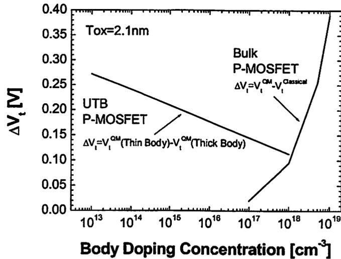
(a) Threshold voltage shift by quantum effect in PMOS UTB and bulk device
