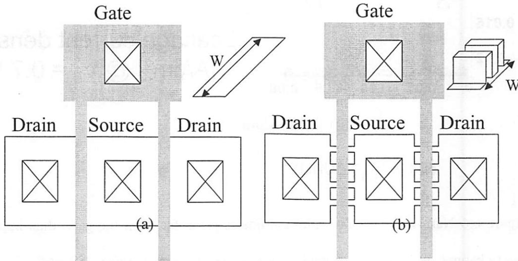
Figure 6.7. Typical layout of (a) conventional MOSFET and (b) FinFET
