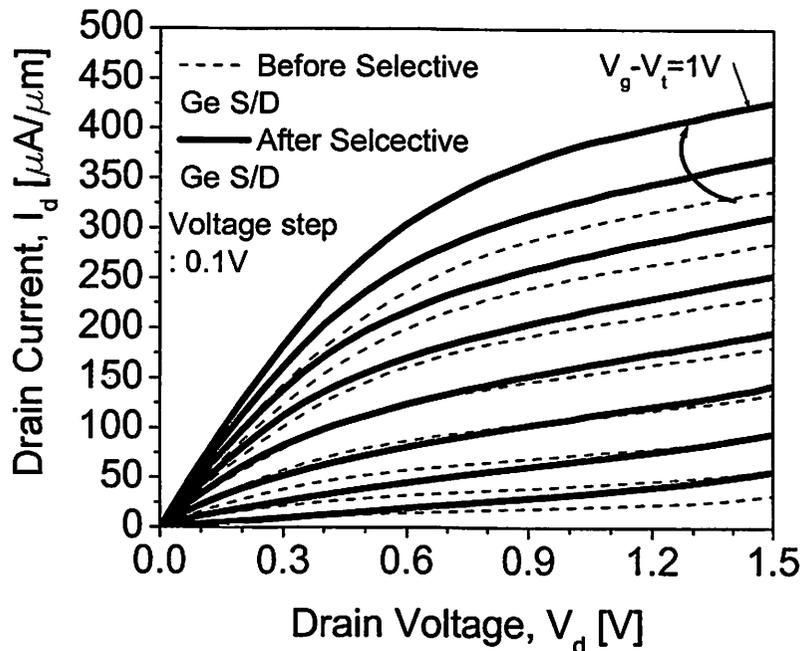
Figure 6.23 Drain current comparison before and after selective Ge deposition. The drain current is increased by 28% after Ge deposition. Data is measured on the same transistor ( $L_g=90\text{nm}/W_{fin}=70\text{nm}$ ).
