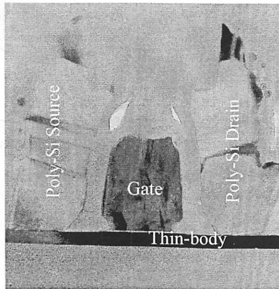
Figure 3.3 Cross-sectional TEM (a-a' direction in Fig. 3.2) photograph of the etched-back poly-Si raised S/D. A spacer oxide tail is seen at the corner of the gate and the thin body.
