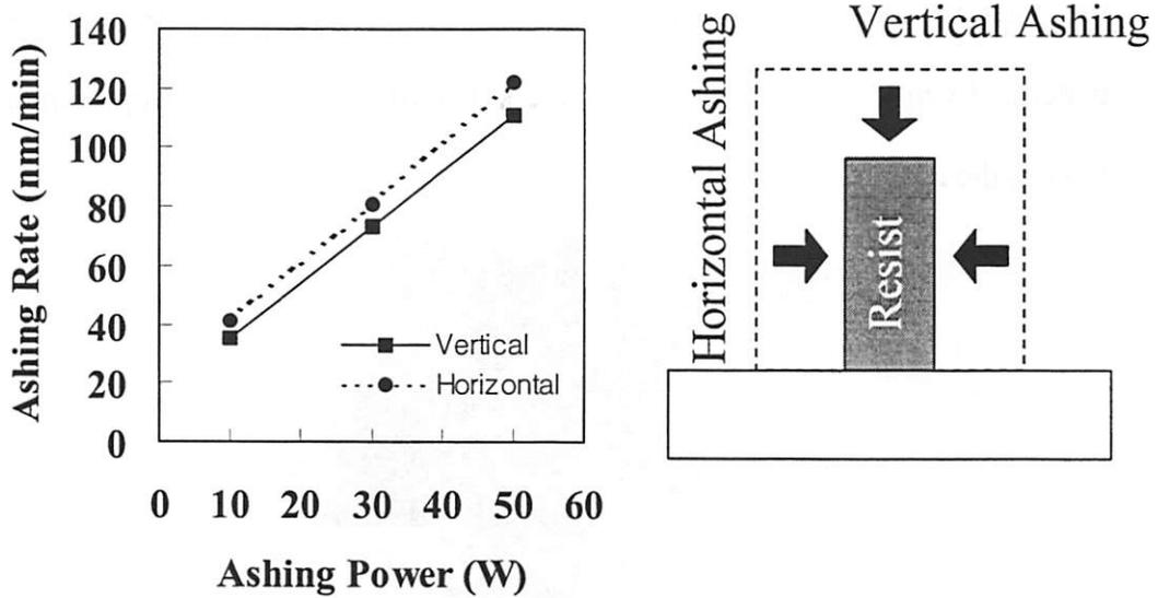
Fig. 2.3 Vertical ashing rate and horizontal ashing rate are linear functions of the microwave power and almost the same.
