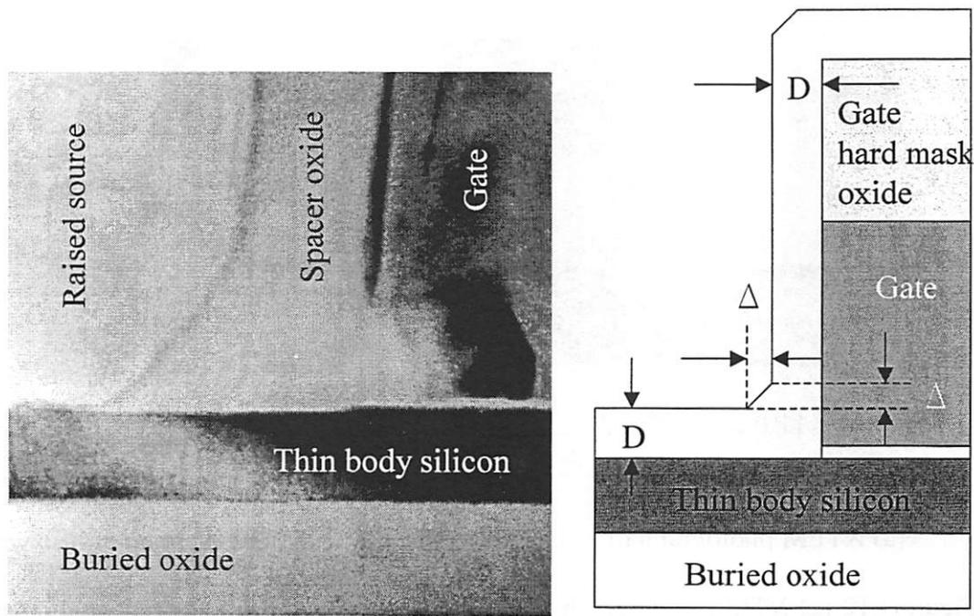
(a) XTEM photograph of tailed spacer (b) Schematic diagram of tailed spacer
