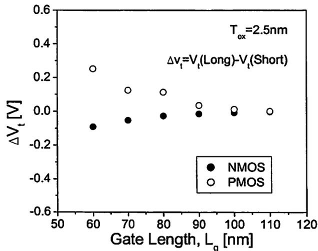
Figure 6.38 Threshold voltage roll-off characteristics. Each data point is the average of five devices ( $W_{fin}=40nm$ ,  $n^+ Si_{0.6}Ge_{0.4}$  gate,  $T_{ox}=2.5nm$ , and  $N_{body}=2.0 \times 10^{17} cm^{-3}$  (n-type)).
