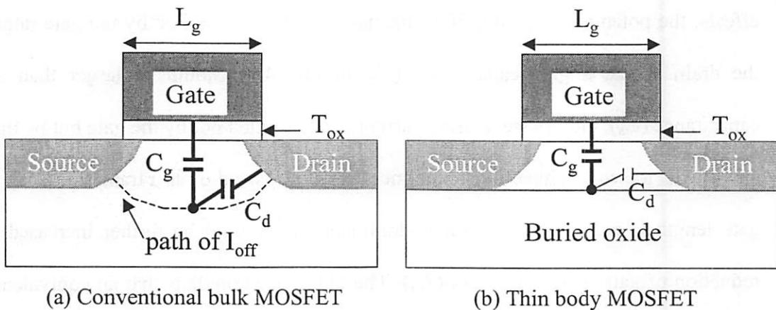
Figure 4.1 Schematic diagrams of conventional bulk silicon MOSFET (a) and thin body silicon-on-insulator MOSFET (b)
