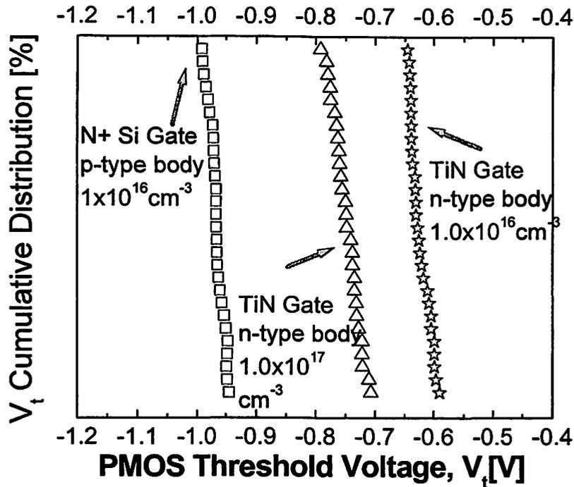
Figure 4.20 PMOS threshold voltage for N+ Si gate and TiN gate with different body doping,  $1 \times 10^{16} \text{ cm}^{-3}$ ,  $1 \times 10^{17} \text{ cm}^{-3}$ .
