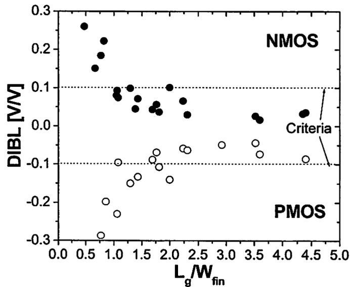
Figure 6. 22 DIBL versus  $L_g/W_{fin}$  for  $T_{ox}=2.1nm$ . When  $L_g/W_{fin}$  is larger than 1.5, both the NMOS and PMOS satisfy the criteria of the DIBL  $\leq \pm 0.1V/V$ .
