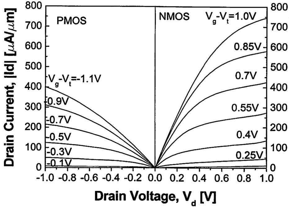
Figure 4.17 Measured  $I_d$ - $V_d$  characteristics for a separate NMOS and PMOS.
