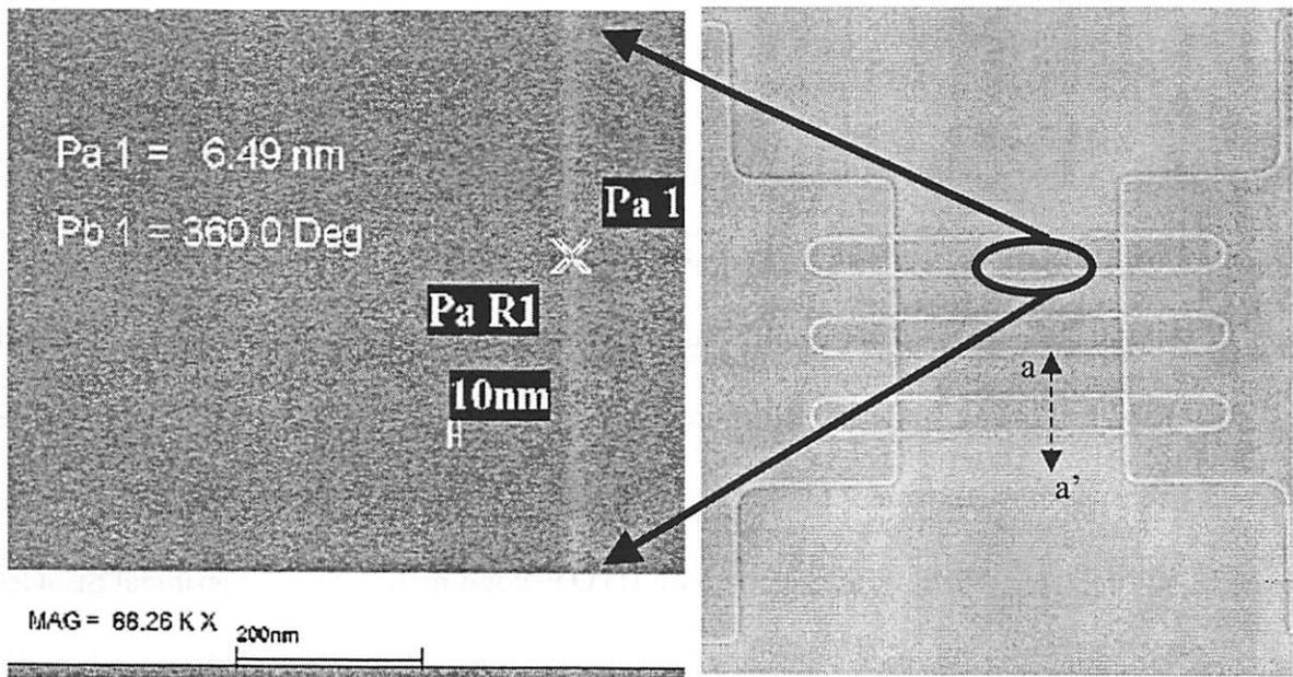
Figure 2.16 SEM photographs of 6.5nm Si fin width after etching a hard mask nitride, pad oxide, and Si.
