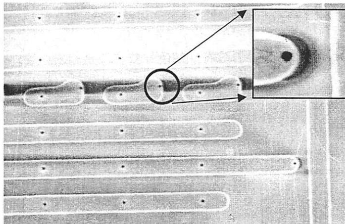
Figure 4.15 Top SEM view of Al interconnection line. The inset shows that the enlarged contact hole by HF makes Al line not to cover that contact hole completely.
