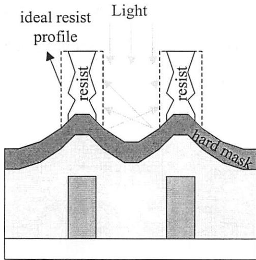
(a) A schematic diagram of cross-sectional view of notched resist
