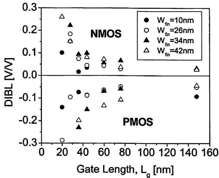
Figure 6. 20 DIBL versus gate length. A narrower fin width shows lower DIBL.
