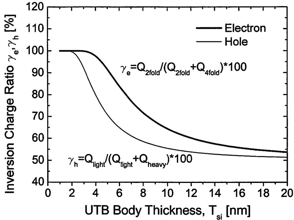
Figure 5.4. Calculated fraction of inversion charge residing at the lowest energy level as a function of body thickness for NMOSFET and PMOSFET using Eq. (5.14).
