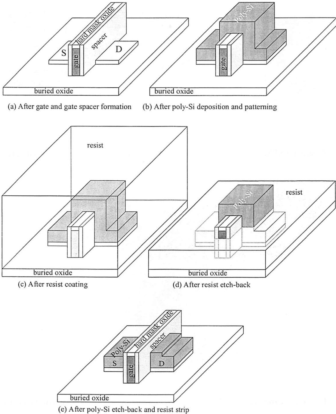
Figure 3.1 Schematic diagrams of the resist and poly-Si etch-back process.
