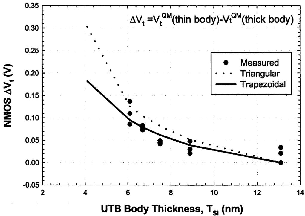
(a) NMOS  $V_t$  shift vs. UTB thickness  $T_{Si}$
