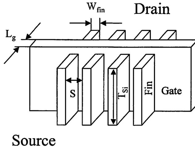
Figure 6.8 3-dimensional view of FinFET with multiple fins.
