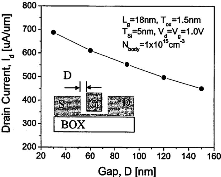
Figure 4.7 Drive current dependence of a series resistance of source and drain.
