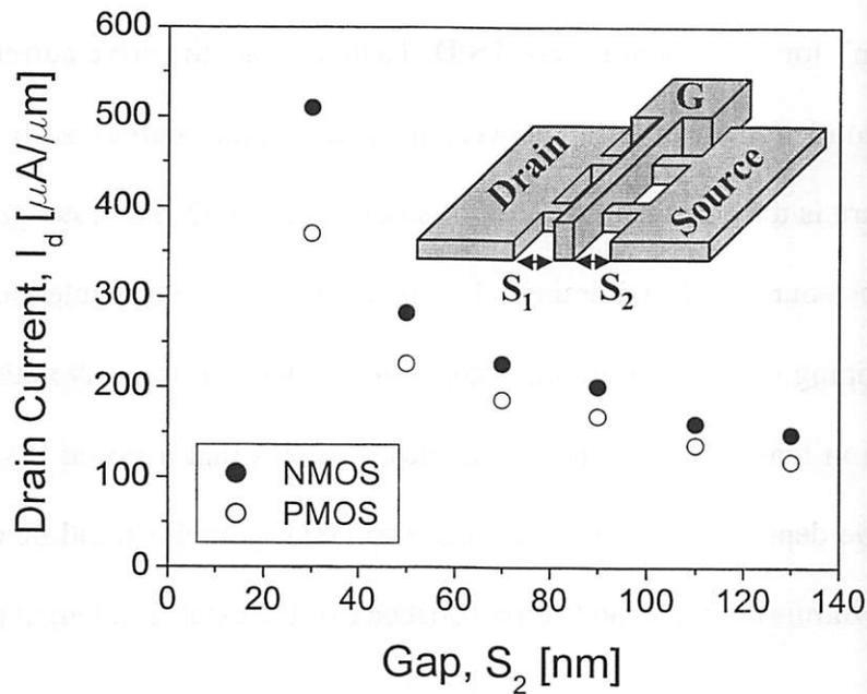
Figure 6.42 Drive current dependence on the gap ( $S_2$ ) between the gate and the source.
