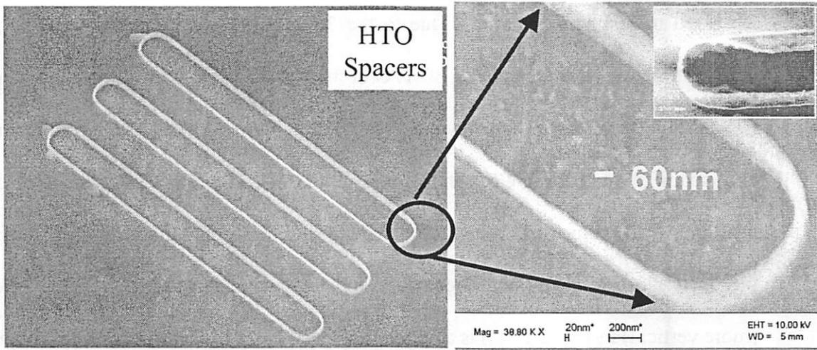
Figure 2.14 Tilted SEM photographs of HTO spacer profile after removal of sacrificial SiGe. HTO film width is 20nm in the right picture. Inset shows a collapse-downed HTO spacer after spin-dry (2000 rpm) process.
