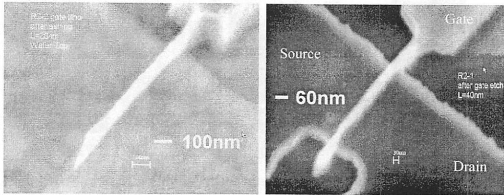
(a) A 20nm hard mask oxide after trimming
