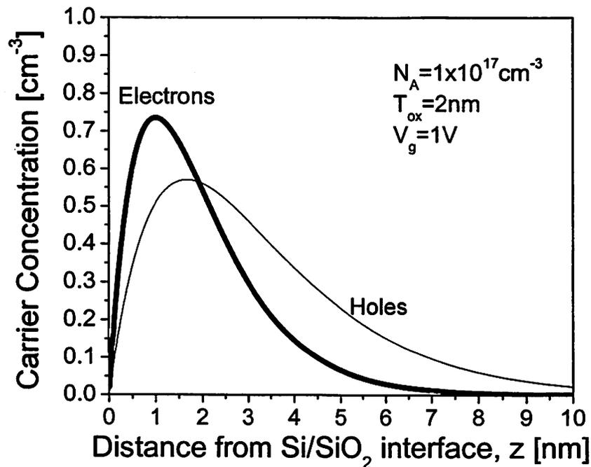
Figure 5.1 Inversion carrier concentration for electrons and holes in bulk device.
