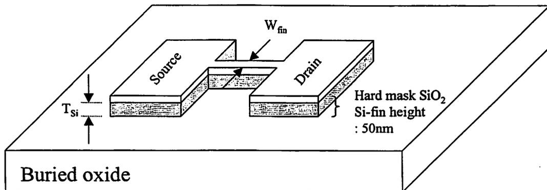
Figure 6.10 FinFET structure after silicon fin etch.
