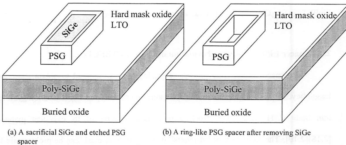
Figure 2.18 Schematic diagrams of a sacrificial SiGe and etched PSG spacer.
