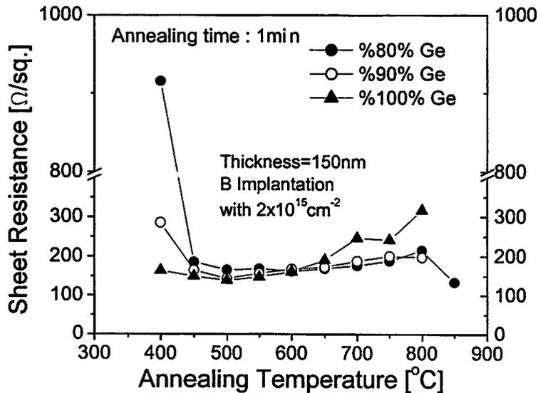
Figure 3.9 Sheet resistance of 150nm-thick boron doped poly- $\text{Si}_{1-x}\text{Ge}_x$  for different annealing temperatures [3.27].
