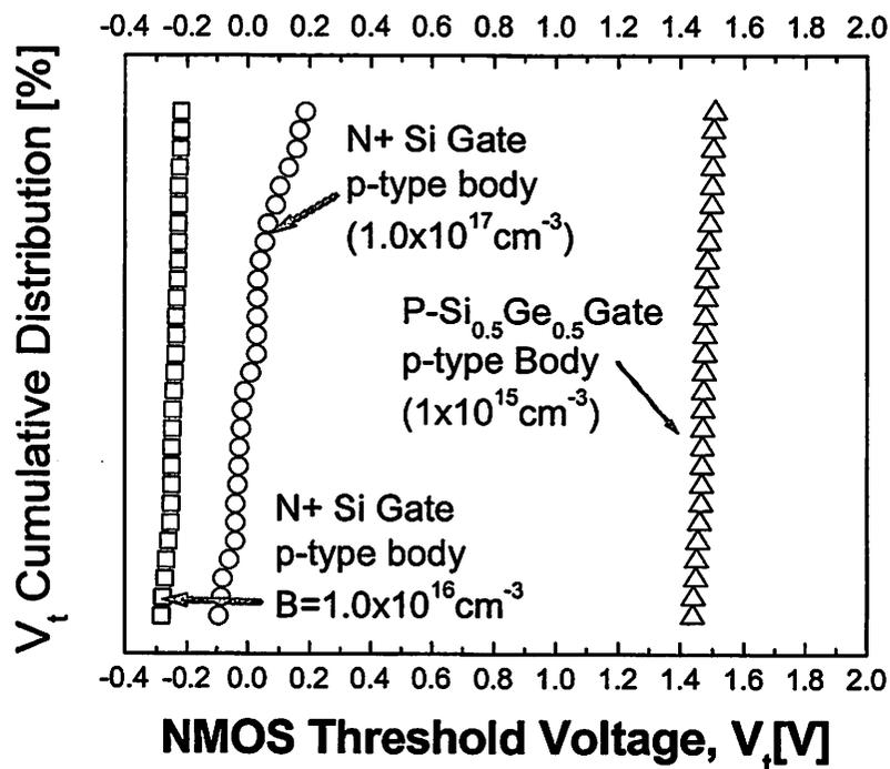
Figure 4.19 NMOS threshold voltage for N+ Si gate and P+ Si<sub>0.5</sub>Ge<sub>0.5</sub> gate with different body doping,  $1 \times 10^{16} \text{ cm}^{-3}$ ,  $1 \times 10^{17} \text{ cm}^{-3}$ .
