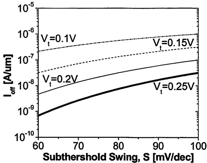
Figure 1.2 Off-state leakage current versus subthreshold swing for different threshold voltages.
