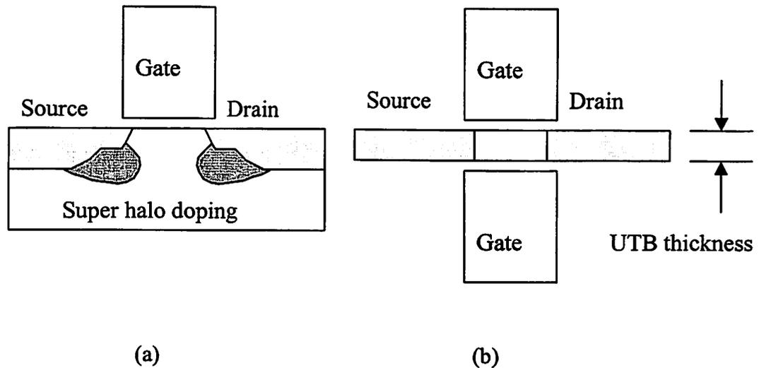
Figure 6.1 Schematic diagrams of (a) a conventional bulk MOSFET structure and (b) a double-gate MOSFET with ultra-thin body.
