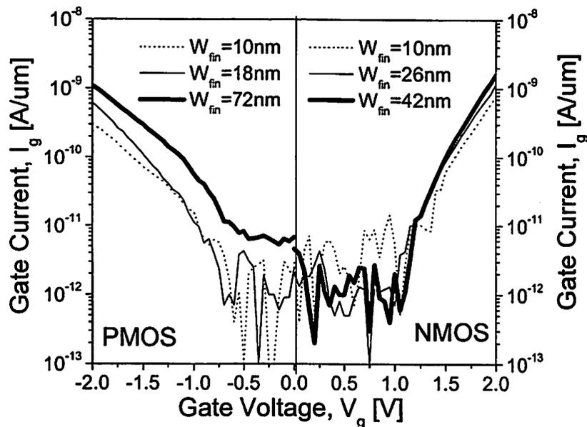
Figure 6.27. Measured gate current versus gate voltage for different fin widths. Narrower fin (thinner body) shows lower gate leakage current. ( $T_{ox}=2.1\text{nm}$ ,  $N_{body}=2.0 \times 10^{18}\text{cm}^{-3}$ ,  $P+$   $Si_{0.6}Ge_{0.4}$  gate)
