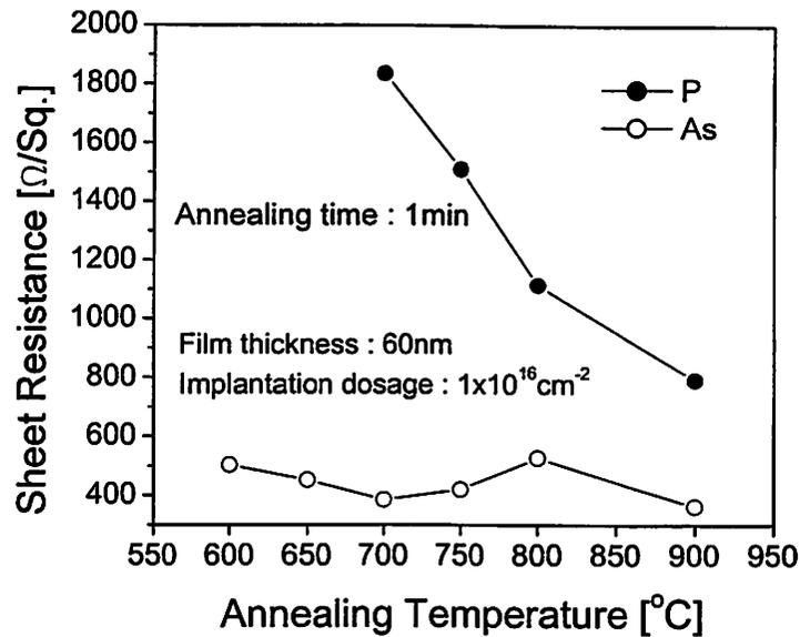
Figure 3.10 Sheet resistance of 60nm-thick phosphorus- and arsenic-doped poly-Ge for different annealing temperatures [3.28].
