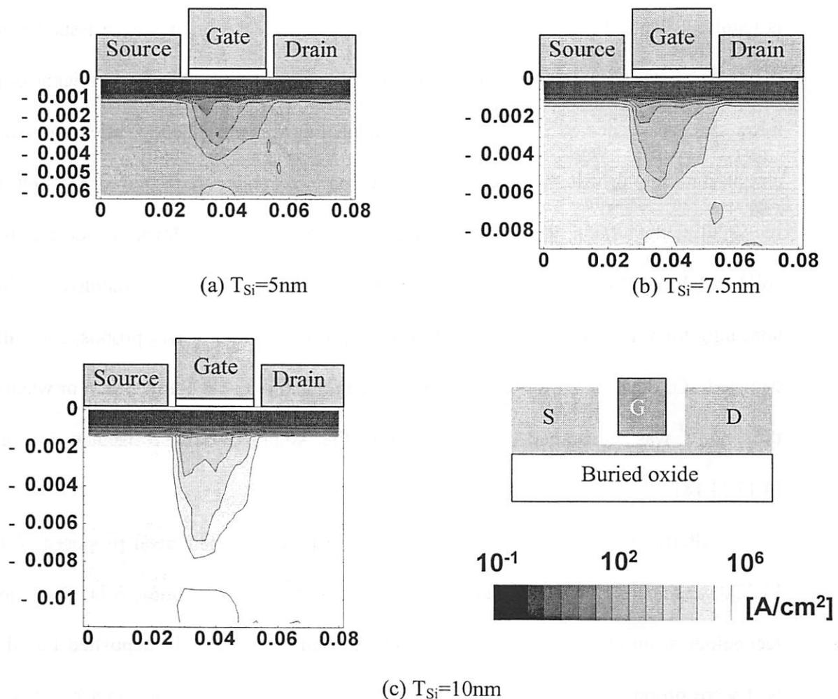
Figure 4.2 NMOS Leakage current density for a different body thickness ( $T_{Si} = 5nm$ ,  $7.5nm$ ,  $10nm$ ) at  $V_g = 0V$ ,  $V_d = 0.7V$ .  $L_g$  is  $25nm$ ,  $T_{ox}$  is  $1.5nm$ , and  $N_{body}$  is  $1 \times 10^{15} cm^{-3}$ .
