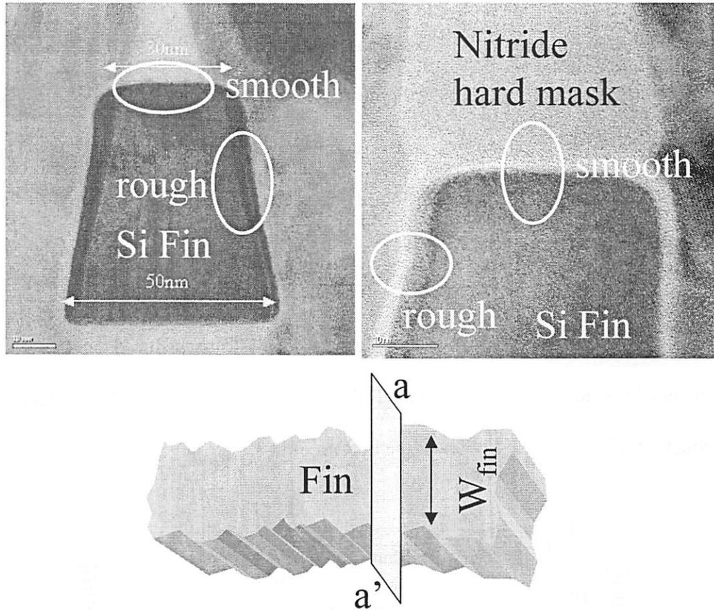
Figure 6. 26 Cross-sectional TEM photographs of a fin along the a-a' direction. The top surface is smooth because the film is thermally oxidized and the sidewall surface is rough because it is formed by lithography and plasma etch.
