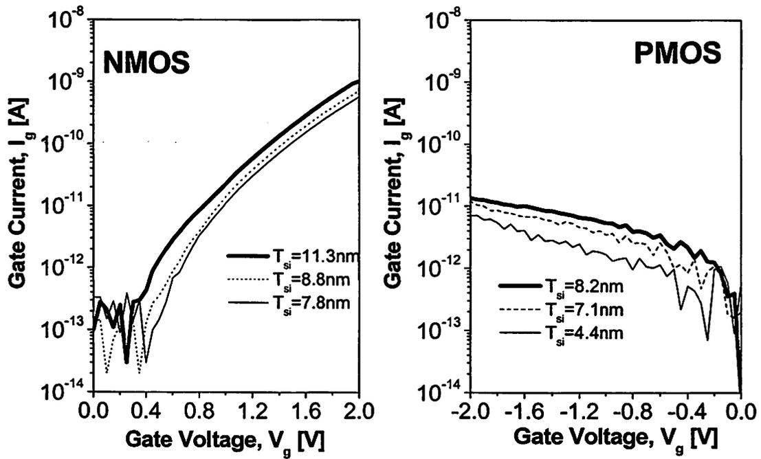
Figure 4.27 Measure gate current ( $T_{ox}=2.1nm$ ) for different body thicknesses.
