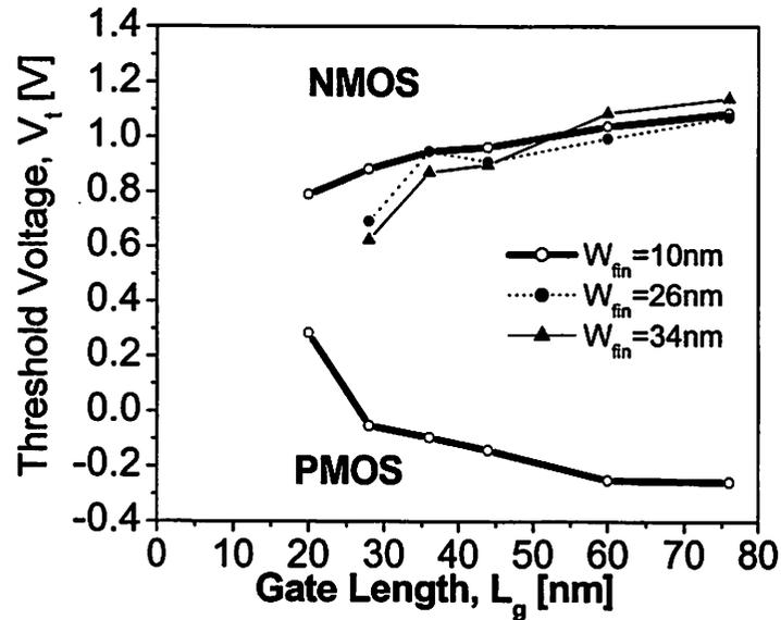
Figure 6. 18 Threshold voltage roll-off characteristics. A narrower fin width shows better roll-off behavior.
