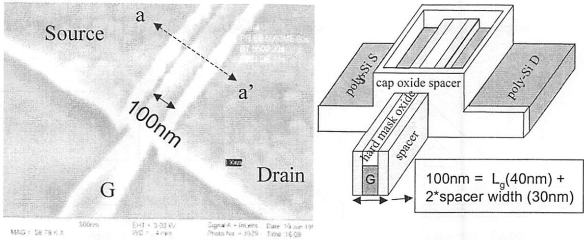
Figure 3.2 SEM photograph and schematic diagram of the etched-back raised poly-Si S/D.
