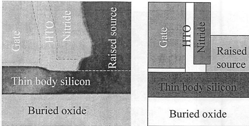
(a) XTEM photograph of bi-layer spacers (b) Schematic diagram of bi-layer spacers.
