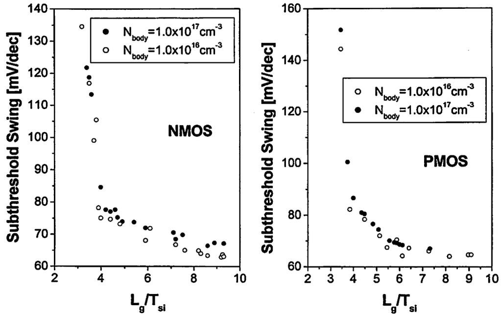
Figure 4.23 Subthreshold swing versus  $L_g/T_{Si}$ .
