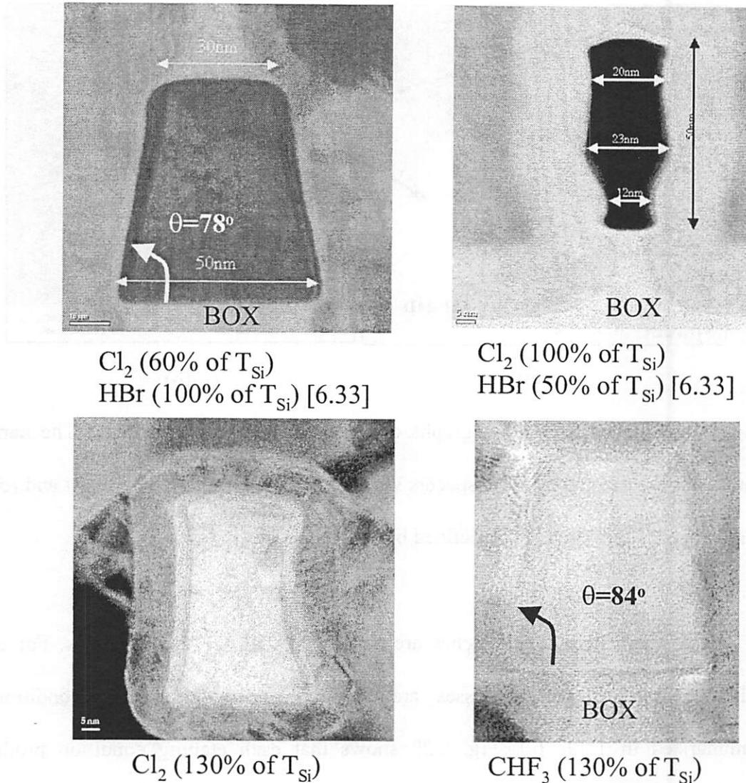
Figure 6.29 Cross-sectional TEM photographs of silicon fin.  $T_{Si}$  is the silicon film thickness, which is the same for all samples. Detailed etch recipes are summarized in Table 6.1
