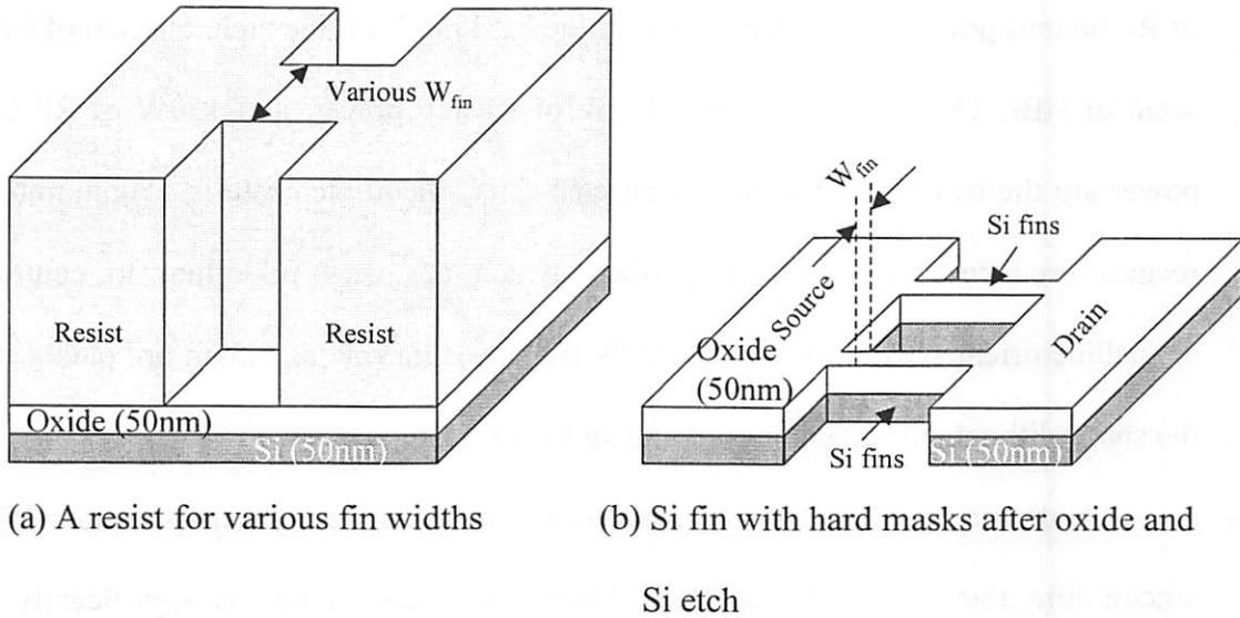
Figure 2.13 Schematic diagrams of a resist for various fin widths and Si fins formed by spacers after a hard mask oxide and Si.
