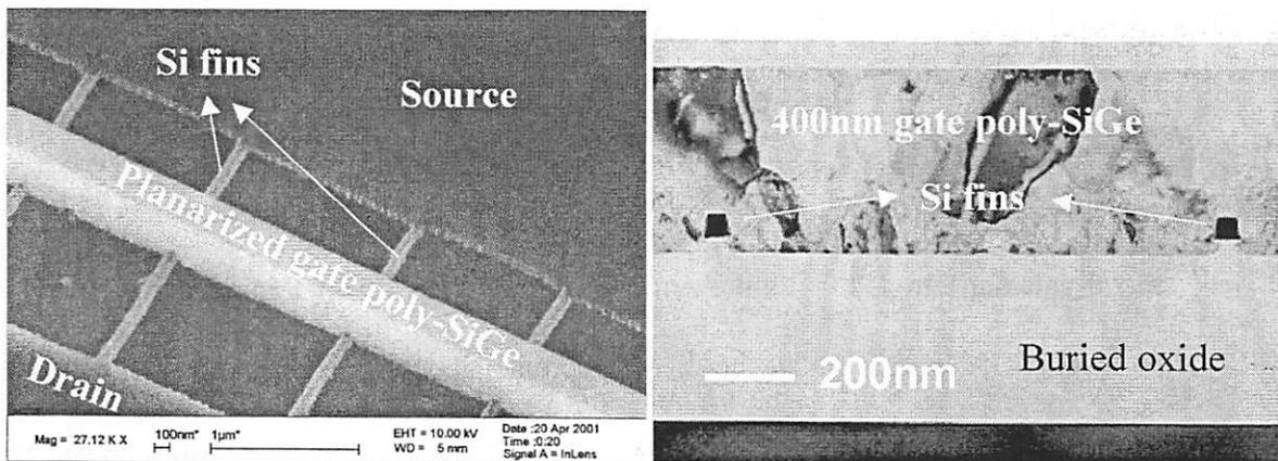
(a) Tilted SEM view of a poly-SiGe gate planarized by CMP after gate patterning
