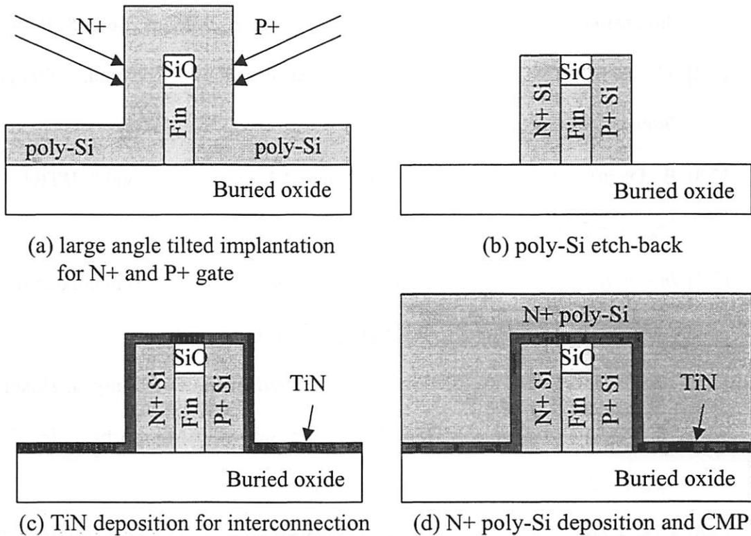
Figure 7.1 Cross-sectional diagrams showing the process flow of asymmetrical double-gate FinFETs.
