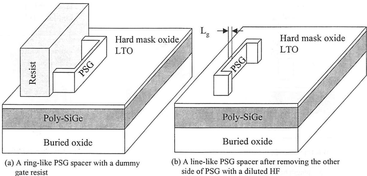
Figure 2.19 Schematic diagrams of a dummy gate resist and a line-like PSG spacer after removing PSG spacer uncovered with the resist.
