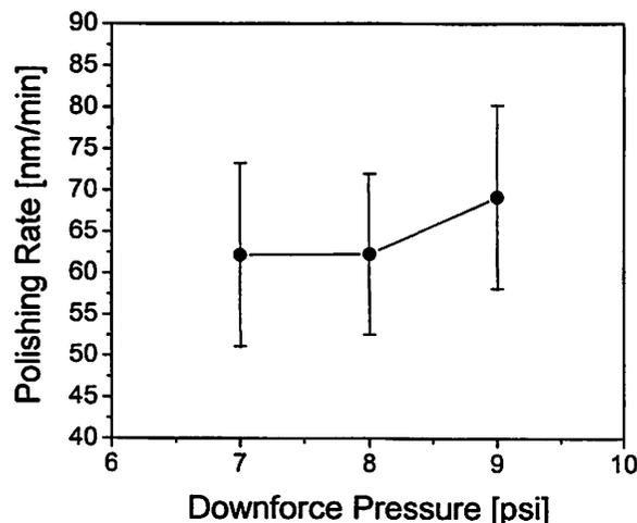
Figure 3.19 Polishing rate versus downforce. The standard deviation is independent of the downforce.
