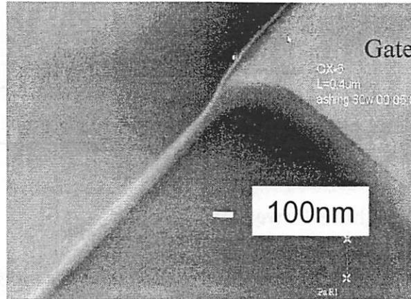
Figure 2.4 Tilted SEM picture of an i-line resist after ashing. It is reduced down to 80nm from 500nm.
