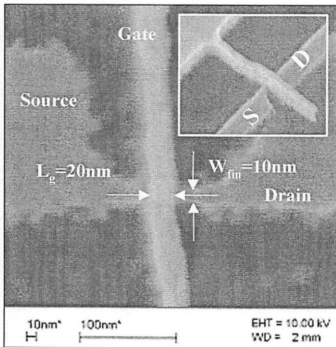
Figure 6.13 SEM top view of a FinFET with 10nm fin width and 20nm top gate length.
