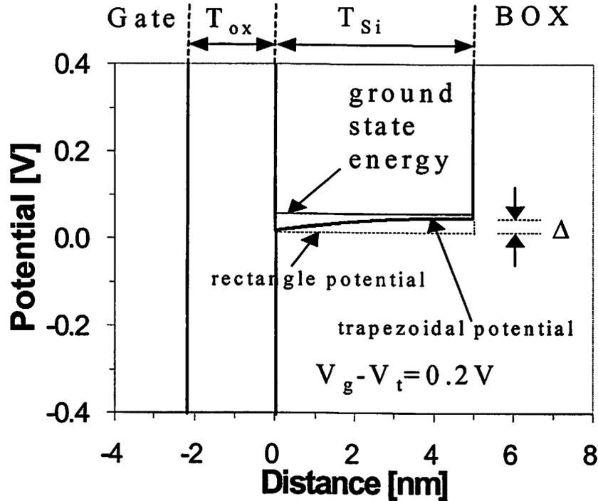
Figure 5.3 Numerical simulation results for the ground state energy for  $V_g - V_t = 0.2 V$  using the simulator Schred [5.25]. The thicknesses of the gate oxide and body is 2.1 nm and 5 nm, respectively. The doping concentration is  $10^{16} \text{ cm}^{-3}$ .
