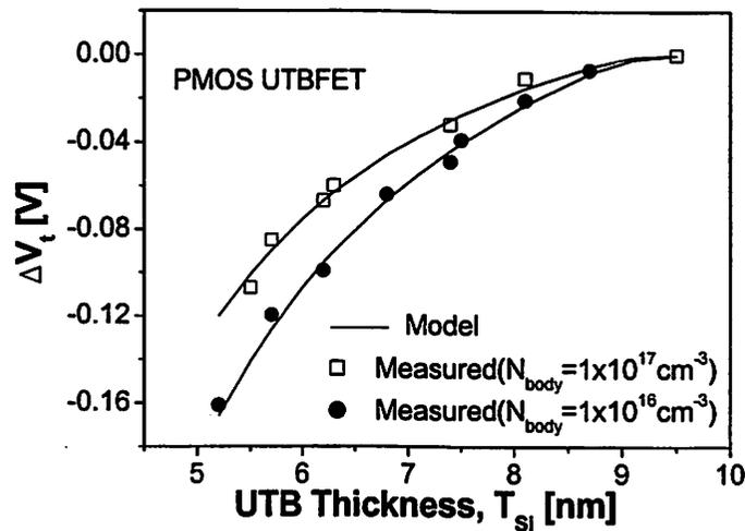
(b) Measured threshold voltage shift by quantum effect in PMOS UTB device.
