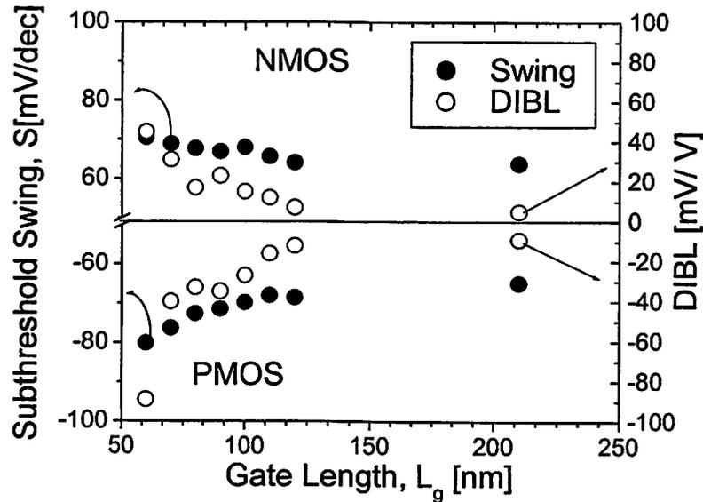
Figure 6.39 Subthreshold swing and DIBL versus the gate length. Each data point is the average of five devices ( $W_{fin}=40nm$ ,  $n+$   $Si_{0.6}Ge_{0.4}$  gate,  $T_{ox}=2.5nm$ , and  $N_{body}=2.0 \times 10^{17} cm^{-3}$  (n-type)).
