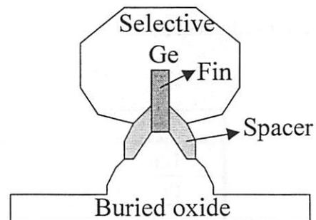
(b) Schematic diagram of selectively deposited raised Ge on a fin
