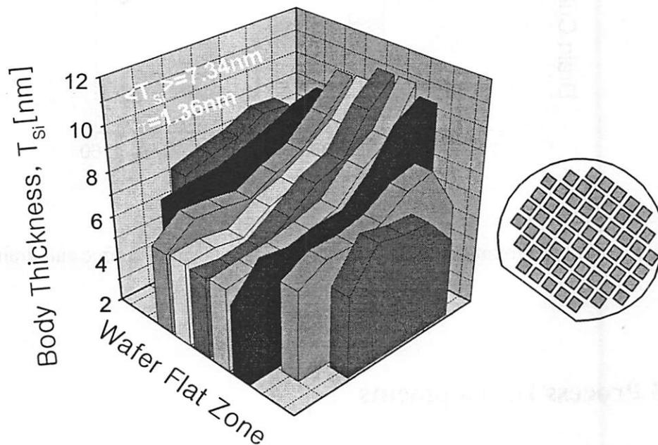
Figure 4.8 Uniformity of silicon film thickness after body thinning oxidation across 4inch wafer. One pixel denotes one die.
