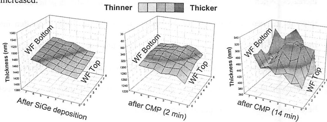
Figure 3.18 Remaining film uniformity before CMP and after CMP.
