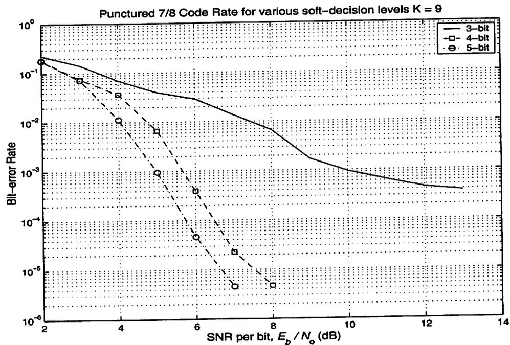
Figure 4.5 BER curve for rate 7/8,  $K=9$
