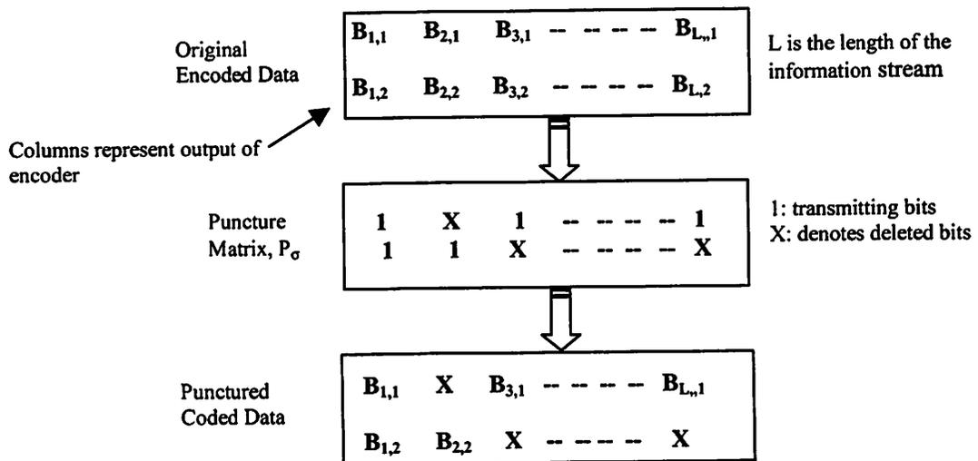
Figure 3.4 Puncture Example
