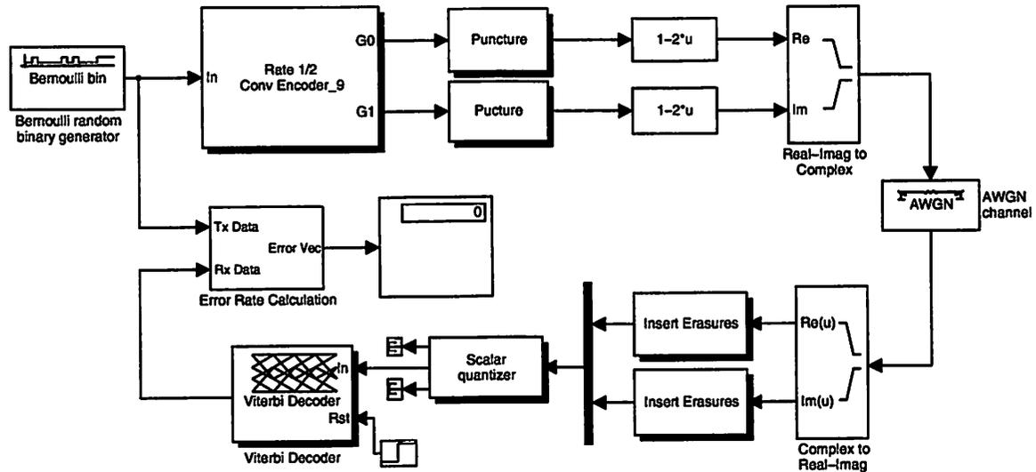
Figure 4.1 Floating Point System Level Model
