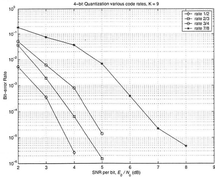
Figure 4.13 4-bit Quantization System Performance
