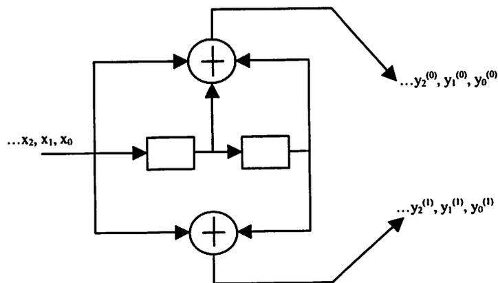
Figure 3.1 Convolutional Encoder
