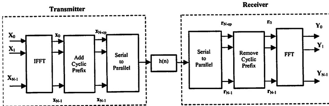
Figure 2.1 OFDM Block Diagram
