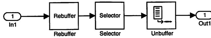
Figure 4.6 Floating Point Puncture Block
