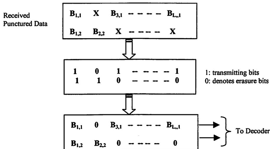
Figure 3.5 Insert Erasure Example
