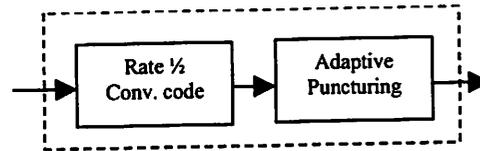
Figure 2.4 Encoding and Puncturing Blocks
