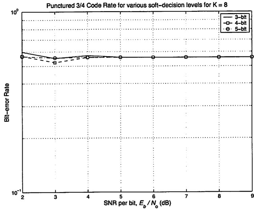
Figure 4.4 BER curve for rate 3/4, K=8
