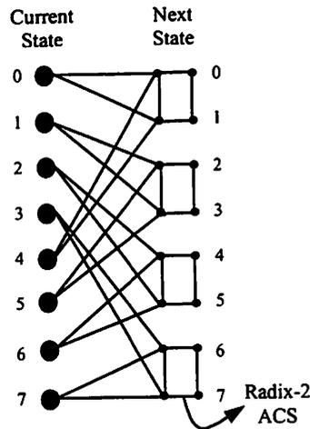
Figure 4.19 8-State Trellis Diagram
