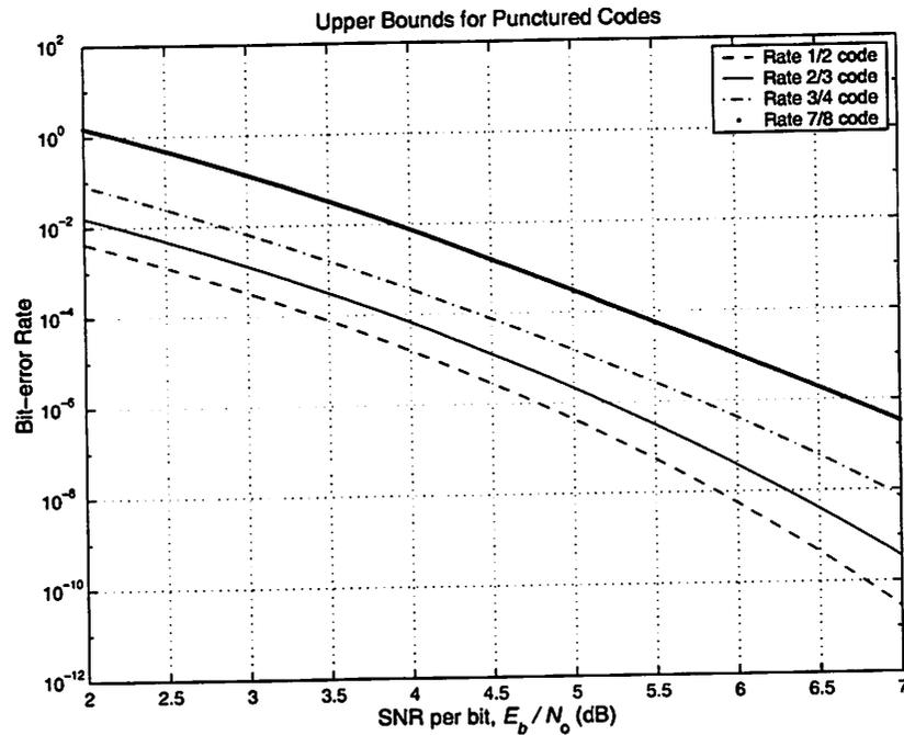
Figure 4.7 BER Upper Bound on Punctured Codes
