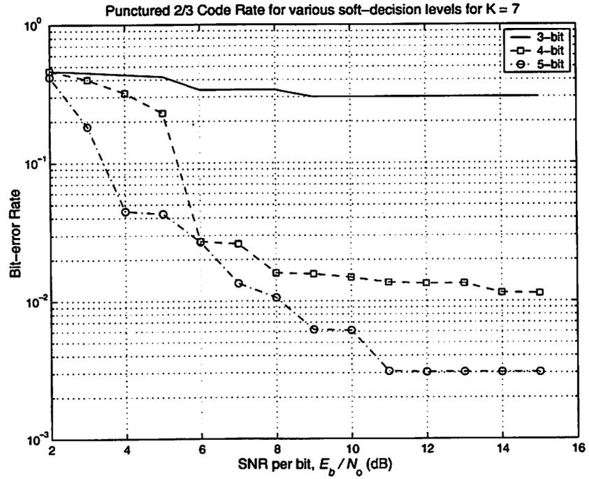
Figure 4.3 BER curve for rate 2/3, K=7
