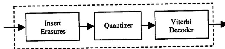
Figure 2.5 Erasure and Decoding Blocks
