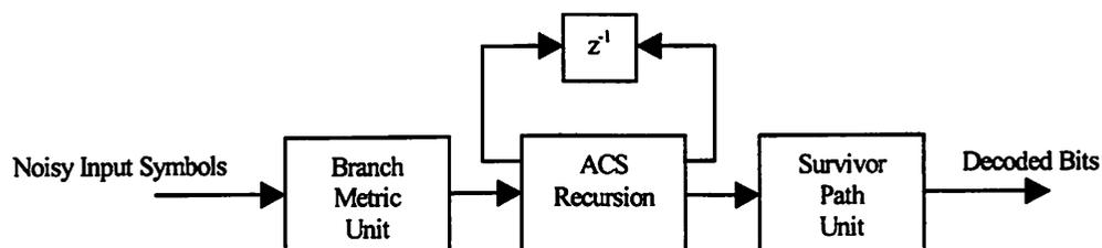
**Figure 4.18** Functional Units of Viterbi Decoder
