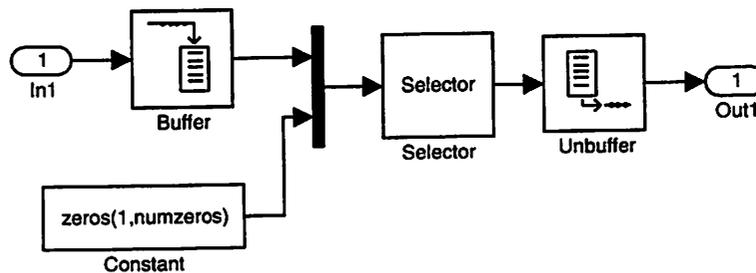
Figure 4.8 Floating Point Insert Erasure Block
