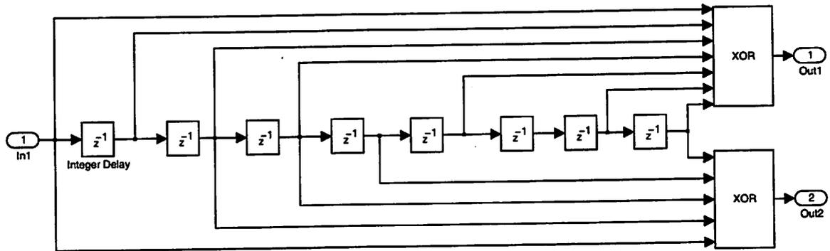
Figure 4.2 Floating Convolutional Encoder, K=9
