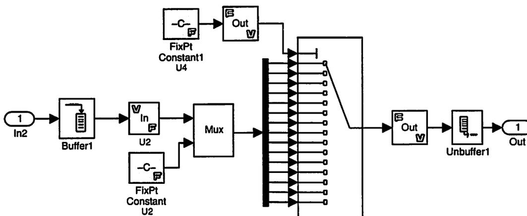
Figure 4.16 Fixed-Point Puncture Block
