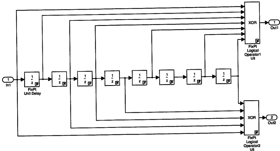
Figure 4.15 Fixed-Point Convolutional Encoder
