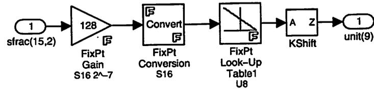
Figure 4.17 Fixed-Point Quantizer Block
