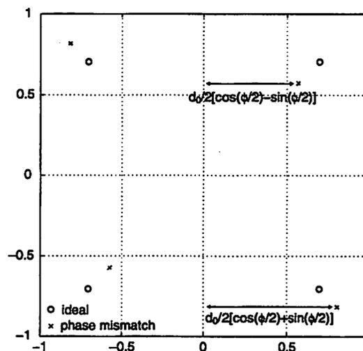
Figure 3.9: Effect of quadrature phase mismatch on a QPSK constellation.
