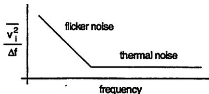
Figure 2.10: Noise power spectral density for MOS transistors.
