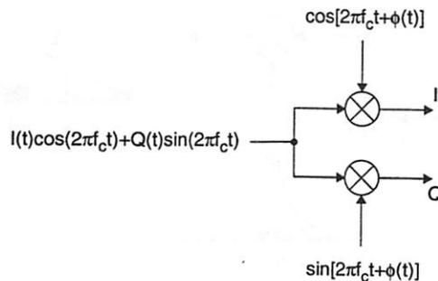
Figure 3.16: Frequency translation using I and Q LO signals with phase noise.
