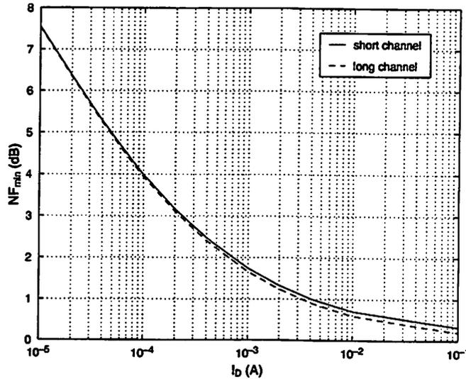
Figure 6.13:  $NF_{min}$  versus  $I_D$  based on short-channel and long-channel equations for the inductively-degenerated LNA topology. ( $\alpha=0.8$ ,  $\delta=4$ ,  $\gamma=2$ ,  $c=j0.395$ ,  $G_s=1/(50\ \Omega)$ ,  $\omega=2\pi 2\times 10^9$  rad/s,  $L=L_{eff}=0.18\ \mu\text{m}$  ( $L_{drawn}=0.25\ \mu\text{m}$ ),  $\mu_{eff}=400\ \text{cm}^2/\text{Vs}$ ,  $E_{sat}=5\times 10^4$  V/cm.)
