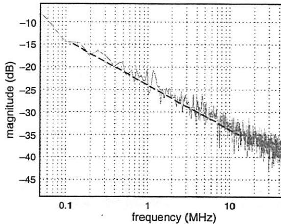
Figure 4.9: Simulated flicker noise power spectral density.
