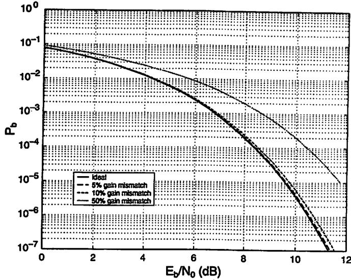
Figure 3.7: Probability of error for QPSK with gain mismatch.
