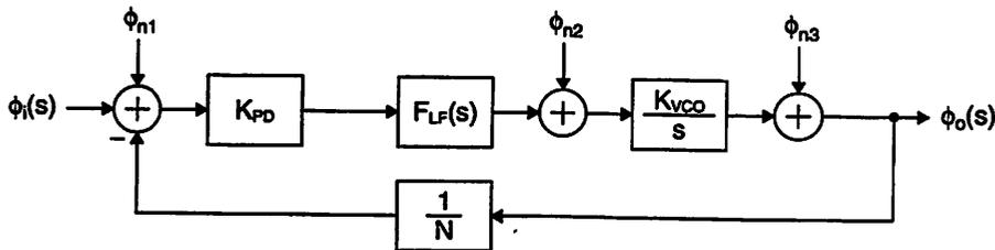
Figure 4.14: Linear model of PLL with noise sources.
