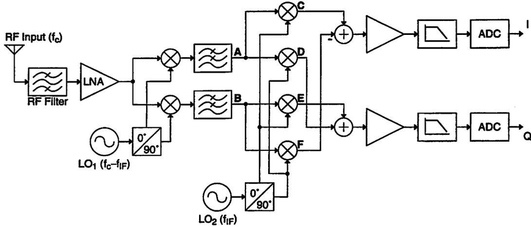
Figure 2.13: Image-reject (Weaver) architecture block diagram.
