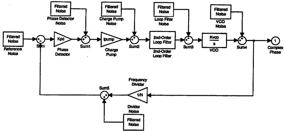
Figure 4.15: Simulink implementation of complex phase noise model.
