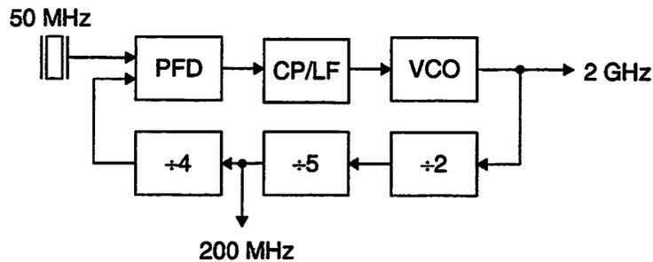
Figure 6.30: Block diagram of phase-locked loop frequency synthesizer.
