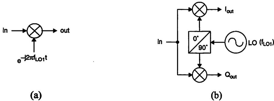
Figure 2.12: Complex mixing. (a) Concept. (b) Implementation.
