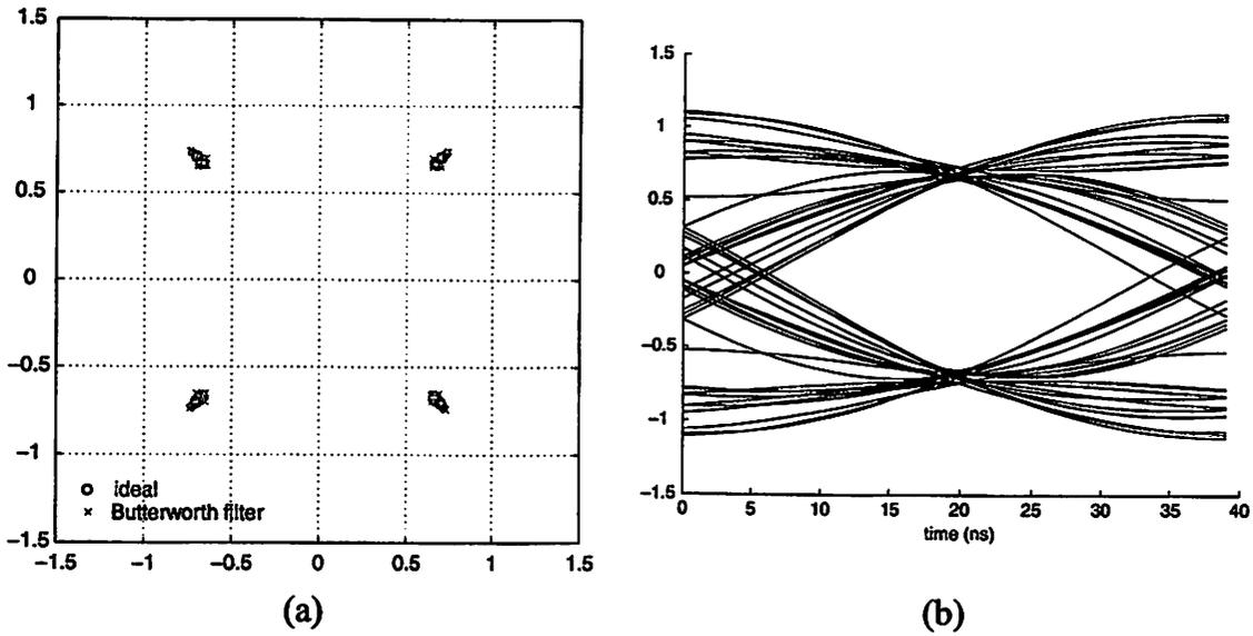
Figure 3.25: Butterworth filter. (a) Effect on a QPSK constellation. (b) Eye diagram.
