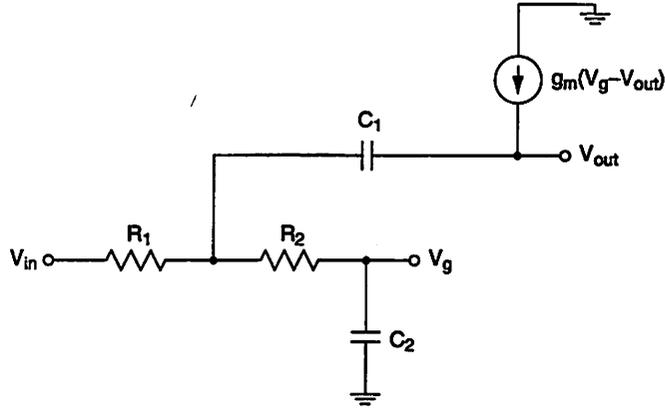
Figure 6.49: Equivalent half-circuit of Sallen and Key filter
