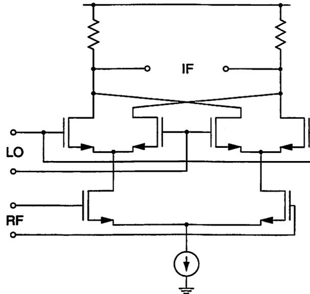
Figure 6.36: CMOS double-balanced current-commutating mixer.
