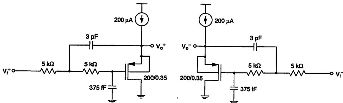
Figure 6.48: Sallen and Key filter circuit schematic.
