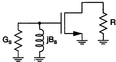
Figure 6.10: Common-source LNA with tuned input.
