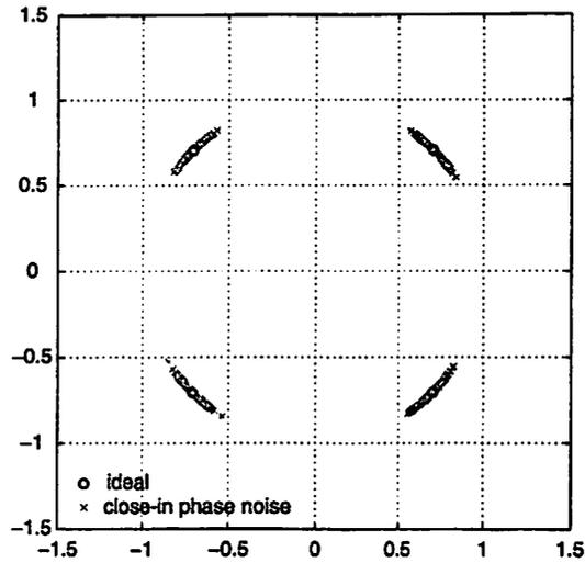
Figure 3.17: Effect of close-in phase noise on a QPSK constellation.
