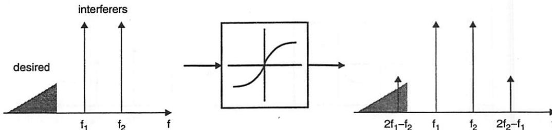
Figure 3.20: Third-order intermodulation distortion.
