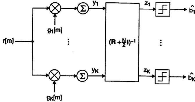
Figure 5.26: MMSE detector.
