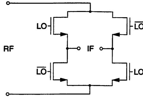
Figure 6.35: CMOS double-balanced passive mixer.
