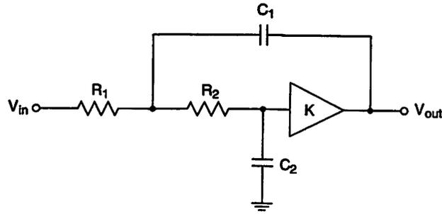
Figure 6.38: Sallen and Key filter block diagram.
