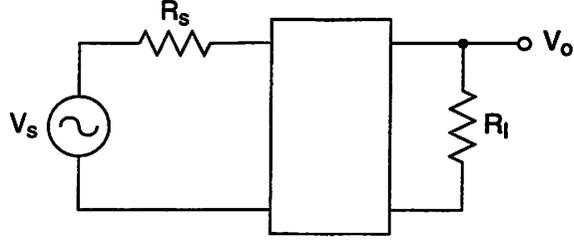
Figure C.2:  $R_s$  and  $R_l$  are fixed but the network connecting them is allowed to vary.
