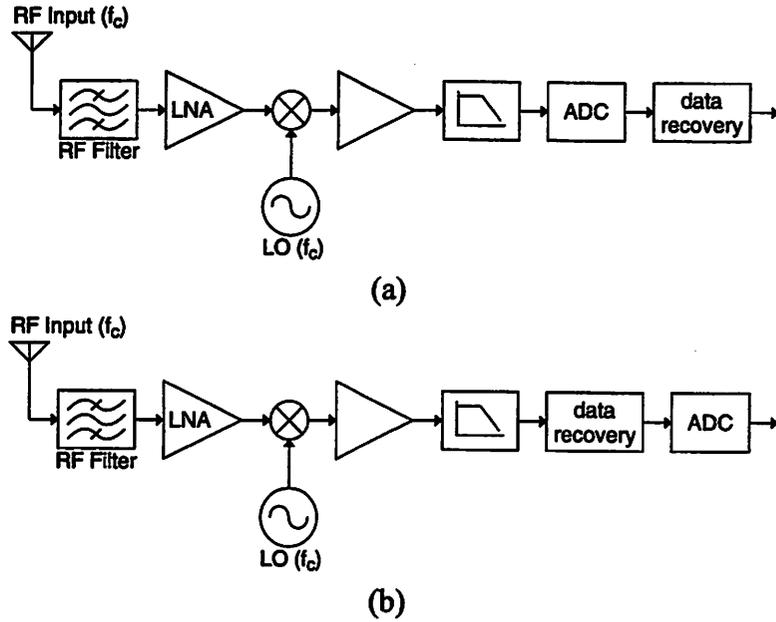
Figure 5.12: (a) ADC before data recovery. (b) ADC after data recovery.
