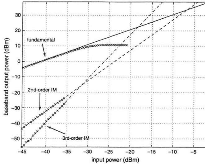
Figure 7.10: Measured receiver distortion performance.
