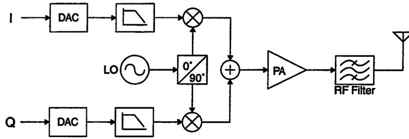
Figure 5.4: Block diagram of base-station transmitter (analog front-end).
