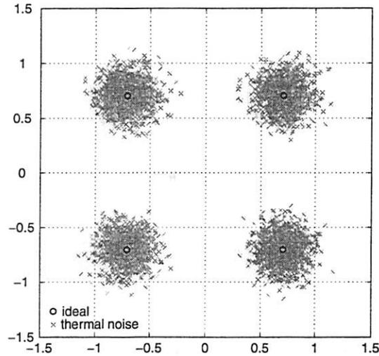
Figure 3.3: Effect of thermal noise on a QPSK constellation.
