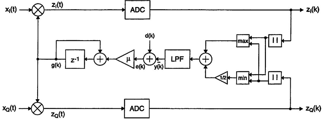
Figure 5.19: AGC loop based on sign-data LMS algorithm using (5.51).
