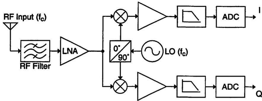
Figure 2.7: Direct-conversion architecture block diagram.
