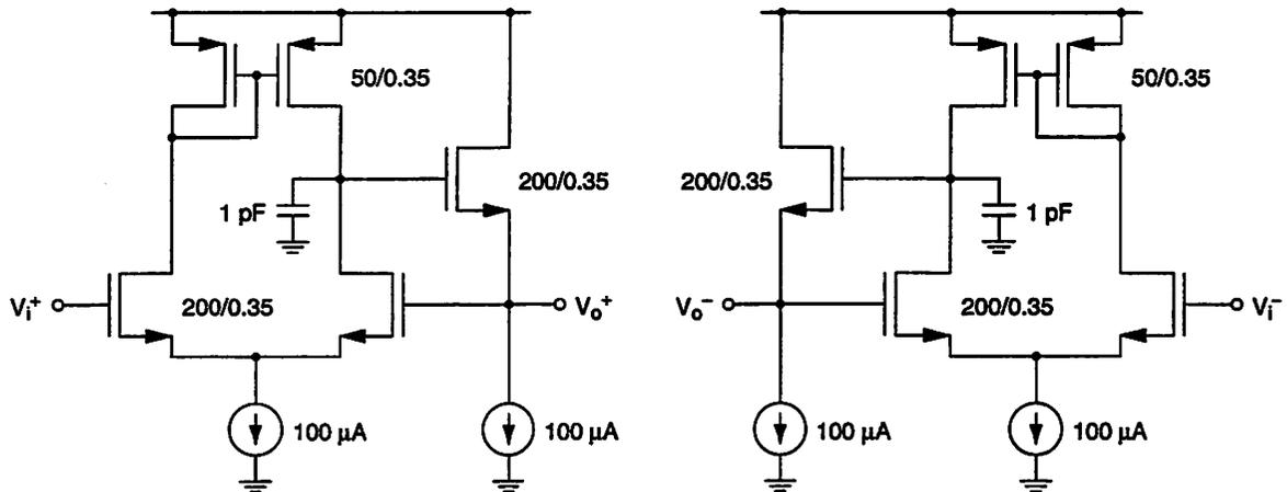
Figure 6.47: Buffer schematic.
