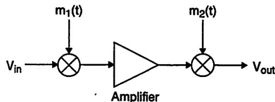
Figure 5.6: Chopper stabilization.
