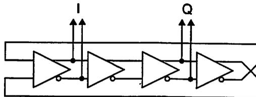
Figure 6.32: Example of a ring-oscillator VCO.
