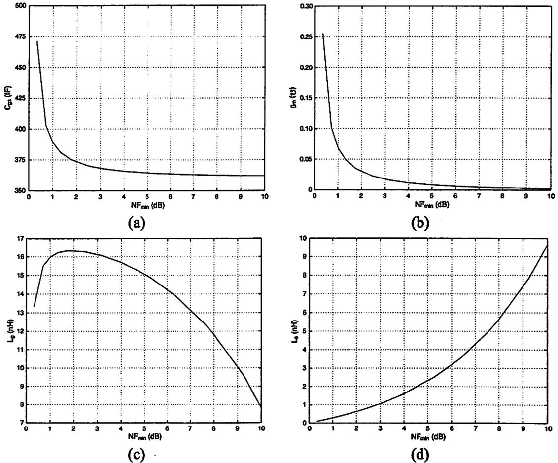
Figure 6.17: Designing for minimum noise figure in the common-source LNA with inductive degeneration. (a)  $C_{gs}$ . (b)  $g_m$ . (c)  $L_g$ . (d)  $L_s$ . ( $\alpha=0.8$ ,  $\delta=4$ ,  $\gamma=2$ ,  $c=j0.395$ ,  $G_s=1/(50\ \Omega)$ ,  $\omega=2\pi 2\times 10^9$  rad/s,  $L=L_{eff}=0.18\ \mu\text{m}$  ( $L_{drawn}=0.25\ \mu\text{m}$ ),  $\mu_{eff}=400\ \text{cm}^2/\text{Vs}$ ,  $E_{sat}=5\times 10^4$  V/cm,  $R_l=350\ \Omega$ .)
