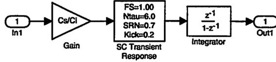
Figure 4.23: Model of integrator with a nonlinear transfer function.
