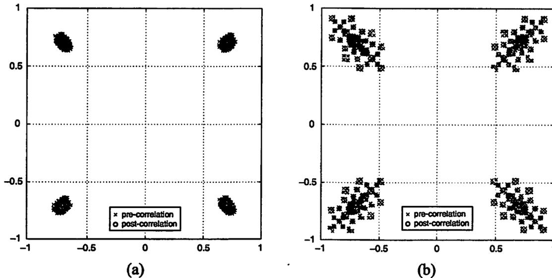
Figure 5.7: Effect of high-pass filtering. (a) 100 kHz. (b) 500 kHz.
