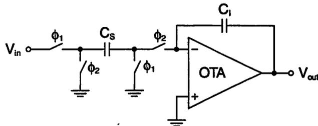
Figure 4.18: Switched-capacitor integrator.
