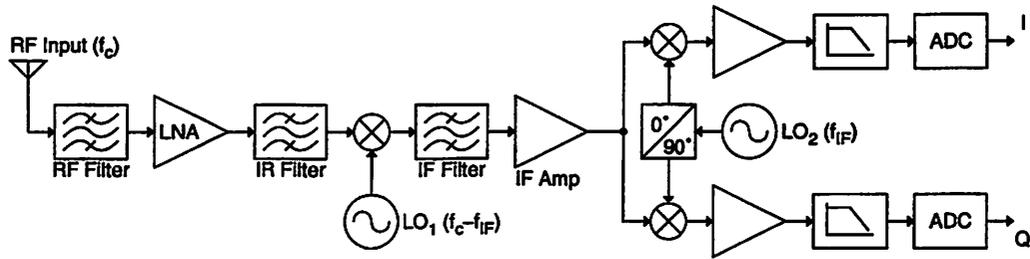
Figure 2.3: Heterodyne architecture block diagram.
