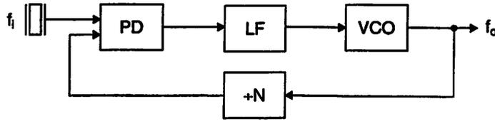
Figure 4.12: PLL block diagram.
