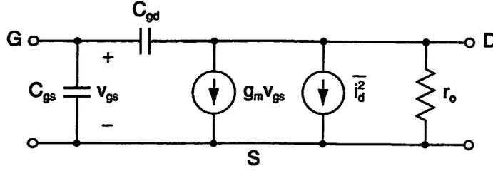
Figure 6.6: MOS small-signal equivalent circuit with noise generators.
