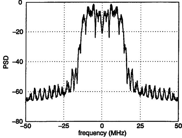
Figure 5.10: Simulated transmit spectrum.
