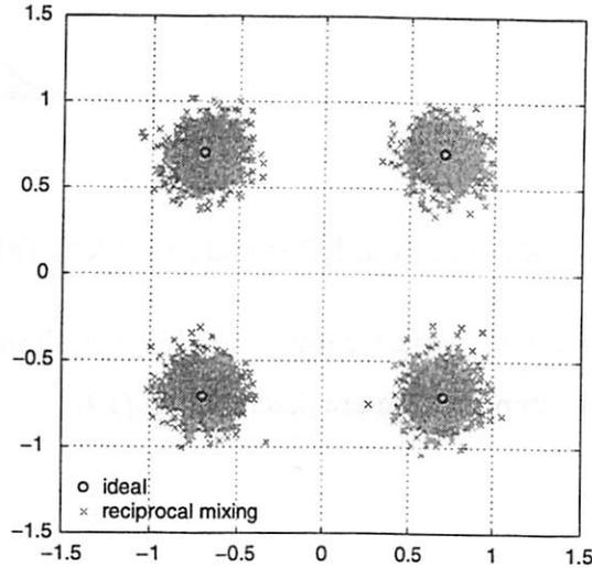
Figure 3.15: Effect of reciprocal mixing on a QPSK constellation.
