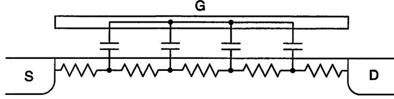
Figure 6.7: Distributed gate capacitance and channel resistance at high frequencies.
