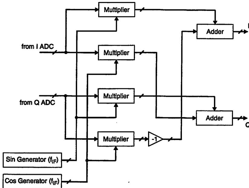
Figure 2.15: Digital frequency translation block diagram.
