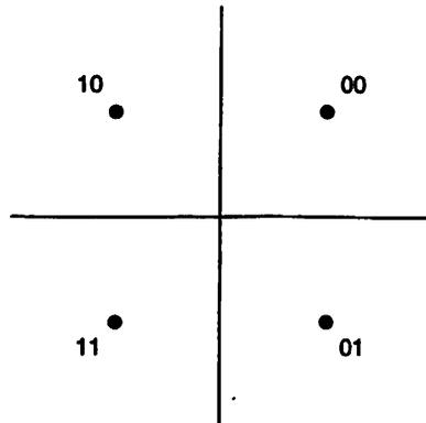
Figure 3.1: QPSK constellation diagram.
