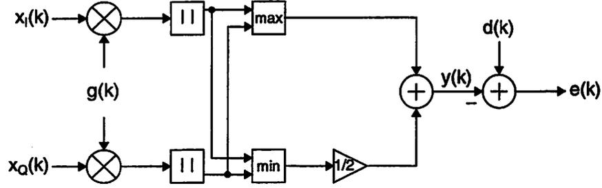
Figure 5.18: Equivalent combiner for feedback AGC loop based on (5.51).
