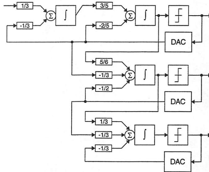
Figure 6.53: 2-1-1 cascade  $\Sigma\Delta$  architecture.
