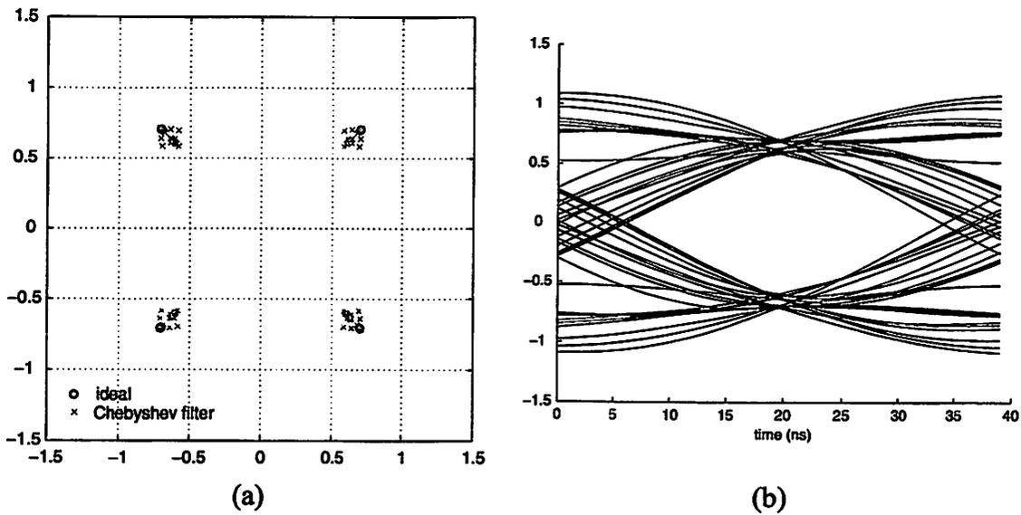
Figure 3.26: Chebyshev filter. (a) Effect on a QPSK constellation. (b) Eye diagram.
