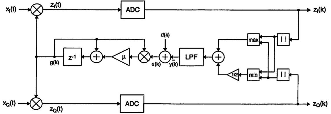
Figure 5.21: AGC loop based on the update equation in (5.101).
