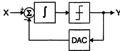
Figure 4.17: First-order  $\Sigma\Delta$  converter.
