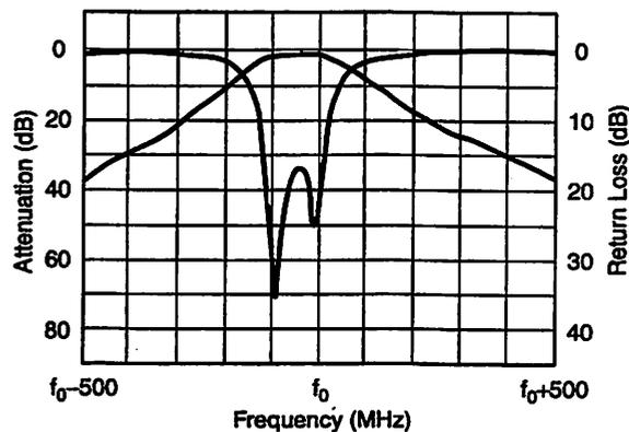
Figure 2.5: Typical ceramic filter characteristic.
