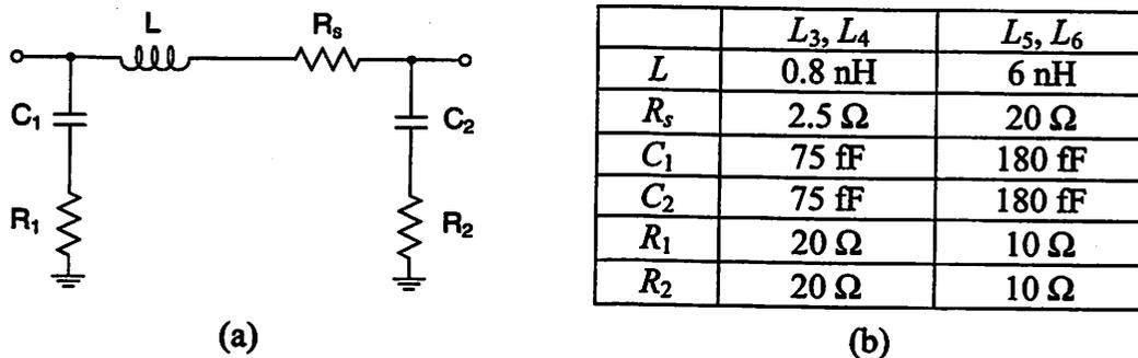
Figure 6.27: (a) Circuit model for on-chip spiral inductors. (b) Component values at 2 GHz.
