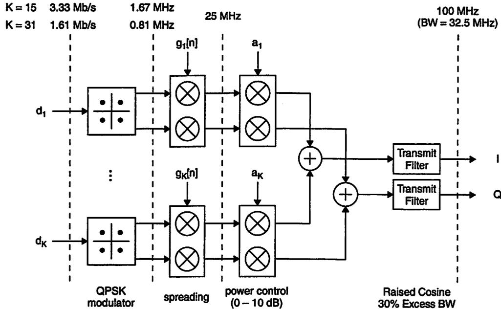
Figure 5.1: Block diagram of base-station transmitter (digital baseband section).
