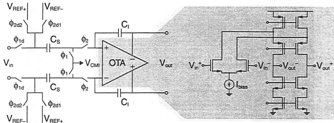
Figure 6.54: Switched-capacitor integrator.
