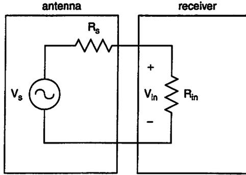
Figure 4.1: Circuit model of antenna with receiver input.
