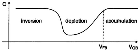
Figure 6.45: Capacitance of poly/n-well structure versus bias voltage.
