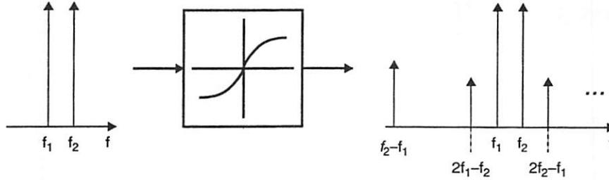
Figure 3.19: Intermodulation distortion.
