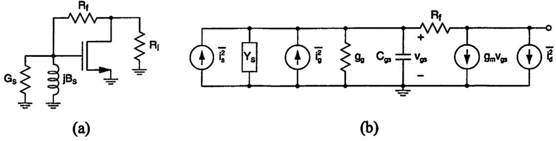
Figure 6.14: (a) Local shunt feedback LNA. (b) Small-signal equivalent circuit.
