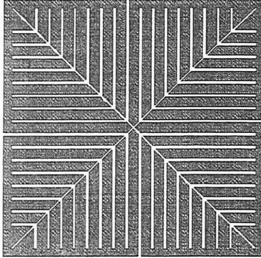
Figure D.4: Patterned polysilicon ground shield.
