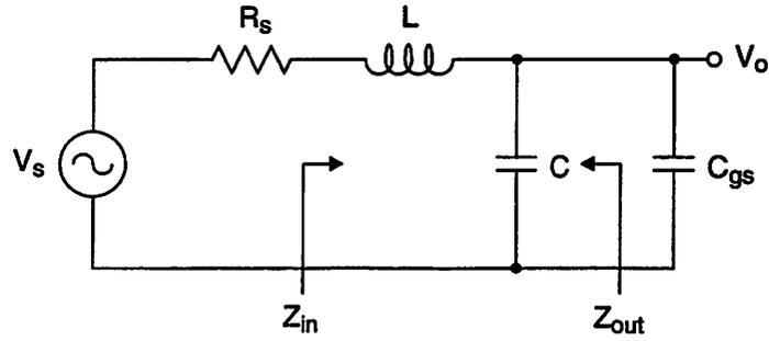
Figure C.5: Singly-terminated RF filter.
