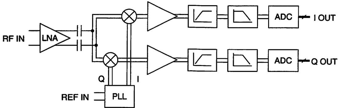
Figure 6.1: Block diagram of receiver prototype.
