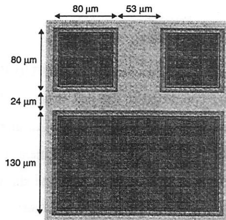
Figure D.3: Pad structure for inductors.
