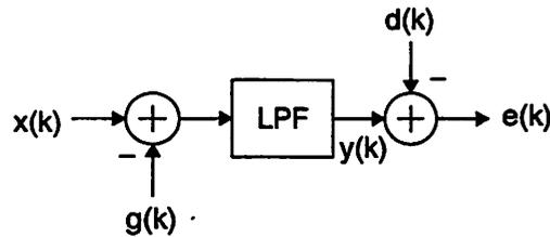
Figure B.3: Equivalent combiner for a feedback dc-offset correction loop.
