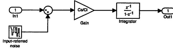
Figure 4.21: Model of integrator with noise.
