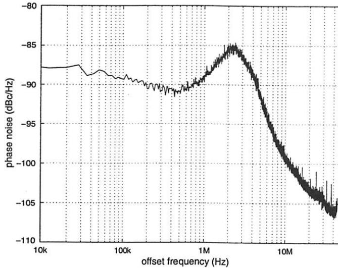
Figure 7.12: Measured phase noise performance of the frequency synthesizer.
