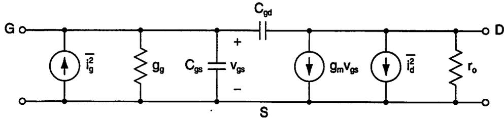
Figure 6.8: Revised MOS small-signal equivalent circuit with noise generators.
