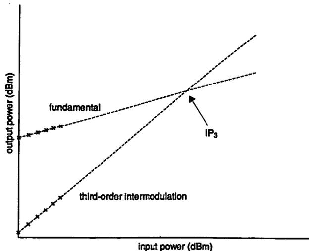
Figure 4.5: Third-order intermodulation intercept point.
