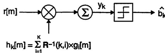
Figure 5.25: Decorrelating detector for a single data channel.
