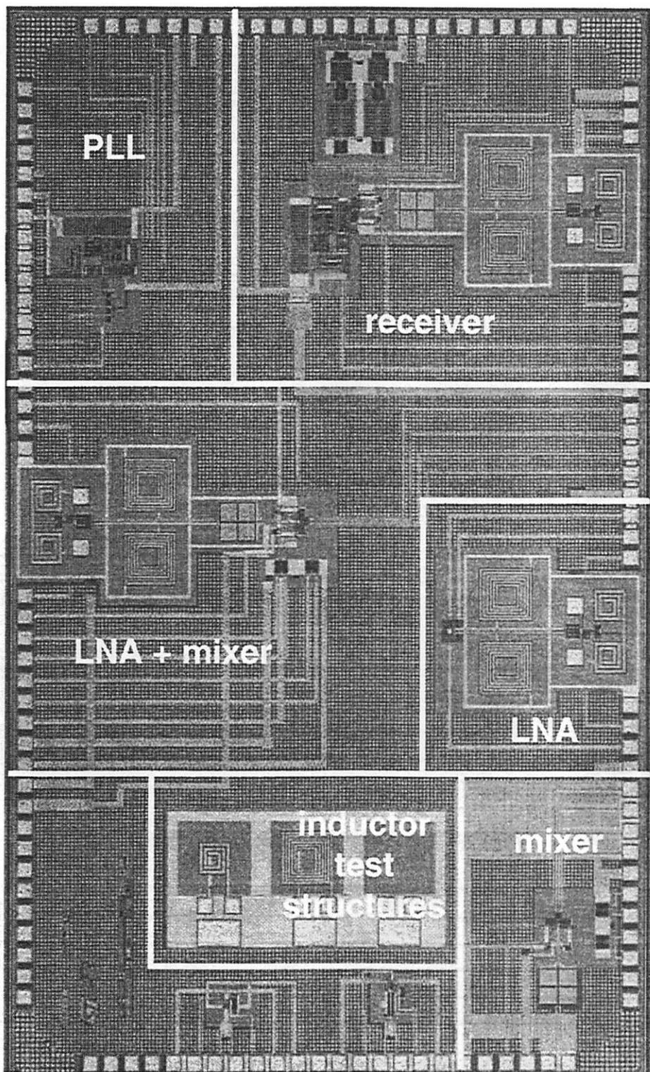
Figure 6.55: Test chip (SCRRX) micrograph.
