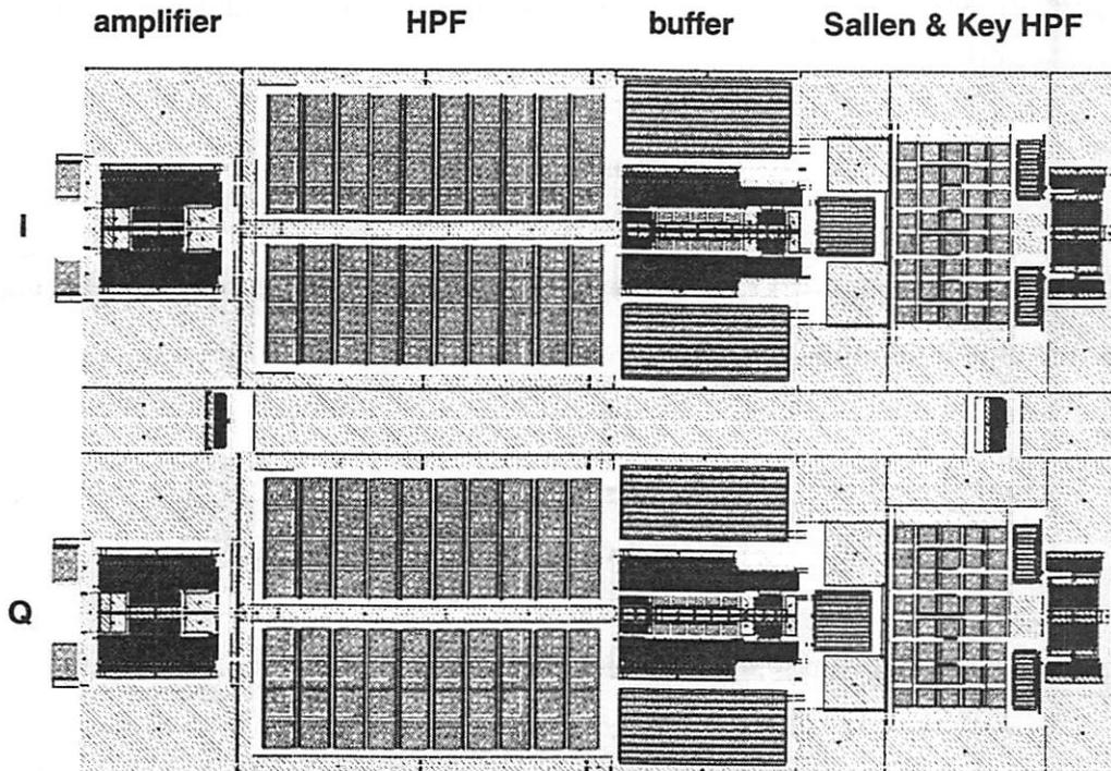
Figure 6.50: Layout of baseband amplifiers and filters.
