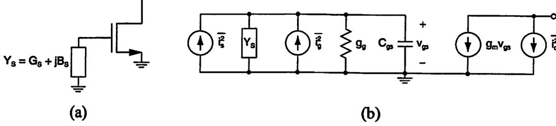
Figure 6.9: (a) Common-source amplifier. (b) Small-signal equivalent circuit.
