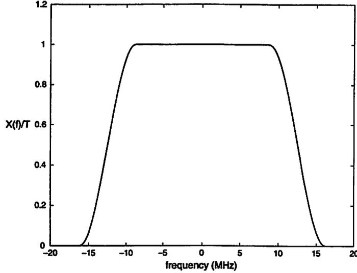
Figure 5.2: Frequency response of raised-cosine pulse ( $1/T = 25$  MHz,  $\beta = 0.3$ ).
