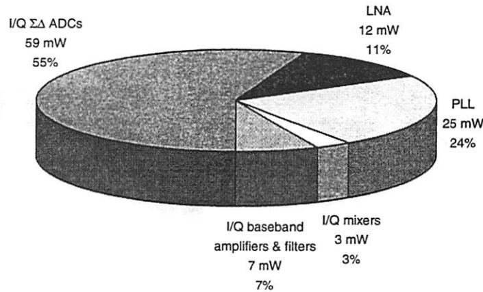
Figure 7.11: Measured receiver power consumption.
