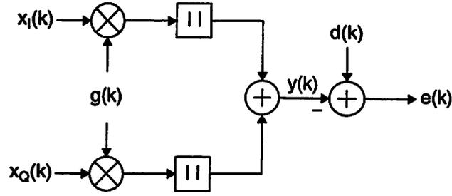
Figure 5.17: Equivalent combiner for feedback AGC loop based on (5.50).
