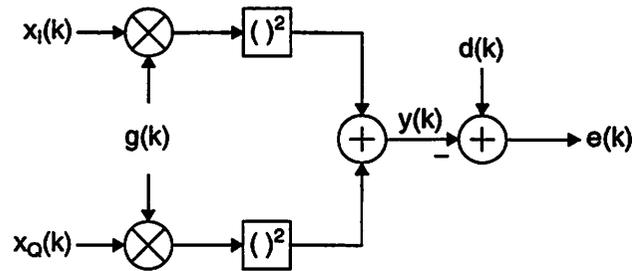
Figure 5.16: Equivalent combiner based on  $I^2 + Q^2$ .
