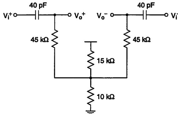
Figure 6.46: High-pass filter schematic.
