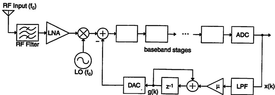
Figure B.4: Implementation of adaptive dc-offset correction loop.
