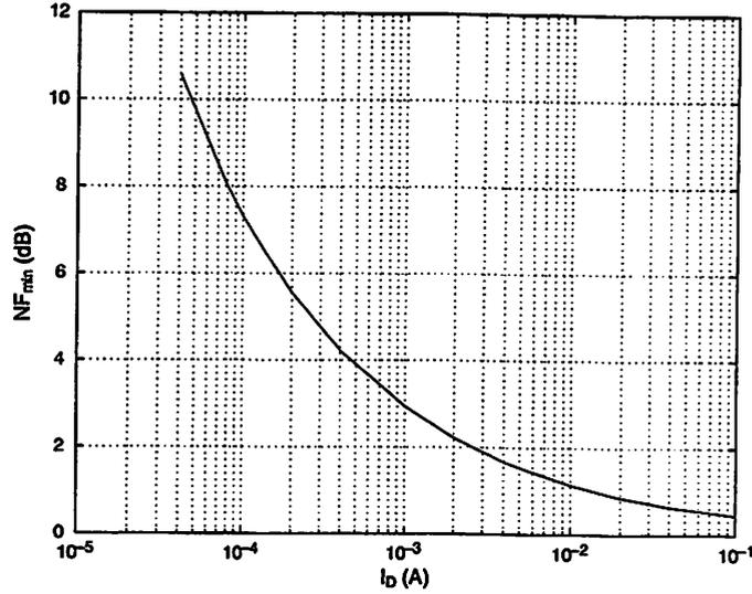
Figure 6.15:  $NF_{min}$  versus  $I_D$  for the LNA topology with local shunt feedback. ( $\alpha=0.8$ ,  $\delta=4$ ,  $\gamma=2$ ,  $c=j0.395$ ,  $G_s=1/(50\ \Omega)$ ,  $\omega=2\pi 2\times 10^9$  rad/s,  $L=L_{eff}=0.18\ \mu\text{m}$  ( $L_{drawn}=0.25\ \mu\text{m}$ ),  $\mu_{eff}=400\ \text{cm}^2/\text{Vs}$ ,  $E_{sat}=5\times 10^4$  V/cm,  $R_l=350\ \Omega$ .)
