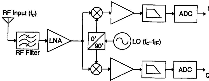
Figure 2.14: Low-IF architecture block diagram.
