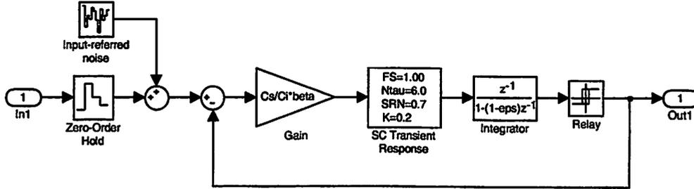
Figure 4.24: Structural model of first-order  $\Sigma\Delta$  converter.
