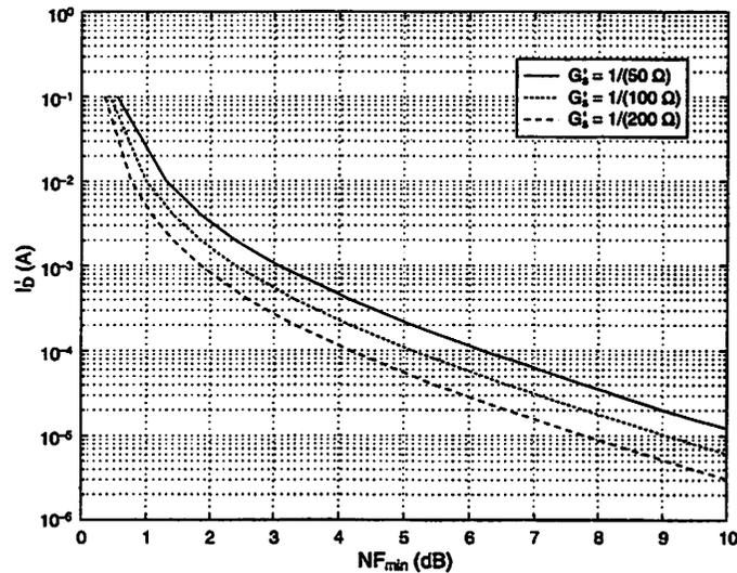
Figure 6.20: Drain current versus noise figure of the inductively-degenerated differential LNA for several values of source conductance.
