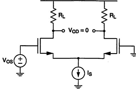
Figure 2.9: Input offset voltage for a differential CMOS amplifier.
