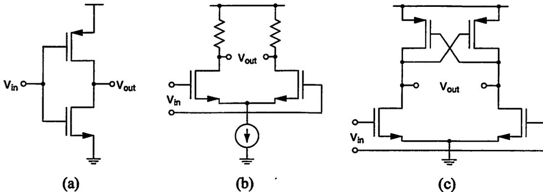
Figure 6.34: Inverter implementations. (a) Static CMOS. (b) SCL. (c) DCVSL.
