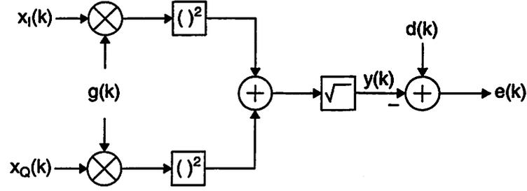
Figure 5.15: Equivalent combiner for feedback AGC loop based on (5.49).
