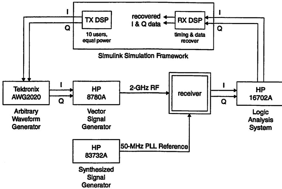
Figure 7.14: Test setup for receiver measurement with a modulated RF input signal.
