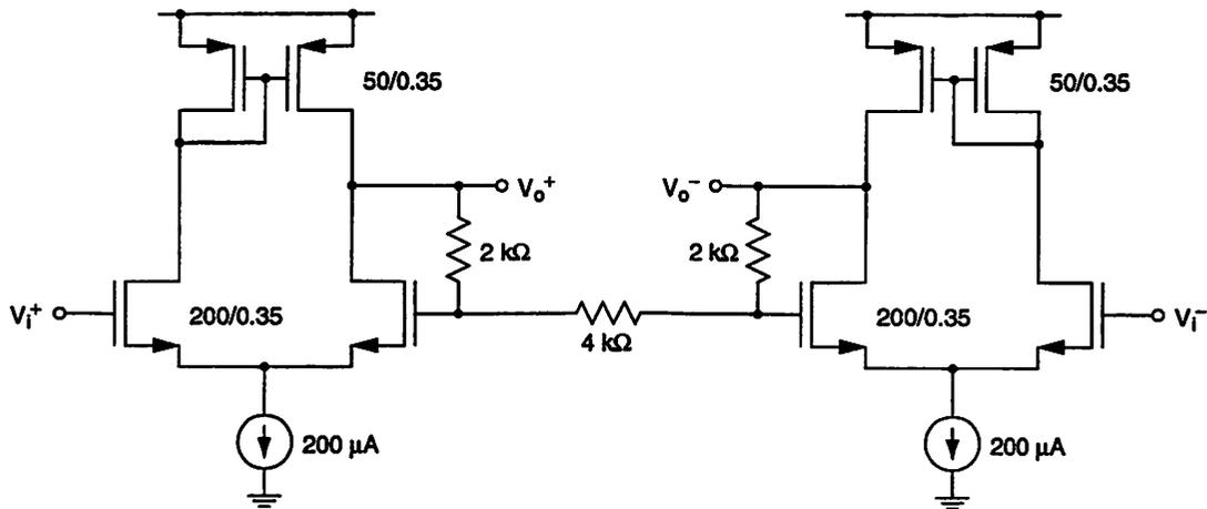
Figure 6.44: Noninverting amplifier schematic.
