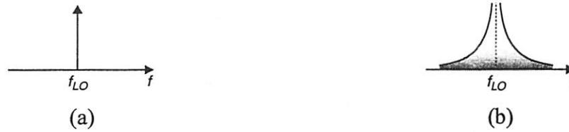
Figure 3.13: Frequency spectra of LO signals. (a) Ideal. (b) With phase noise.
