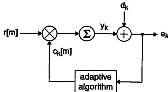
Figure 5.27: Adaptive MMSE detector for a single data channel.
