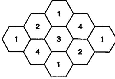
Figure 5.3: Cellular reuse pattern with  $N = 4$ .
