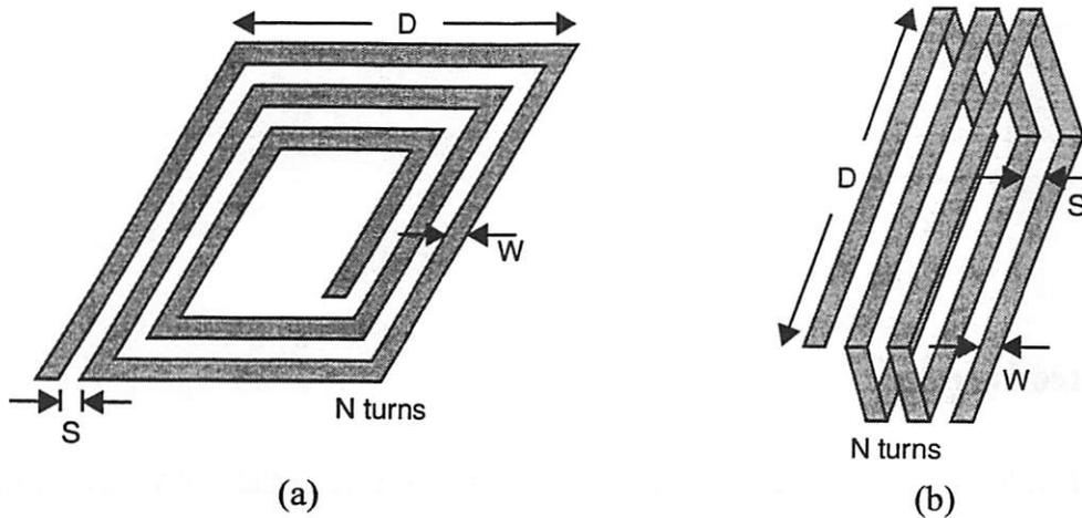
Figure D.1: Definition of geometric parameters. (a) Inductors 1 – 6. (b) Inductor 7.
