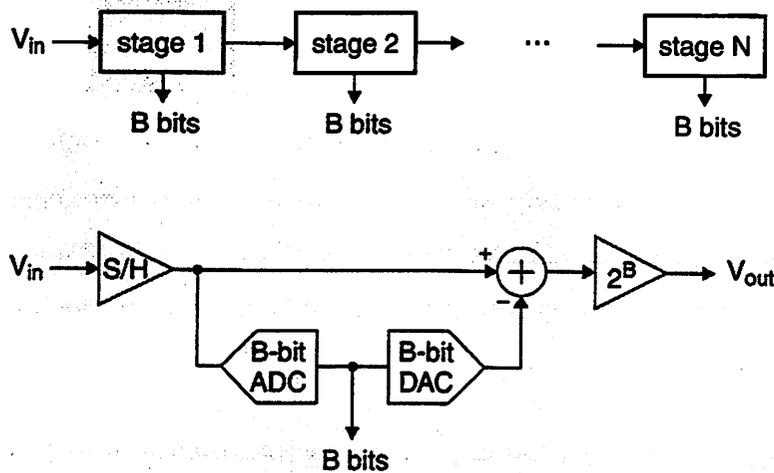
Figure 6.51: Pipeline ADC architecture.
