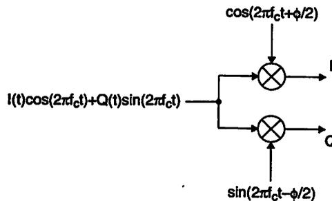
Figure 3.8: Quadrature phase mismatch in a direct-conversion receiver.
