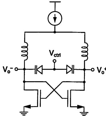
Figure 6.31: Example of a differential LC-tuned VCO.
