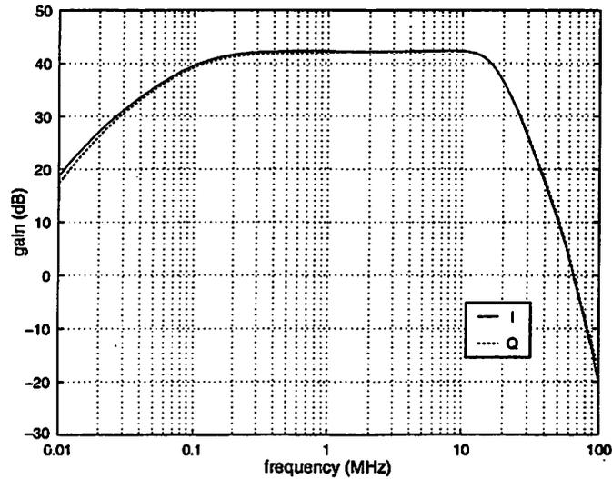
Figure 7.7: Measured frequency response at the output of each of the I and Q Sallen and Key filters.
