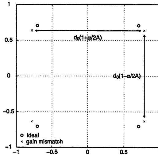
Figure 3.6: Effect of gain mismatch on a QPSK constellation.
