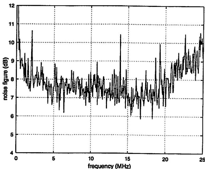
Figure 7.9: Measured receiver noise performance.
