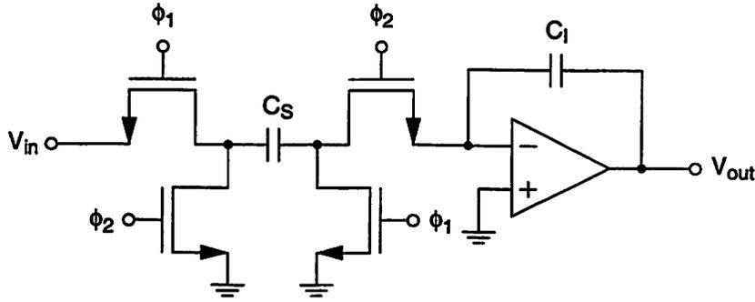
Figure 6.42: Switched-capacitor integrator.
