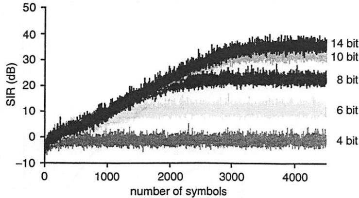
Figure 3.29: Effect of ADC resolution on an adaptive MUD algorithm [22].
