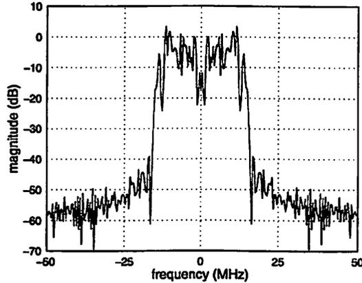
Figure 7.3: Baseband transmit spectrum from Simulink.
