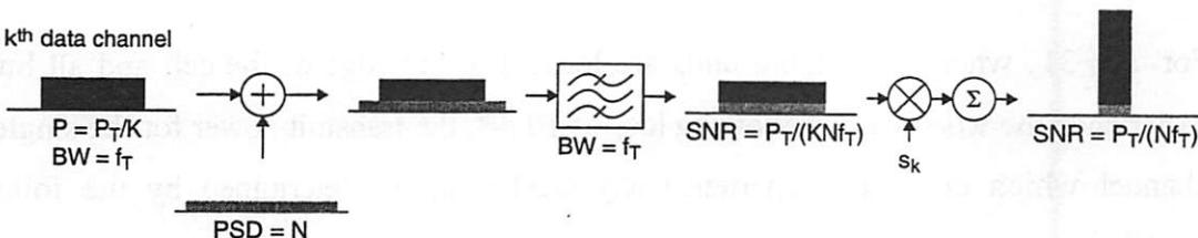
Figure 5.5: Comparison of FDMA and CDMA systems.
