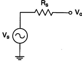
Figure C.7: Antenna circuit model.
