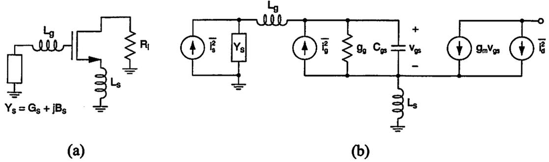
Figure 6.12: (a) Common-source LNA with inductive degeneration. (b) Small-signal equivalent circuit.
