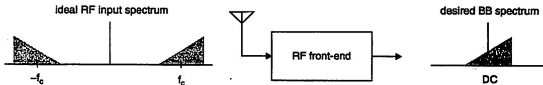
Figure 2.1: RF front-end for an ideal RF input signal.
