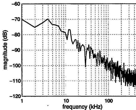
Figure 4.11: Example spectrum of phase noise generated by simple behavioral model.
