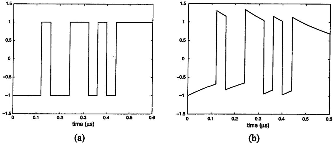
Figure 5.8: (a)  $K = 15$  spreading code. (b) After 500-kHz high-pass filter.
