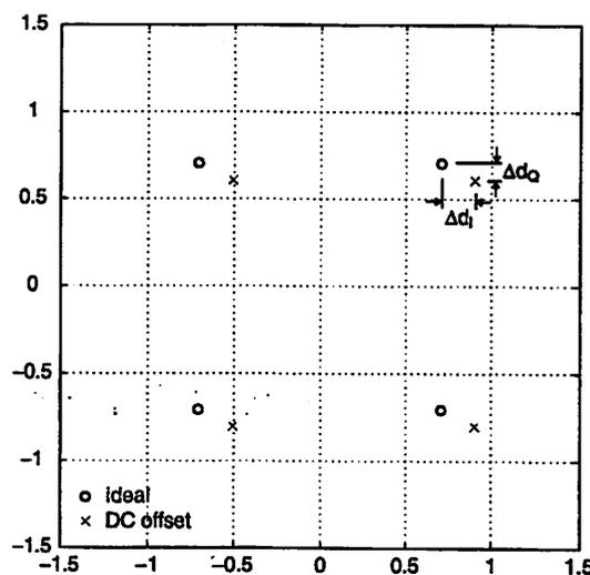
Figure 3.27: Effect of dc offsets on a QPSK constellation.
