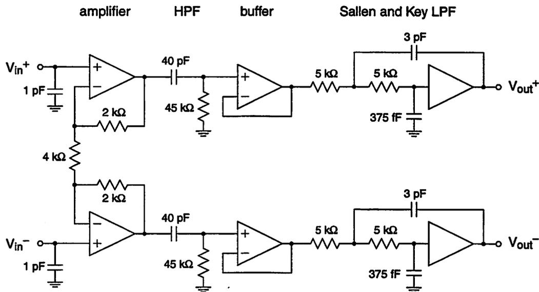
Figure 6.43: Block diagram of baseband amplification and filtering.
