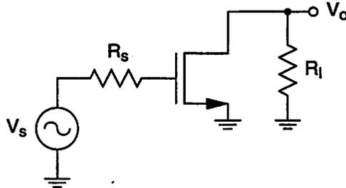
Figure C.4: Common-source LNA.
