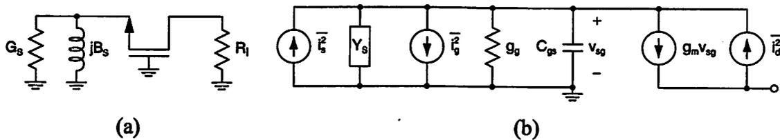
Figure 6.11: (a) Common-gate LNA. (b) Small-signal equivalent circuit.
