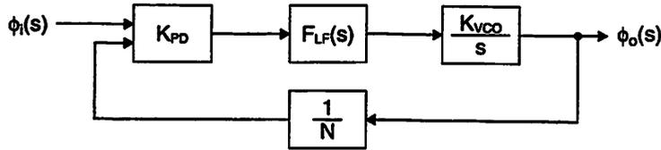
Figure 4.13: Linear model of PLL.
