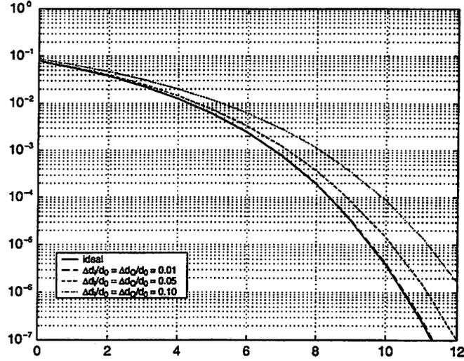
Figure 3.28: Probability of error for QPSK with dc offsets.
