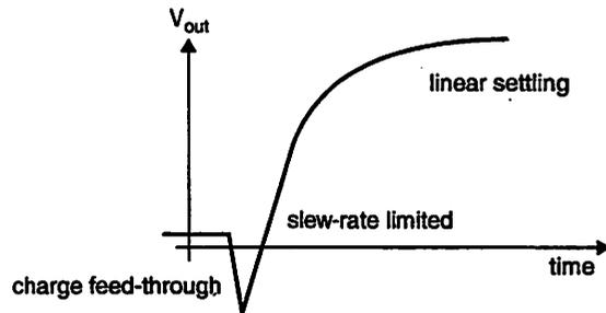
Figure 4.22: Switched-capacitor integrator transient response.
