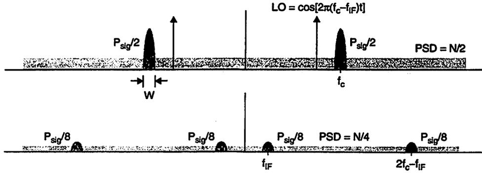
Figure 4.3: Frequency translation of RF signal to an intermediate frequency.
