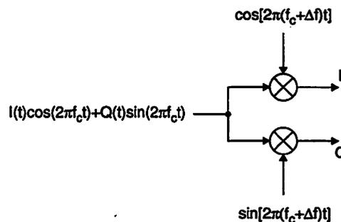
Figure 3.11: Frequency translation using I and Q LO signals with frequency offset.
