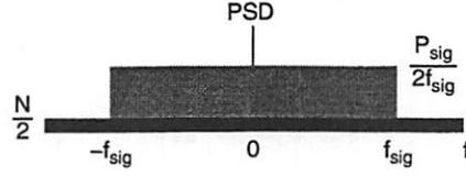
Figure 5.9: Signal and noise power spectral densities.
