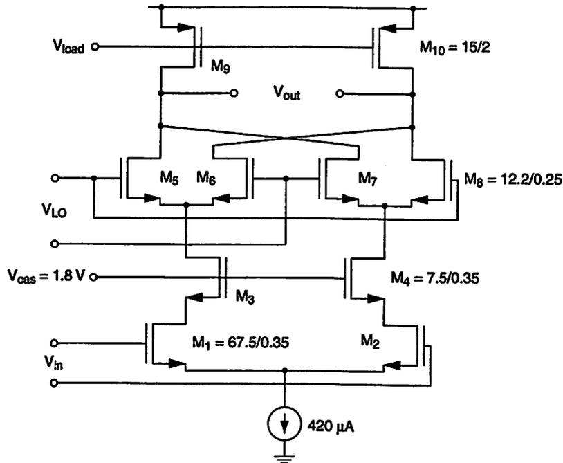
Figure 6.37: Mixer topology used in the receiver prototype.
