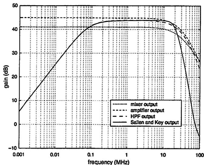
Figure 7.2: Simulated frequency responses at the outputs of various receiver components (typical process corner).
