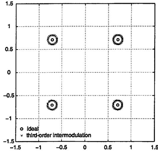
Figure 3.21: Effect of intermodulation distortion on a QPSK constellation.
