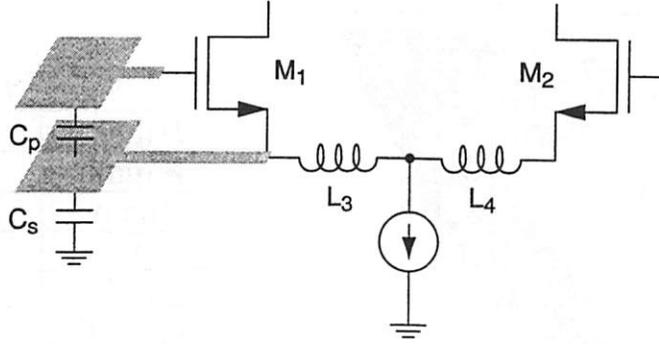
Figure 6.24: Interface between LNA and input pads.
