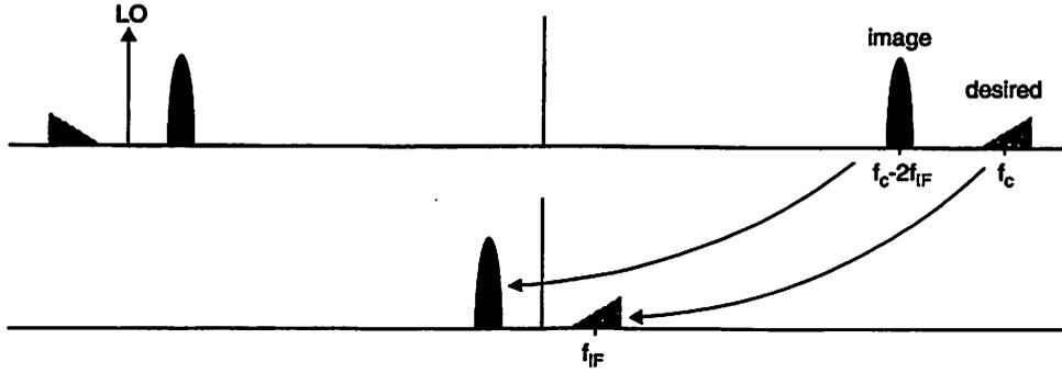
Figure 2.11: Frequency translation to  $f_{IF}$  using a complex sinusoidal LO signal.
