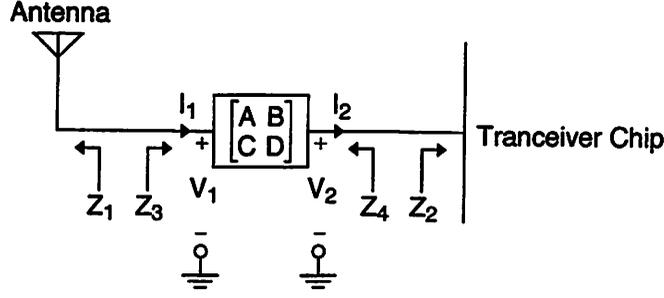
Figure C.1: Transmission matrix representation of the RF filter.
