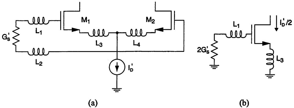
Figure 6.19: (a) Differential LNA with source conductance  $G'_s$  and tail current  $I'_D$ . (b) Equivalent half-circuit.
