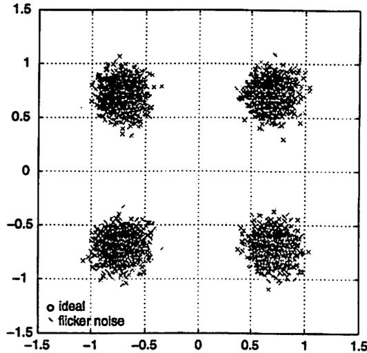
Figure 3.4: Effect of flicker noise on a QPSK constellation.
