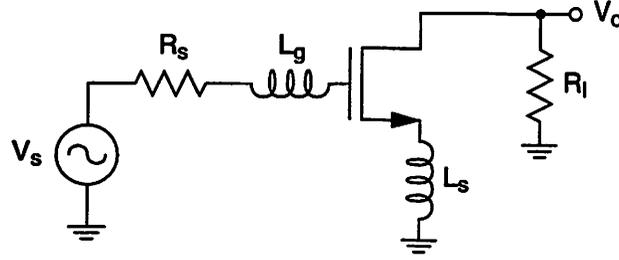
Figure C.6: Inductively-degenerated common-source LNA.
