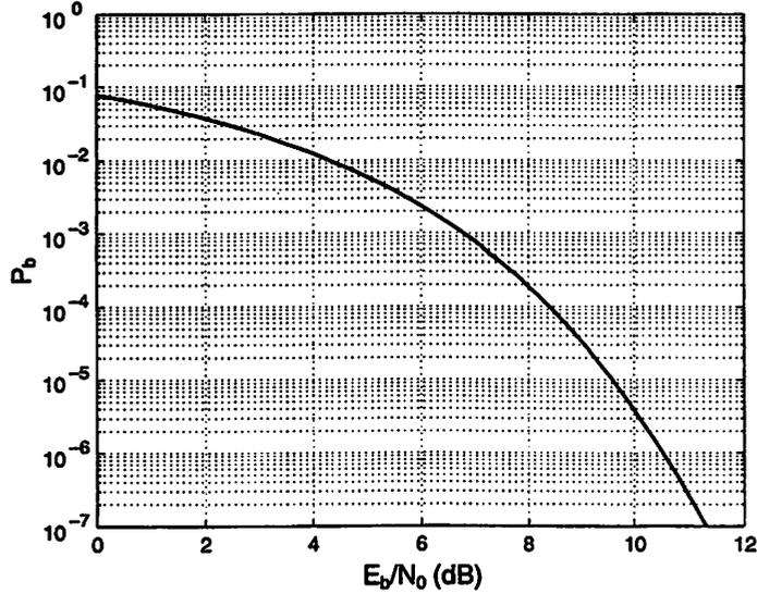
Figure 3.2: Probability of error for QPSK.
