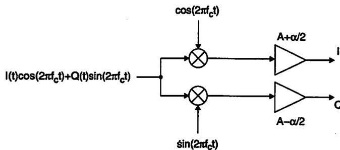
Figure 3.5: I and Q gain mismatch in a direct-conversion receiver.
