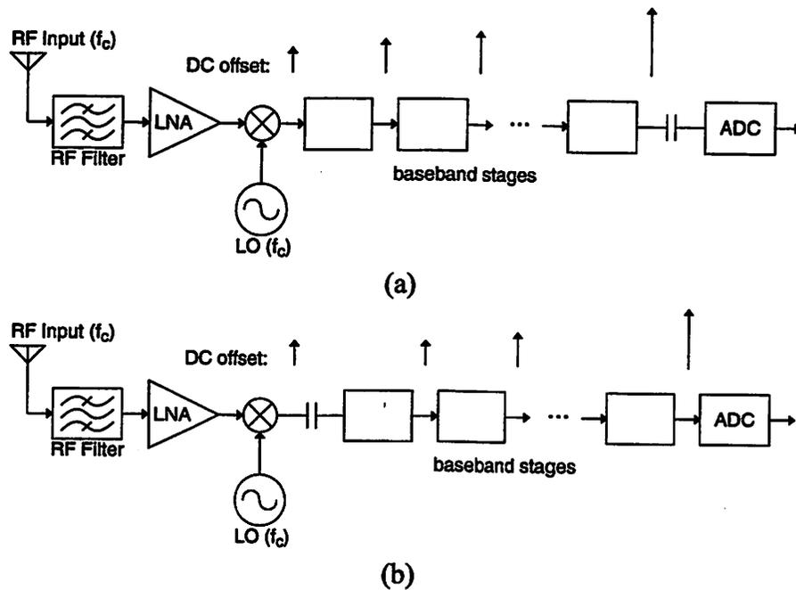
Figure 5.11: DC offset removal. (a) Before ADC. (b) After mixer.
