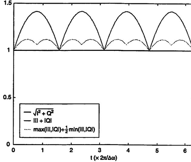
Figure 5.14: Amplitude estimates with frequency offset  $\Delta\omega$ .
