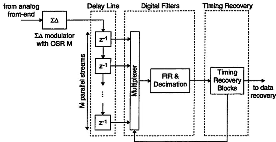
Figure 6.52:  $\Sigma\Delta$ -assisted timing recovery scheme.
