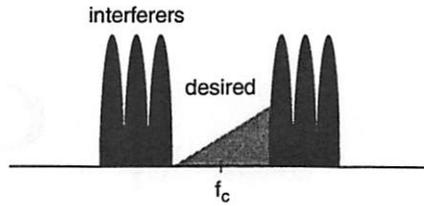
Figure 2.2: RF input signal with a weak desired signal and strong adjacent interferers.
