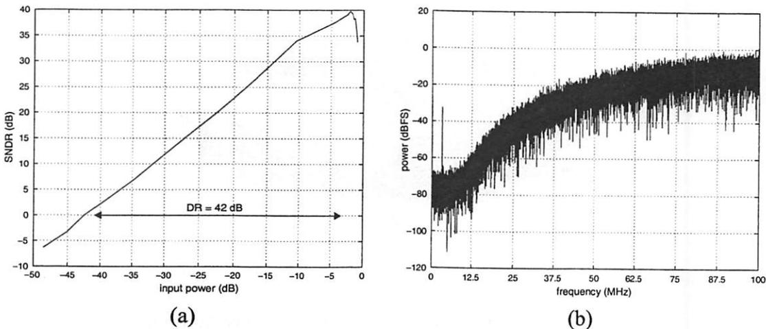
Figure 7.13:  $\Sigma\Delta$  modulator operating at 200 MHz. (a) Measured dynamic range. (b) Measured output spectrum.
