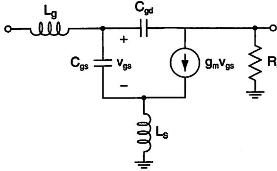
Figure 6.22: Small-signal equivalent circuit of the inductively-degenerated LNA including gate-drain overlap capacitance.
