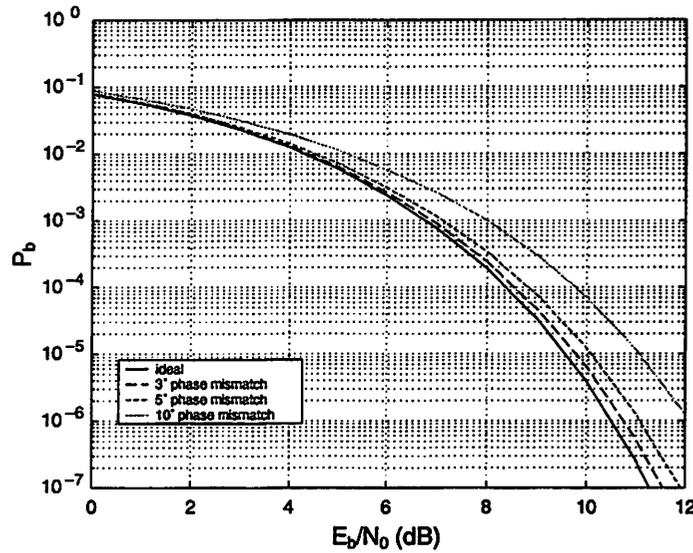
Figure 3.10: Probability of error for QPSK with quadrature phase mismatch.
