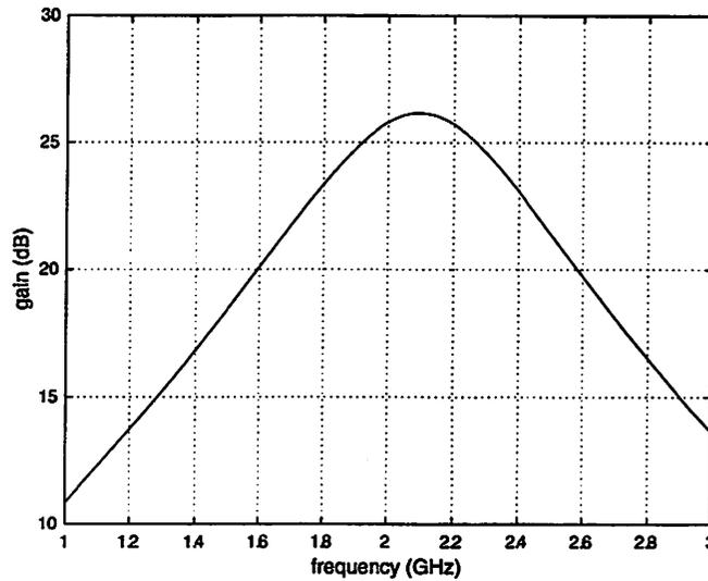
Figure 6.28: Simulated LNA gain.
