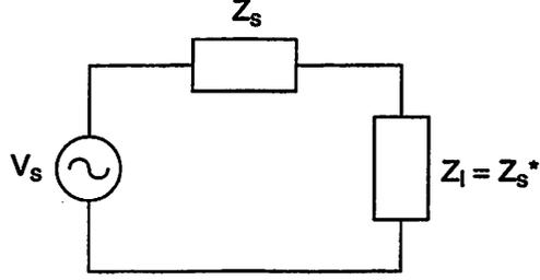
Figure 6.3: Conjugate impedance matching for maximum power transfer.
