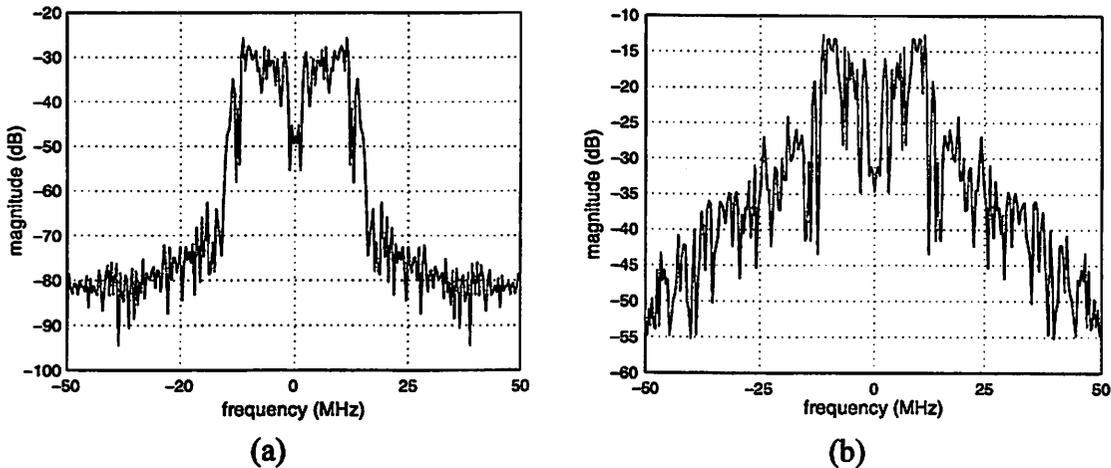
Figure 7.4: Spectrum of receiver output signal from transient envelop simulations. (a)  $-43$ -dBm input power. (b)  $-33$ -dBm input power.
