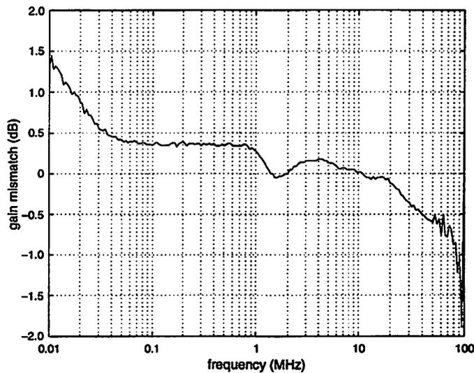
Figure 7.8: Measured I and Q gain mismatch.
