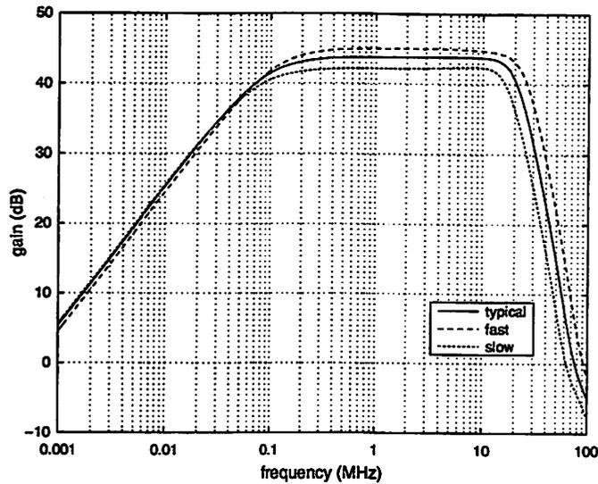
Figure 7.1: Simulated frequency response at the output of the Sallen and Key filter over process corners.
