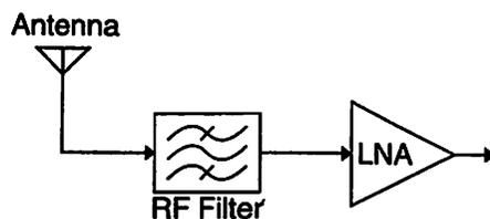
Figure 6.2: Antenna, RF filter, and LNA.
