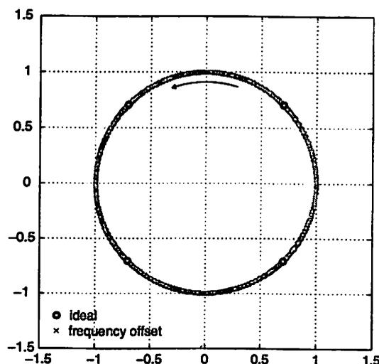
Figure 3.12: Effect of frequency offset on a QPSK constellation.
