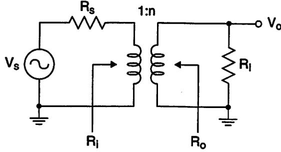
Figure C.3:  $R_s$  and  $R_l$  are connected through a transformer.
