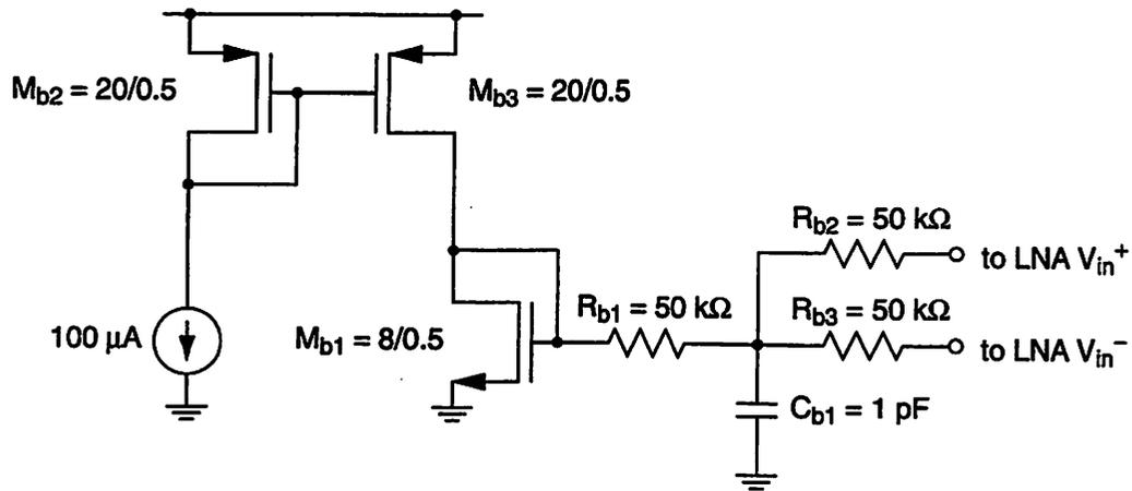
Figure 6.26: Bias circuit for the LNA input.
