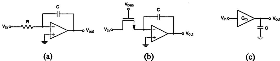
Figure 6.41: Integrators. (a) *RC*. (b) MOSFET-C. (c) Transconductance-C.
