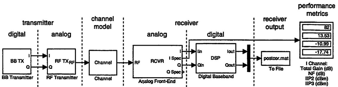
Figure 5.29: Top-level schematic of system downlink simulation.
