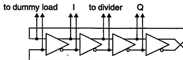
Figure 6.33: Four-stage ring-oscillator VCO.
