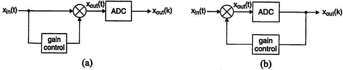
Figure 5.13: AGC architectures. (a) Feedforward. (b) Feedback.
