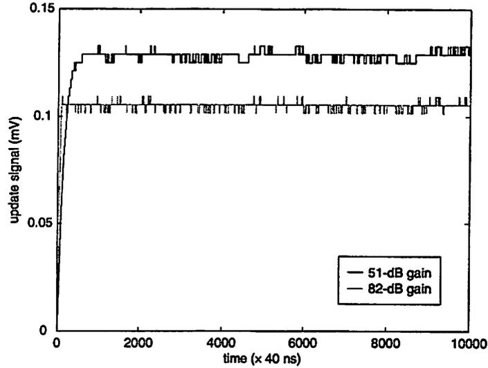
Figure B.5: Simulation of dc-offset cancellation loop.
