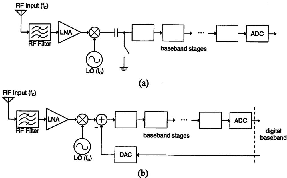
Figure B.2: DC-offset cancellation. (a) Capacitive storage. (b) Feedback DAC.
