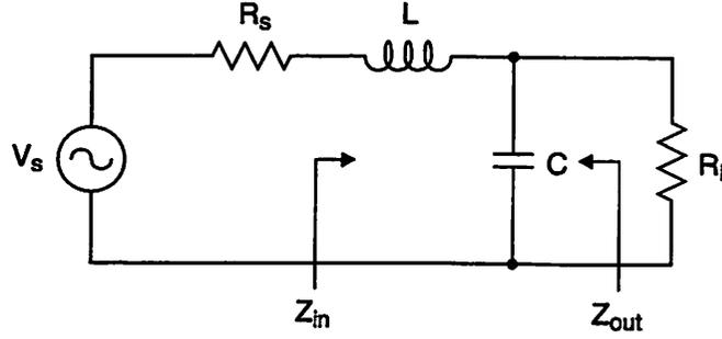
Figure 6.4: Circuit for second-order Butterworth low-pass filter.
