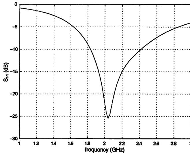
Figure 6.29: Simulated LNA  $S_{11}$ .
