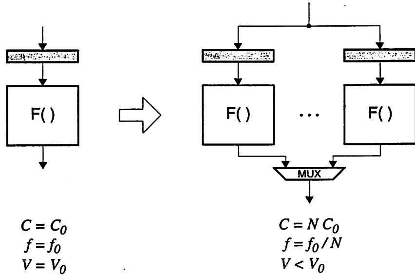
**Figure 2.6: Parallel Processing**
