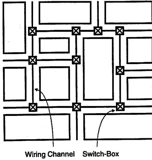
**Figure 5.8: Generalized Mesh Interconnect Structure**
