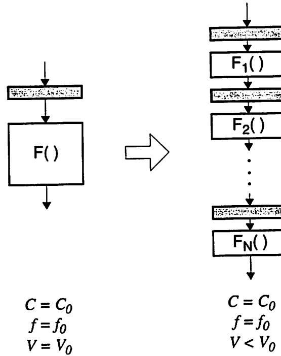
**Figure 2.7: Pipelined Processing**
