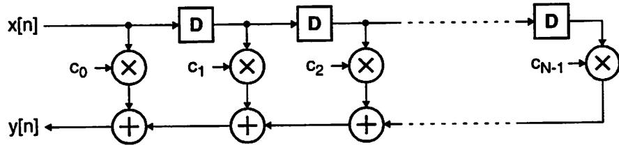
**Figure 3.1: Finite Impulse Response Filter**
