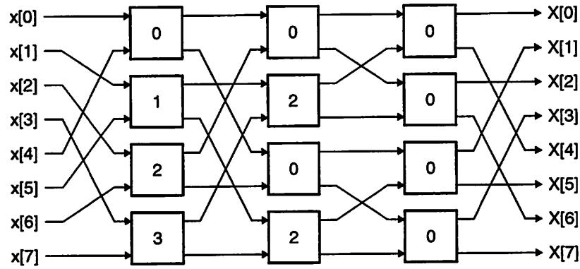
**Figure 3.3: 8-Point, Radix-2, Decimation-in-Frequency FFT**
