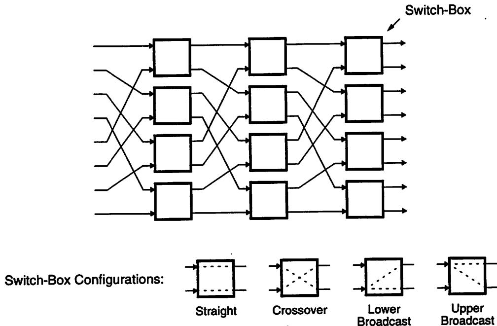
**Figure 5.5:  $8 \times 8$  Omega Multistage Interconnection Network**
