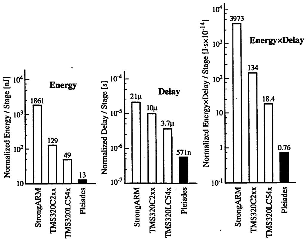
**Figure 7.6: Comparison Results for the FFT Benchmark**
