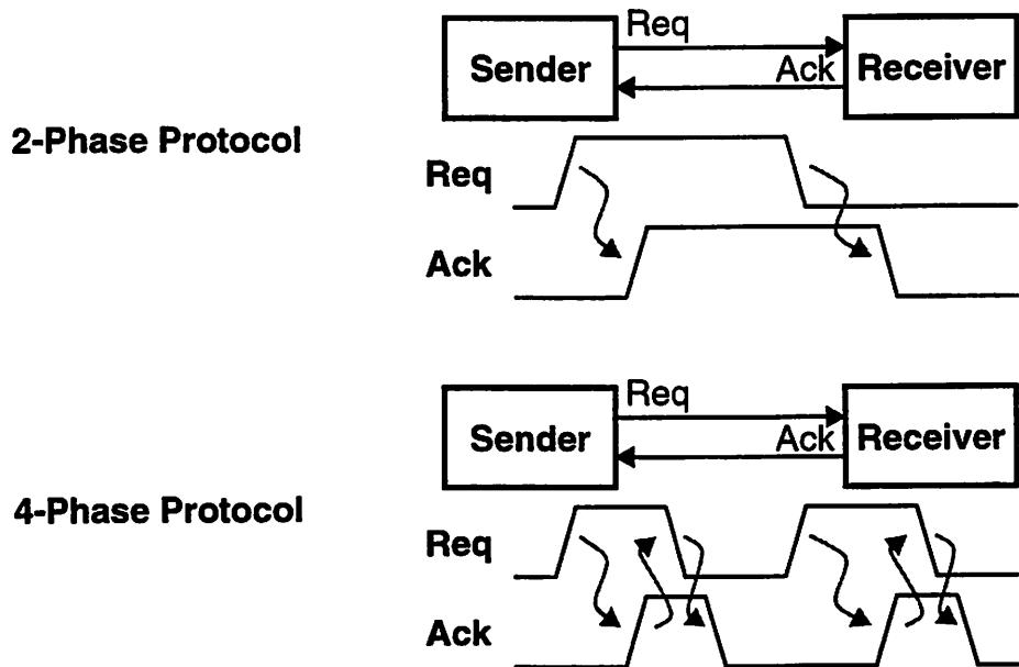
**Figure 5.17: Asynchronous Handshake Protocols**
