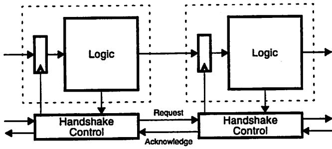
**Figure 2.8: Asynchronous Processing with Handshake Control**
