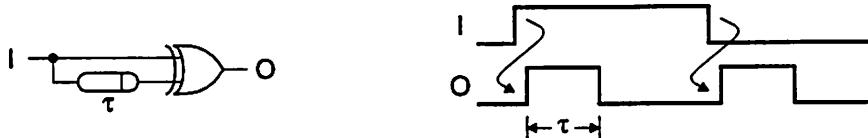
**Figure 5.18: Transition-to-Pulse Converter**
