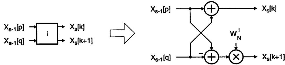
**Figure 3.4: Radix-2 FFT Butterfly Computation**
