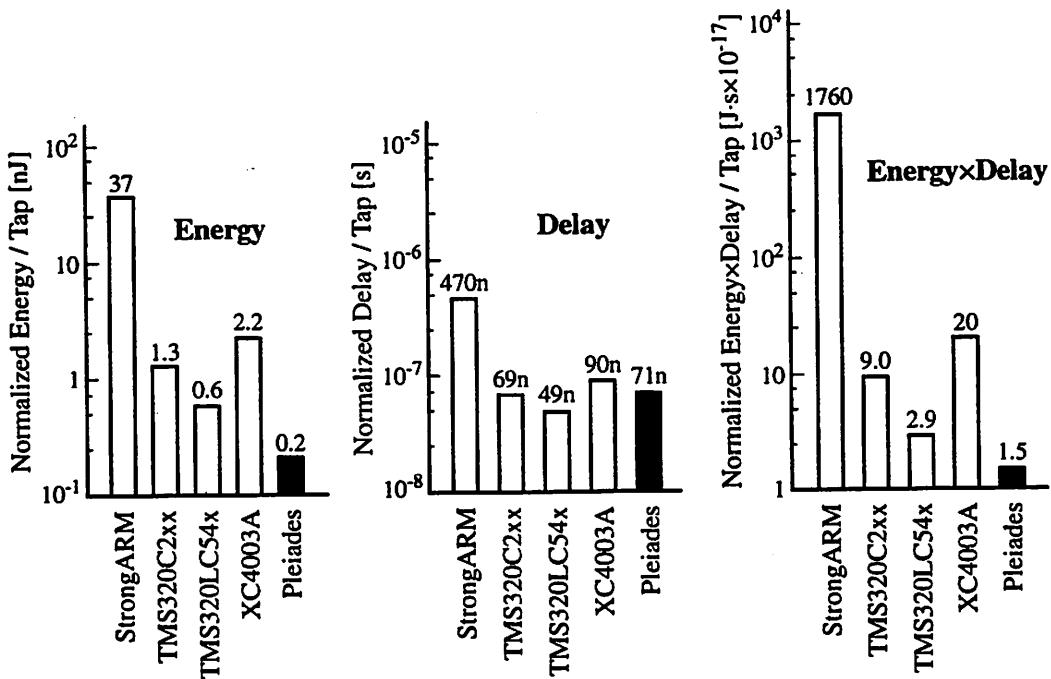
Figure 7.4: Comparison Results for the FIR Benchmark
