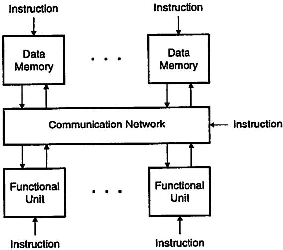
**Figure 4.1: Basic Model for Programmable Processors**
