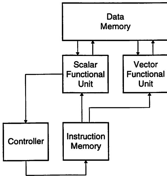
**Figure 4.6: Basic Architectural Model for Vector Processors**
