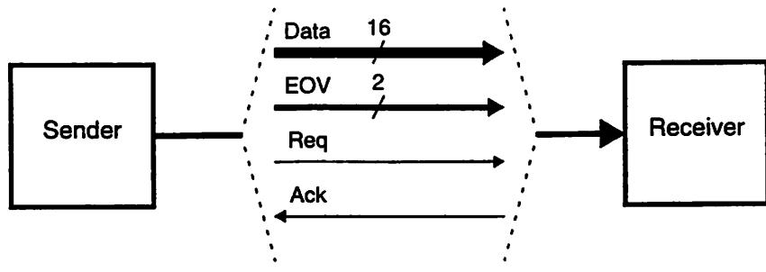
**Figure 5.24: Bundled Signals of a Communication Network Channel**
