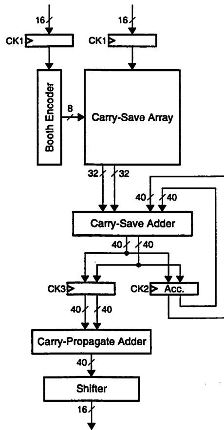
**Figure 6.8: Block Diagram of the Functional Core of the MAC Unit**
