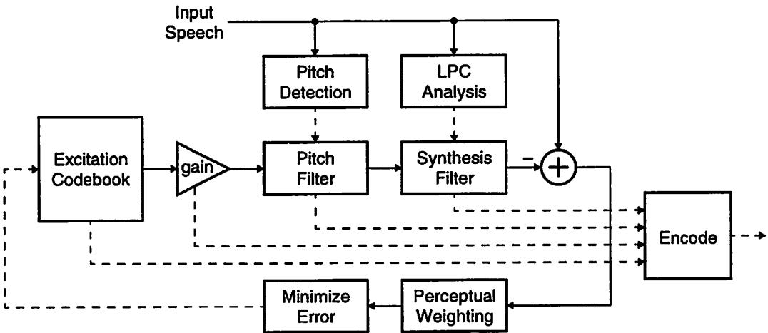
**Figure 3.8: Structure of a CELP Speech Coder**
