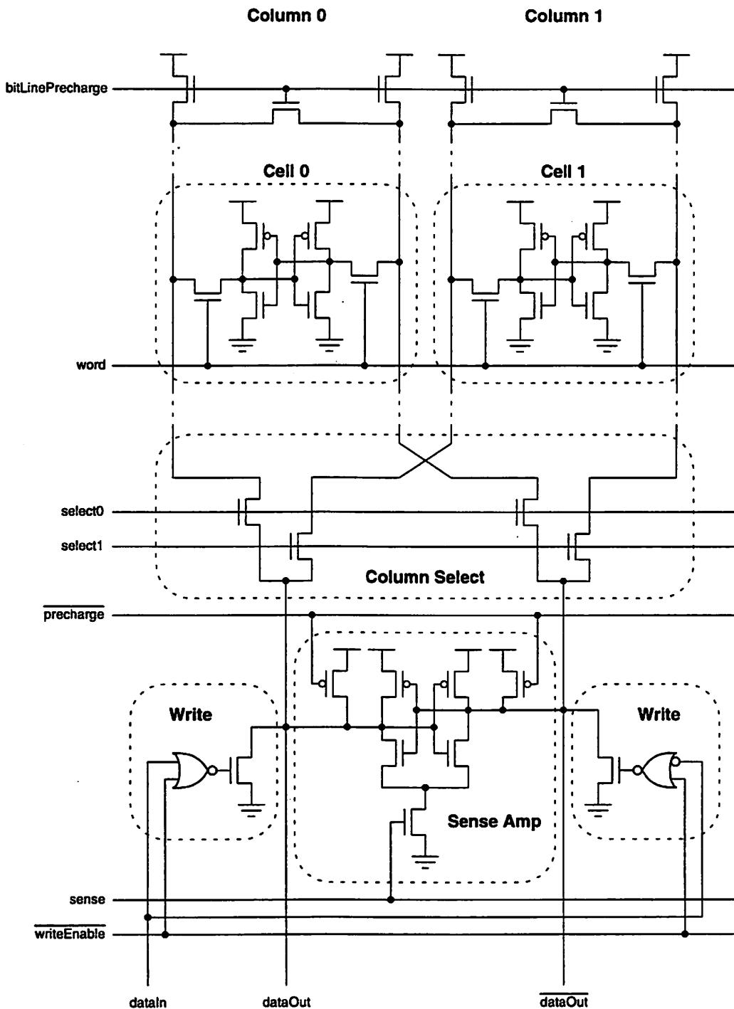
**Figure 6.9: Bit-Line Structure of the P1 SRAMs**
