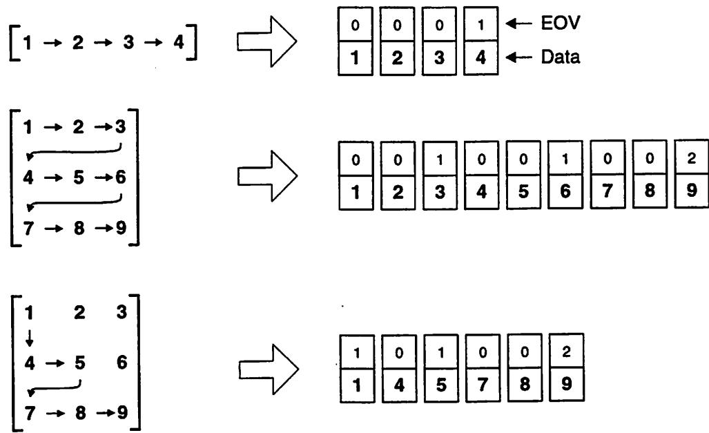
**Figure 5.13: Data Stream Examples for Accessing Vectors and Matrices**
