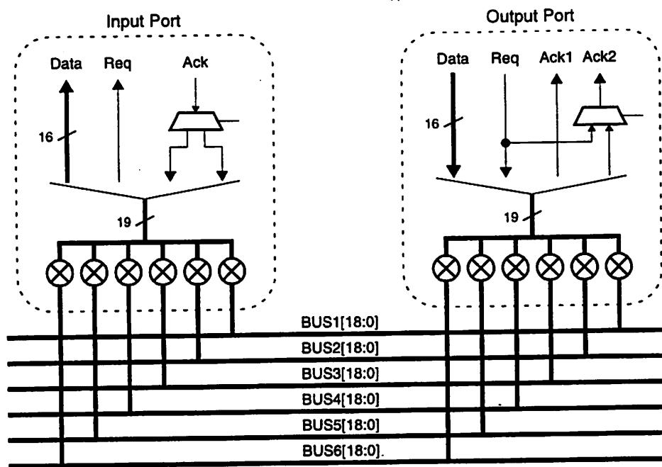
**Figure 6.6: Port Structure of the Satellite Processors**
