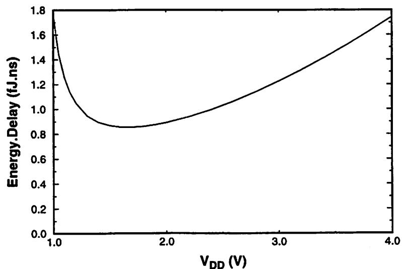
**Figure 6.3: Energy-Delay Product vs. Supply Voltage**
