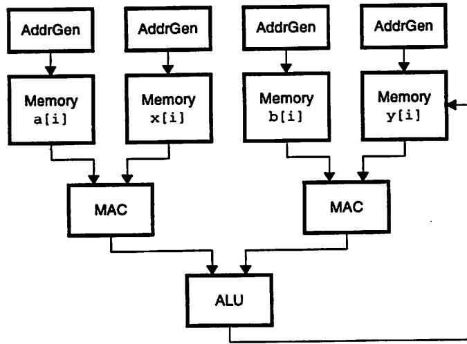
**Figure 7.1: Pleiades Mapping for the IIR Kernel**
