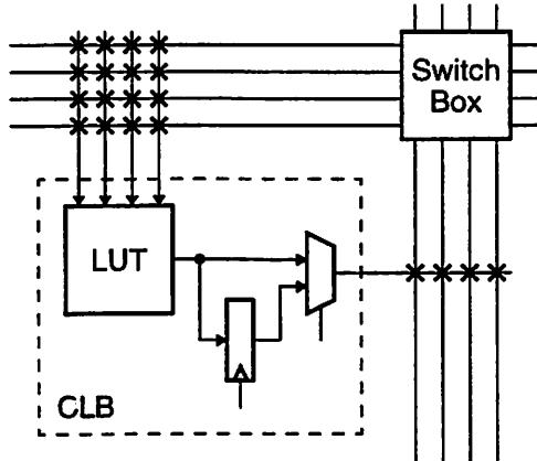
**Figure 4.9: Basic CLB + Switch Matrix Tile of an FPGA**
