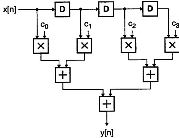
**Figure 4.2: Custom Implementation of a 4-Tap FIR Filter**
