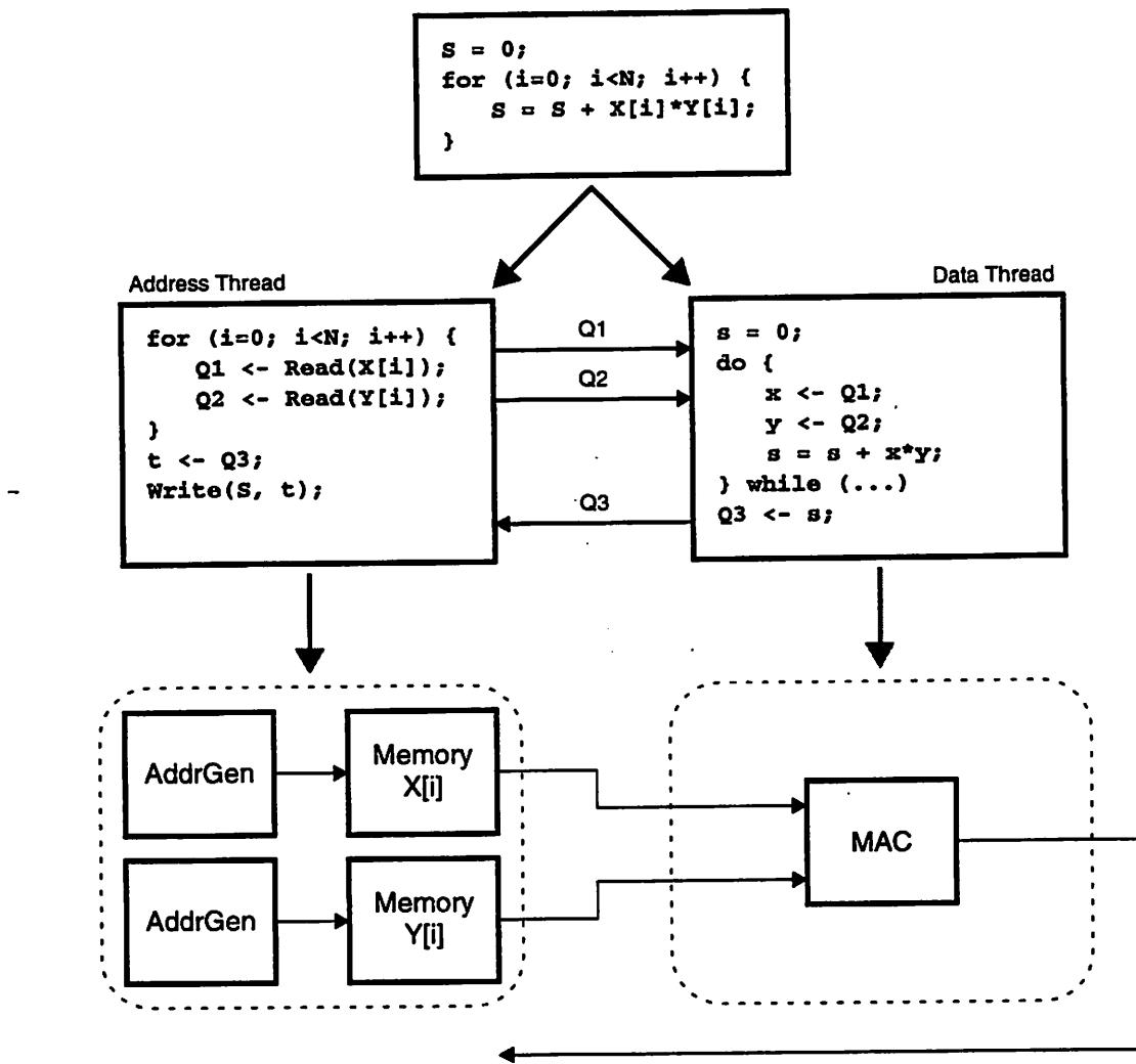
Figure 5.12: Address and Data Threads for Computing Vector Dot Product
