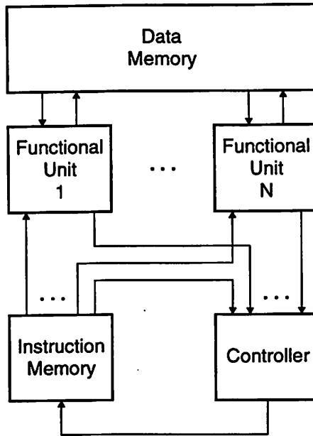
**Figure 4.5: Basic Architectural Model for Superscalar and VLIW Processors**
