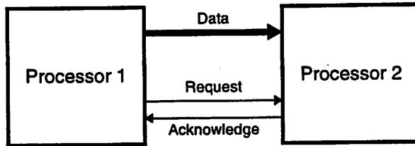
**Figure 5.11: Data-Driven Execution via Handshaking**
