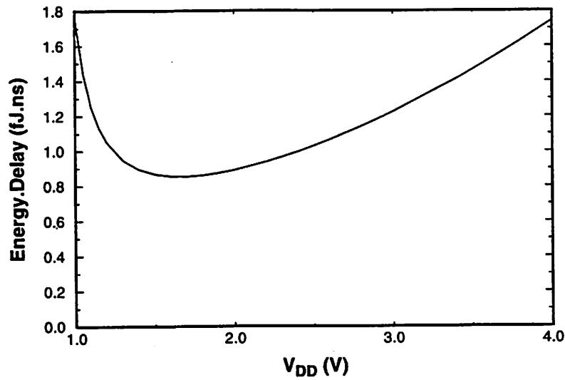
**Figure 2.5: Energy-Delay Product vs. Supply Voltage**
