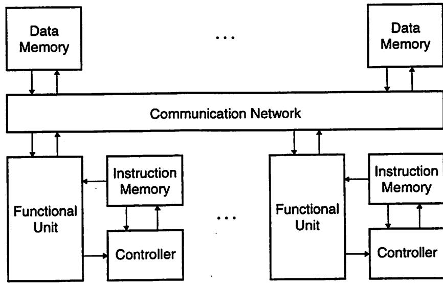
**Figure 4.8: Basic Architectural Model for MIMD Processors**
