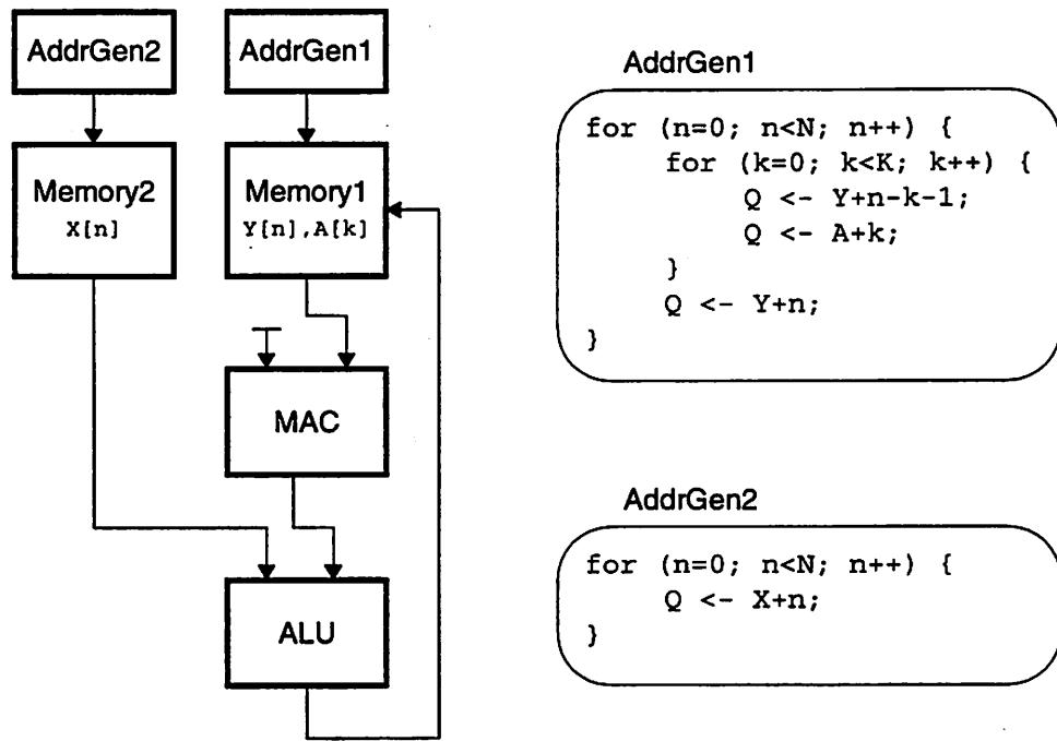
**Figure 5.31: A Mapping for the VSELP Synthesis Filter**
