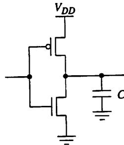
**Figure 2.1: CMOS Inverter**
