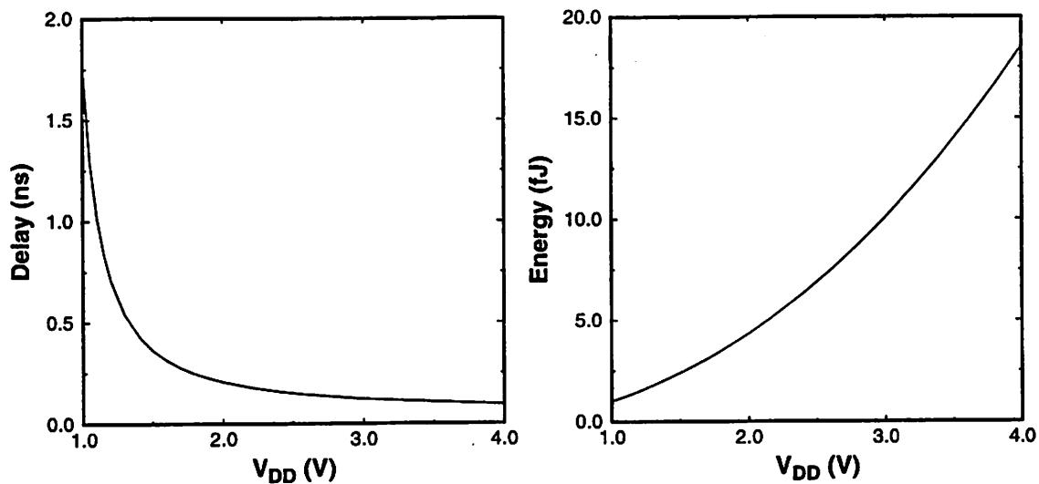
**Figure 2.4: Dependence of Delay and Power on Supply Voltage**
