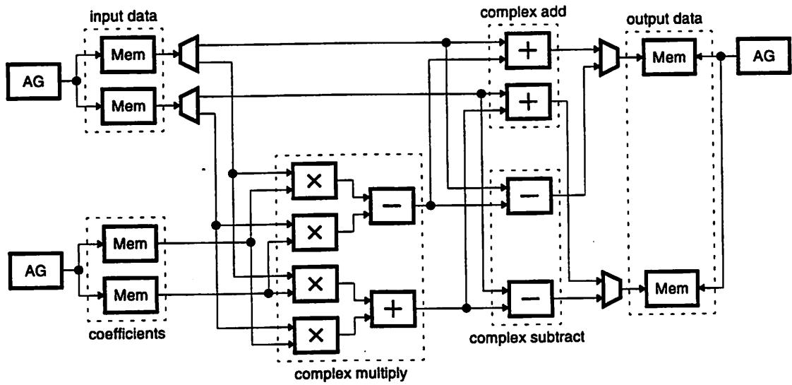
**Figure 7.2: Pleiades Mapping for the FFT Kernel**
