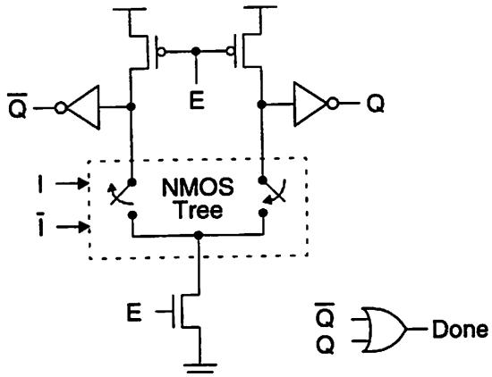
**Figure 5.15: Completion Signal Generation in Asynchronous CMOS Circuits**
