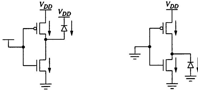
**Figure 2.2: Leakage Currents in a CMOS Inverter**
