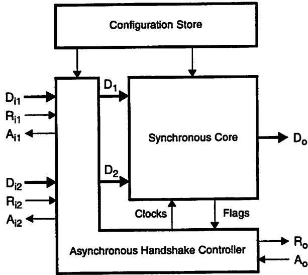
**Figure 5.16: General Structure of a Satellite Processor**
