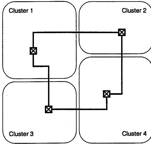
**Figure 5.9: Hierarchical Generalized Mesh Interconnect Structure**
