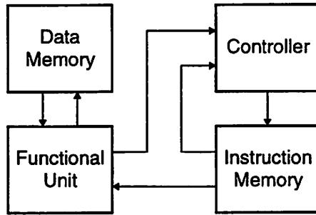
**Figure 4.3: Basic Architectural Model of a General-Purpose Processor**
