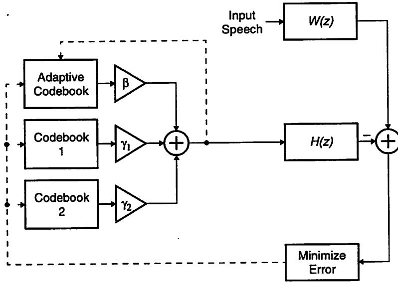
**Figure 3.9: Basic Structure of the VSELP Coder**
