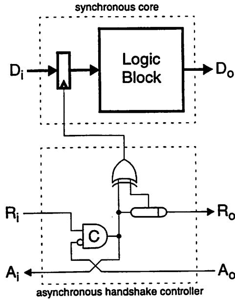
**Figure 5.19: Example of a Handshake Controller**
