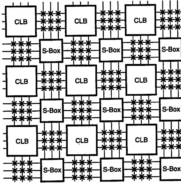
**Figure 5.7: Simple FPGA Mesh Interconnect Structure**
