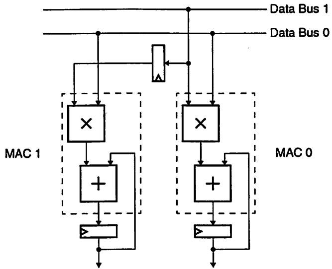
**Figure 4.4: Dual-MAC Structure of the TCSI LODE Processor**
