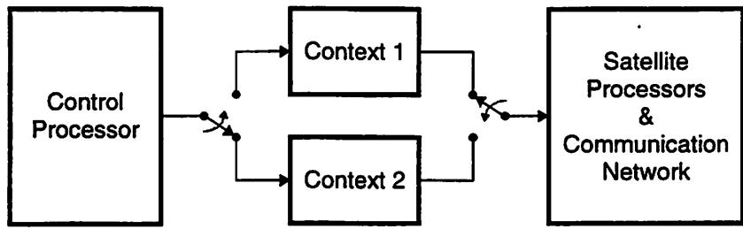
**Figure 5.10: Concurrent Reconfiguration and Kernel Execution**
