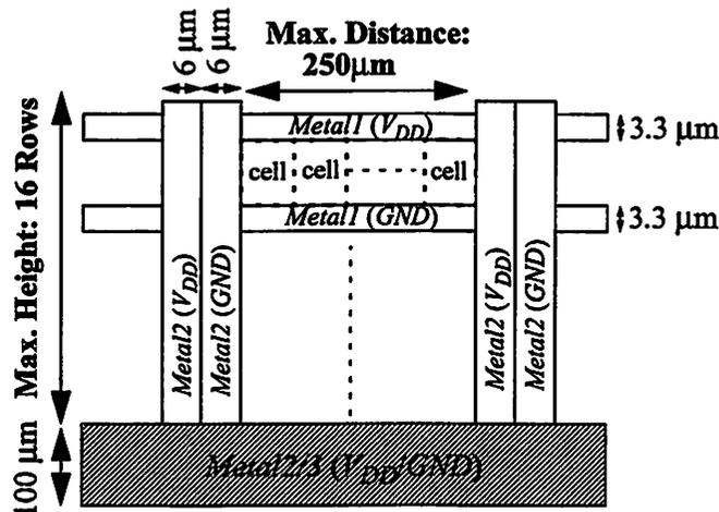
FIGURE 4.16 : Local Standard Cell Power Routing.
