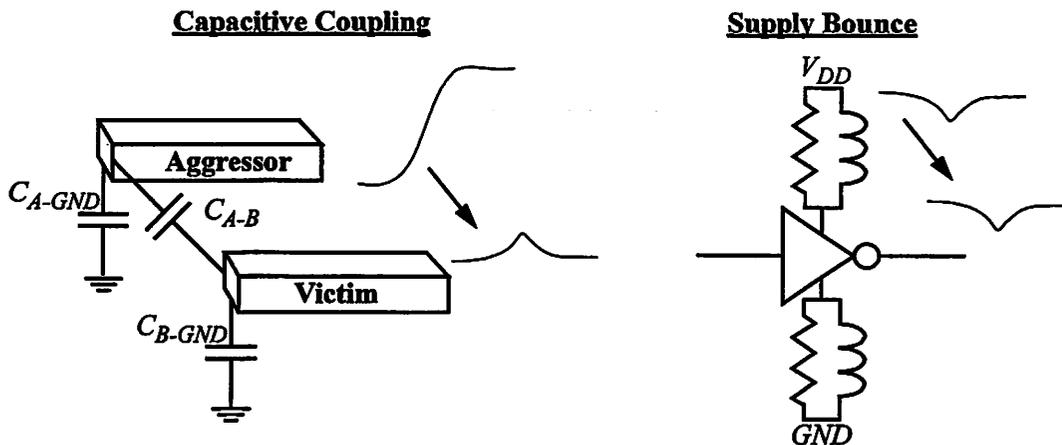
FIGURE 3.12 : Noise Margin Degradation.
