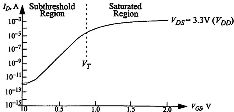
**FIGURE 2.6 :  $I_D$  vs.  $V_{GS}$  for MOSFET in Subthreshold Region.**
