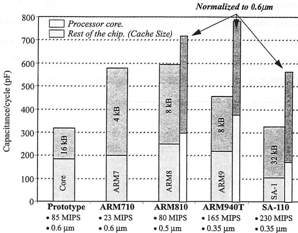
**FIGURE 7.50 : Capacitance/cycle of Various ARM Microprocessors.**
