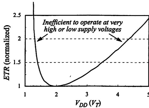
FIGURE 2.9 : *ETR* as a function of  $V_{DD}$ .
