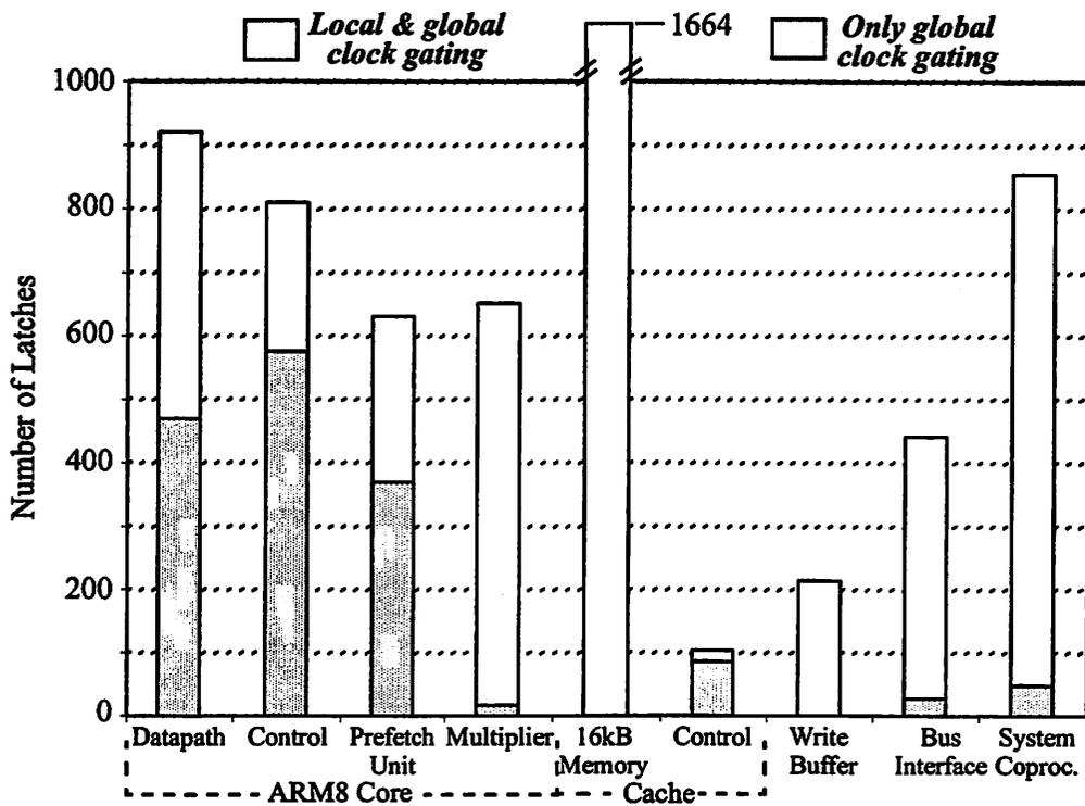
FIGURE 6.5 : Latches in the Prototype Microprocessor
