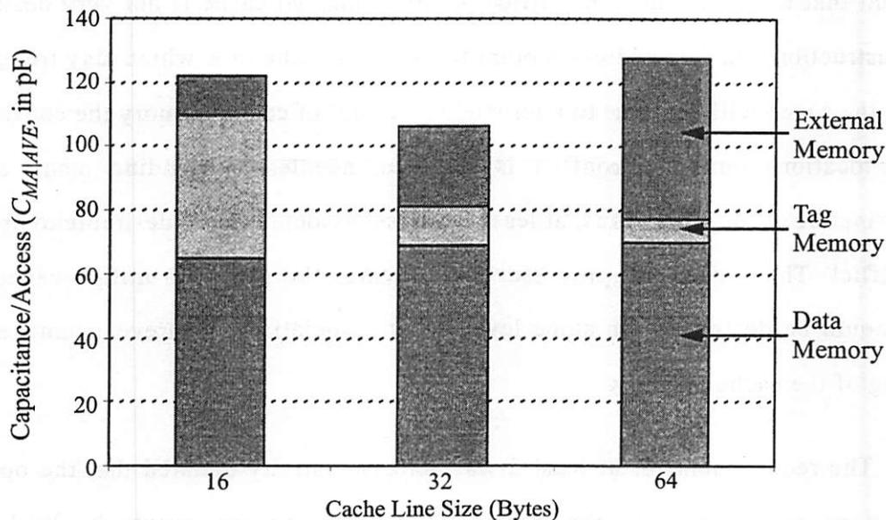
**FIGURE 5.10 : Average Capacitance/Access versus Cache Line Size (0.6 $\mu$ m CMOS).**
