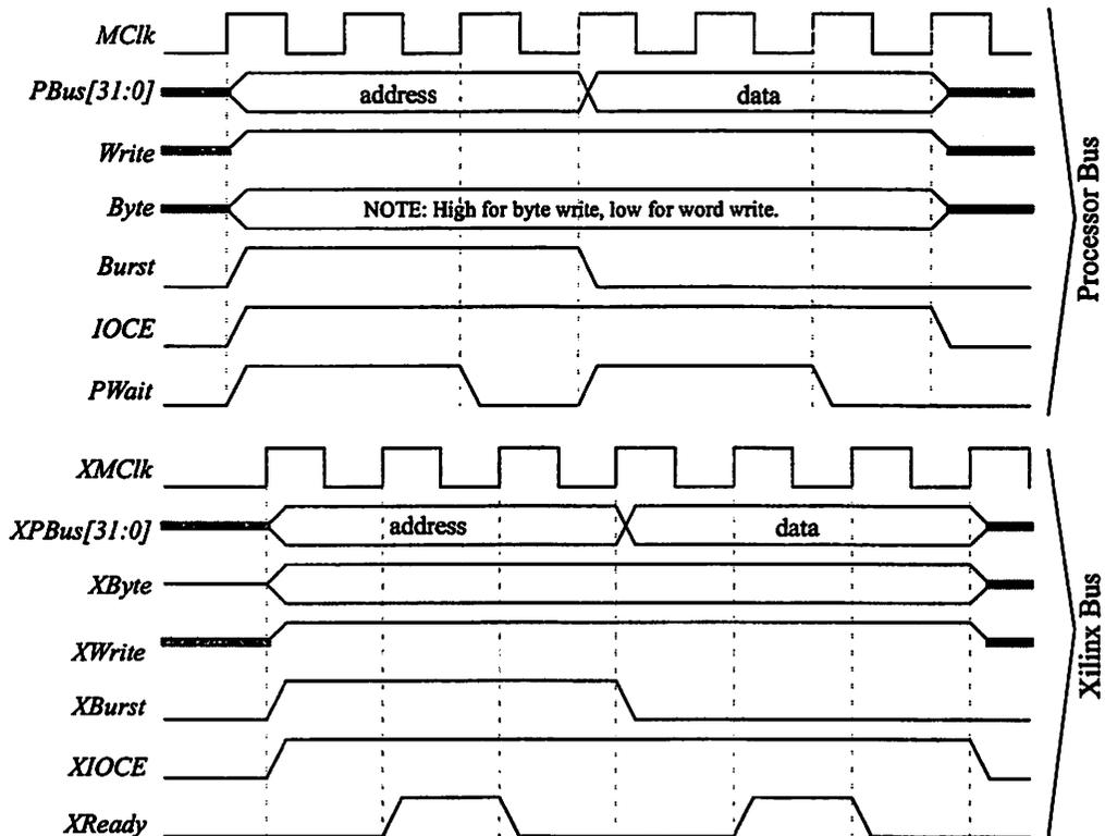
**FIGURE 7.37 : Timing Diagram for a Single I/O Write Request to the Interface Chip.**
