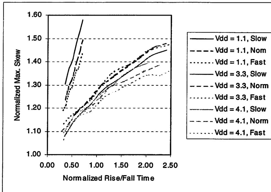
FIGURE 4.13 : Skew as a Function of Enable Rise/Fall Time.
