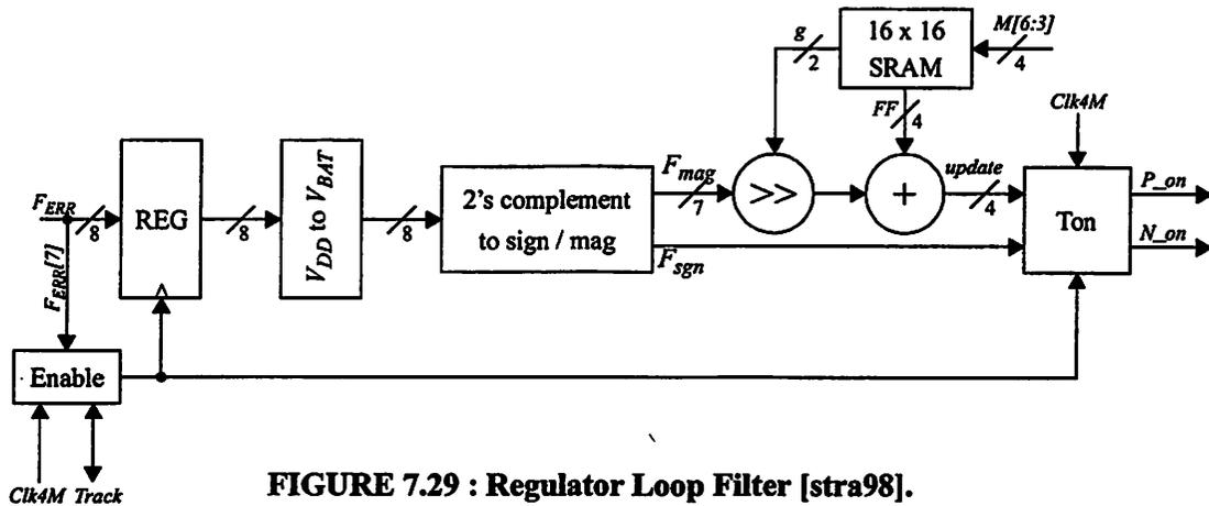
FIGURE 7.29 : Regulator Loop Filter [stra98].
