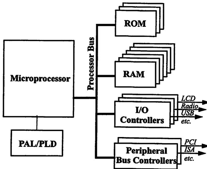
**FIGURE 5.1 : Generic Microprocessor System Architecture.**
