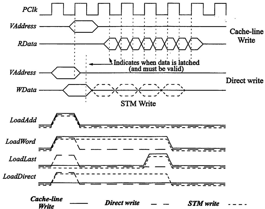
FIGURE 7.20 : Write Buffer Timing.
