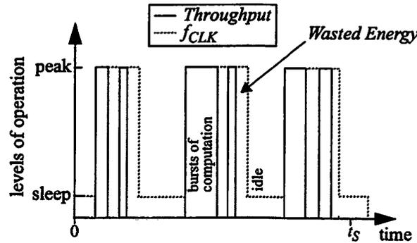
**FIGURE 2.11 : Wasted energy due to idle**
