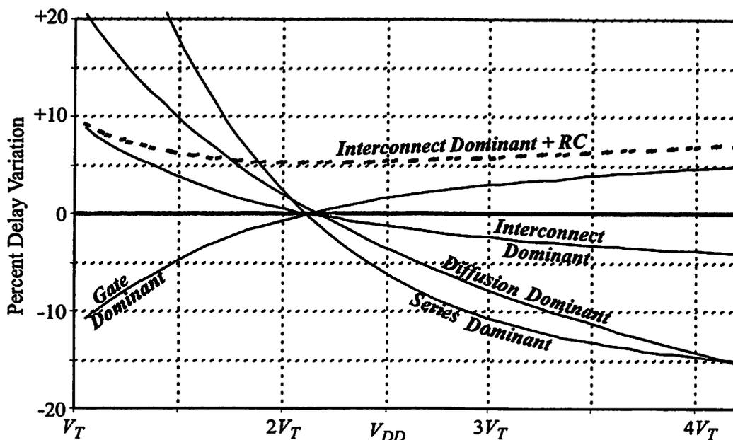
FIGURE 3.11 : Relative CMOS Circuit Delay Variation over Supply Voltage.
