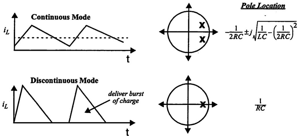
**FIGURE 3.8 : Reducing the Buck Converter to a One Pole System**
