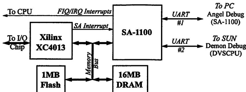
FIGURE 7.43 : StrongArm Board Architecture.
