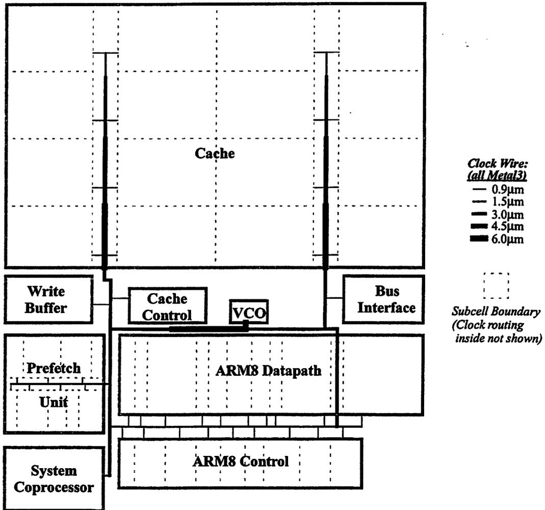
FIGURE 4.12 : Prototype Processor IC Clock Distribution Network (Top Level).
