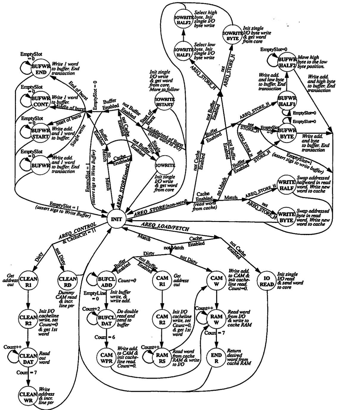
FIGURE 7.15 : Cache Controller State Diagram.
