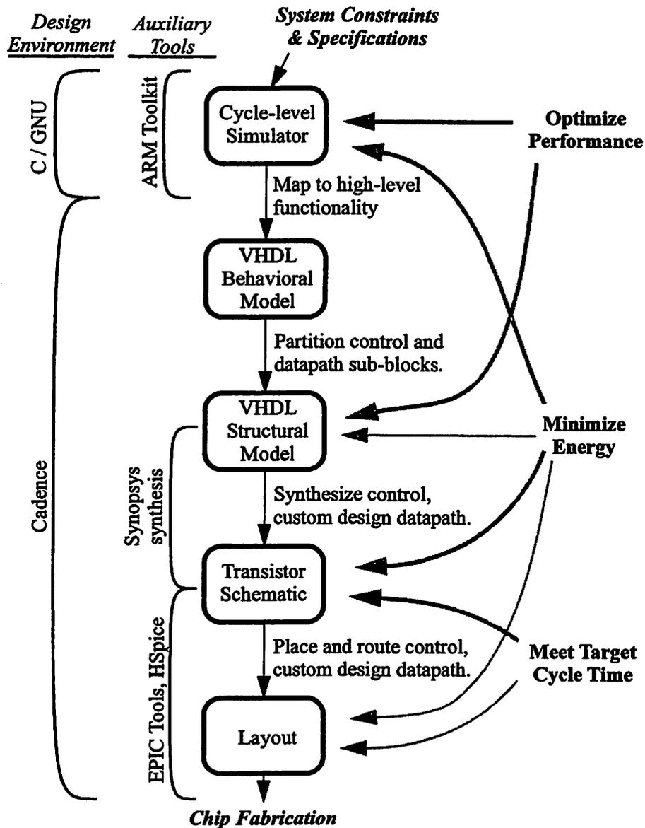
FIGURE 4.1 : General Design Flow from Specification to Layout.
