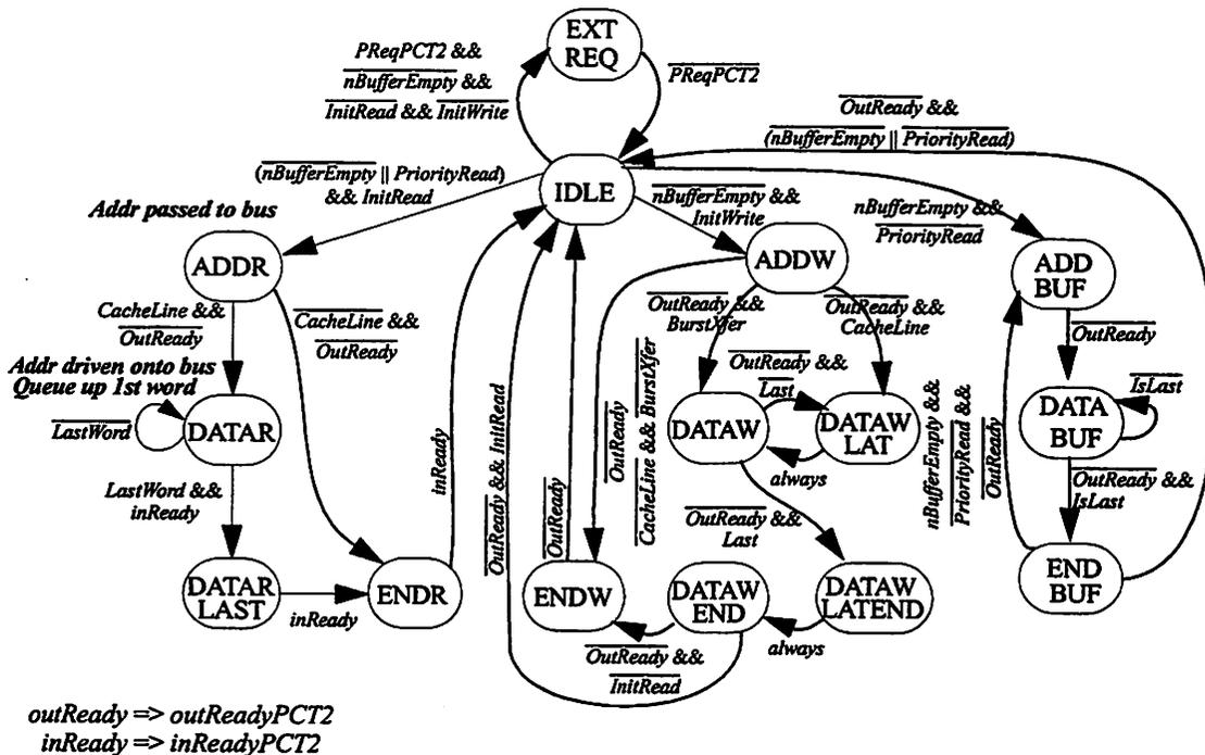
FIGURE 7.22 : Bus Interface State Machine.
