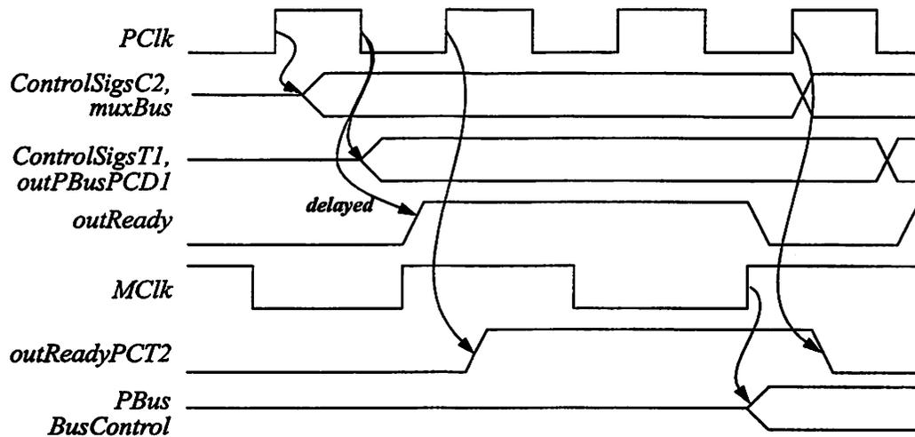
FIGURE 7.23 : Core-side to Bus-side Timing.
