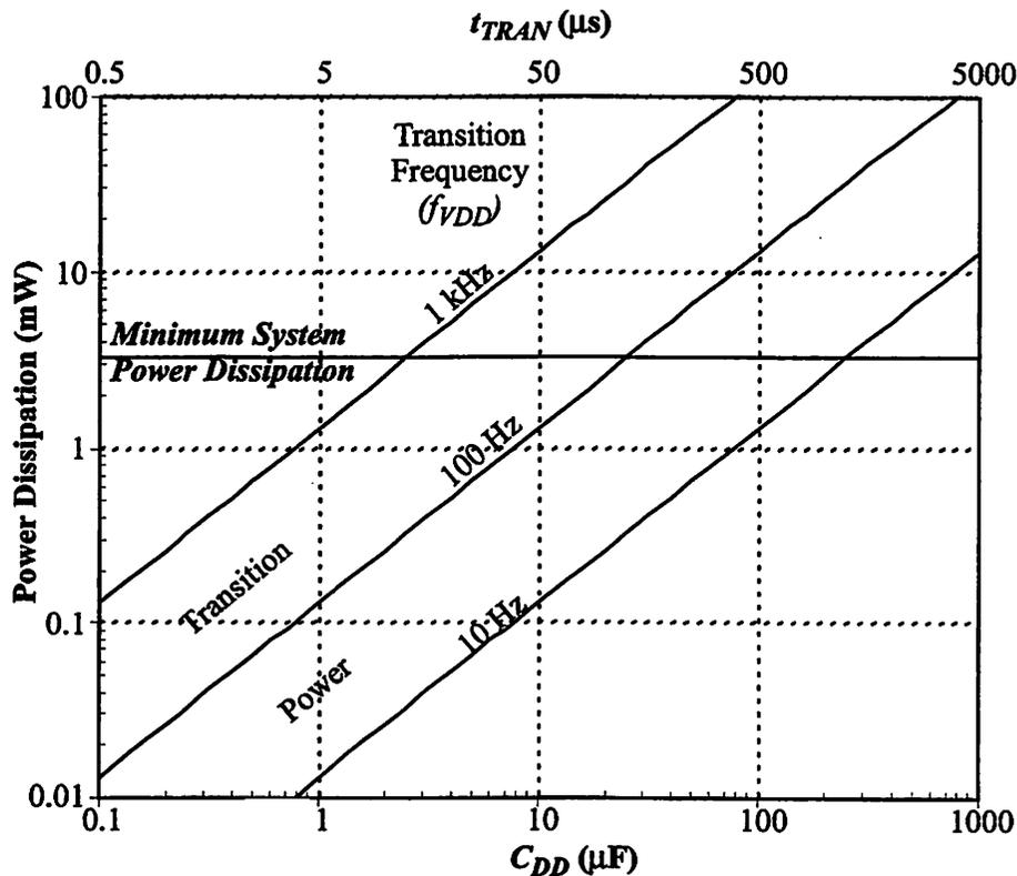
**FIGURE 3.9 : Transition Time and Power Dissipation vs.  $C_{DD}$ .**
