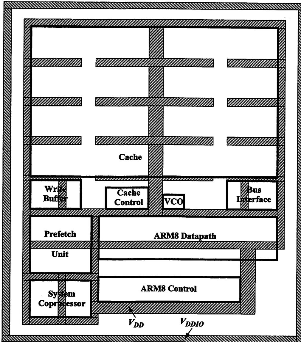
FIGURE 4.14 : Prototype Processor IC Power Distribution Network.
