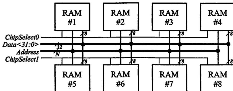
**FIGURE 5.4 : Typical Main Memory Architecture.**
