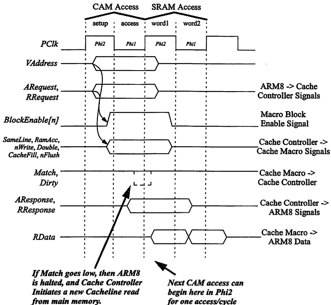
**FIGURE 7.16 : Cache Memory Timing for a Cache Double-Read Hit.**
