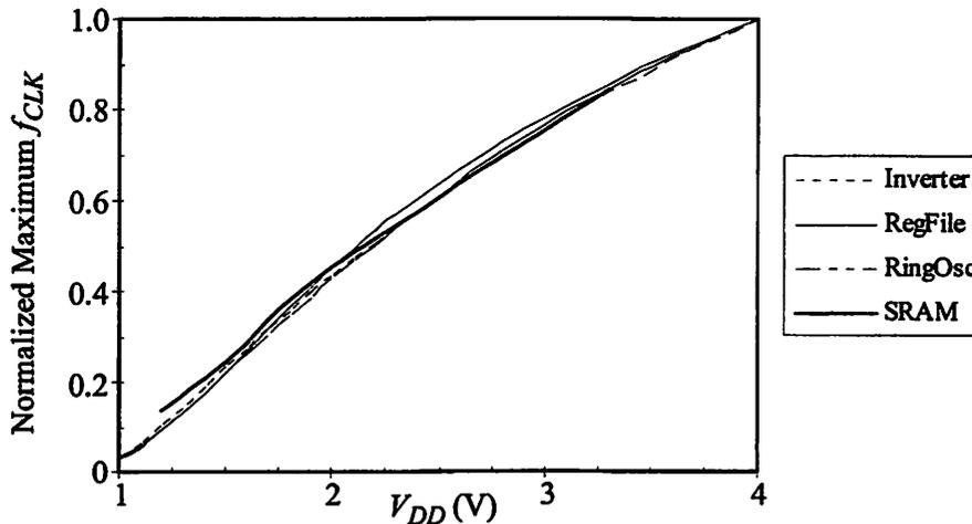
FIGURE 3.1 : Various Circuit Delays vs. Supply Voltage
