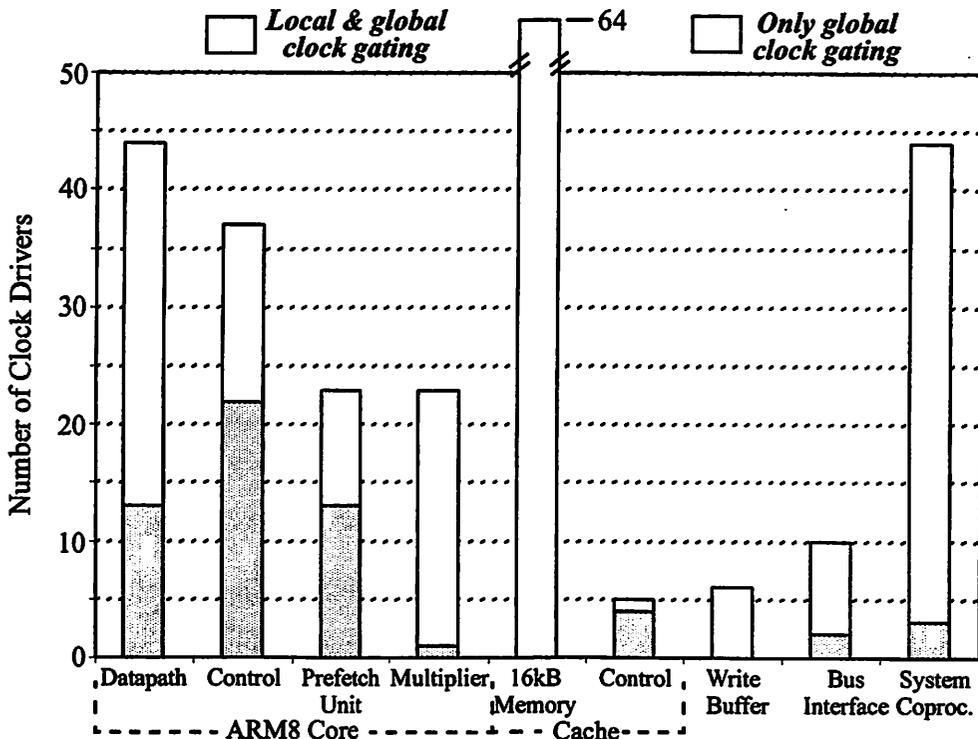
FIGURE 6.4 : Clock Drivers in the Prototype Microprocessor
