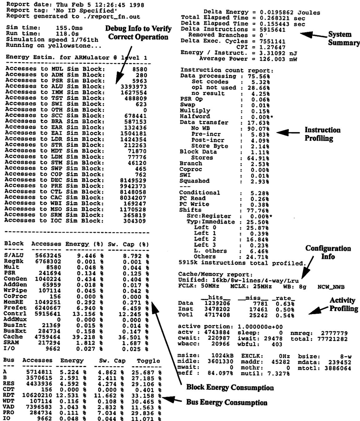
FIGURE 4.4 : Simulator Report File for Crypto Benchmark.
