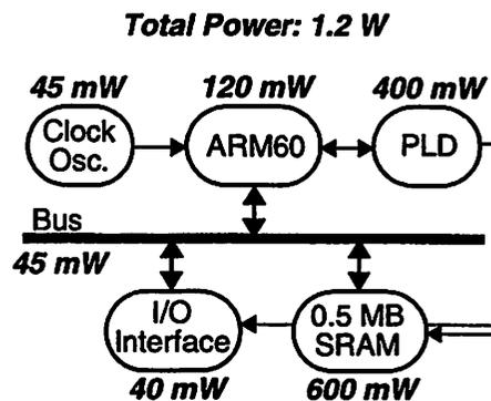
**FIGURE 2.2 : InfoPad Processor Subsystem.**
