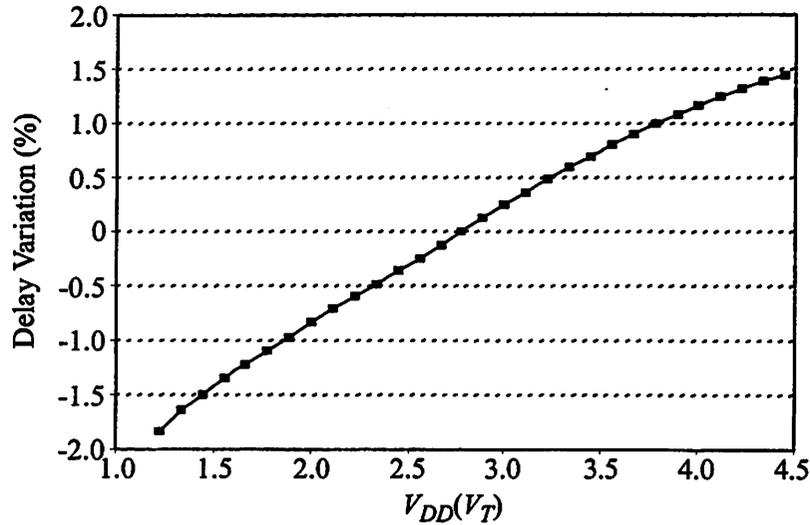
**FIGURE 6.11** : Relative Delay from  $Word$  to  $V_{out}$  vs. Static CMOS logic for Constant  $V_{DD}$ .
