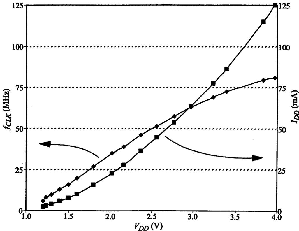
FIGURE 7.45 : Measured Clock Frequency and Supply Current vs. Supply Voltage.
