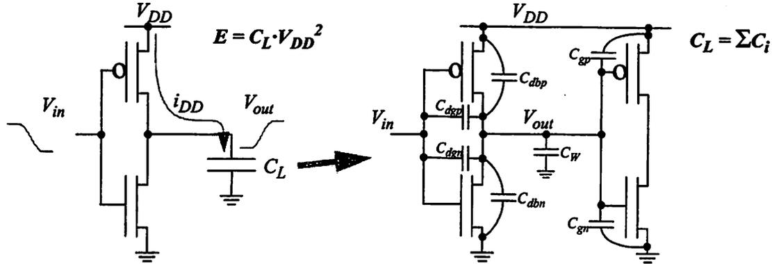
FIGURE 2.3 : Dynamic Switching Power Dissipation; Sources of Capacitance.
