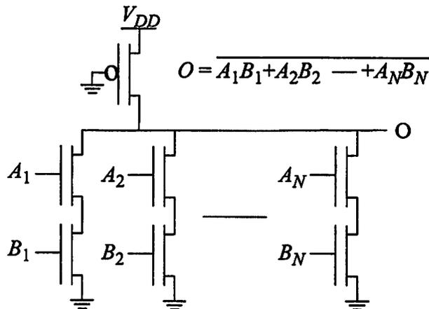
**FIGURE 2.7 : Implementing Complex Logic with Static Biasing (pseudo-NMOS)**
