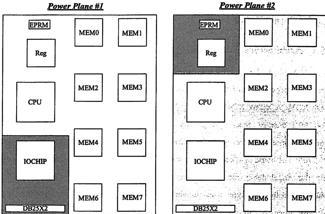
FIGURE 7.42 : Prototype Board Power Planes.
