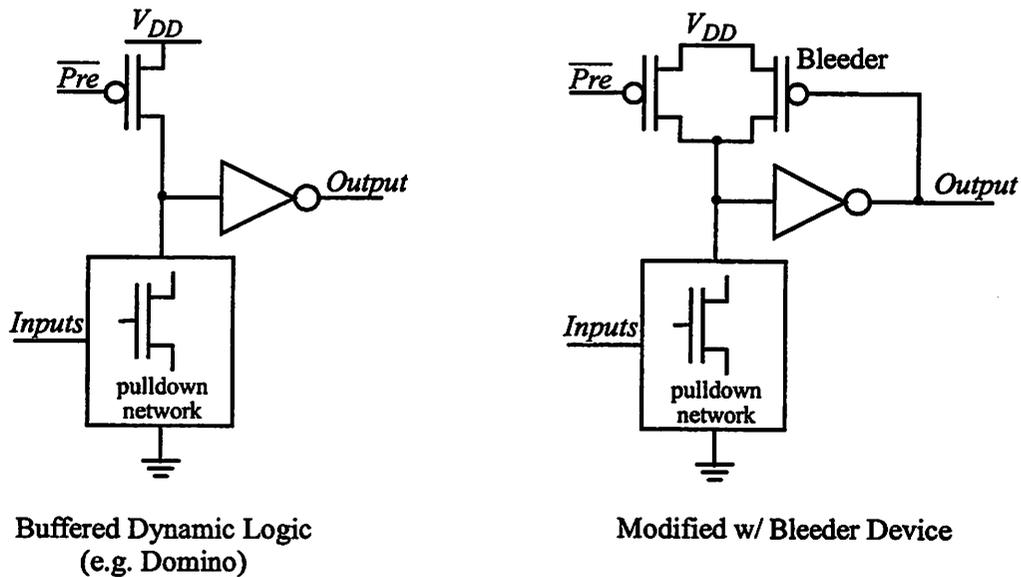
FIGURE 6.1 : Bleeder Circuit for Dynamic Logic.
