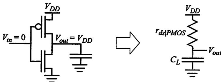
**FIGURE 3.16 : Equivalent RC Network for Static CMOS Inverter.**
