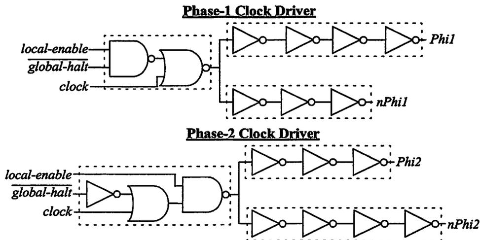
FIGURE 4.9 : Modular Clock Driver Design.
