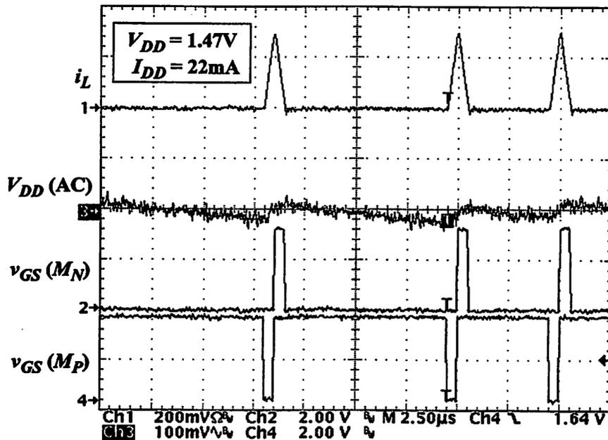
FIGURE 7.47 : Converter Waveforms in Regulation Mode [stra98].
