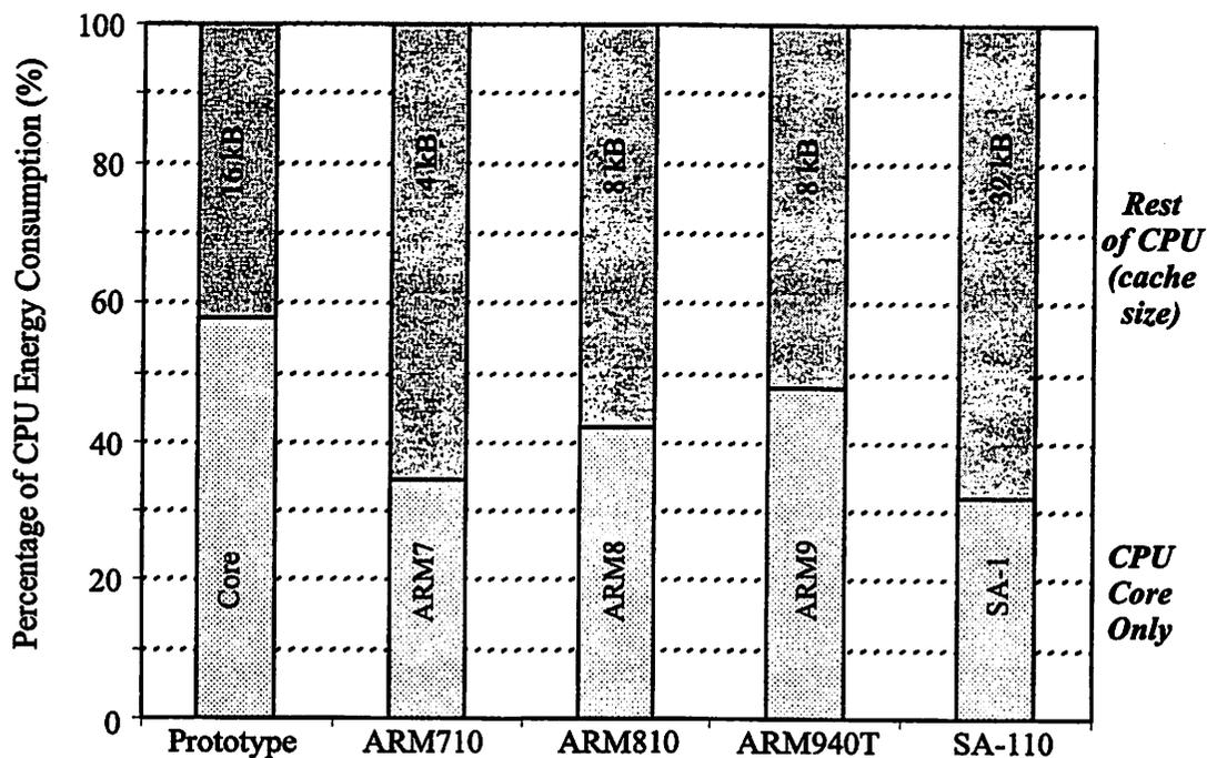
**FIGURE 5.15 : Energy Breakdown of Various ARM Microprocessors.**
