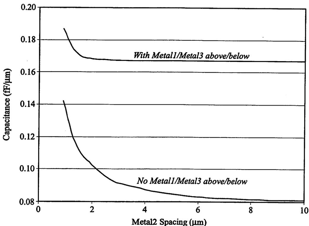
**FIGURE 6.7 : *Metal2* Wire Capacitance/ $\mu\text{m}$  With Adjacent *Metal2* Wires.**
