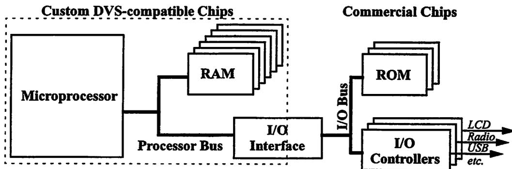
**FIGURE 5.2 : Prototype System Architecture Incorporating DVS.**
