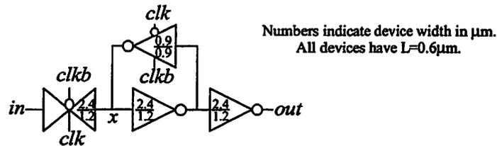
**FIGURE 4.7 : Basic Two-phase Latch Design.**
