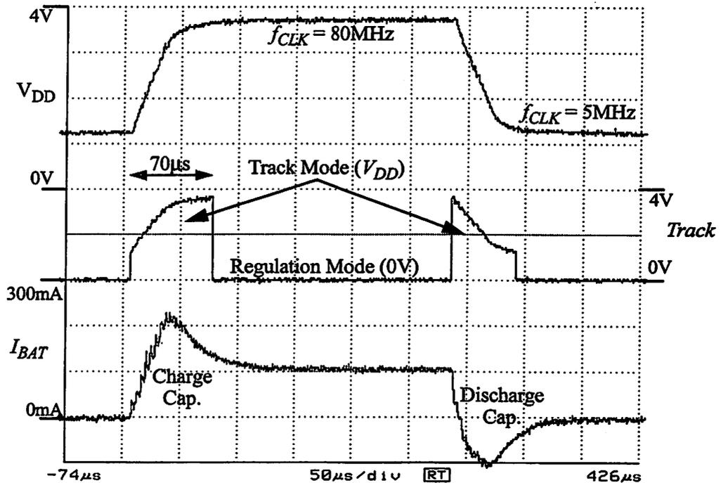
FIGURE 7.46 : Transient Response of the Converter Loop.
