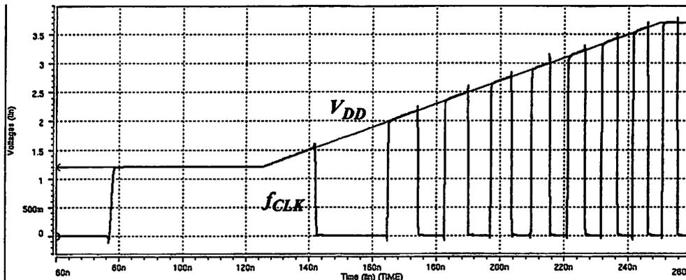
FIGURE 3.17 : Ring Oscillator Transient Performance.
