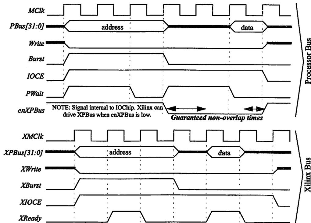
**FIGURE 7.38 : Timing Diagram for a Single I/O Read Request to the Interface Chip.**
