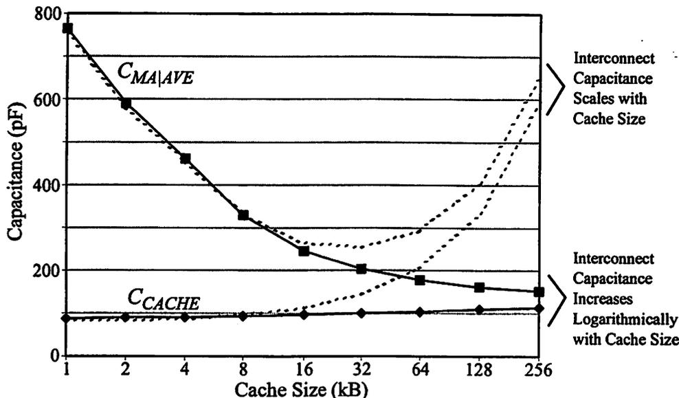
FIGURE 5.7 : Average and Cache Capacitance/access versus Cache Size (0.6 $\mu$ m CMOS).
