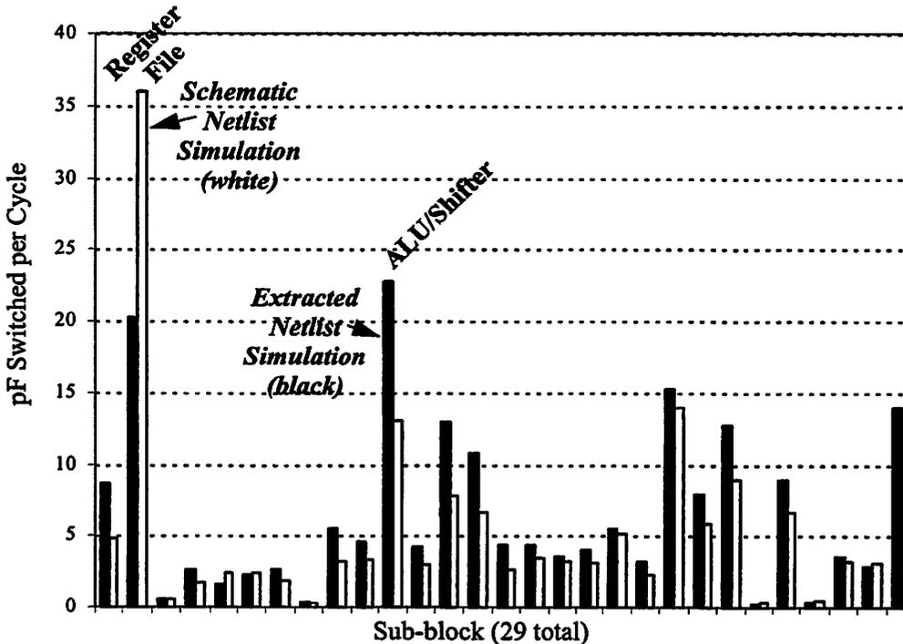
**FIGURE 7.10 : ARM8 Capacitance Comparison of Schematic vs. Extracted Simulation.**
