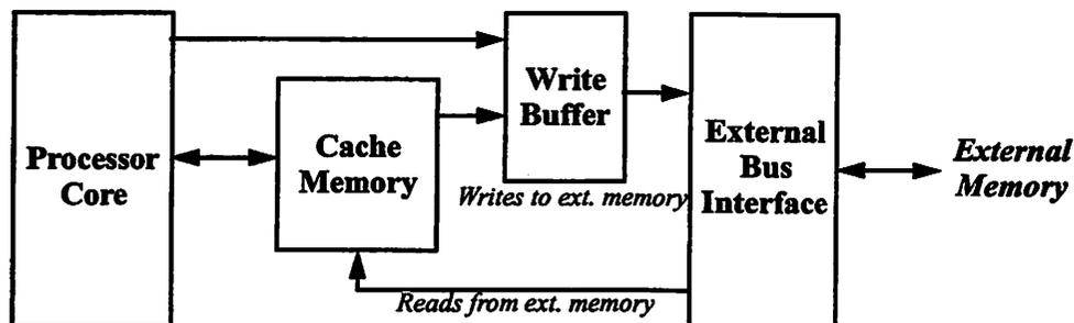
FIGURE 5.14 : Cache Architecture Utilizing a Write Buffer.
