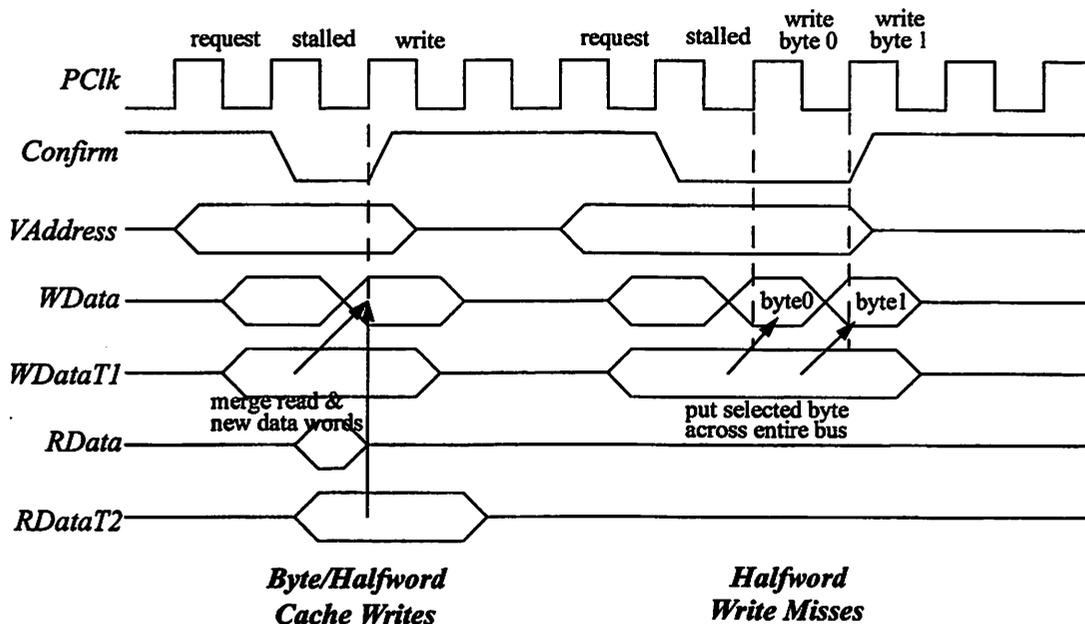
FIGURE 7.17 : Timing for Non-word Writes to the Cache and Main Memory.
