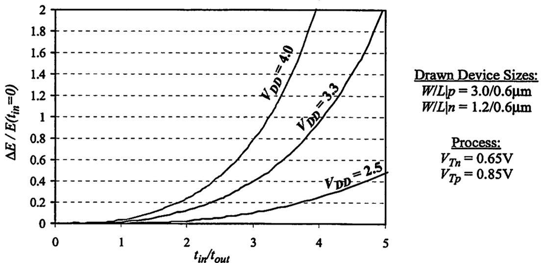
FIGURE 2.4 : Short-circuit Energy Consumption vs. Input Rise/fall Time.
