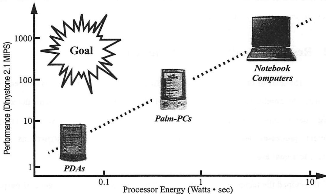
FIGURE 1.1 : Processor Performance vs. Energy Consumption.
