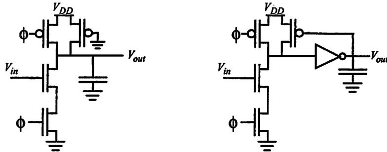
FIGURE 3.19 : Using Bleeder Devices to Improve Robustness over Varying  $V_{DD}$ .
