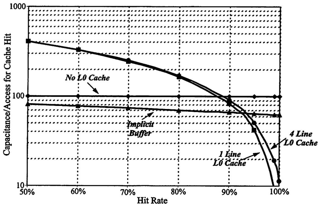
FIGURE 5.13 : Capacitance/Access of a Cache Hit for L0 Architectures (0.6µm CMOS)
