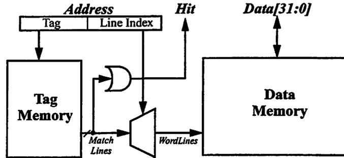
FIGURE 5.9 : Optimized CAM/RAM Cache Memory Architecture.
