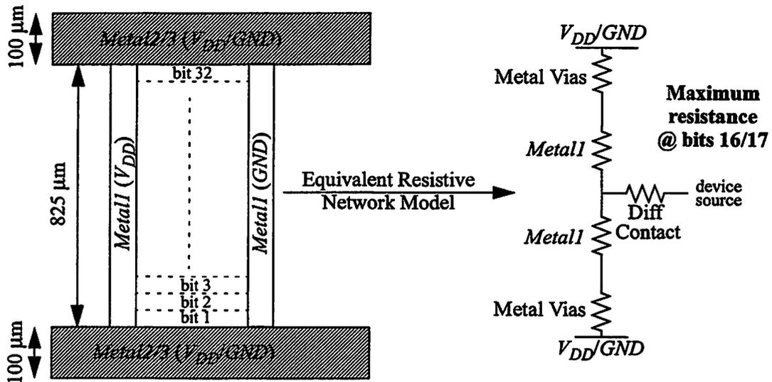
**FIGURE 4.15 : Local Datapath Power Routing.**
