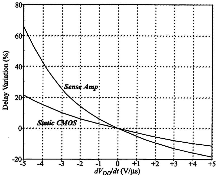
**FIGURE 3.22 : Sense-Amp Delay Variation with Varying Supply Voltage.**
