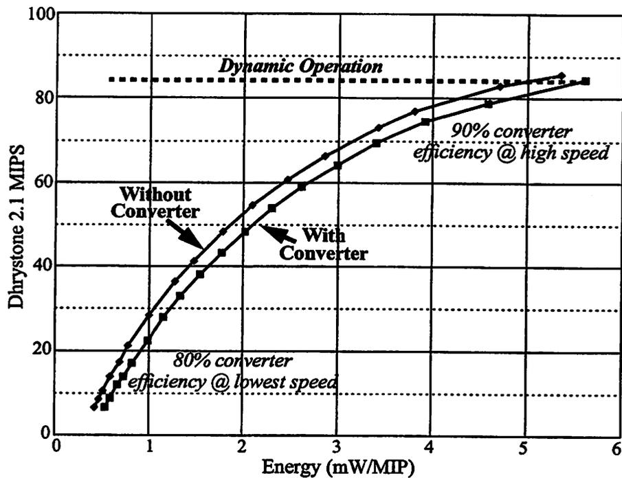
FIGURE 7.48 : Measured Throughput vs. Energy Consumption.
