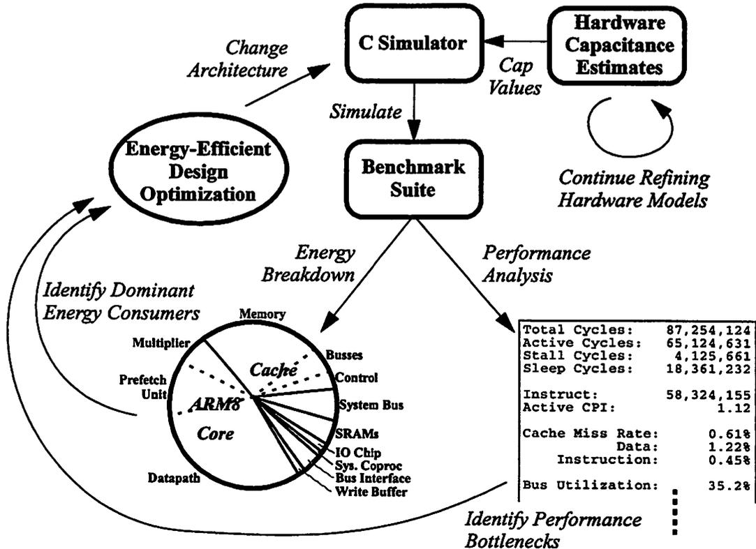
**FIGURE 4.3 : High-level Simulation Performance & Energy Estimation Methodology**
