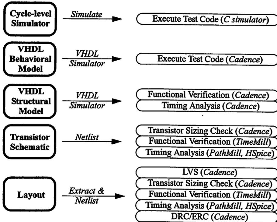
**FIGURE 4.2 : Validation Checks for Each Design Phase**
