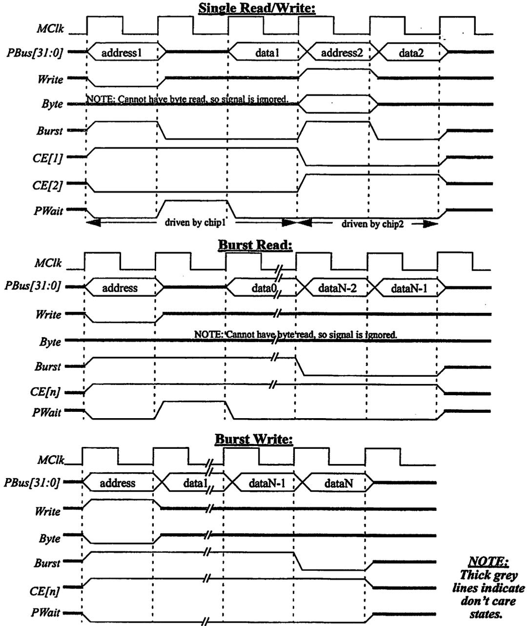
FIGURE 7.31 : Timing Diagrams for Processor Bus.
