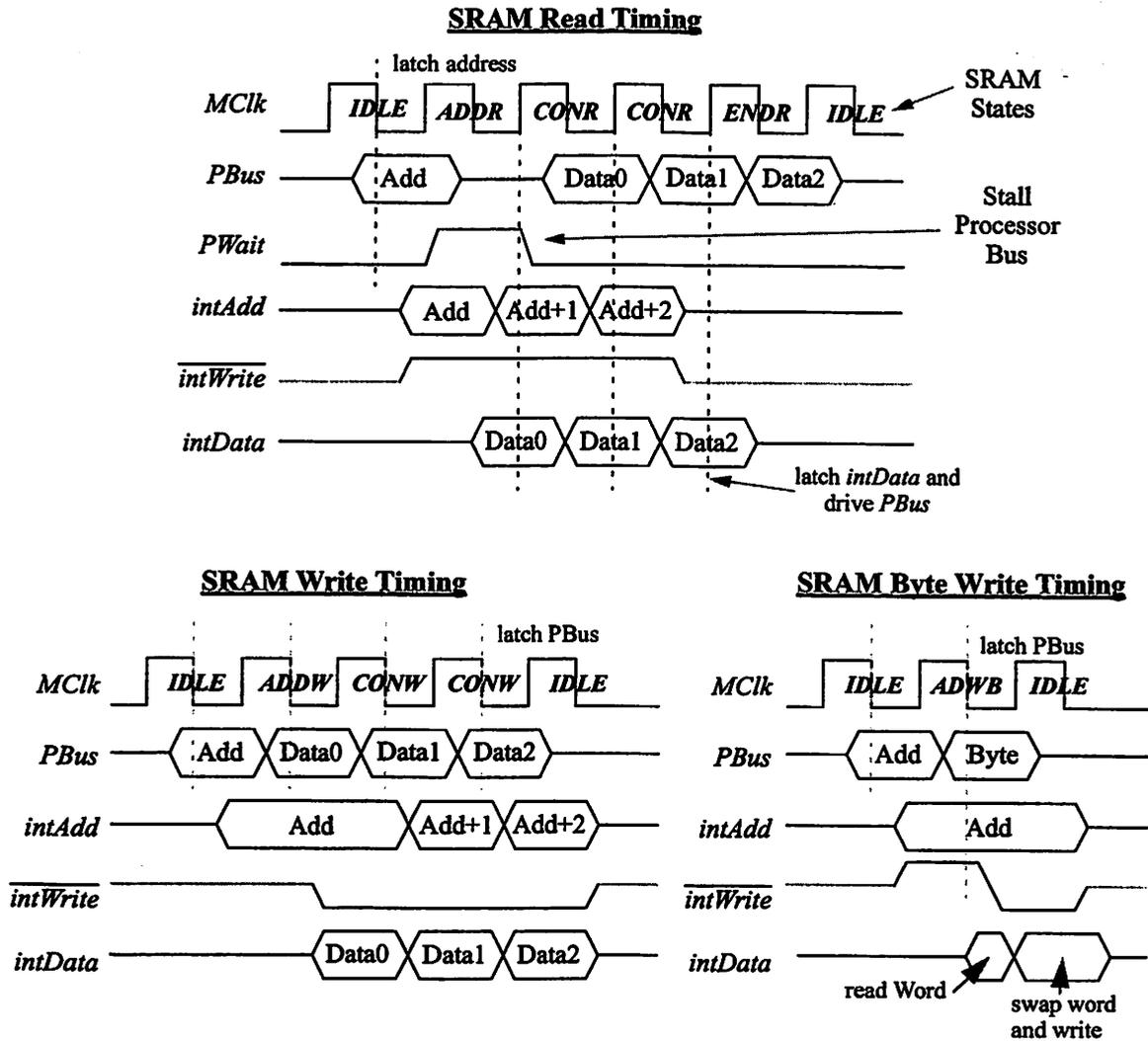
FIGURE 7.34 : Internal SRAM Timing.
