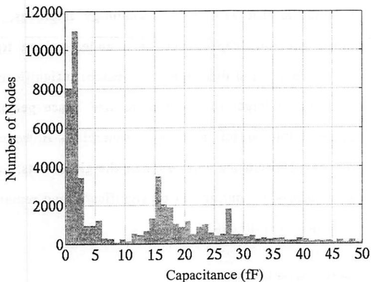
**FIGURE 6.2 : Histogram of Nodal Capacitance for ARM8 Core. (53k nodes)**
