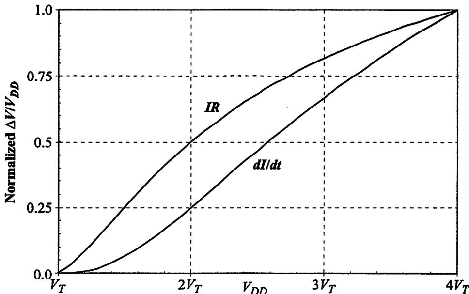
FIGURE 3.14 : Normalized Noise Margin Reduction due to Supply Bounce.
