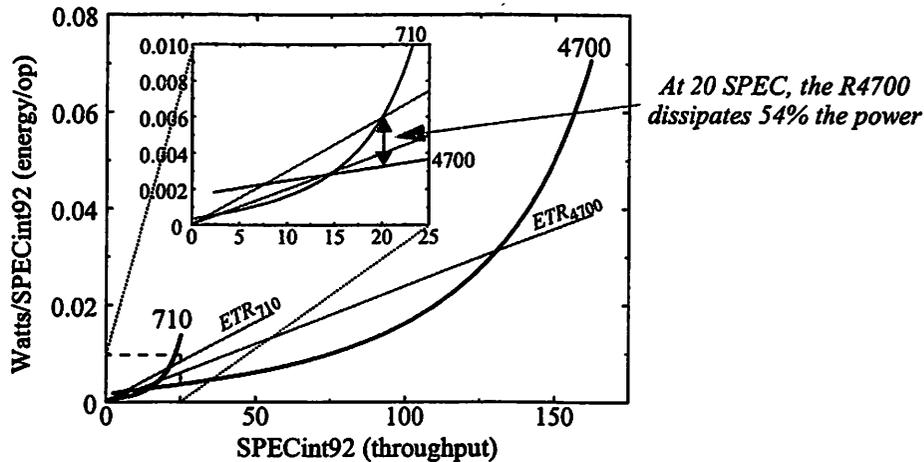
**FIGURE 2.12 : Energy vs. Throughput of R4700 and ARM710.**
