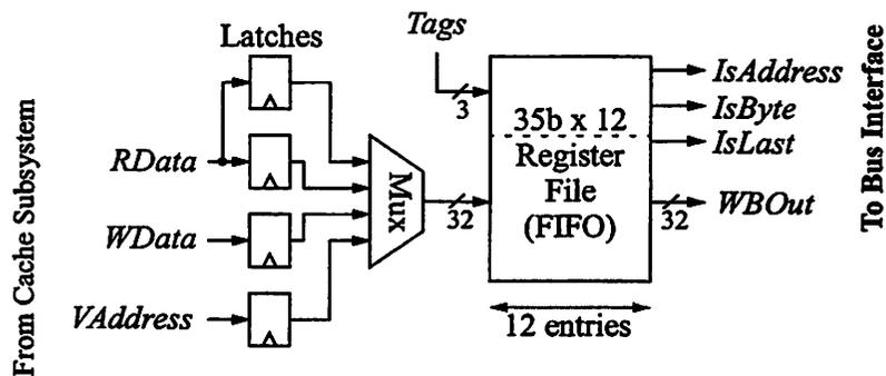
FIGURE 7.19 : Write Buffer Architecture.
