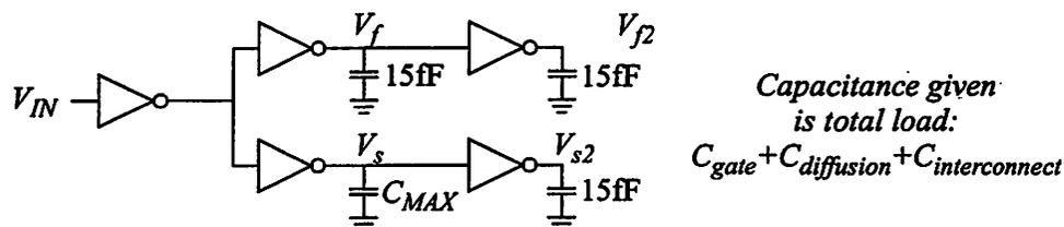
**FIGURE 6.3 : Test Circuit for Finding  $C_{MAX}$  for a 1x Gate Output Driver.**
