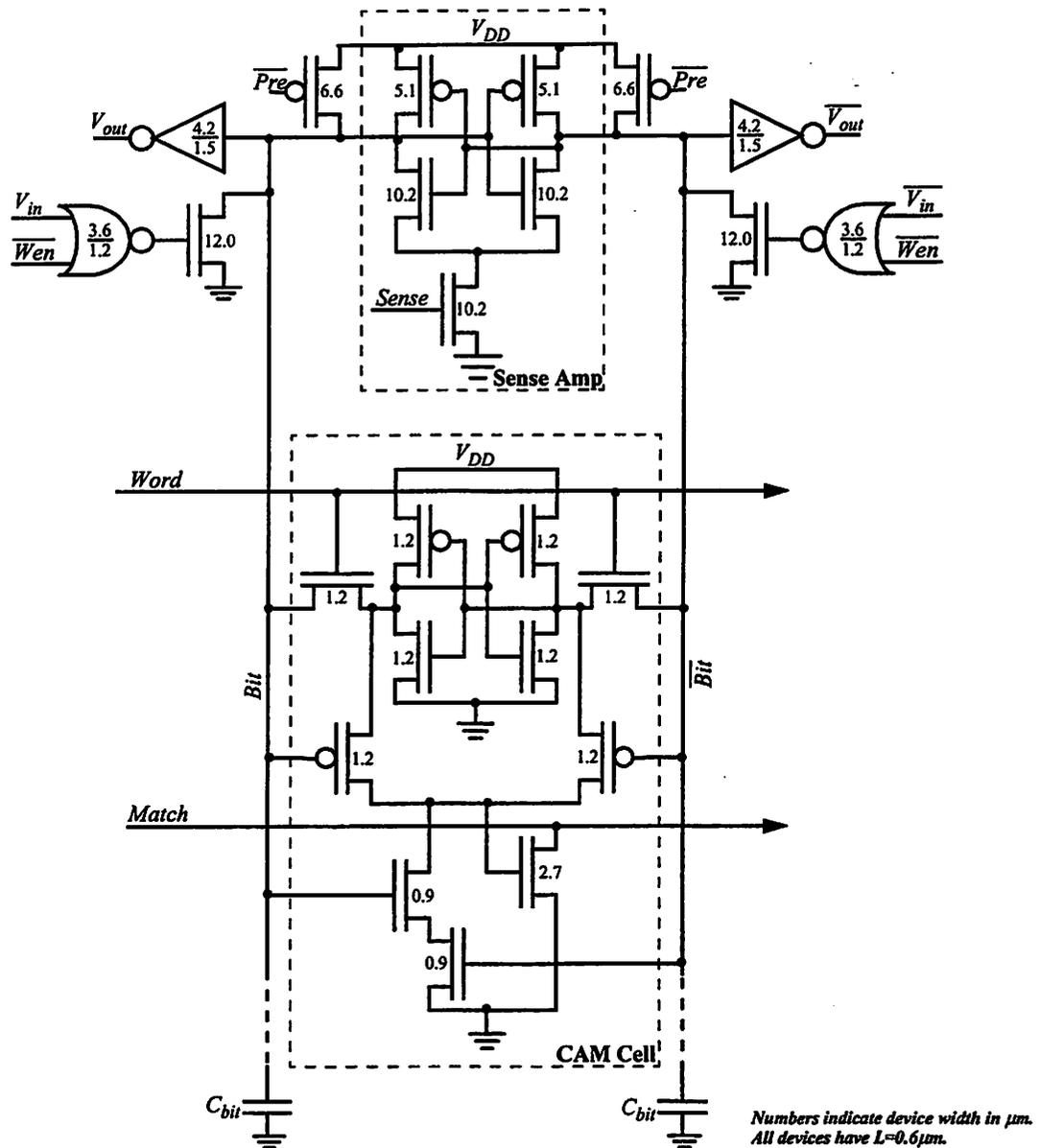
FIGURE 6.13 : CAM Cell and Sense Amp.
