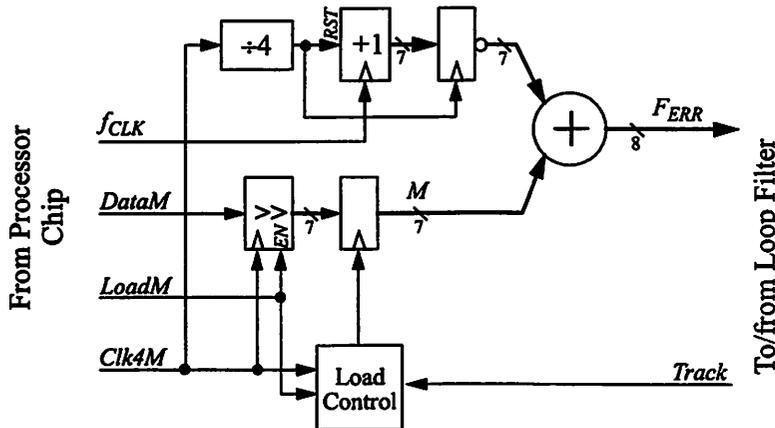
FIGURE 7.28 : Regulator Frequency Detector.
