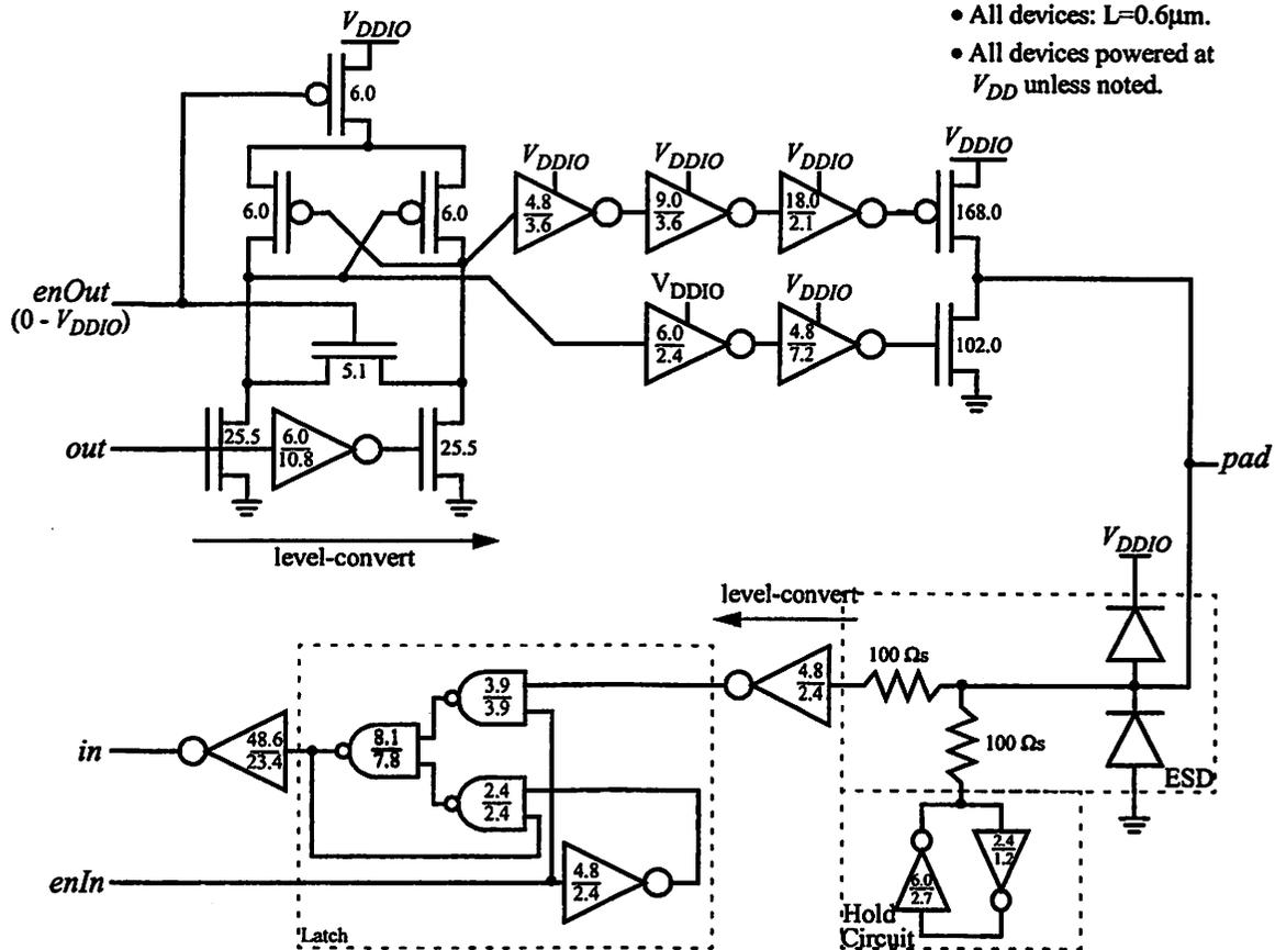
FIGURE 7.26 : Level Converting I/O Pad.
