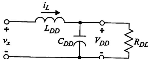
FIGURE 3.7 : Converter Loop RLC Filter.
