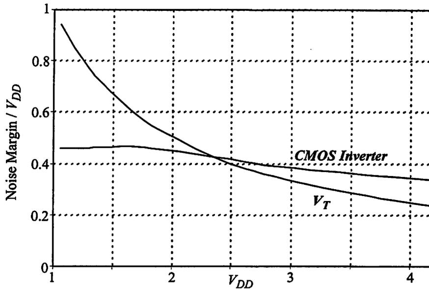
FIGURE 3.13 : Noise Margin vs. Supply Voltage.
