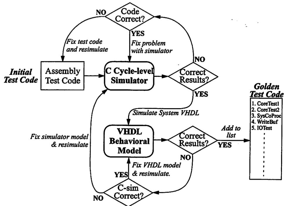
**FIGURE 4.17 : Behavioral Verification Flow for Developing Test Code Suite.**
