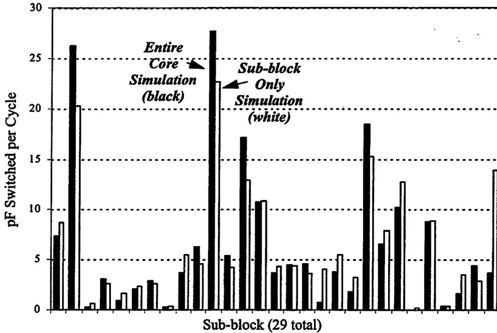
**FIGURE 7.9 : ARM8 Capacitance Comparison of Sub-block vs. Entire Core Simulation.**
