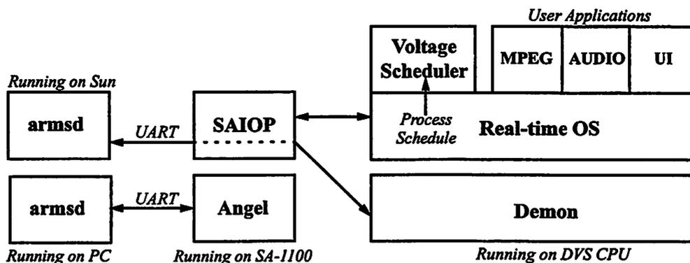
FIGURE 7.44 : Software Architecture.
