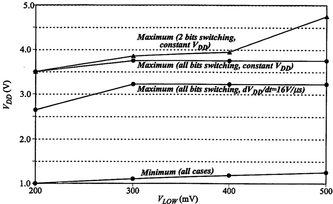
FIGURE 6.22 : Range of Operation for Low-Swing Interchip Bus.
