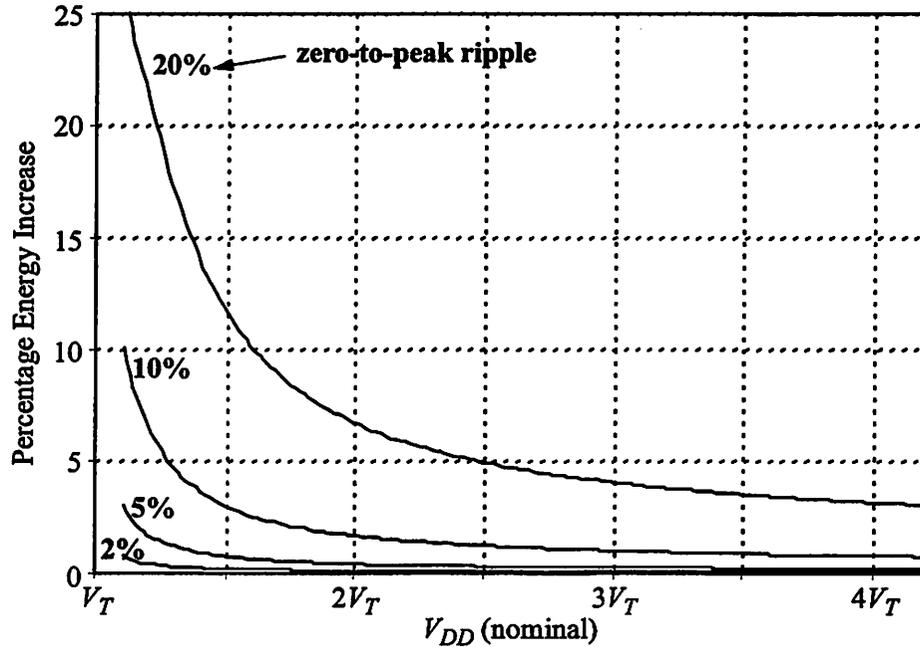
FIGURE 3.10 : Energy Loss Due to Voltage Supply Ripple.
