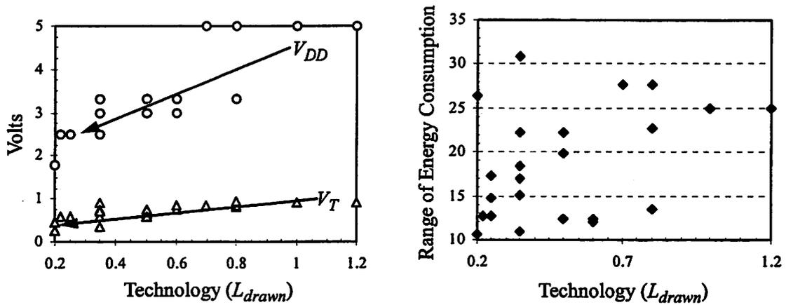
FIGURE 3.4 :  $V_{DD}$ ,  $V_T$  and Range of Energy Consumption vs. Process Technology.
