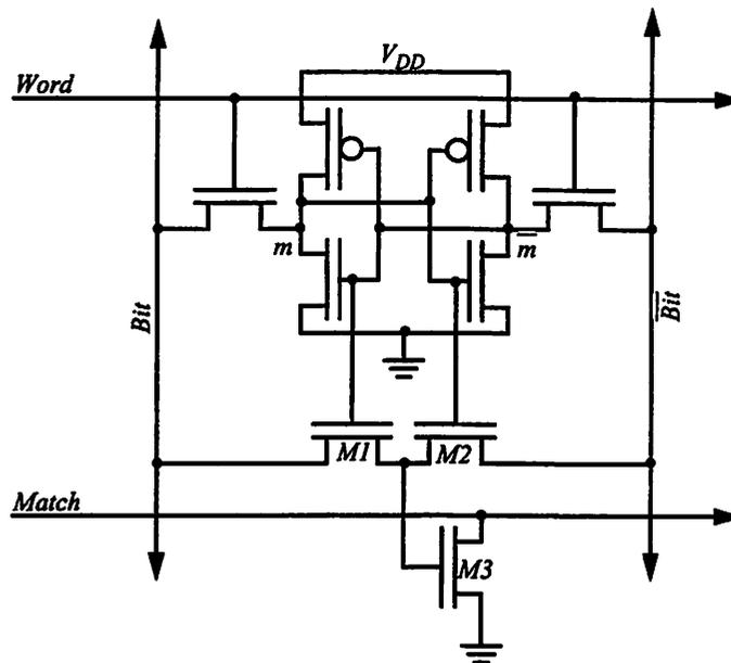
FIGURE 6.12 : Traditional CAM Cell.
