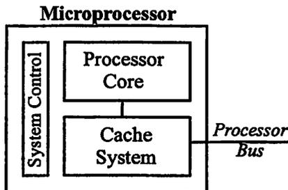
FIGURE 5.3 : Prototype Microprocessor Architecture.
