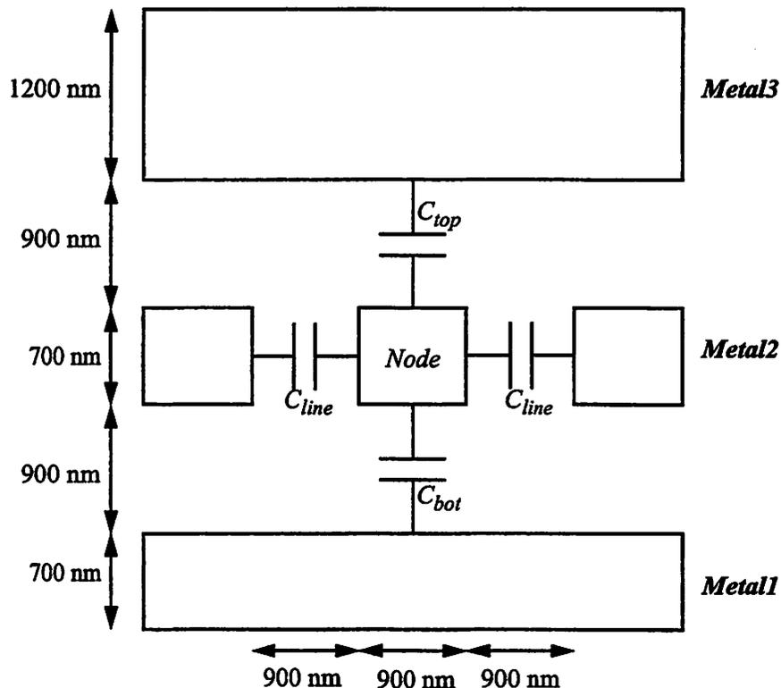
FIGURE 6.6 : Interconnect Dimensions and Capacitance Components (MOSIS  $0.6\mu\text{m}$ )
