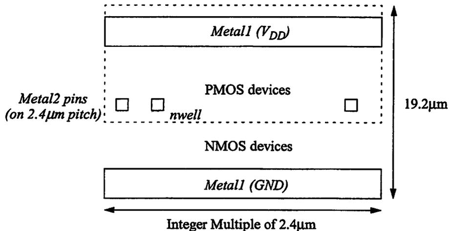
FIGURE 6.9 : Standard Cell Layout Constraints.
