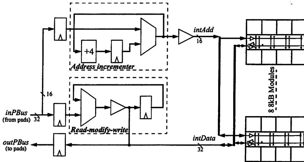
FIGURE 7.33 : SRAM Architecture.
