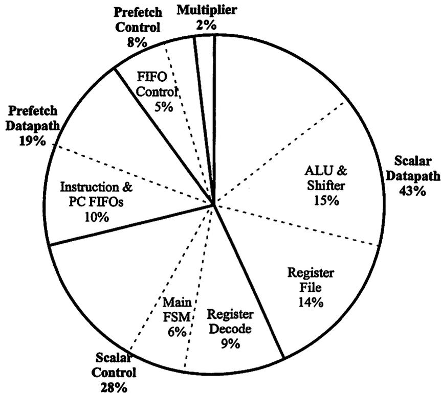
**FIGURE 7.11 : ARM8 Energy Breakdown (Full Core Simulation).**
