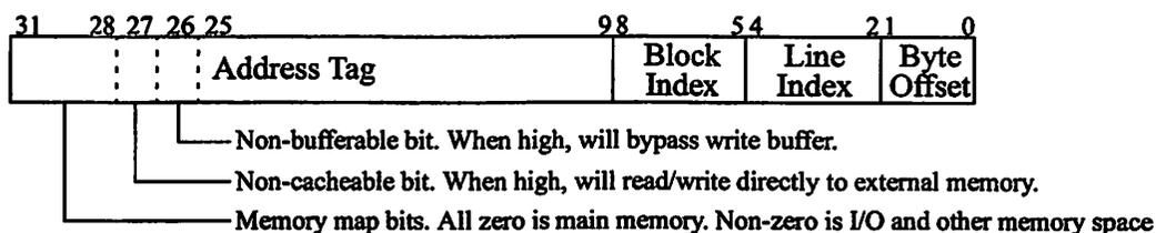
**FIGURE 7.12 : Address Space Breakdown.**
