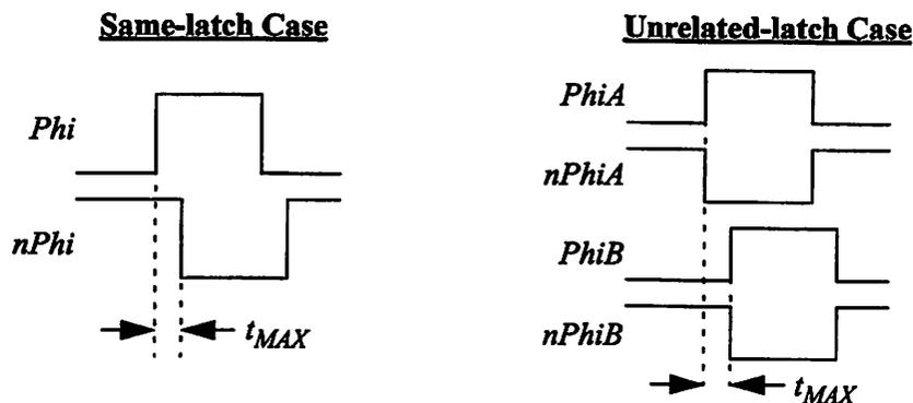
**FIGURE 4.10 : Maximum Allowable Clock Skew Measurement for Race Immunity.**
