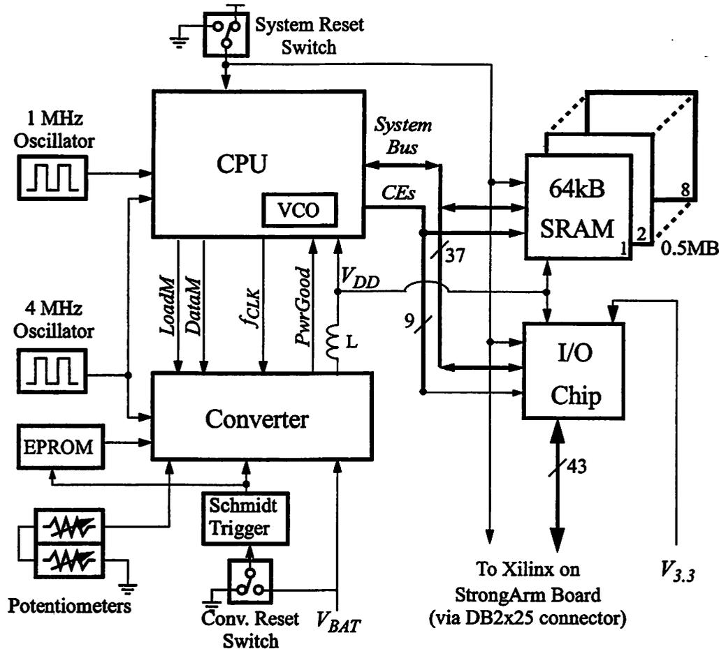
FIGURE 7.39 : Prototype Board Architecture.
