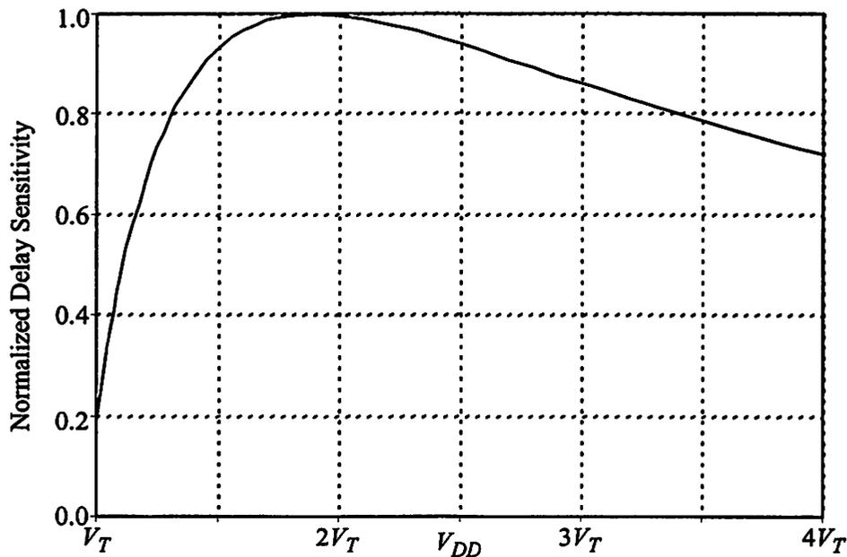
FIGURE 3.15 : Normalized Delay Sensitivity vs. Supply Voltage.
