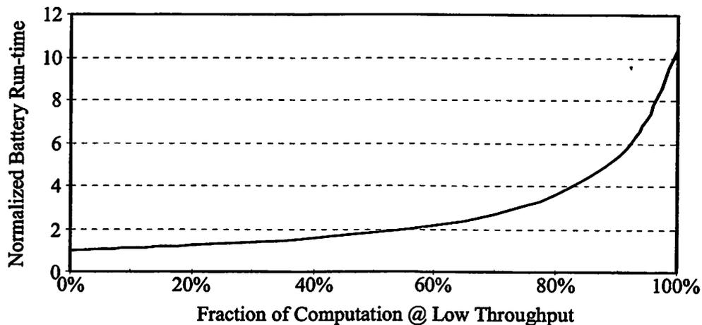
**FIGURE 3.3 : Battery Run-time vs. Workload**
