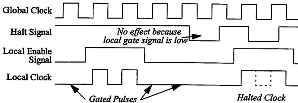
**FIGURE 4.8 : Clock Gating & Halting Timing.**
