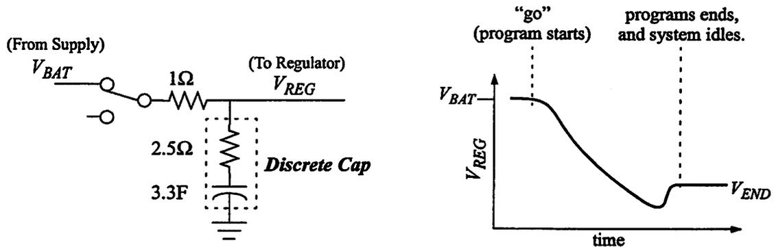
FIGURE 7.49 : Energy Measurement Circuit & Transient Response.
