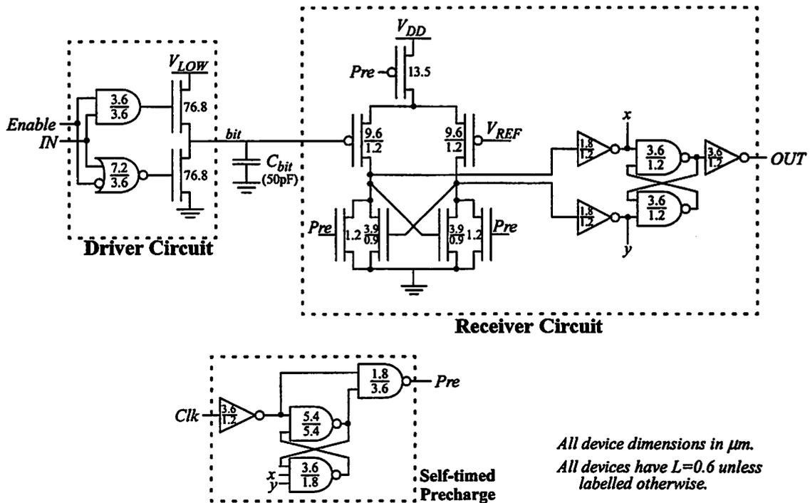
**FIGURE 6.17 : Single-ended Low-Swing Bus Transceiver Circuit.**
