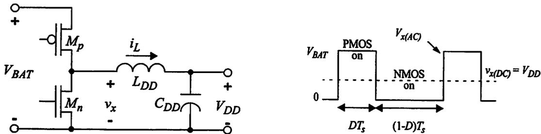
**FIGURE 3.5 : Buck Converter Design and Operation.**
