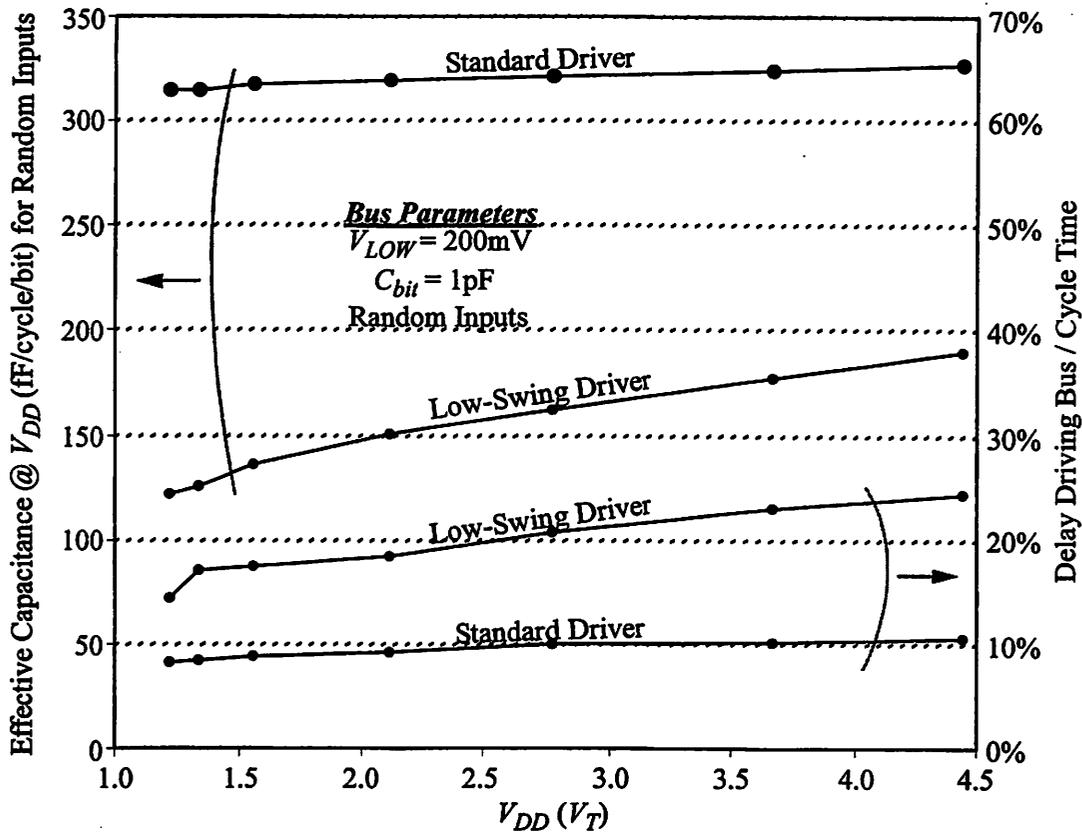
**FIGURE 6.16 : Low-Swing vs. Standard Driver for Intrachip Busses (Simulated).**
