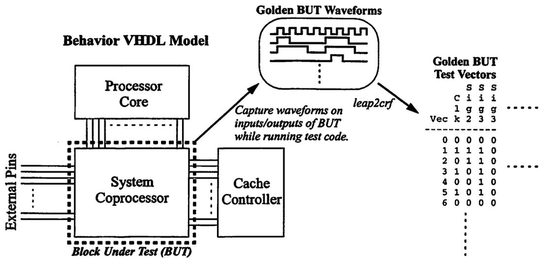
FIGURE 4.18 : Automatic Test Vector Generation
