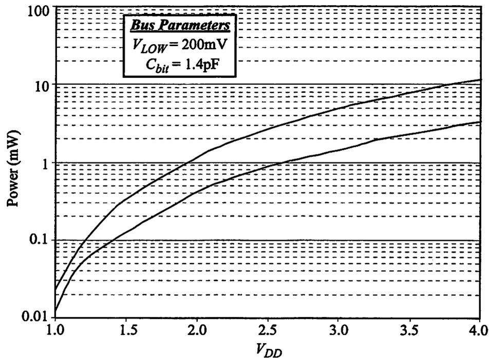
**FIGURE 6.21 : Power Dissipation of Low-Swing and Standard Driver for Intrachip Busses.**
