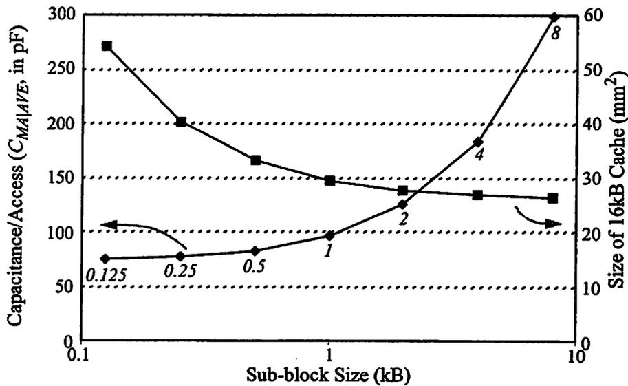
FIGURE 5.8 : Capacitance/access and Cache Size versus Sub-block Size (0.6 $\mu\text{m}$  CMOS).
