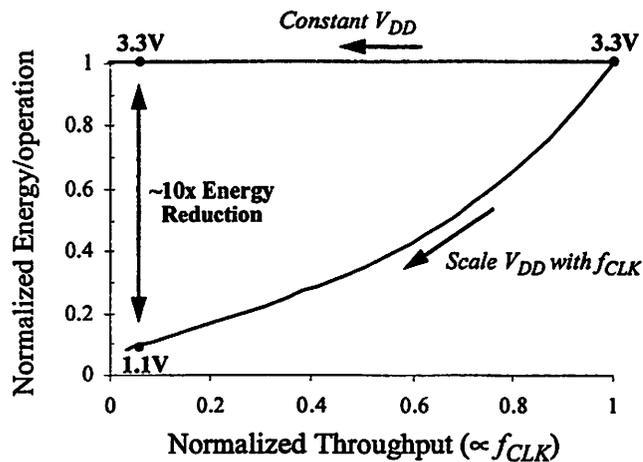
FIGURE 3.2 : Scaling  $V_{DD}$  with  $f_{CLK}$ .
