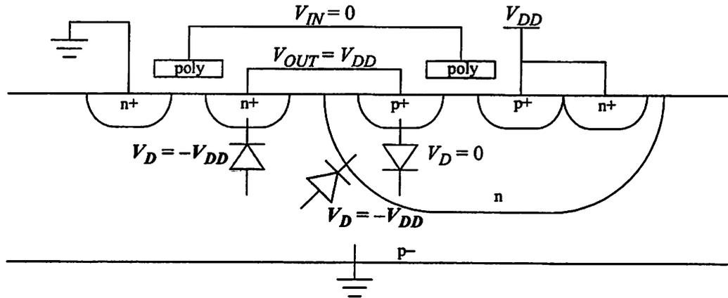
**FIGURE 2.5 : Reverse-biased Diodes in CMOS Inverter.**
