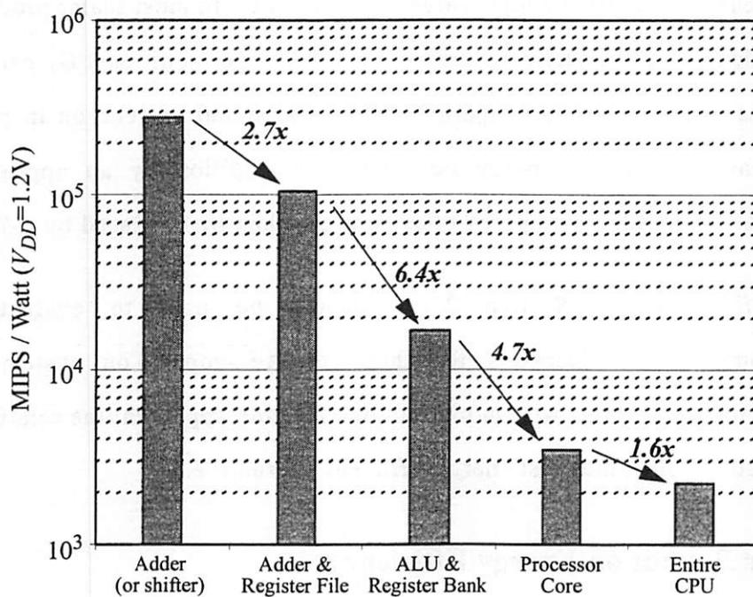
**FIGURE 5.6 : Energy Consumption for the CPU and its Base Components (0.6 $\mu$ m CMOS).**
