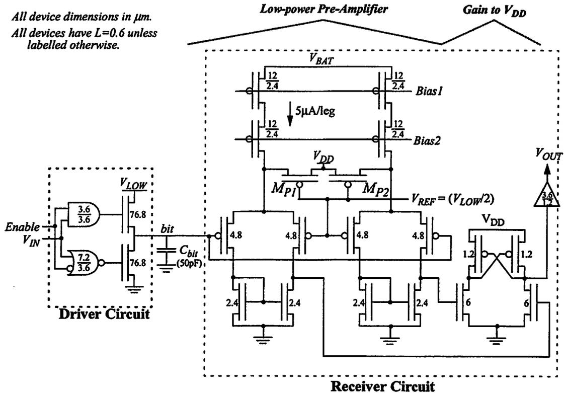
FIGURE 6.19 : Single-ended Low-Swing Clock Transceiver Circuit.
