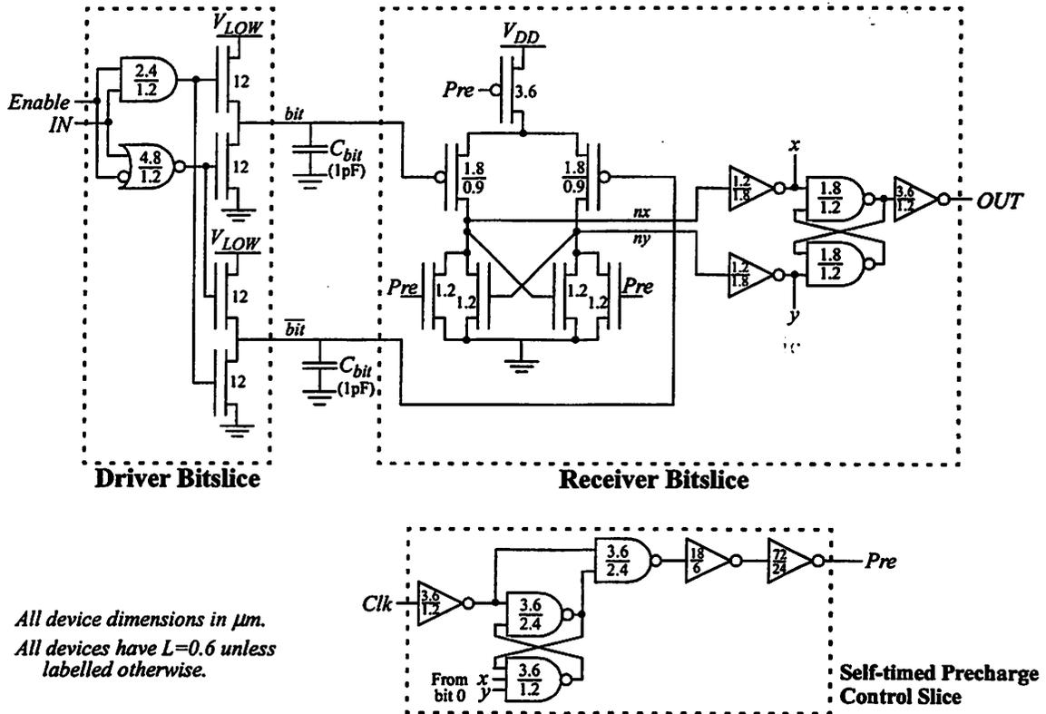
**FIGURE 6.15 : Differential Low-Swing Bus Transceiver Circuit**
