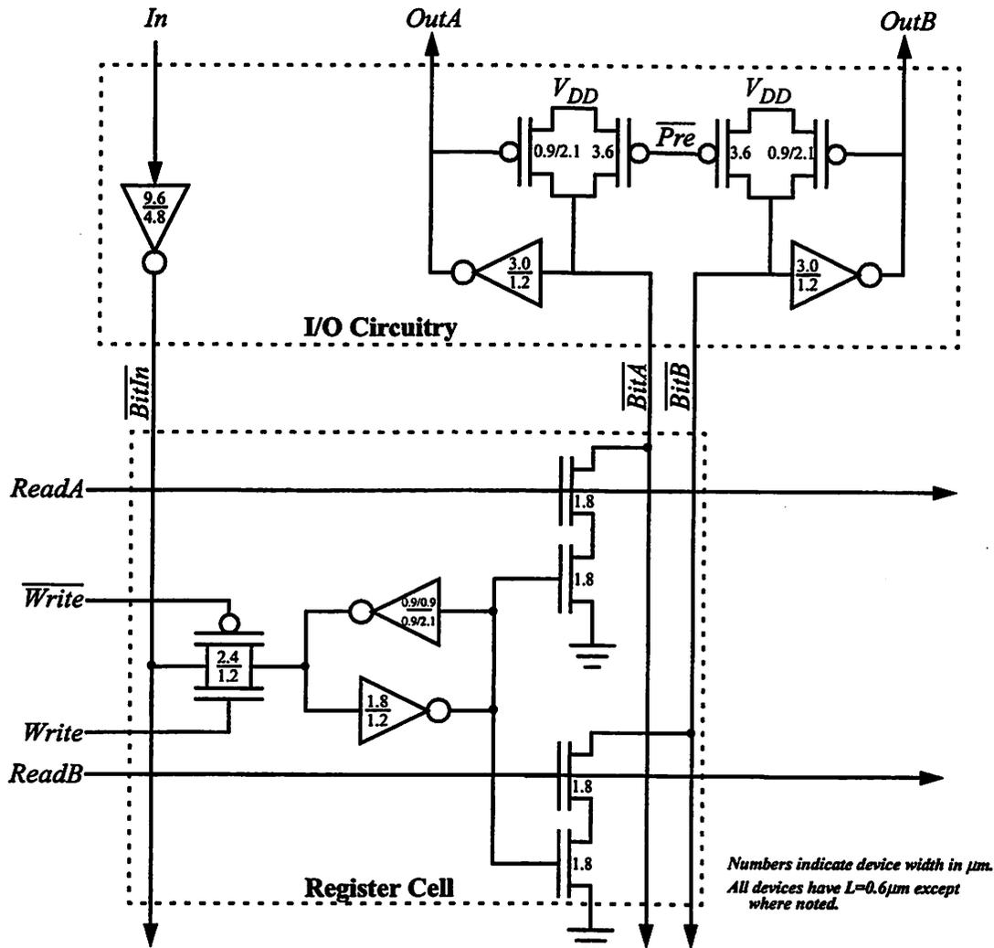
FIGURE 6.14 : Register File Cell and I/O Circuits.
