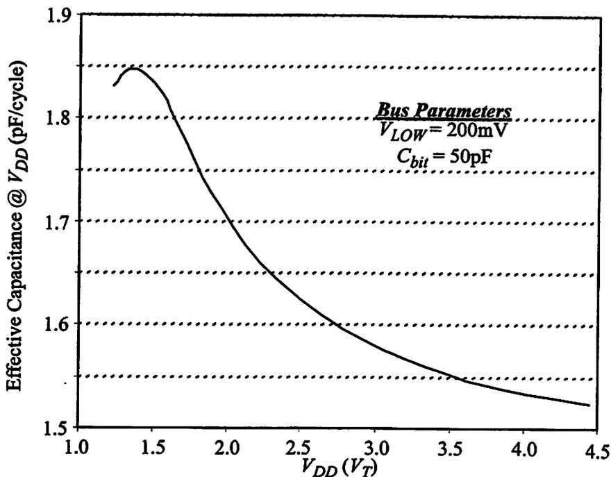
FIGURE 6.20 : Low-Swing Clock Transceiver Energy Consumption (Simulated).
