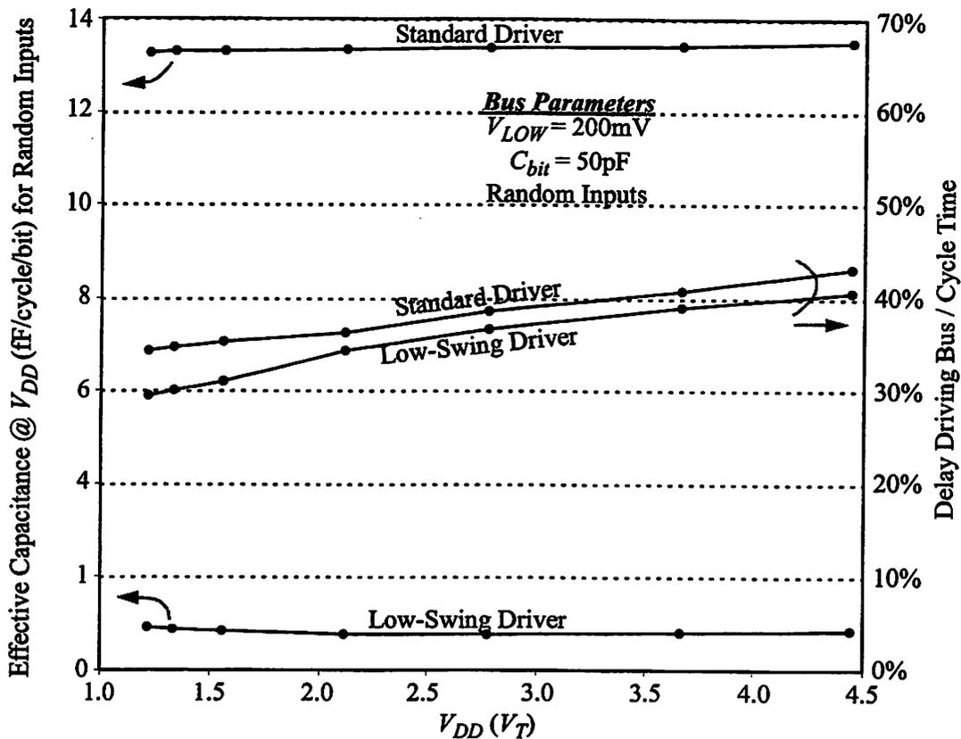
**FIGURE 6.18 : Low-Swing vs. Standard Driver for External Busses (Simulated).**
