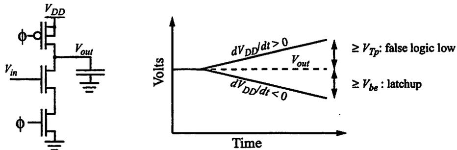
FIGURE 3.18 : Failure Modes for Dynamic Logic with Varying  $V_{DD}$ .
