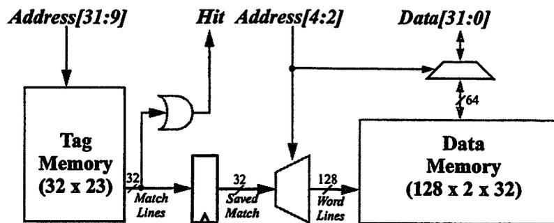
**FIGURE 5.12 : Implementing an Implicit Buffer in the CAM/RAM Architecture.**
