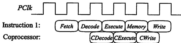
**FIGURE 7.24 : ARM8 Coprocessor Pipeline.**
