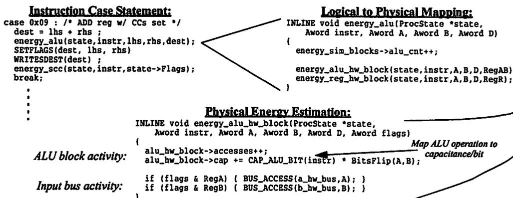
FIGURE 4.5 : Energy Estimation Implementation Example.
