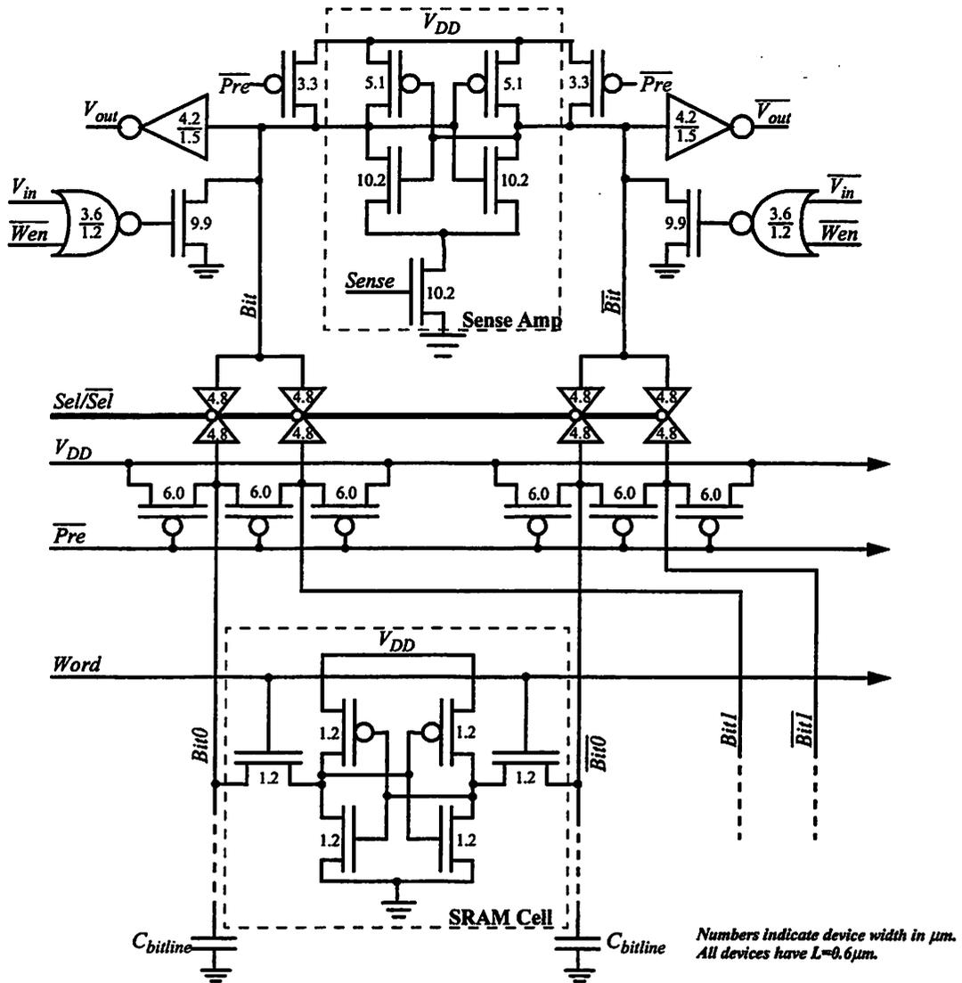
FIGURE 6.10 : SRAM Cell and Sense Amp.
