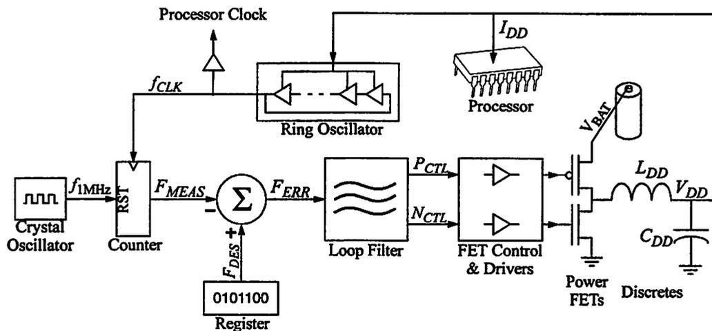
FIGURE 3.6 : DVS Voltage Converter Loop Architecture.
