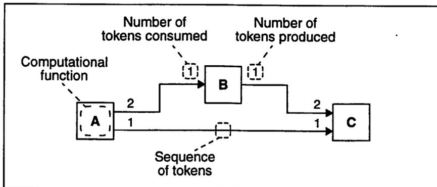
Figure 3.13 A synchronous dataflow (SDF) system.
