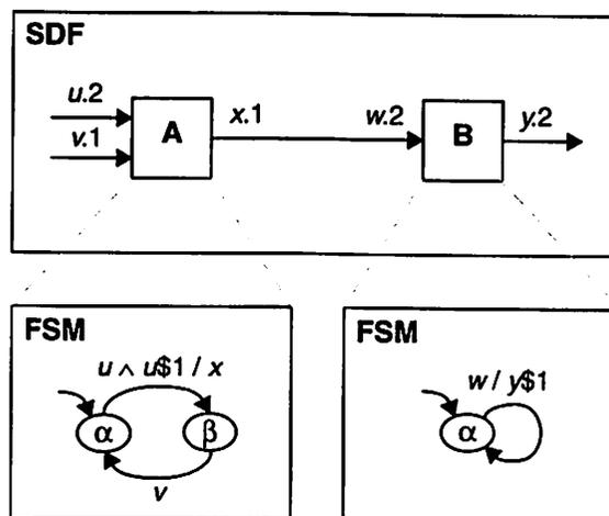
**Figure 3.17** Two FSMs are embedded within a non-homogeneous SDF system.
