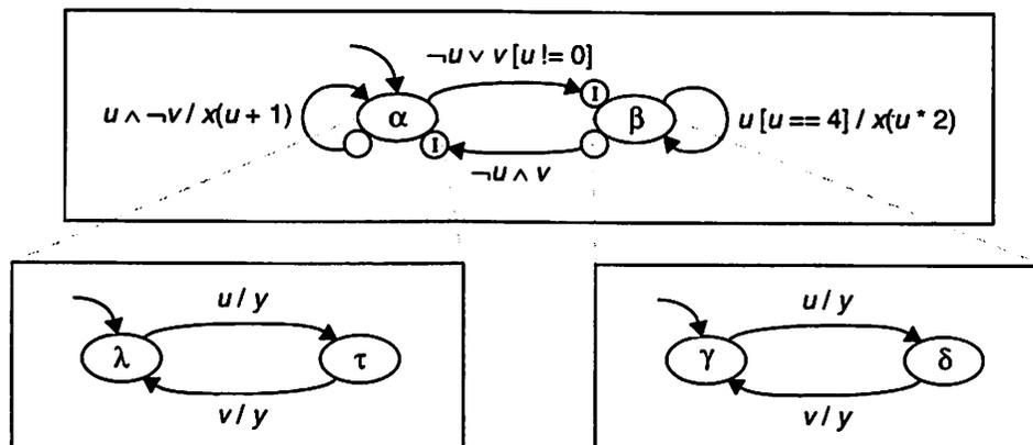
Figure 2.11 A hierarchical FSM with hierarchical entries and exits.
