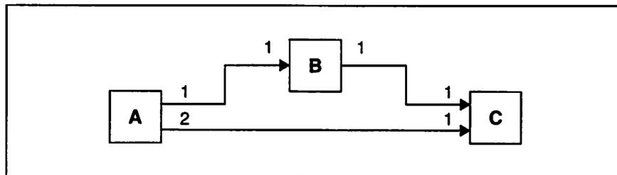
Figure 3.14 An inconsistent SDF graph.
