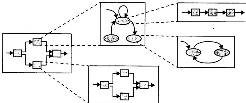
Figure 3.1 Hierarchical nesting of FSMs with concurrency models.
