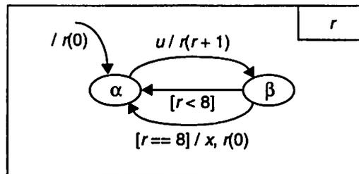
Figure 2.20 An FSM with instantaneous transitions and an instantaneous state.
