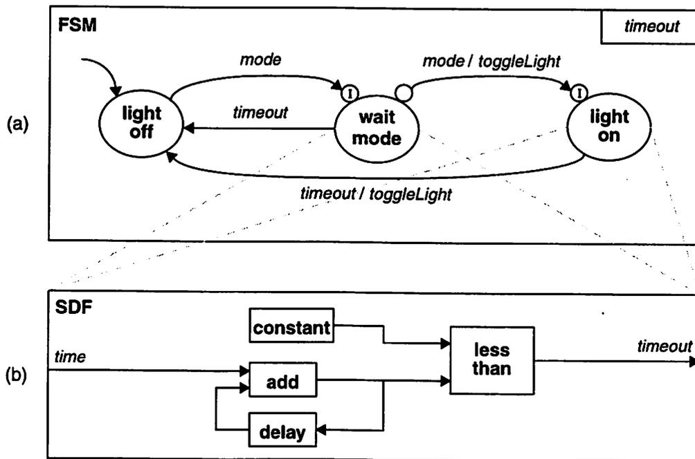
Figure 4.4 Inside the light control of figure 4.2, we have this hierarchical FSM.
