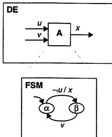
**Figure 3.6** The guard “ $\neg u$ ” of the upper transition is incomplete due to event-driven semantics of the DE model.
