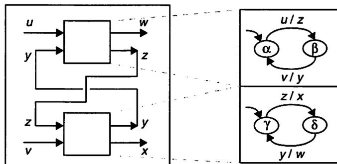
Figure 2.10 Two FSMs are embedded inside the modules of another model.
