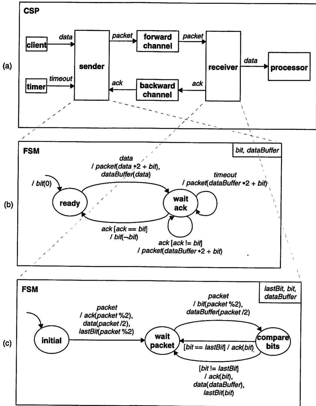
Figure 4.12 Our \*charts realization of the alternating bit protocol: (a) the topmost level, (b) the sender, and (c) the receiver.
