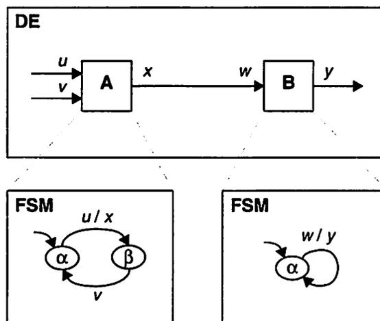
Figure 3.5 Two FSMs are embedded within a DE system.
