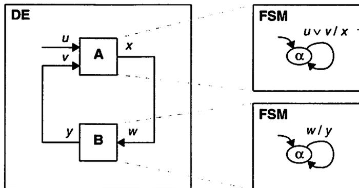
Figure 3.7 A directed loop that has zero delay can cause a problem in a DE system.
