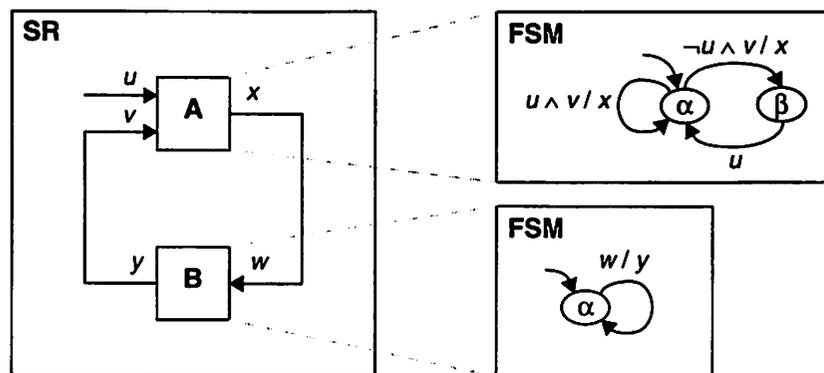
Figure 3.12 Two FSMs are embedded within an SR system and are enclosed in a directed loop.
