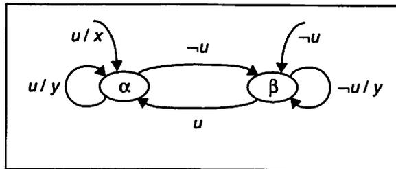
Figure 2.18 An FSM with conditional initial states.
