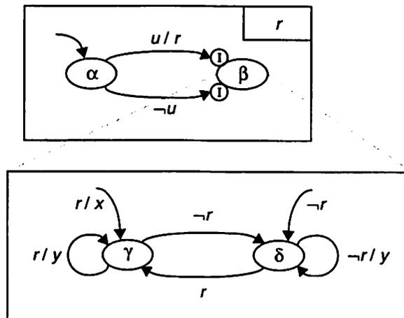
Figure 2.19 The incoming inter-level transition can be replaced by a transition with initial entry entering a conditional initial state.
