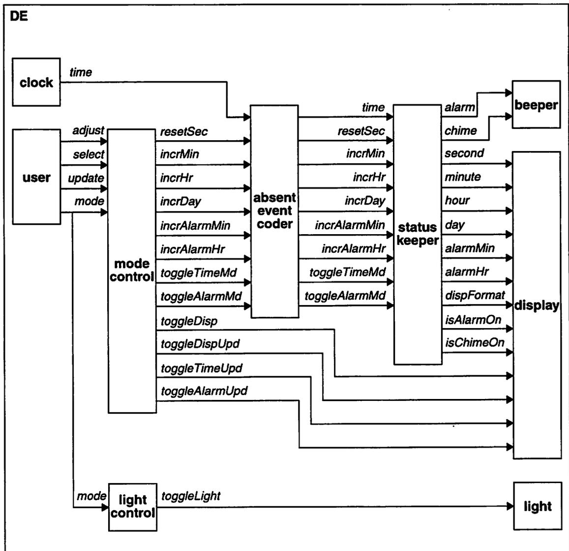
Figure 4.2 The topmost level of the \*charts realization for our digital watch.
