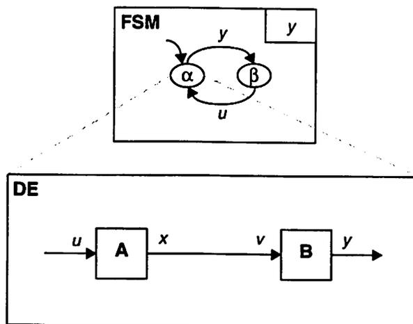
Figure 3.8 A DE subsystem refines a state of an FSM.
