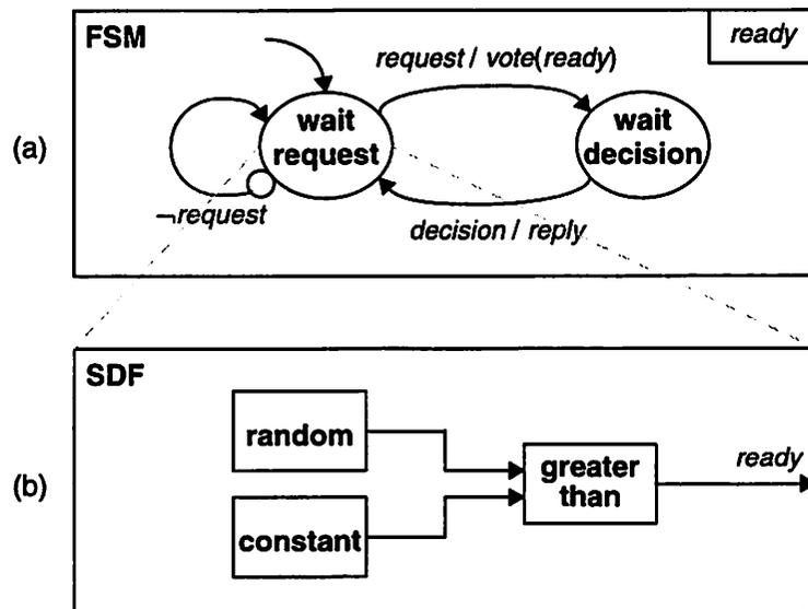
Figure 4.10 The participant1 and the participant2 in figure 4.9 are both modeled by this hierarchical FSM.
