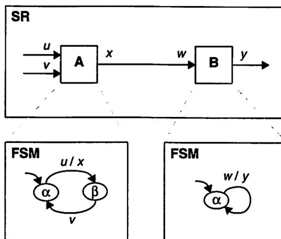
Figure 3.11 Two FSMs are embedded within an SR system.
