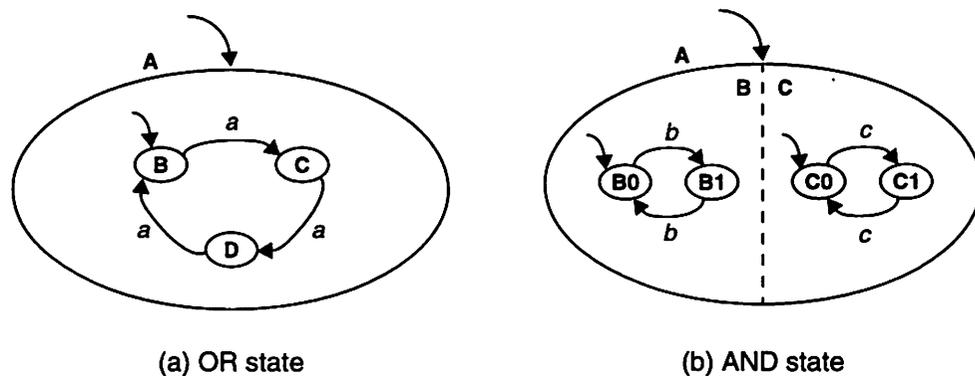
Figure 1.5 Examples of an OR state and an AND state in Statecharts.
