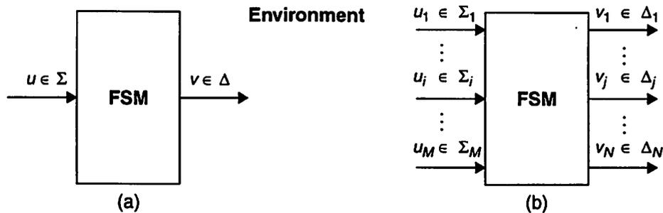
Figure 2.3 Interaction of the FSM with the environment: (a) single input and single output, and (b) multiple inputs and multiple outputs.
