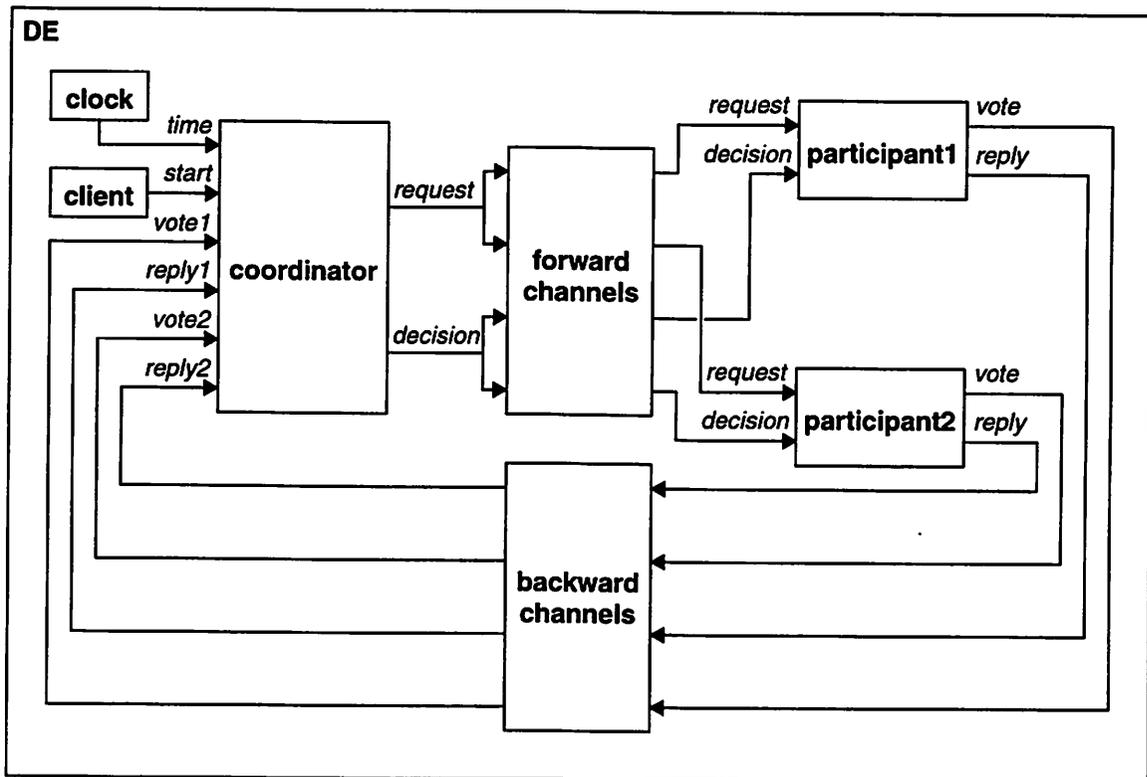
Figure 4.9 The topmost level of our \*charts realization for the two-phase commit protocol.
