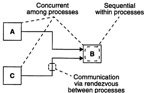
Figure 3.20 A communicating sequential processes (CSP) system.
