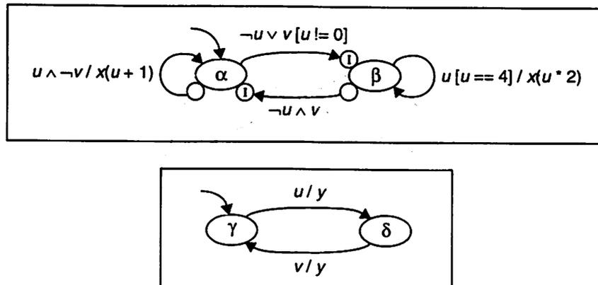
Figure 2.13 A hierarchical FSM with a shared slave.
