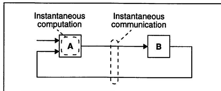
Figure 3.9 A synchronous/reactive (SR) system.
