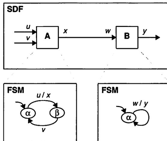
**Figure 3.16** Two FSMs are embedded within a homogeneous SDF system.
