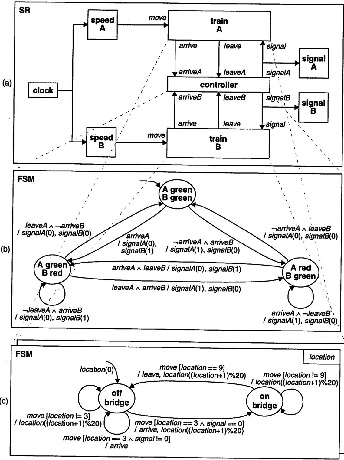
Figure 4.7 Our \*charts realization for simulating the railroad control problem.
