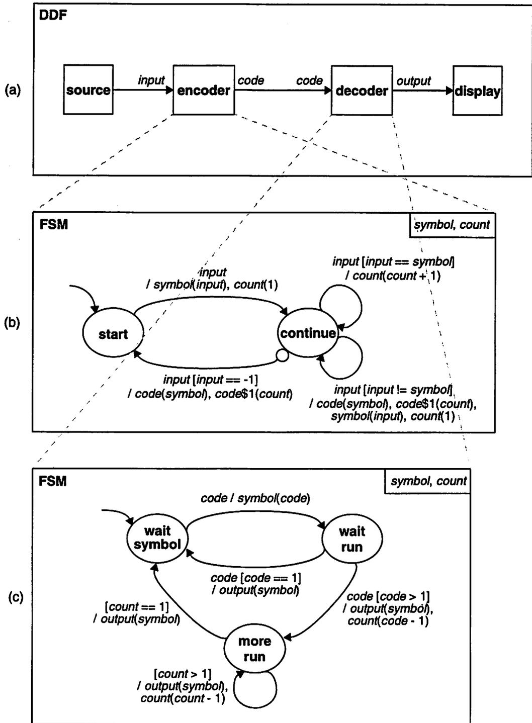
Figure 4.8 Our realization of the run-length coding using \*charts.
