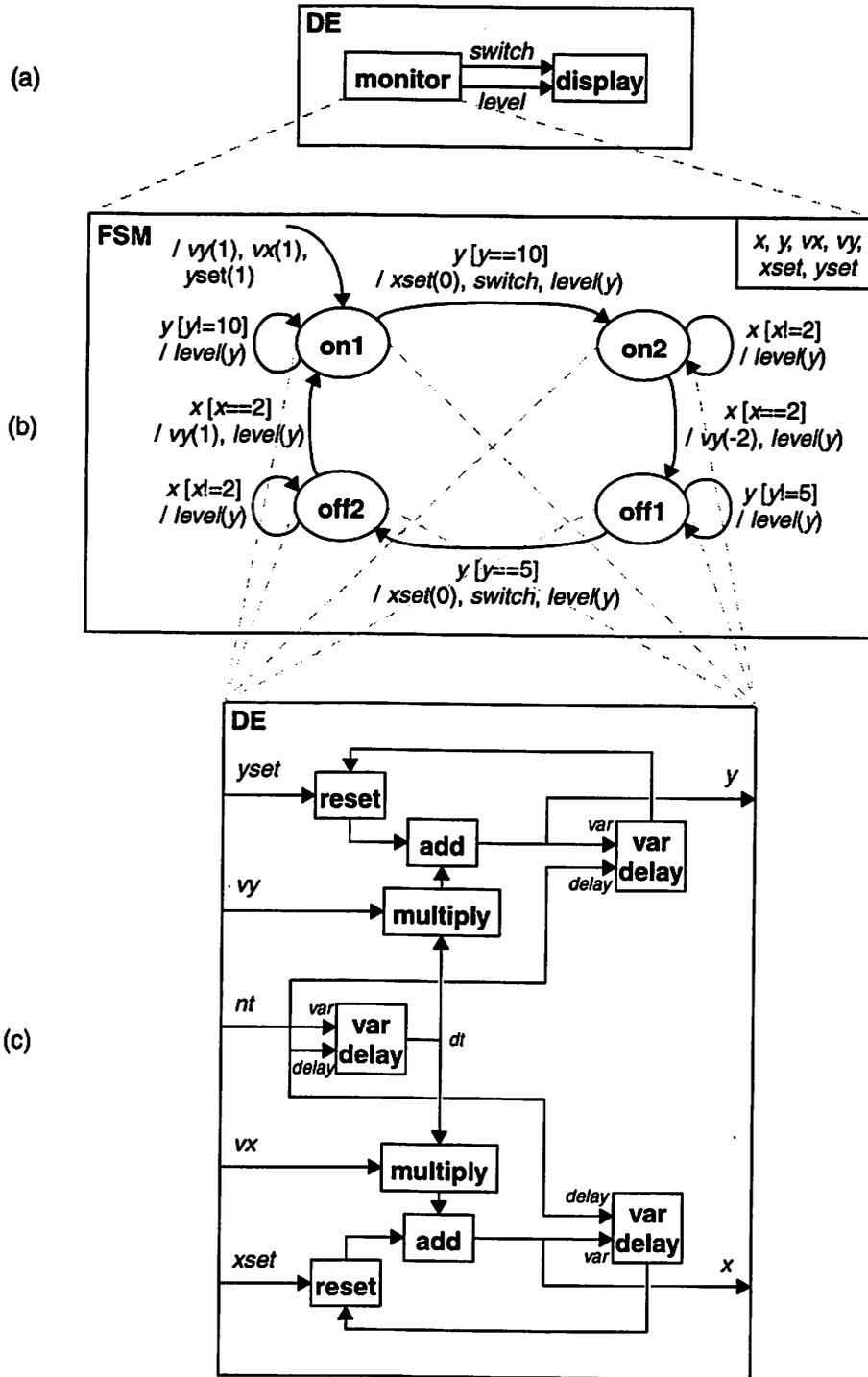
Figure 4.14 The \*charts realization of the water-level monitor.
