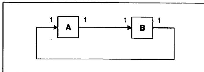
Figure 3.15 A deadlocked SDF graph.
