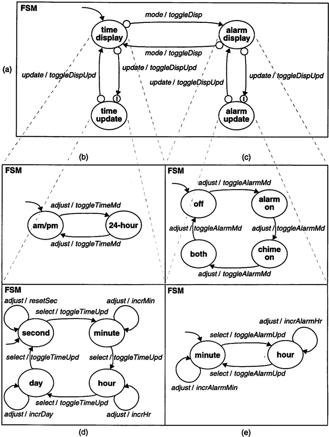
Figure 4.5 Inside the mode control of figure 4.2, we have this hierarchical FSM.
