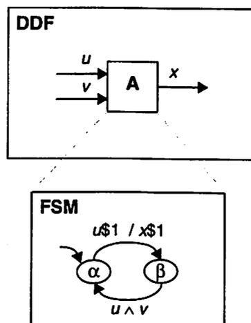
Figure 3.19 An FSM are embedded within a DDF system.
