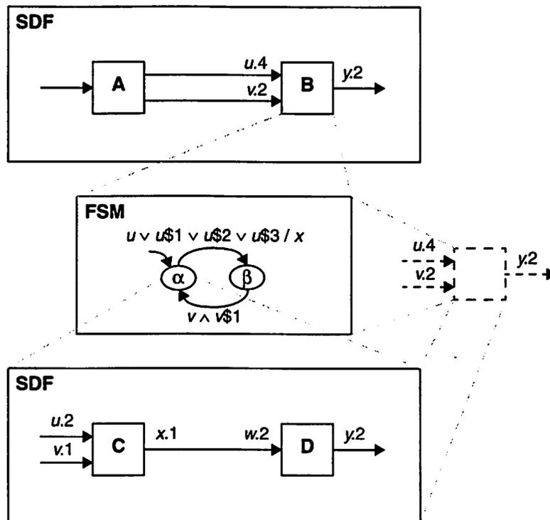
**Figure 3.18** The type signature of the inner SDF subsystem becomes the type signature of the FSM itself. Thus, the outer SDF system treats the FSM as a non-homogeneous block with the given type signature.
