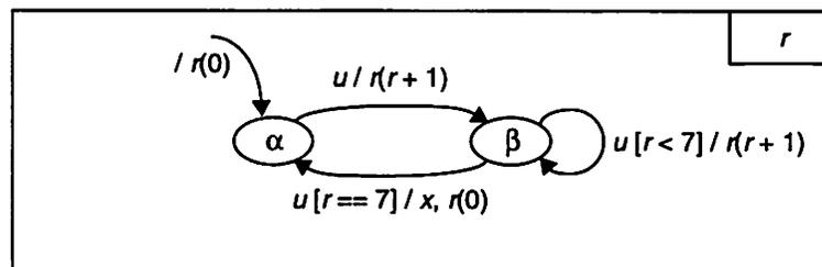
Figure 2.17 An FSM with an initial transition to initialize a local event.
