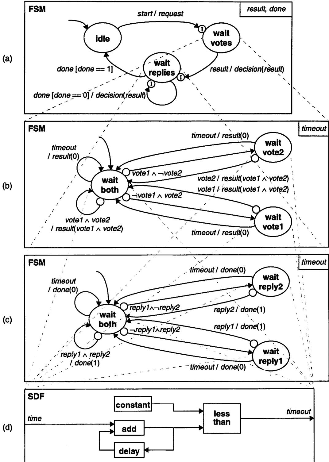
Figure 4.11 This hierarchical FSM models the coordinator in figure 4.9.
