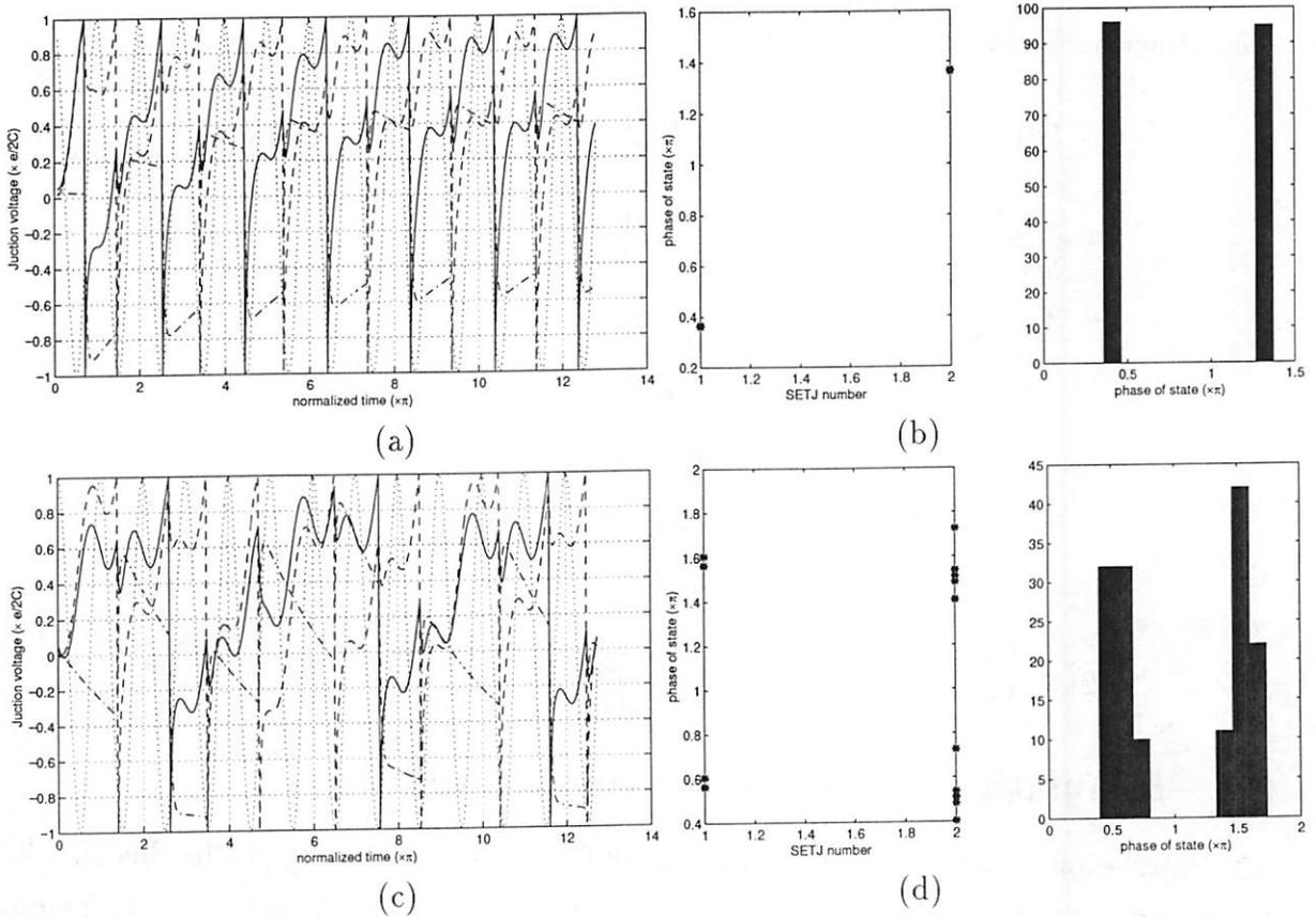
Figure 4: Simulation results of two coupled SETJs. (a) The phase states of two SETJs are stable when  $a_1 = a_2 = 2$ . (b) The histogram of the two phase states corresponding to (a). (c) The phase states of the two SETJs are no longer stable when we change  $a_1$  to 1 while other conditions are kept unchanged. (d) The histogram of the two phase states corresponding to (c).
