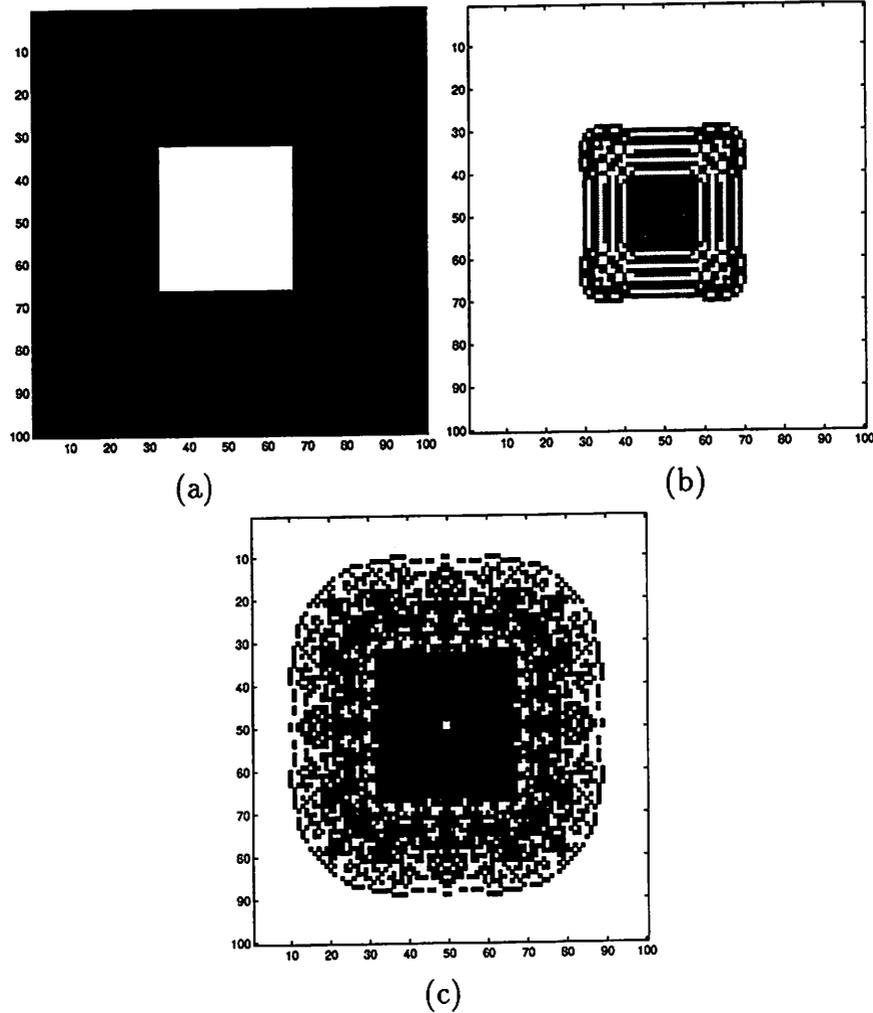
Figure 12: Simulation result of corner and edge detection performed by a SETJ CNN. Parameters are given by:  $b = 2$ ,  $\gamma = 1/3$ ,  $\epsilon = 1$ , and  $k = 0.1$ . The fixed simulation step is 0.1. The initial conditions are:  $x_{ij}(0) = u_{ij}$ ,  $p_{ij}(0) = q_{ij}(0) = 0$ . (a) The input image  $u_{ij}$ . (b) The phase state at  $t = 30$  time units shows the boundaries, corners and center. (c) The phase state at  $t = 200$  time units shows some characteristics of a 2D CA.
