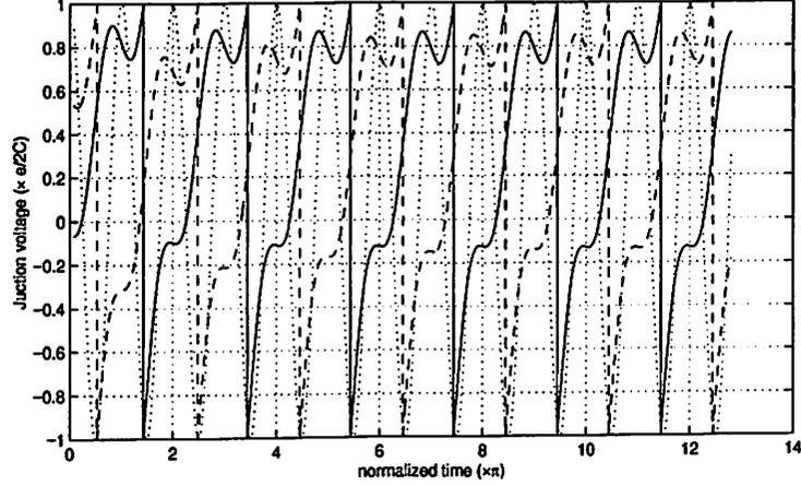
Figure 2: Simulation results of the two phase states generated by an isolated SETJ cell with two different initial conditions.
