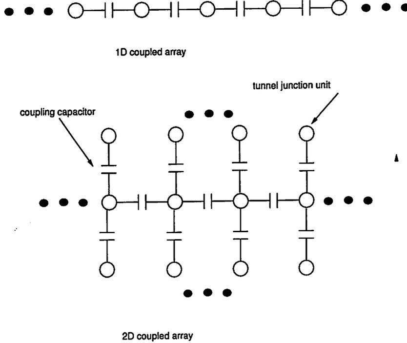
Figure 10: Coupling single-electron junctions into 1D or 2D CNN arrays.
