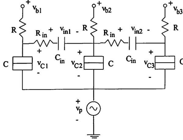
Figure 8: Block diagram of three coupled SETJs.
