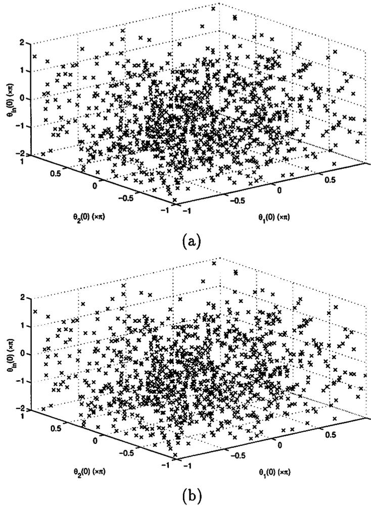
Figure 7: The stable phase states of two coupled SETJs under different initial conditions. The symbols “\*” and “o” denote logic TRUTH and logic FALSE, respectively. The symbol “x” denotes that a SETJ can show both logic TRUTH and logic FALSE in its evolution. (a) SETJ 1. (b) SETJ 2.
