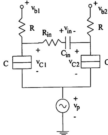
Figure 3: Circuit block diagram of two coupled SETJs.
