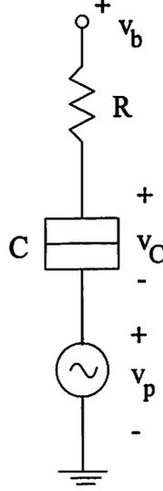
Figure 1: Circuit block diagram of an isolated single-electron tunneling junction.
