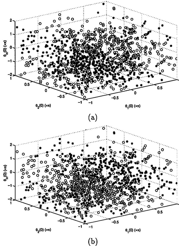
Figure 6: The stable phase states of two coupled SETJs under different initial conditions. The symbols “\*” and “o” denote logic TRUTH and logic FALSE, respectively. (a) SETJ 1. (b) SETJ 2.
