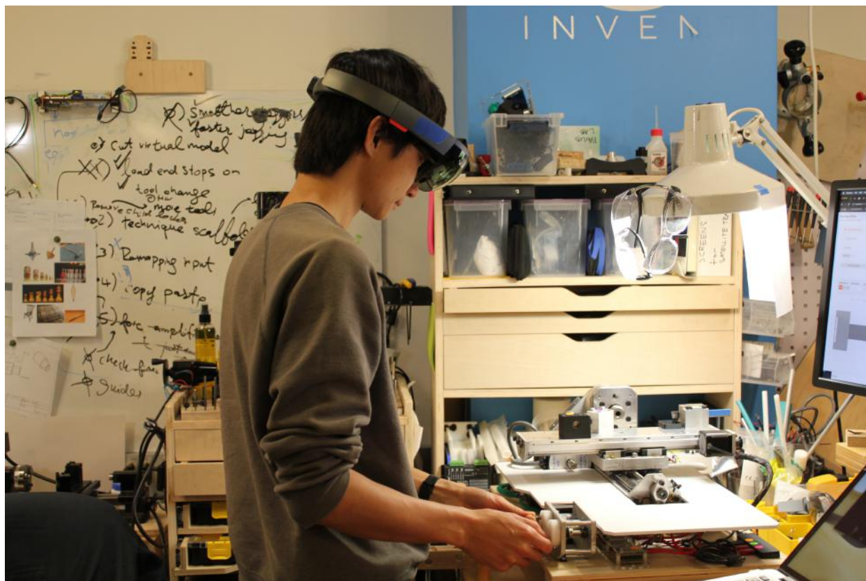
Figure 6.1: A user views the virtual work piece on the Turn-by-WiARlathe through the Microsoft HoloLens AR headset.
