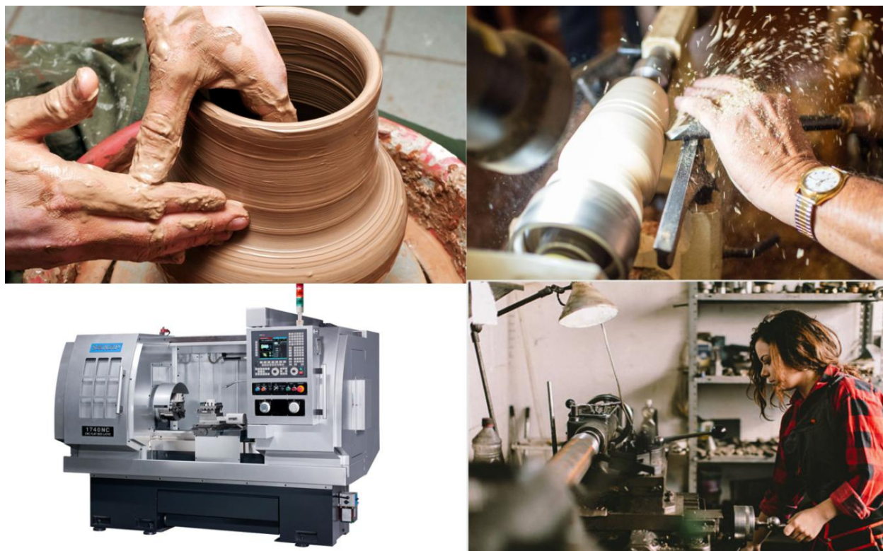
Figure 1.1: Different kinds of lathes. From top-left clockwise: A ceramicist's pottery wheel, a wood lathe, a manual lathe, a CNC lathe [9], [21], [50], [20].
