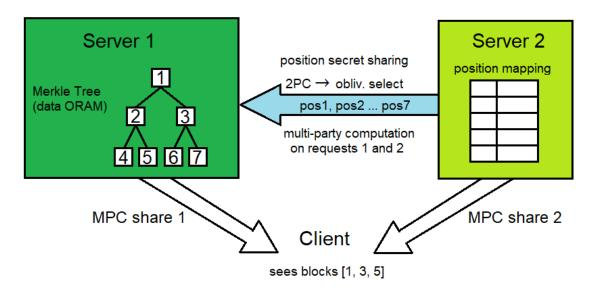
Figure 3.1: The two servers use two-party computation to create the client's request, without knowing the other's share.
