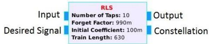
Figure 9. The Recursive Least Square function block (GNU Radio)
