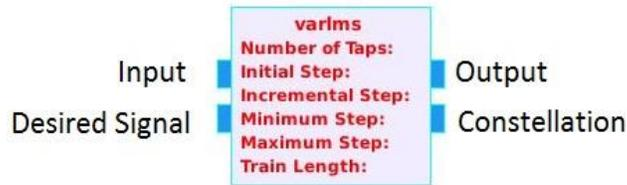
Figure 8. The Variable Step LMS function block(GNU Radio)
