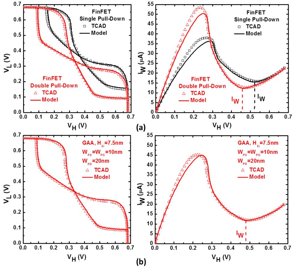
Fig. 2.9 Butterfly plots (left) and write-N curves (right) for 6-T SRAM cells implemented with SOI FinFETs (a) or GAA MOSFETs (b). Good agreement in SNM and  $I_w$  between TCAD (mixed-mode) simulations and the compact model is seen.
