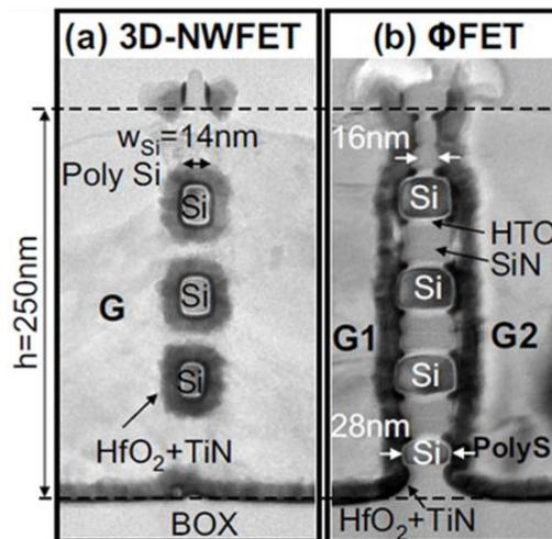
Fig. 1.5 Cross-sectional TEM images of stacked GAA MOSFETs [1.11].
