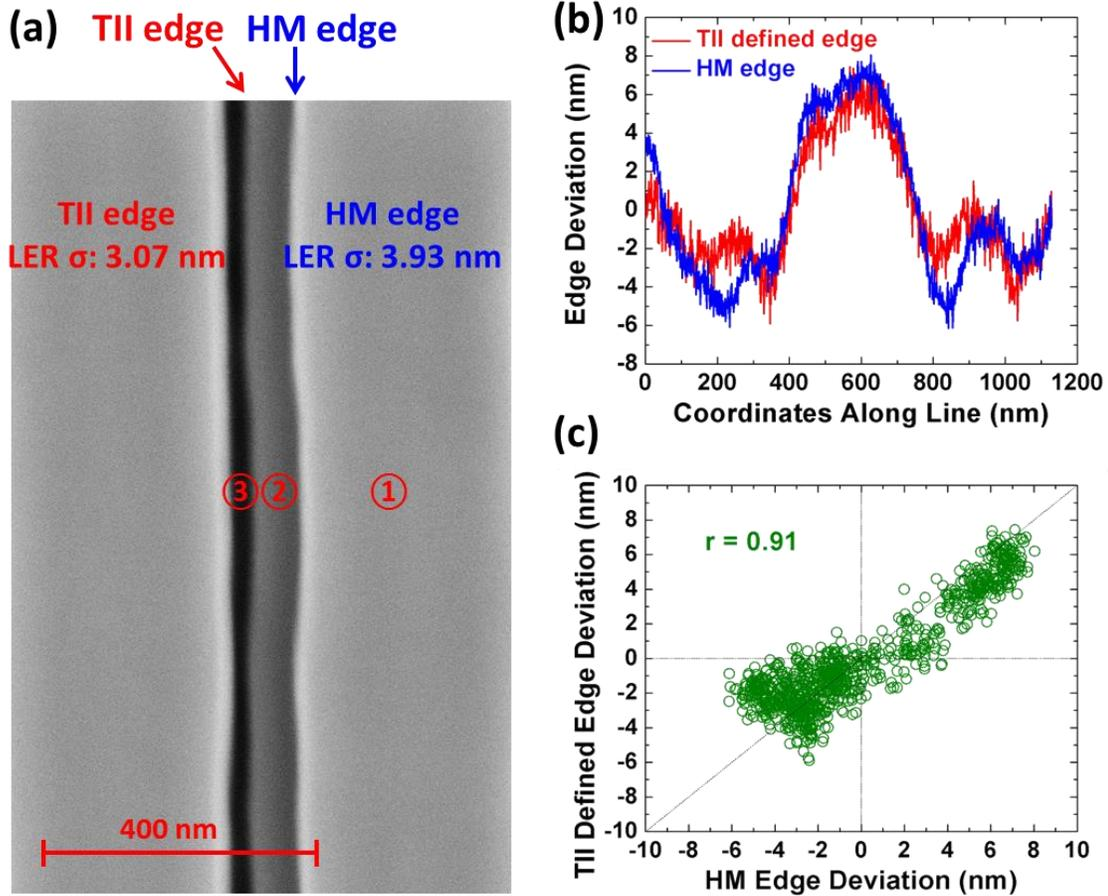
Fig. 4.14 (a) Plan-view SEM image showing that the line-edge roughness (LER) of a TII-defined edge is lower than that of its corresponding HM edge. ①: a-Si hard mask, ②: c-Si (unetched, due to SiO<sub>2</sub> protection), ③ Sub-lithographic trench in c-Si. (b) deviations (from average position) of TII-defined edge and HM edge along the length of the masking feature (*i.e.* in the vertical direction in Fig. 4.14(a)). (c) correlation between deviations of TII-defined edge and HM edge.
