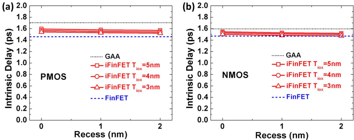
Fig. 3.15 Dependence of iFinFET intrinsic delay on inserted-oxide thickness ( $T_{iox}$ ) and recess distance, for (a) PMOS and (b) NMOS. For reference, the intrinsic delay values for the FinFET (dashed line) and for the stacked-NW GAA FET (dotted line) are shown.
