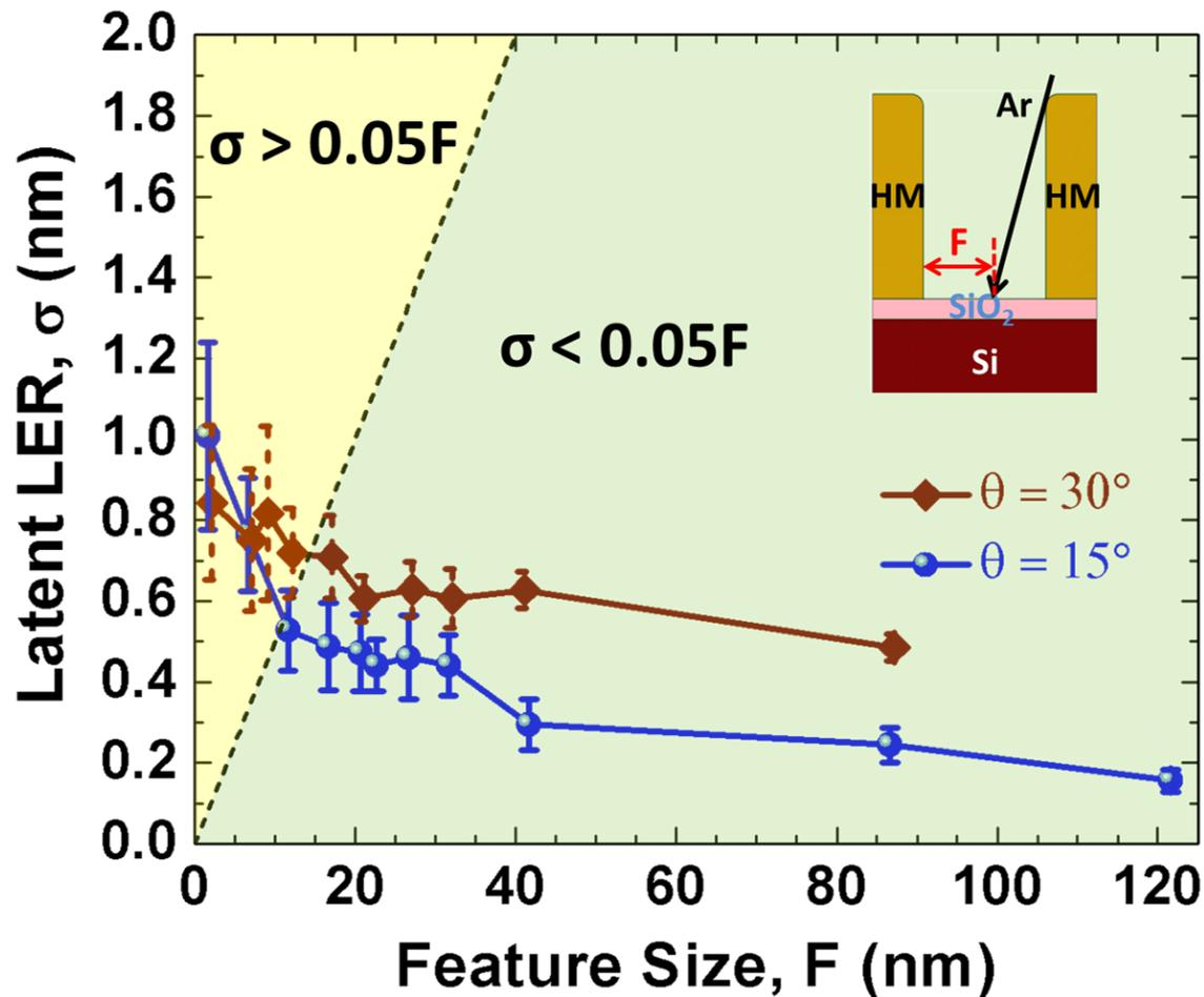
Fig. 4.13 Simulated impact of ion backscattering from the HM sidewall, on the latent line-edge roughness (LER) of the implanted oxide region. (The average implant-defined feature size,  $F$ , is changed by adjusting the HM pitch, and the HM corner radius is fixed at 3 nm.) Tilted ion implantation is projected to be suitable for patterning features as small as 10 nm with good fidelity. Error bars represent  $\pm 1$  standard deviation.
