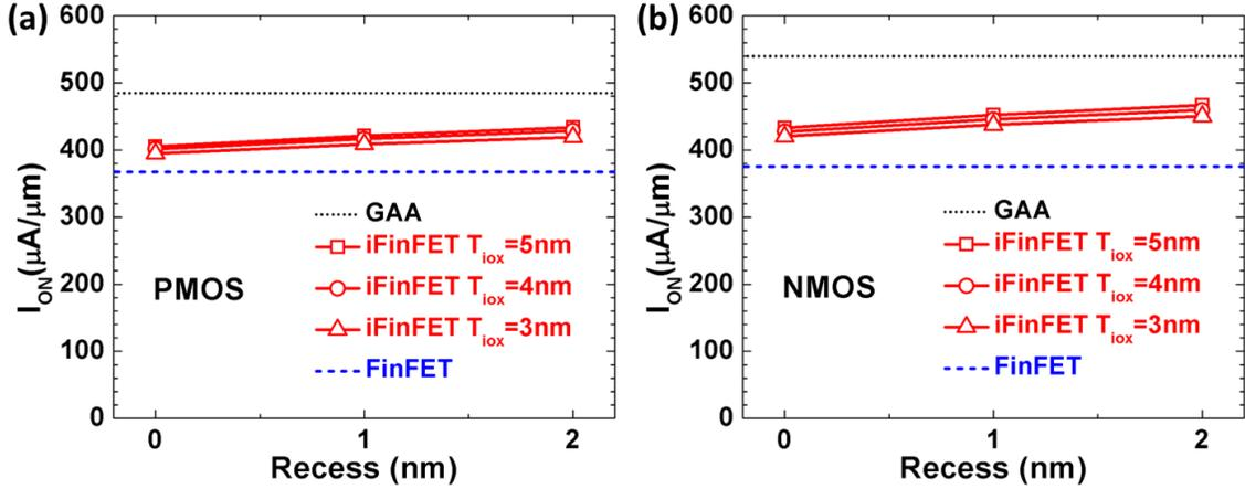
Fig. 3.14 Dependence of iFinFET ON-state drive current on inserted-oxide thickness ( $T_{iox}$ ) and recess distance, for (a) PMOS and (b) NMOS. For reference, the ON-state drive current values for the FinFET (dashed line) and for the stacked-NW GAA FET (dotted line) are shown.
