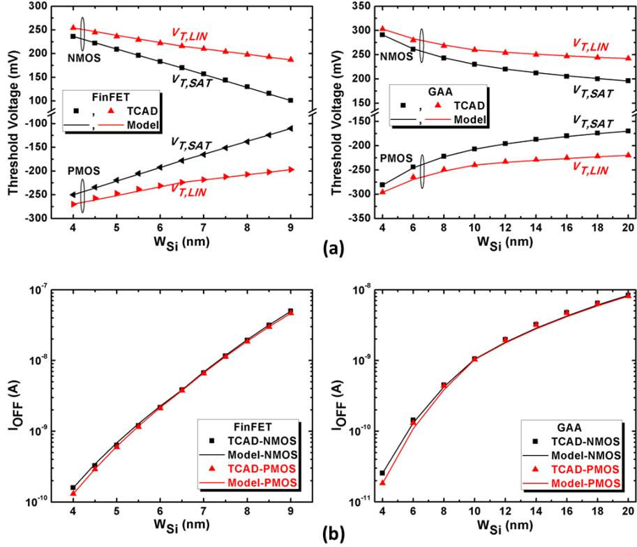
Fig. 2.5 (a) Impact of variations in fin/stripe width for  $V_T$  of SOI-FinFETs (left) and GAA MOSFETs (right). (b)  $I_{OFF}$  sensitivity to  $W_{Si}$  variation for SOI-FinFETs (left) and GAA MOSFETs (right).
