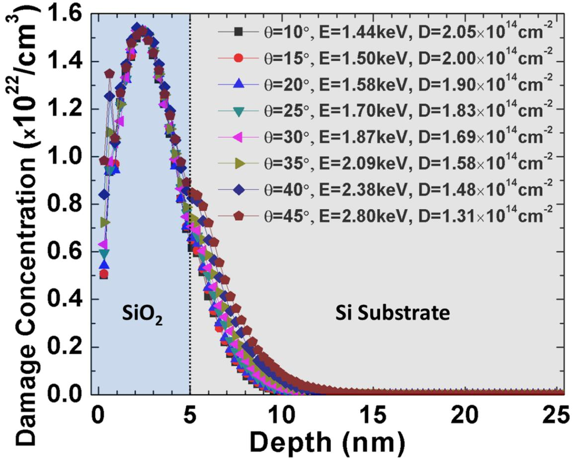
Fig. 4.6 Simulated  $\text{Ar}^+$  implantation-induced damage depth profile obtained using SRIM [4.15]. For different values of the implant tilt angle ( $\theta$ ), the implant energy ( $E$ ) and dose ( $D$ ) are adjusted to achieve the same projected range and peak damage value, respectively, in the  $\text{SiO}_2$  layer.
