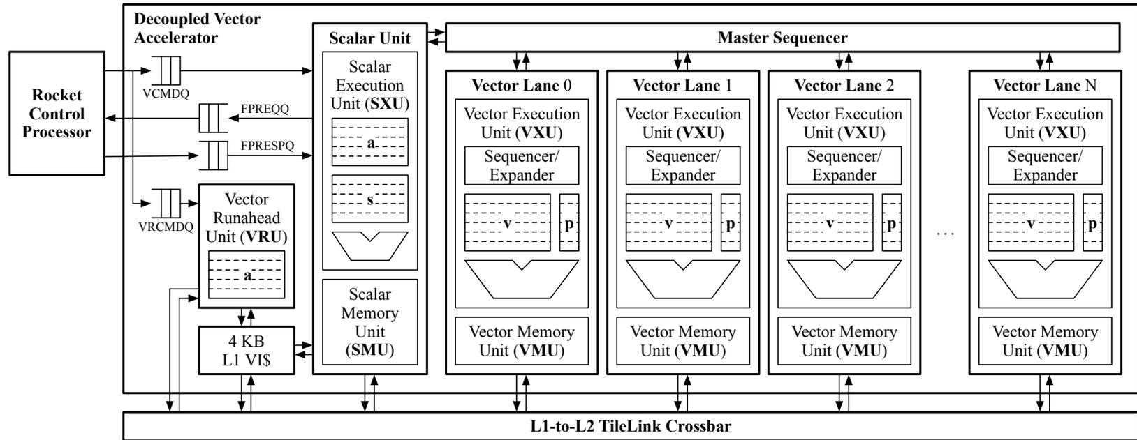
**Figure 2: Block Diagram of the Decoupled Vector Accelerator.** VCMDQ = vector command queue, VRCMDQ = vector runahead command queue, FPREQQ = floating-point request queue, FPRESQ = floating-point response queue.
