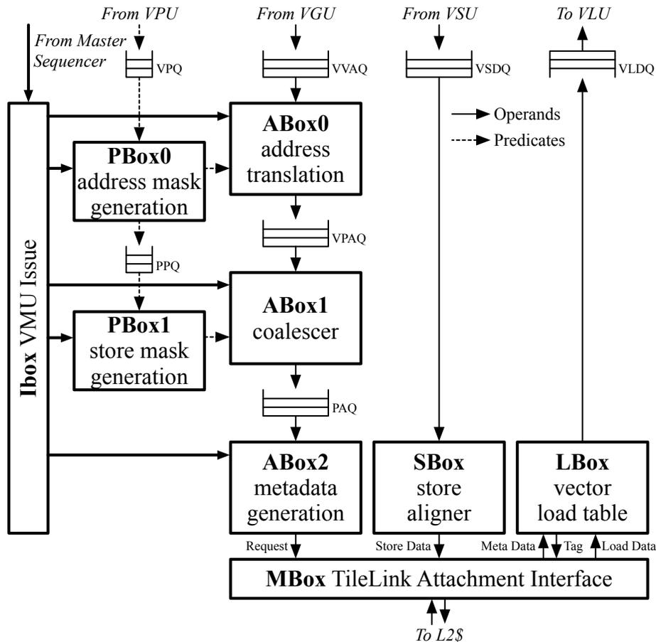
**Figure 5: Block Diagram of Vector Memory Unit (VMU).** Consult Figure 3 for VPU, VGU, VSU, VLU, VPQ, VVAQ, VSDQ, VLDQ. VPAQ = vector physical address queue, PPQ = pipe predicate queue, PAQ = pipe address queue.
