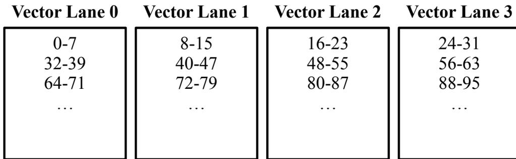
Figure 7: Mapping of elements across a four-lane machine.
