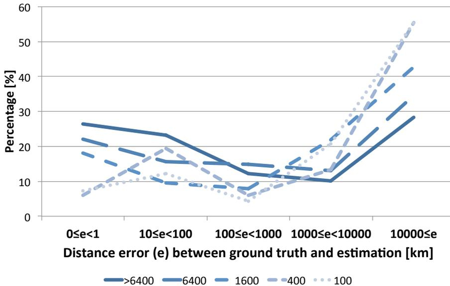
Figure 4.2: Comparison of the performance of a data-driven algorithm[18] on grids with different training data density. Query video from a denser area has higher chance of being estimated with lower error in distance.
