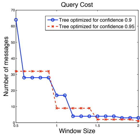
Figure 12: Comparison of hierarchies built on different confidence. The query workload is of confidence 0.95.
