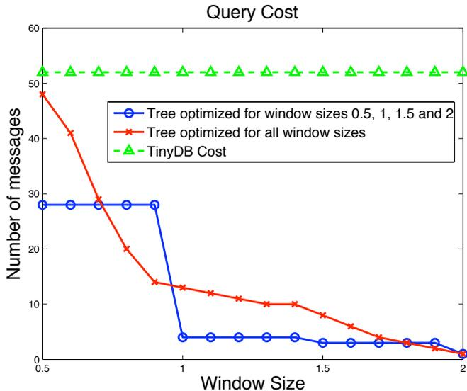
**Figure 13:** Comparing tree construction with a few vs a broader range of windows
