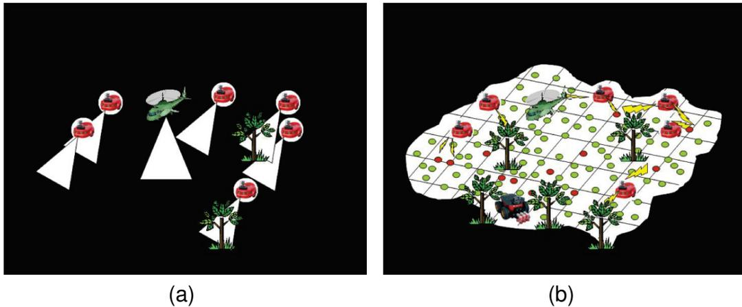
Figure 6.1: (a) Sensor visibility in PEGs without sensor network. (b) Sensor visibility in PEGs with sensor network. Dots correspond to sensor nodes, each provided with a vehicle detection sensor. Courtesy of [Sinopoli *et al.*, 2003].
