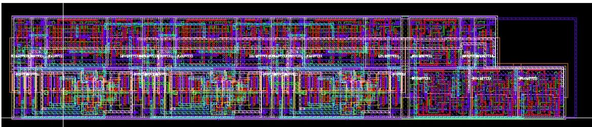
Figure 14: Programmable Divider Layout
