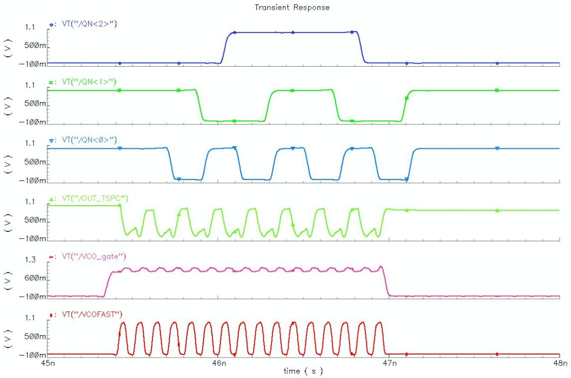
**Figure 11: Divider Waveforms for div 16 at 10 GHz**
