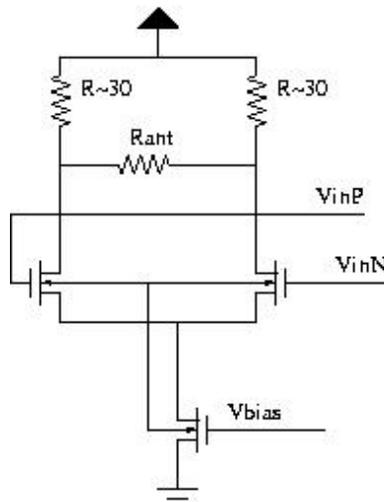
Figure 7: Power Amplifier /Antenna Driver
