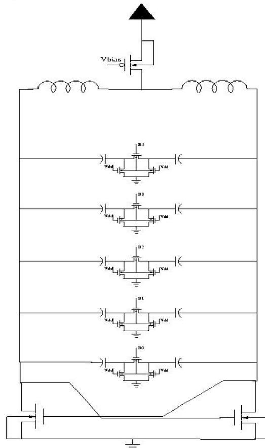
Figure 6: LC Oscillator Schematic
