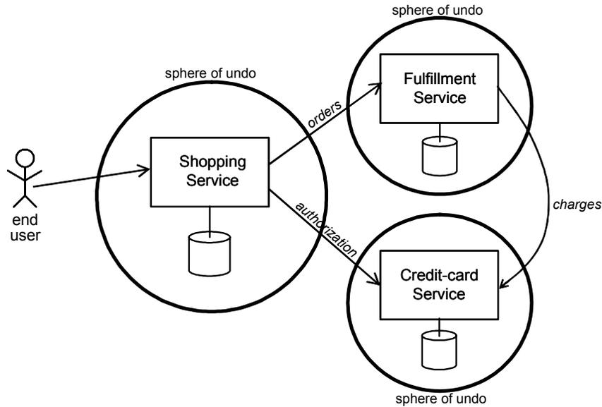
Figure 4: Spheres of undo for hypothetical online retailer architecture. Each module from Figure 3 is placed in its own sphere of undo.
