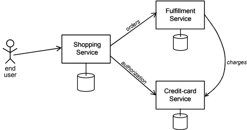
**Figure 3: Hypothetical architecture for online retailer.** The retailer’s systems are composed of three interacting modules: a front-end web service that interacts with the user, a fulfillment service that accepts orders from the front end, and a credit card service that handles authentication for the front-end and charge requests from the fulfillment service. Each module maintains its own state database.
