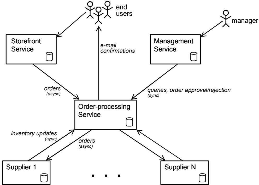
Figure 8: PetStore architecture. PetStore is comprised of three core services, the storefront, management, and order-processing services, and one or more supplier services.
