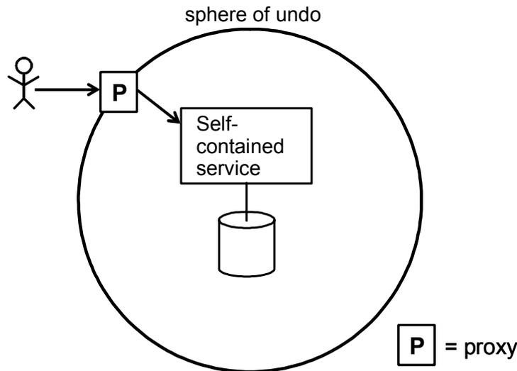
Figure 2: Self-contained single-service architecture. A self-contained service encompasses a single sphere of undo that communicates only with human end users. Requests from those end users are proxied, logged, and replayed at the sphere boundary.
