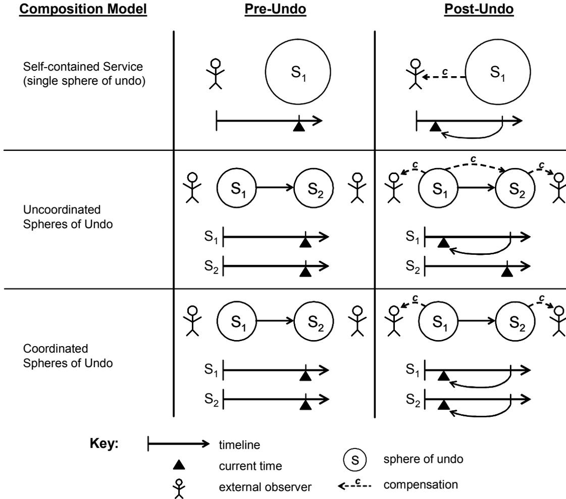
**Figure 5: Summary of composition approaches for spheres of undo.** For each model, the figure shows the schematic representation of the system and each sphere’s timeline both before and after undo is invoked. Unless otherwise noted,  $S_1$  is the sphere on which undo is invoked. If the undo process can cause compensations or explanatory messages to flow outside of a sphere, these are indicated with dashed arrows tagged with the letter  $c$ .
