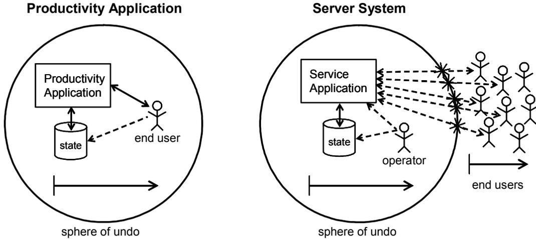
Figure 1: Spheres of Undo for productivity applications and server systems. In server systems, the undo model is complicated by the presence of end users external to the sphere of undo. While the administrator or operator can be considered to exist inside the sphere, much as the end user is in the productivity-application sphere, end users in the server case have their own timelines, independent of the timeline inside the sphere, and must therefore be kept outside of the sphere.
