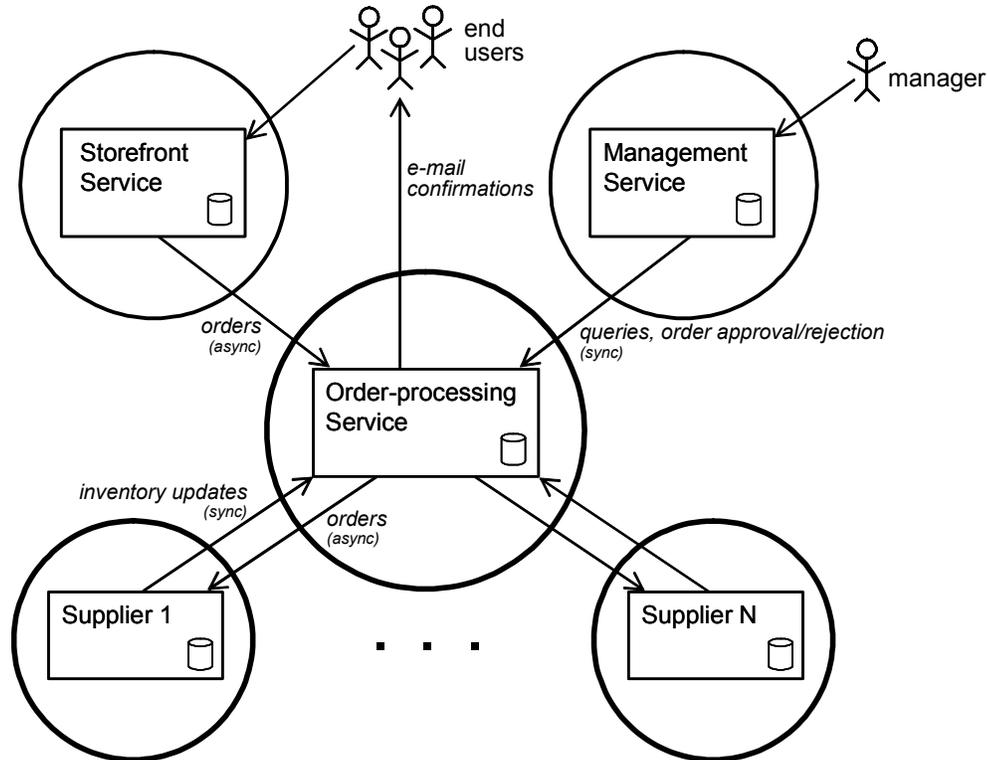
Figure 9: PetStore architecture as spheres of undo. Each subservice of the PetStore architecture naturally maps to its own sphere of undo.
