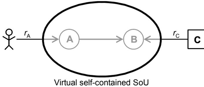
**Figure 13: Restricted model for coordinated multi-sphere undo.** The coordinated spheres A and B are treated as if they form a single larger self-contained SoU with respect to external output. The only output allowed from that virtual self-contained SoU is in response to external requests, like  $r_A$  and  $r_C$ .
