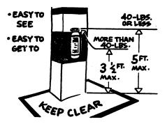
Figure 26: Placement of fire extinguishers. (NIOSH Health and Safety Guide for Foundries. April, 1976.)
