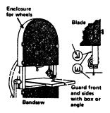
Figure 20: Band saw guarding. (NIOSH Health and Safety Guide for Foundries. April, 1976.) pusher stick must be provided and used. [8 CAC 4300(d)]
