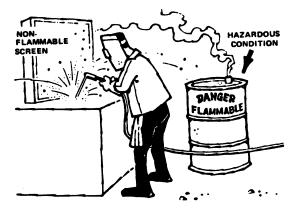
Figure 25: Flammable liquids must be stored safely. (NIOSH: Good Practices for Employees - Auto Body Repair Shops. August, 1977.) disconnected. If the work requires using a flame or other source of ignition, the vessel must be cleaned and fire tested beforehand. [8 CAC 5420(a)]
