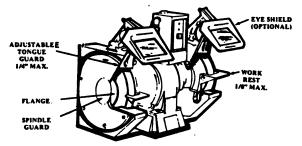
Figure 18: Grinder safety guards. (NIOSH Health and Safety Guide for Manufacturers of Lighting Fixtures.)
