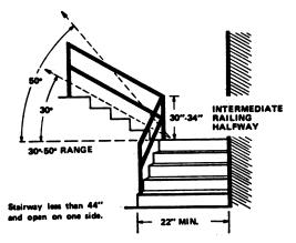
Figure 17: Specifications for industrial stairs. (NIOSH Health and Safety Guide for Foundries. April, 1976.)
