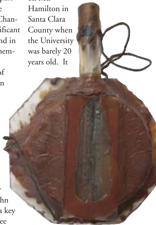
Model for Cyclotron Chamber, 1931. One of the earliest particle accelerators, built by Lawrence and a graduate student, Stanley Livingston, using shards of glass, metal, wires, and wax. Courtesy Lawrence Hall of Science.
